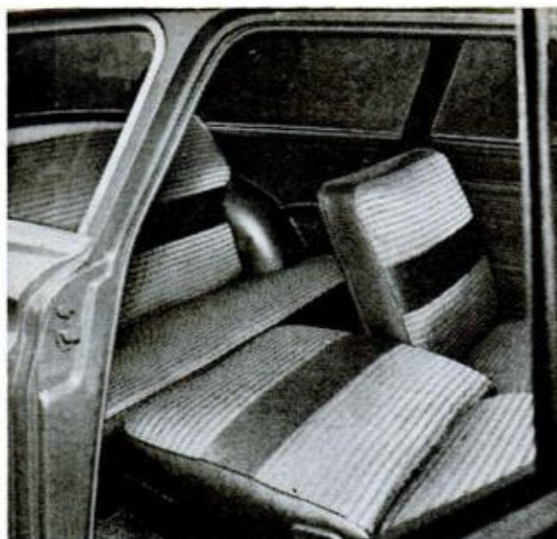
FRONT PASSENGER can relax in reclining seat; driver's seat also reclines for overnight stops on long trips
