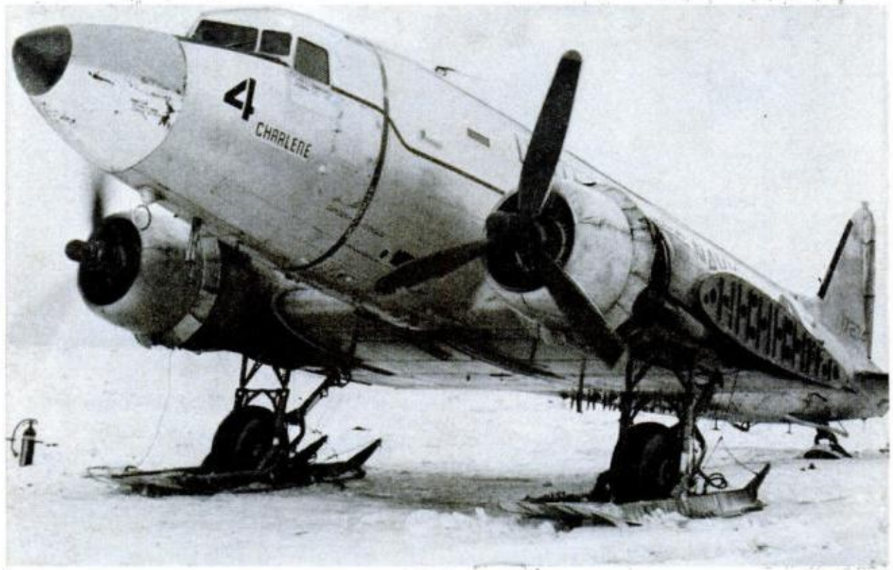
SUPER TAXICAB is used to ferry men from ships to base. It was made by clipping wings of an old, tired R4D
