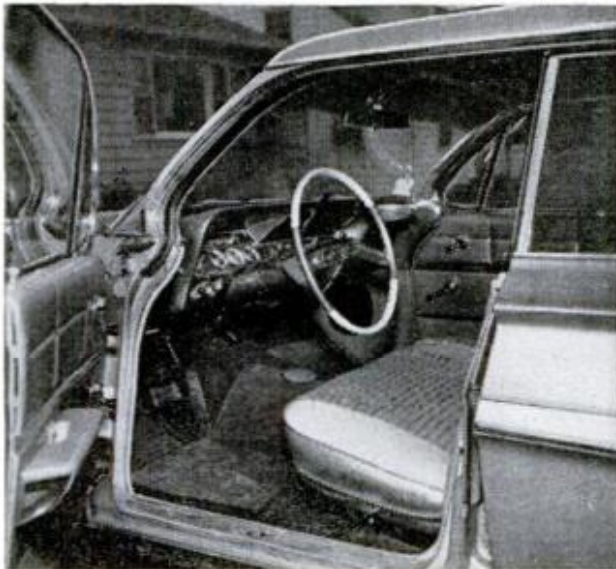
GONE IS THE DOGLEG from Chevy's front door. With this out of the way, entry or exit is much easier
