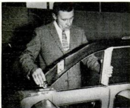
Side frames are salvaged from original top structure and covered with padding. They lock easily in place by means of fittings from kit
