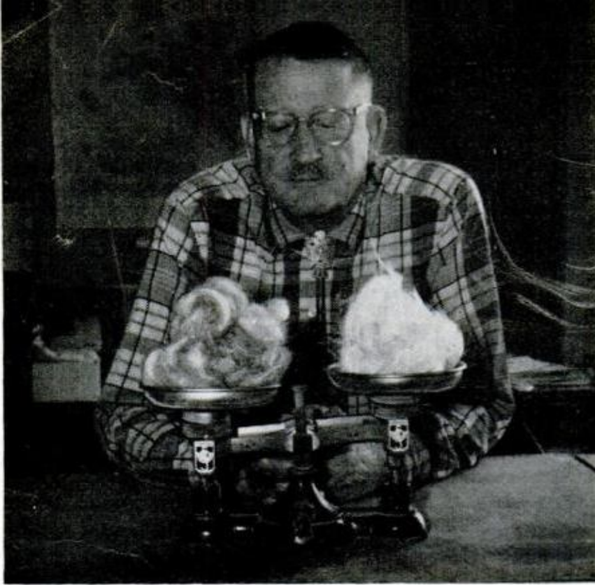
WEAPON AGAINST SMOG? Exhaust from the same car was caught in glass wool filters after it had idled one hour on regular gas, another on supplemented gas. Untreated gas caused filter at left to pick up a gram of weight. Treated gas gave off fewer unburned solids that cause smog, filter stayed white
