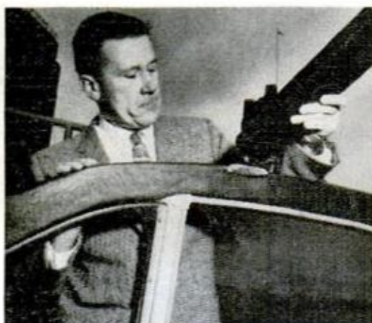
Above, inventor Joe Brodowski latches on roof bows prior to stretching vinyl-fabric top over padded framework to complete the job
