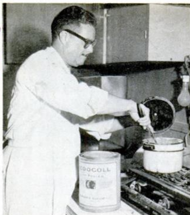
NEGACOLL PLASTIC is heated slowly in double boiler, stirring every 20 min. or so to break up any lumps
