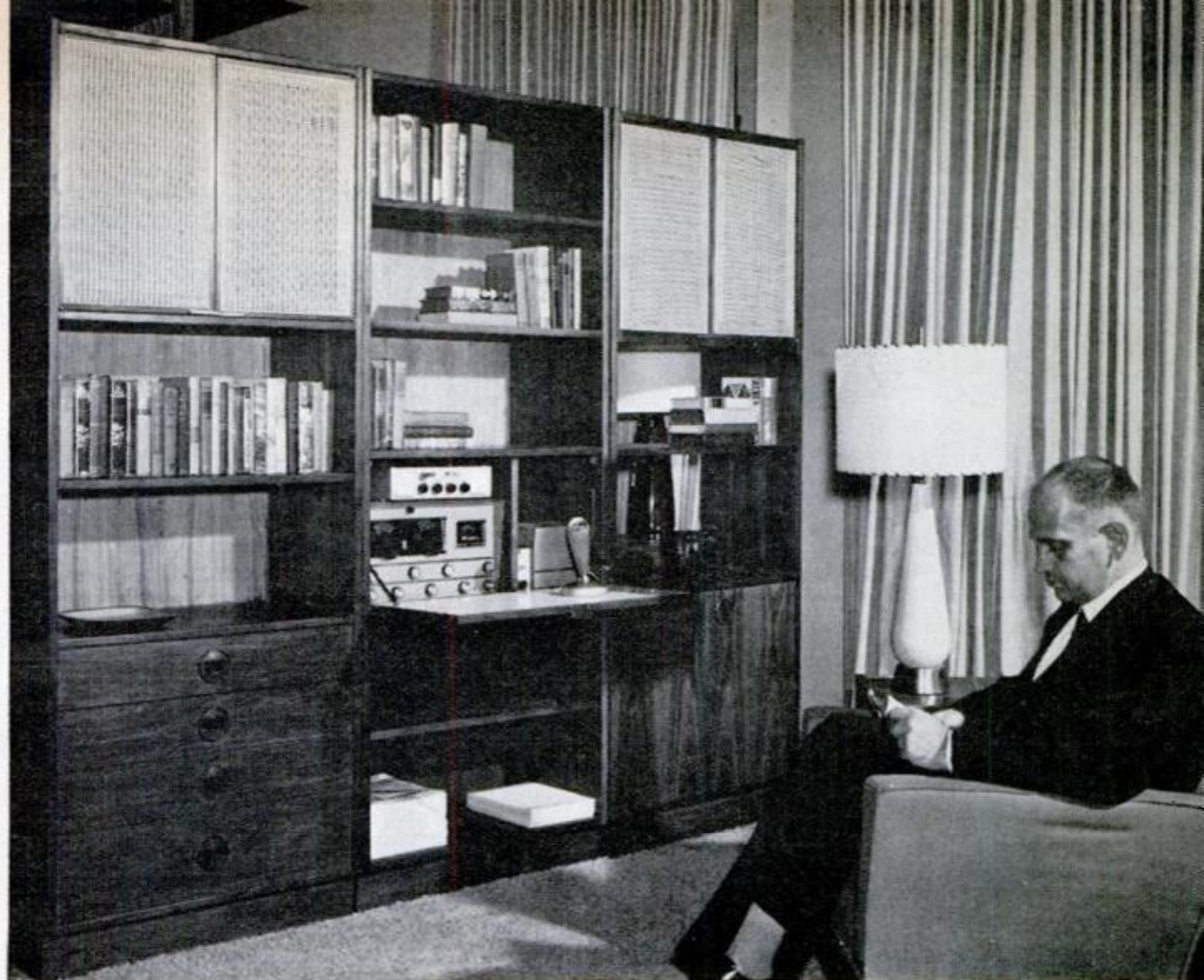
In the desk unit of this wall-divider section are the Knight-kit R-100 receiver, the Neil Beta six-meter transmitter, the Viking 6N2 converter and the Lafayette microphone—a compact, complete amateur station
