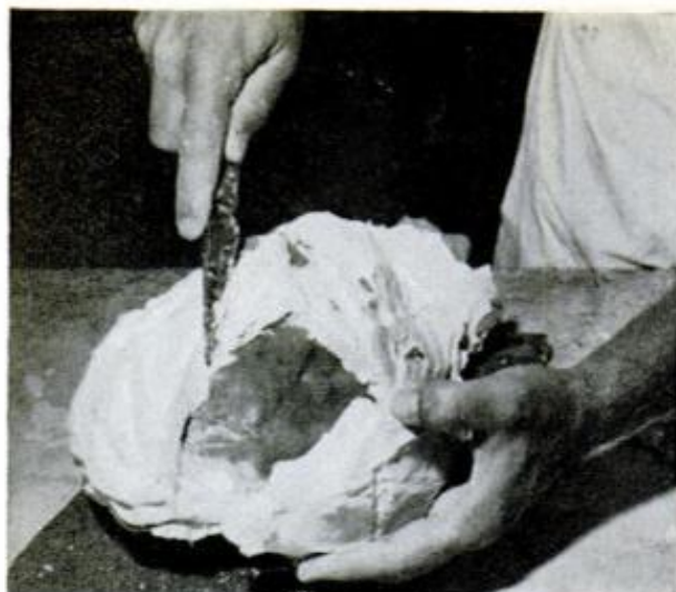
WHEN FINAL PLASTER cast hardens, matrix is turned face up on protective rubber pad and overcoating is chipped away, above. Below, plaster scored by knife tapped with hammer, falls away in big pieces
