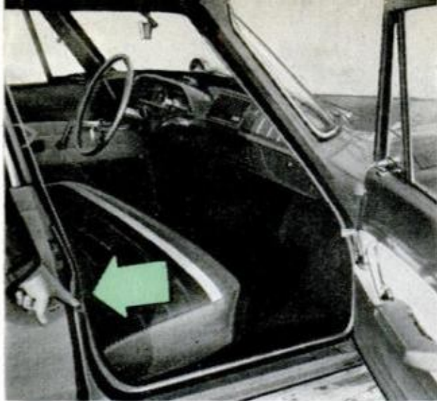
Wide front door opening provides good entry but protruding door latch (arrow) is a coat catcher
