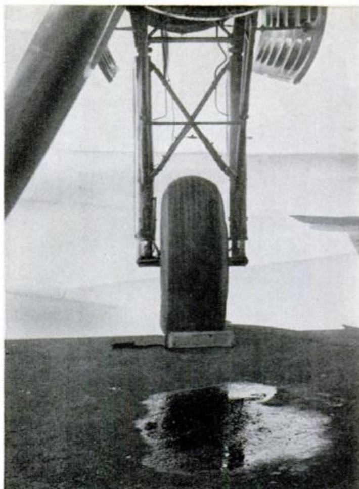
Pool of oil is sad insignia of misused aircraft, indicating poor maintenance or plane too old to fly
