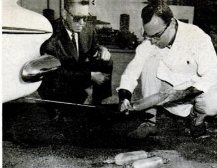
EXHAUST FUMES are drawn off and bottled so they can be analyzed for content of smog-producing particles of hydrocarbon
