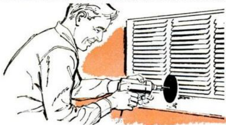
SANDING DISK chucked in electric drill is best way to clean metal surfaces such as you find on window air conditioner
