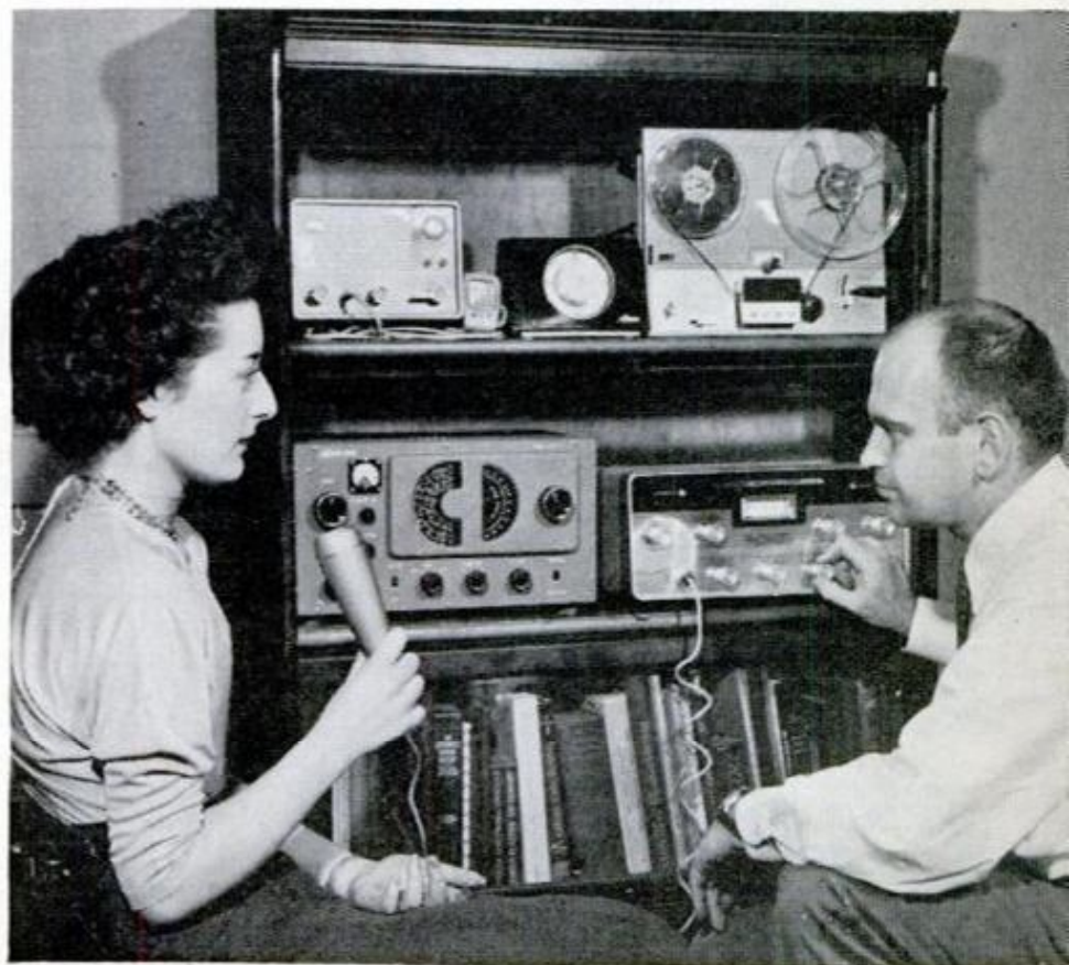
In the desk unit of this wall-divider section are the Knight-kit R-100 receiver, the Neil Beta six-meter transmitter, the Viking 6N2 converter and the Lafayette microphone—a compact, complete amateur station
