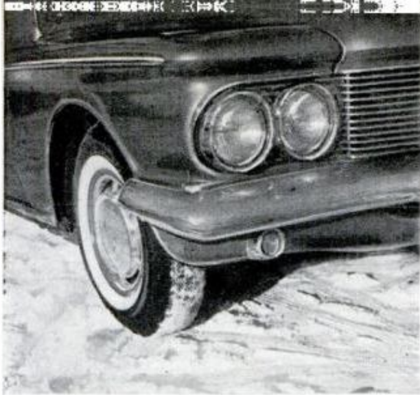
Designers of handsome front end should have moved parking lamps away from this mud-catching location
