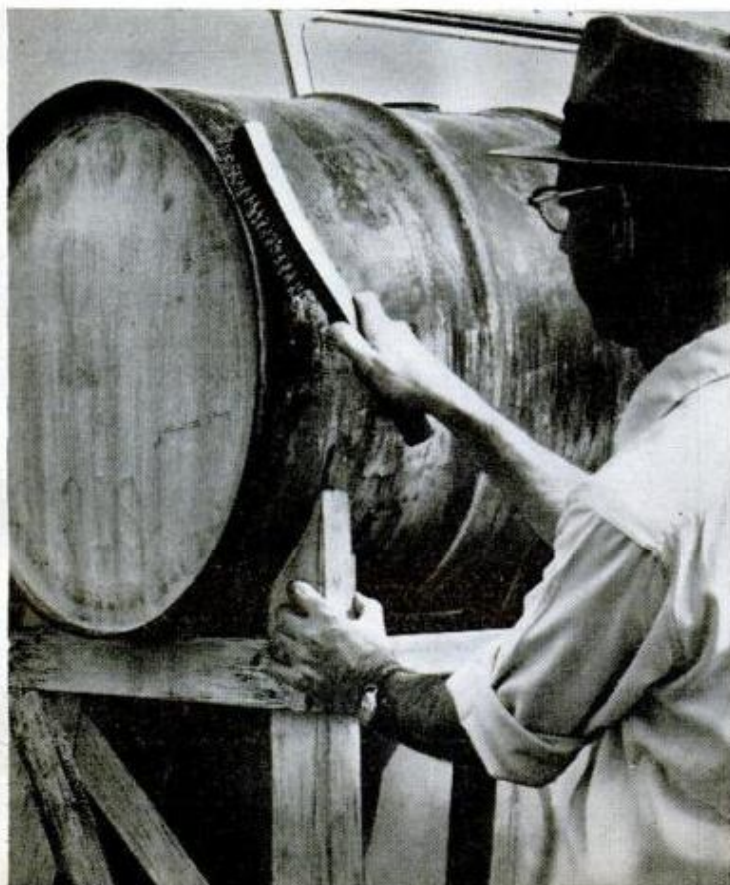
SANDING DISK chucked in electric drill is best way to clean metal surfaces such as you find on window air conditioner
