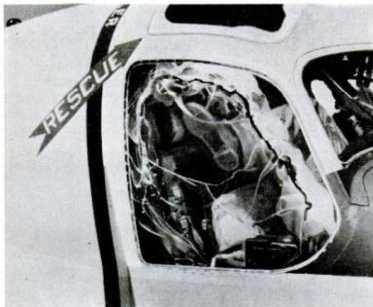
After breaking through safety glass with knife, pilot pushes window out with feet. Total time: one minute and 50 seconds
