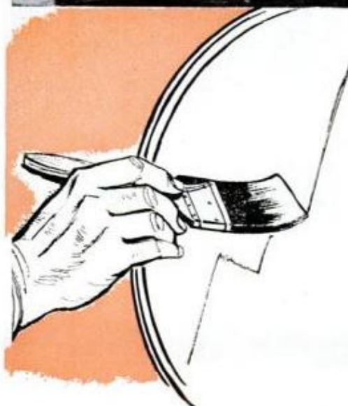
FUEL-OIL TANK should be thoroughly cleaned with wire brush before applying a rust-resistant paint. Use a strong detergent to remove oil spots from the surface of tank
