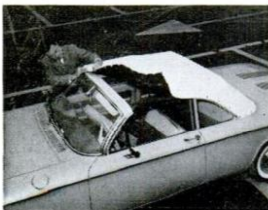
Below, one person alone can easily snap the top in place for a wind and watertight fit
