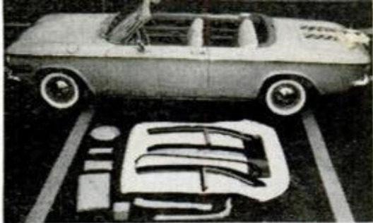
Above, Corvair coupe converted. Bows and side pieces rest on the new vinyl top surrounded by packages of parts comprising the kit
