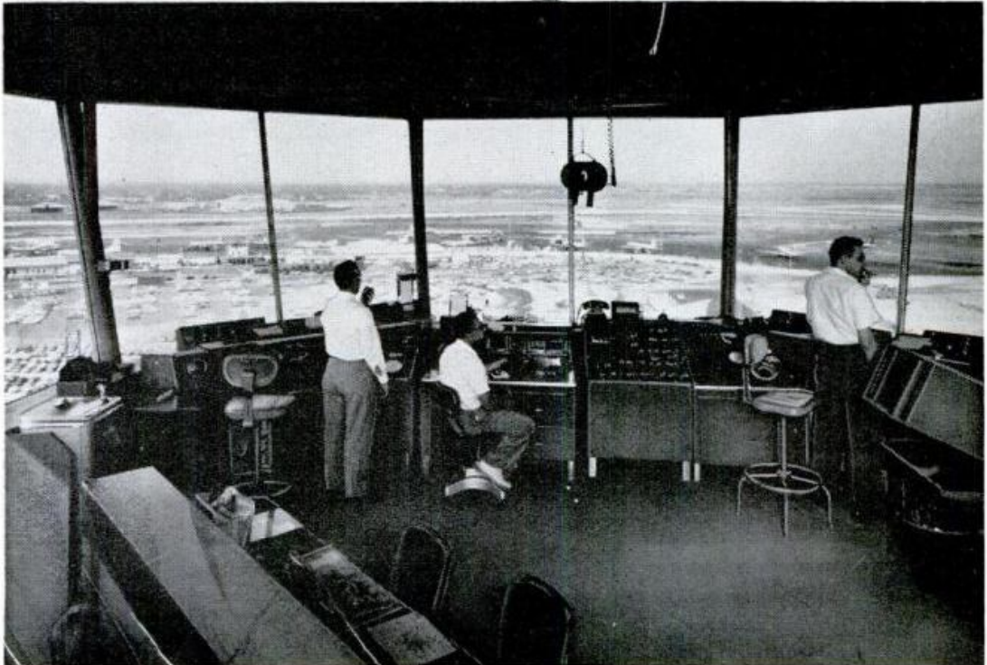
View from the tower, facing the runway and taxiway system. The five long runways stretch as far as 14,600 feet. One runway, lit with flush-set fixtures, has taxiway exits taking planes from runway at 60 knots
