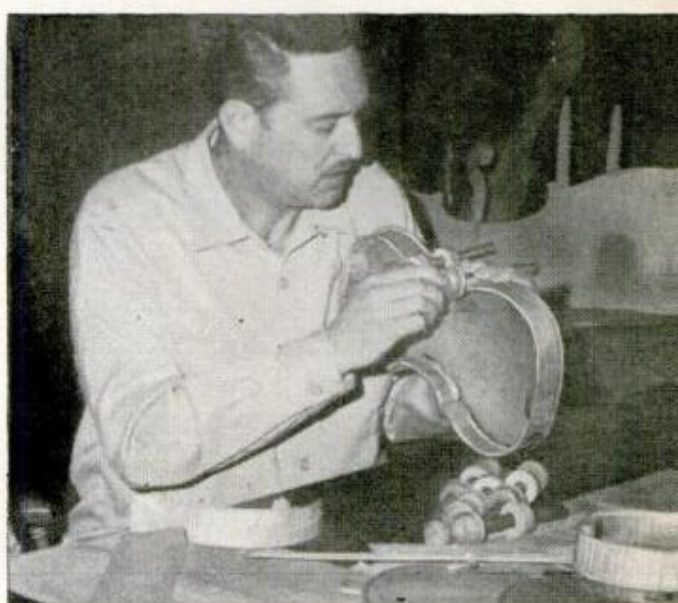
4. Finished ribs are glued to back. Ribs, back, neck and sides of violin are made of maple imported from Carthaginian Alps in Central Europe
