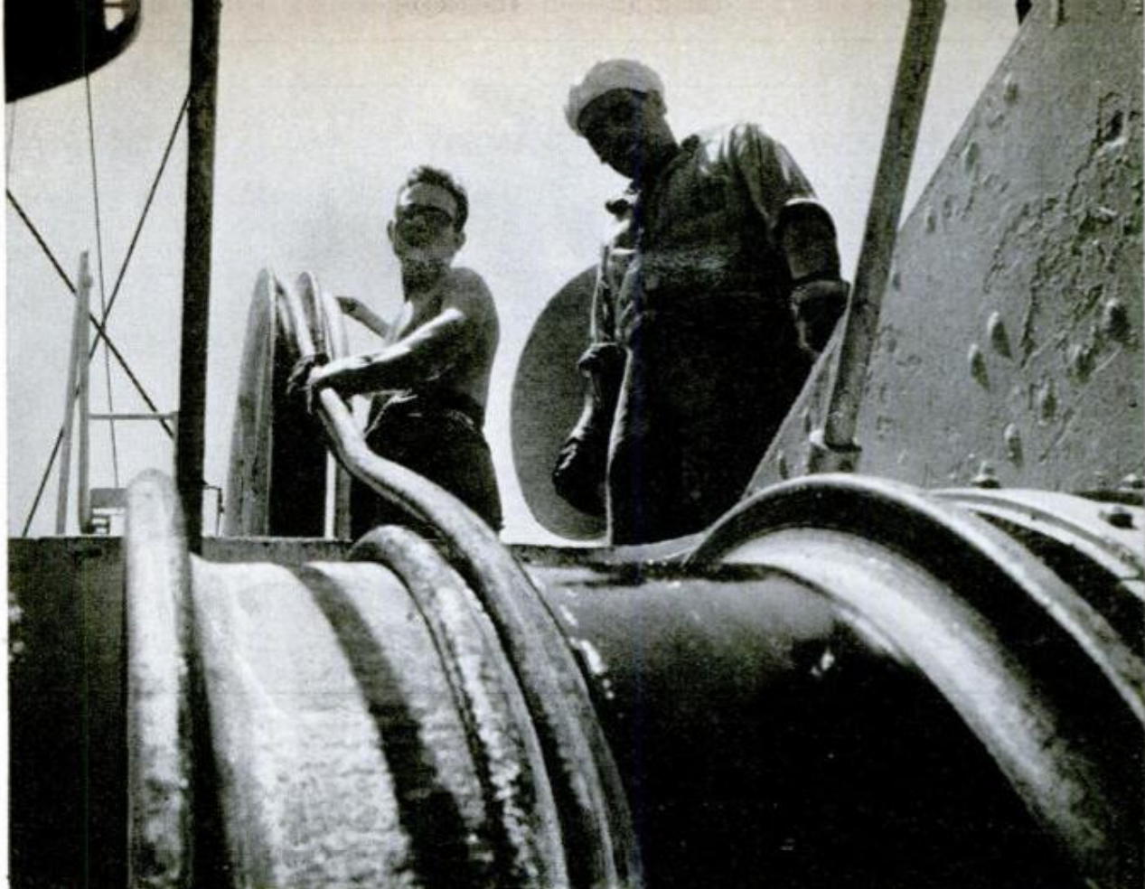
Tricky job of lifting and lowering the cable without changing the tension is helped by this tension drum. Using stripping disks to keep all the wires separated and in order, all hands fall to stripping a new section
