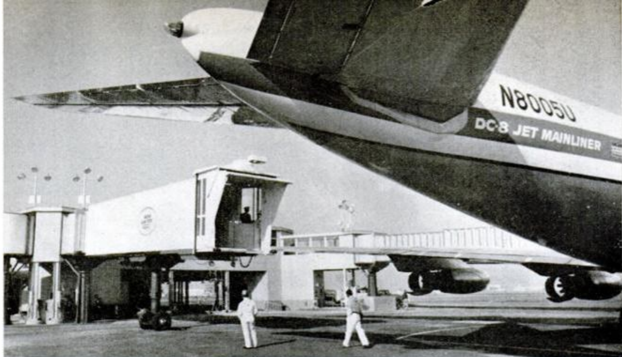
Covered bridge called Jetway is extended from the United Air Lines terminal to jet's door in less than a minute. It is driven by a passenger agent in outboard cab section, and can be raised or lowered
