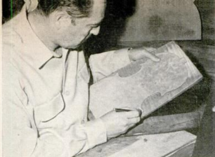
1. Back is foundation of violin and its most important piece, giving violin its brilliance of tone. Roberds uses template to trace its shape in block of maple
