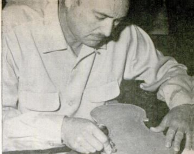
2. Back is arched out with woodworking tools, then planed to shape with special tools Roberds made himself. Wood is all imported from Europe
