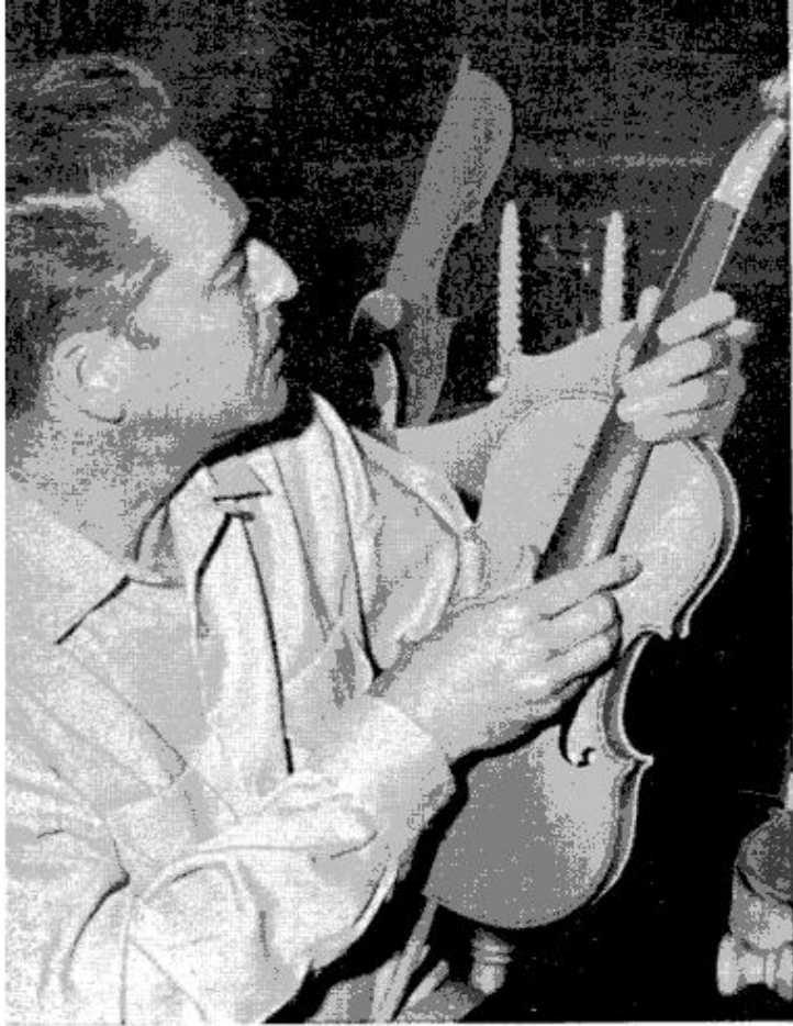
7. Roberds adjusts ebony fingerboard on violin. Pegs which stretch four strings to give proper tune are made of rosewood or boxwood. Finished violin is given six to eight coats of varnish. First, oil varnish filler is used to fill pores and make wood sparkle. After a week, a second coat is applied. Then a week separates each new coat of varnish
