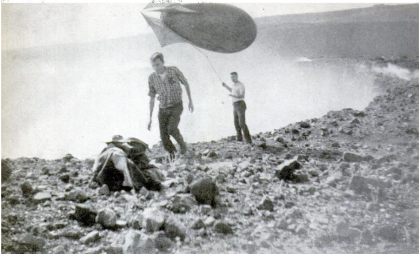
Into the air: Observatory scientists often have to improvise. To get gas samples free of contamination, they sent a balloon and sampling flask over this smoking pit. The balloon crashed. Pit is 3000 feet across
