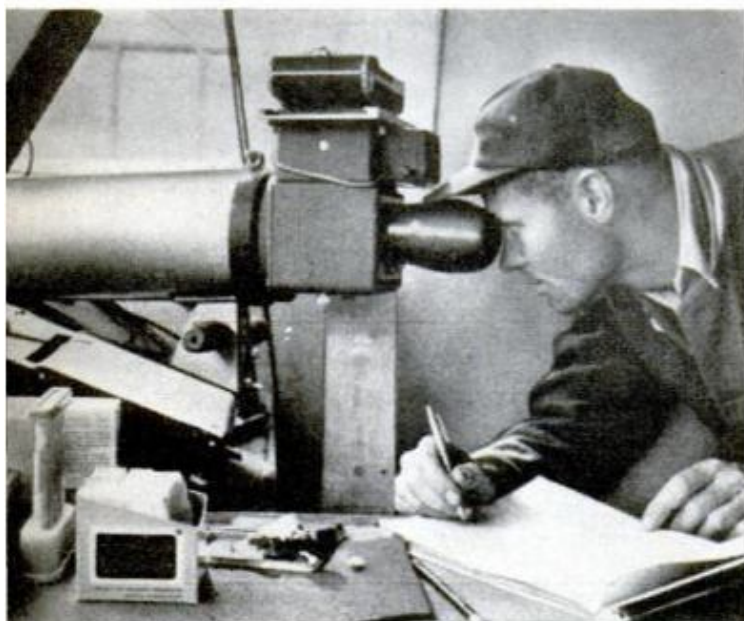
Polaroid camera, mounted on radar set, gives immediate picture at time of shot. Below, firing of shots was controlled from cabin of river boat
