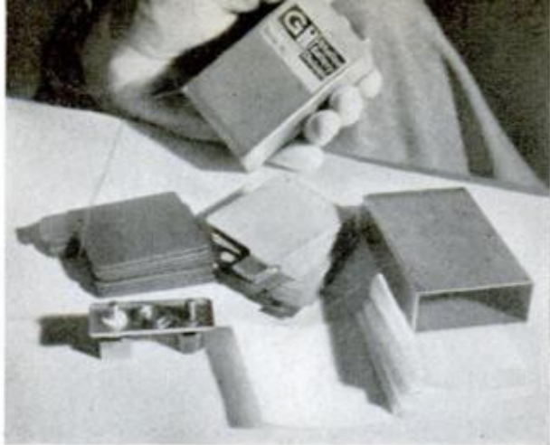
COMPONENTS of the sealed battery are the welded steel case, nickel-oxide (dark) plates, cadmium (light) plates, special-alloy cover with terminal studs and separator of synthetic fabric. Dr. Robert Shair (right) shows how the separator weaves between plates
