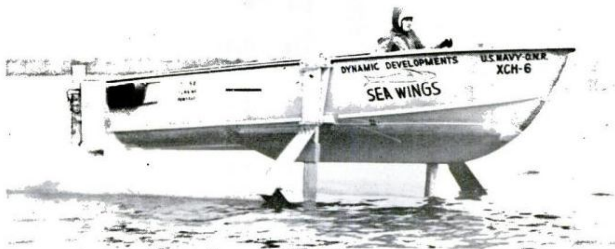
Sea Wings, above, Grumman's 23-foot test boat for the Office of Naval Research, turns in 70 miles an hour. Italian Freccia del Sole, below, does 45 carrying 75 passengers across the Strait of Messina to Sicily
