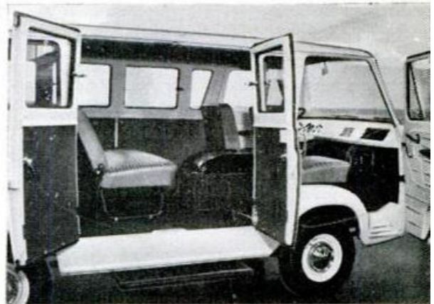
Econoline's engine box necessitates locating the second and third seats nearer to the rear of body
