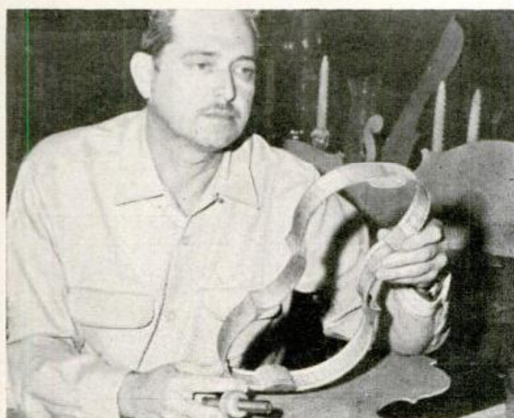
3. Ribs are made from six strips of maple, planed down to 1-mm. thickness and bent and glued to corner and end blocks. Ribs are lined for additional strength
