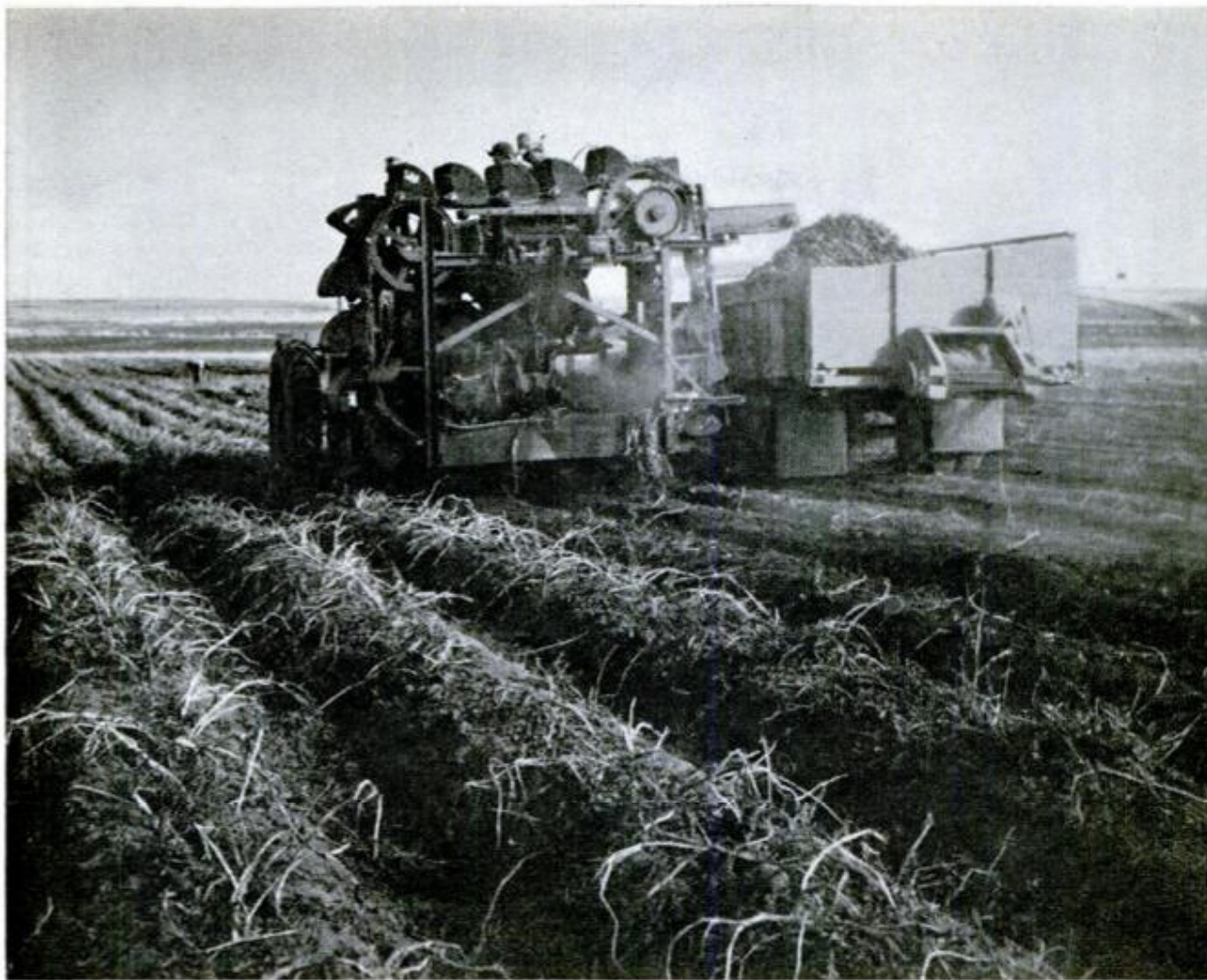
Moving along with a truck, a combine digs potatoes, frees them of debris and dumps them into rubberized bed
