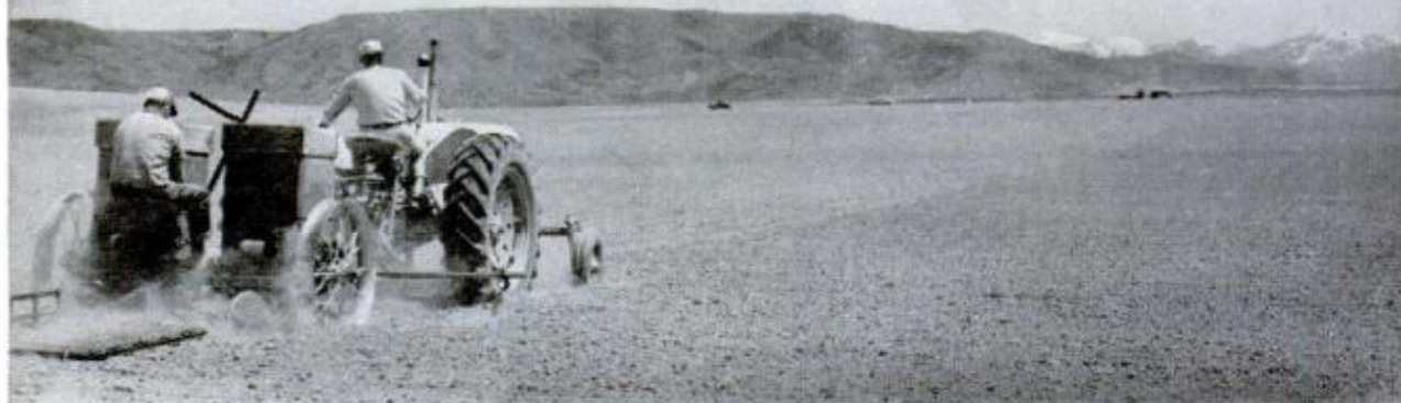
Rolling across an Idaho field, a tractor-drawn mechanical planter drops seed potatoes, covers them with dirt
