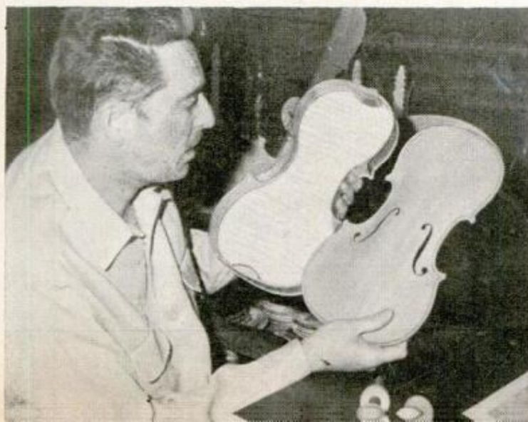
5. Front, or top, of violin is made of spruce imported from Austrian Alps. Since spruce cracks easily, top is glued on very lightly so that it can be replaced
