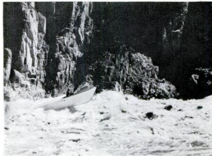
Big water flexed its muscles and tossed this boat clear out of the river. The tough plastic hull survived, and the jet system, all inside the hull, wasn't damaged. All hands turned to, shoved it back into the current and drove it away. Below, another boat hangs up in the rapids
