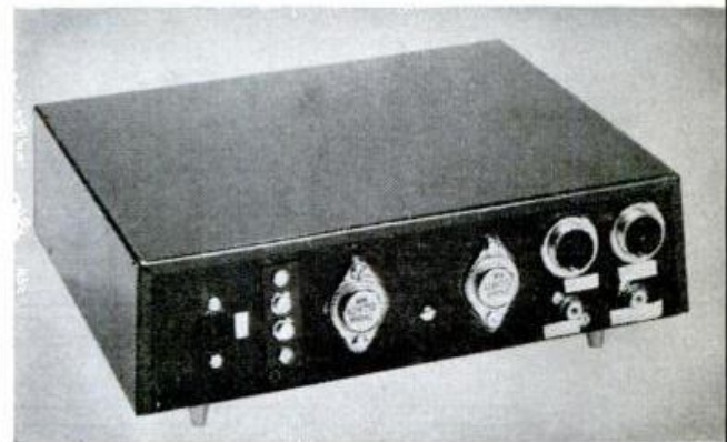
Above, three views of amplifier. Note transistor mounting on back of chassis pan. Transistor heat is drawn off by chassis which serves as heat sink. Below, proper method of assembling transistor and hardware provided with transistor, to the chassis
