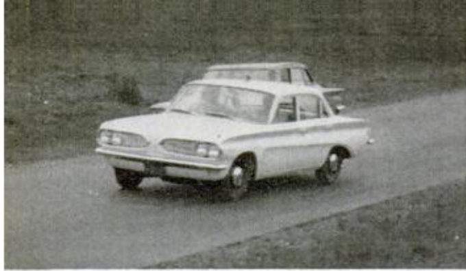
Stick-shift Tempest made 0 to 60 m.p.h. in 15.7 sec. Good passing punch logs 50-70 m.p.h. in 9.5 sec., 60-80 m.p.h. in 10 sec. Top speed, just under 90
