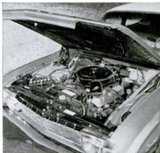
Plugs, carburetor, distributor and other accessories are easy to reach on the Buick Special. Generator is placed low on right side
