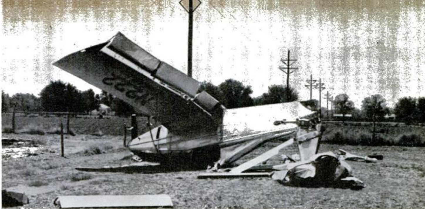
Crop duster (left) actually did crash, but pilot miraculously escaped with only a bruised thumb. Wreckage (above) shows the plane's cockpit area still intact. Plane was built to AvCIR crash-survival specifications
