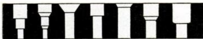
19 COUNTERSINKS PRODUCED WITH VARIOUS TYPES OF STEP DRILLS
