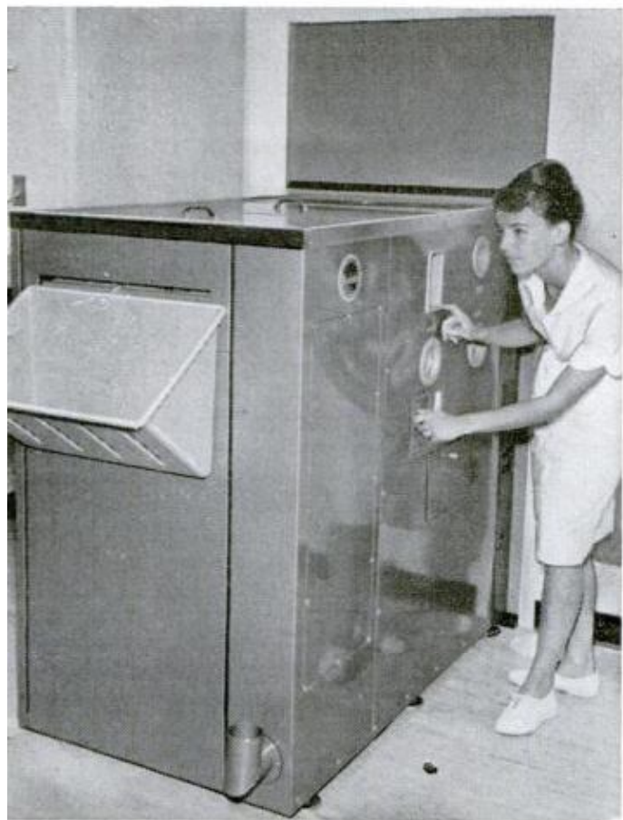
X-ray film is processed in seven minutes in this developer. Older method took a minimum of 30 minutes
