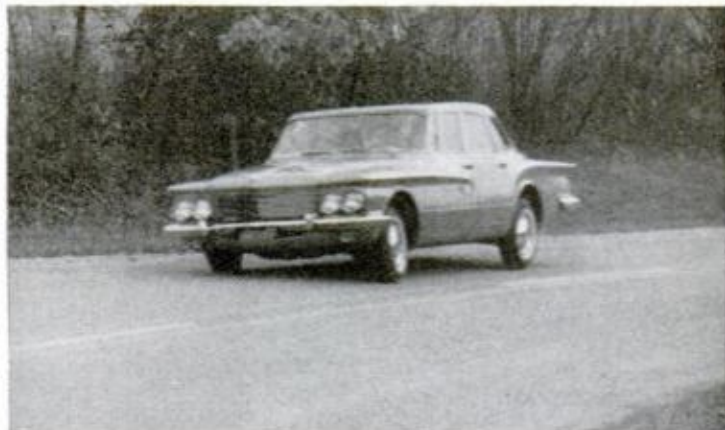
Lancer steers easily, precisely; rolls least of all four in cornering; hugs the curves nicely and stays on course better when the going starts getting rough
