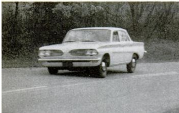
Tempest handles well at normal speeds. Steering—precise, though slow. Corners hard under light load, rear swing-axles "camber"—rear end slides out
