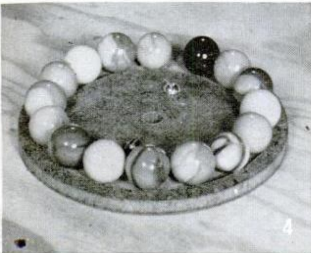
ABOVE, FAUCET WASHERS provide ready-made rollers to support rotating top. Below, 16 glass marbles are held between grooved hardboard race by pivot
