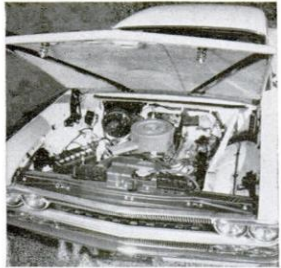
Even the compact engine compartment of the Olds F-85 seems huge as it surrounds the neatly designed, lightweight aluminum V-8
