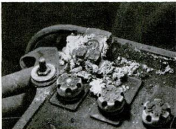
Overcharged battery—internal heat forces acid out
