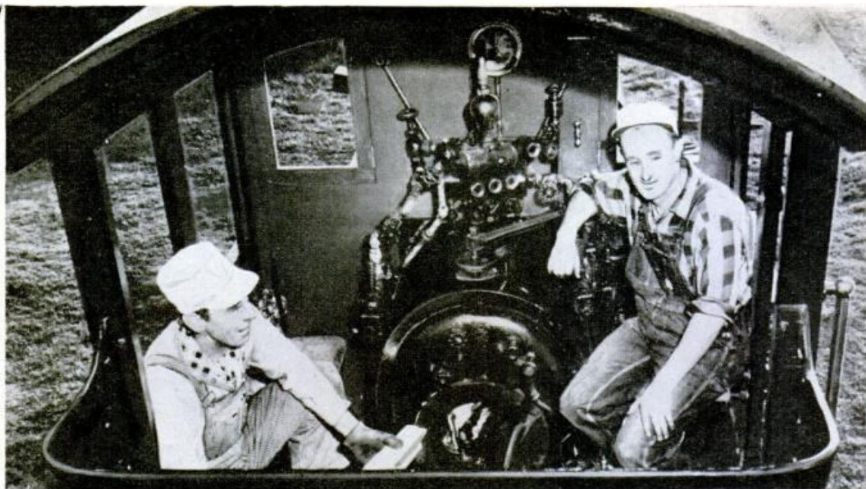
Entire cab had to be rebuilt by hand, since most of it had eroded away. Sorensen (right) took special night class in woodworking to learn how. Most of the engine's instruments and fittings had to be replaced
