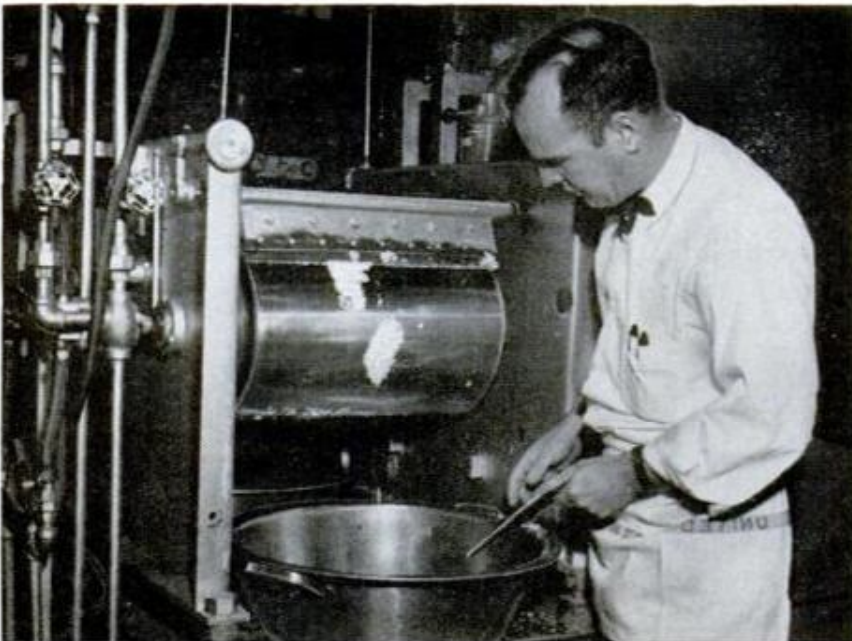
Drum dryer is used by a Department of Agriculture researcher in studies that seek to develop an improved, dehydrated mashed potato—another "instant" food
