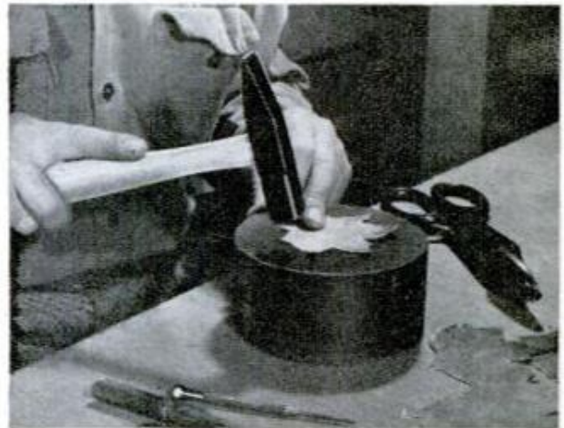
LEAVES ARE FLATTENED on a solid surface by tapping curled edges with hammer. Then edges are filed smooth
