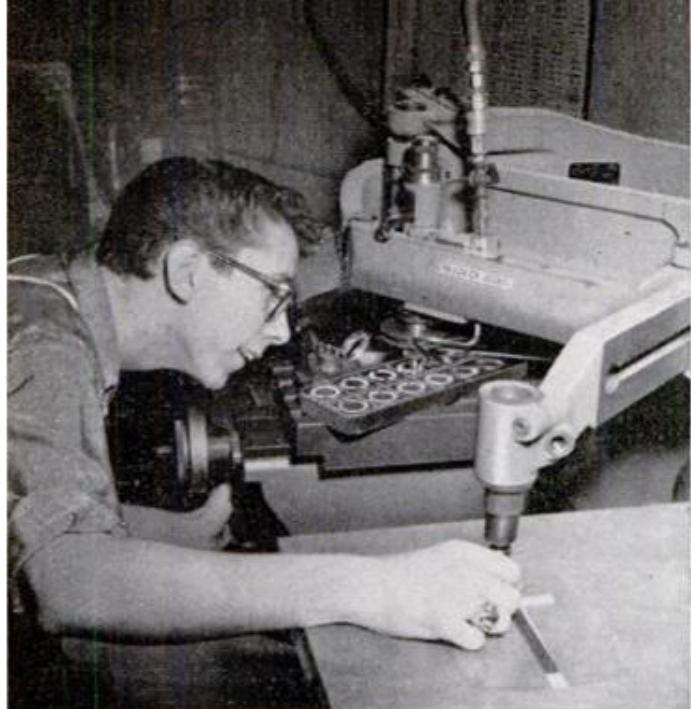
3. Pilot models are then broken down to provide patterns for molds of the many parts which go into kits
