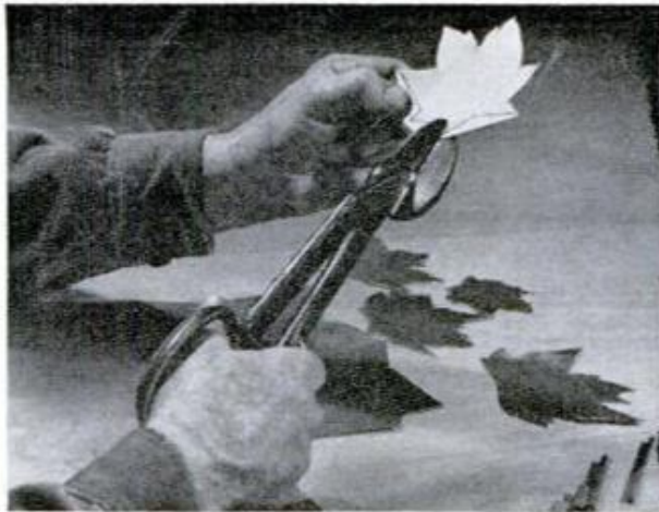
EACH LEAF PATTERN is first scribed on 24-ga. sheet brass and the outline carefully cut with duckbill snips
