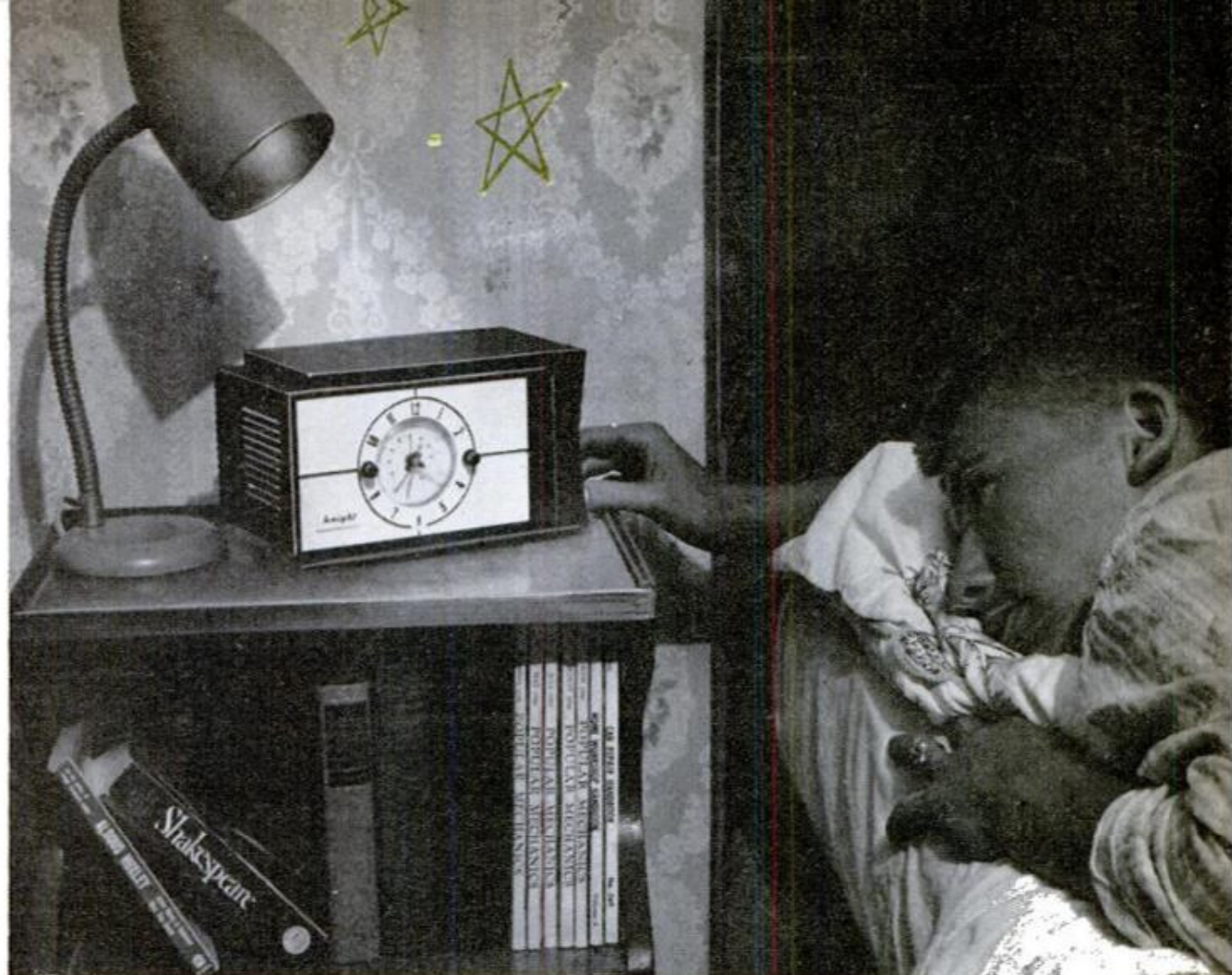
Clock radio kit can be preset to shut off radio after user falls asleep to music, start radio in morning. After 10 minutes of radio, an alarm buzzer sounds. Rear outlet can turn on electric coffee percolator
