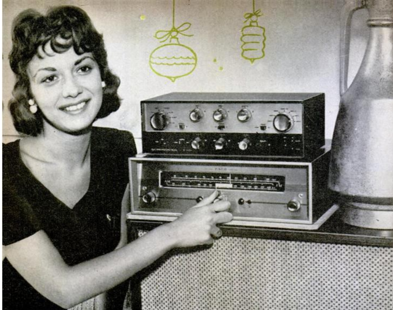
Component installation uses stereo preamplifier atop FM-AM tuner. Combination rests on one of the two matched loudspeaker systems. Tuner can be purchased as a kit, semikit, or fully wired and tested
