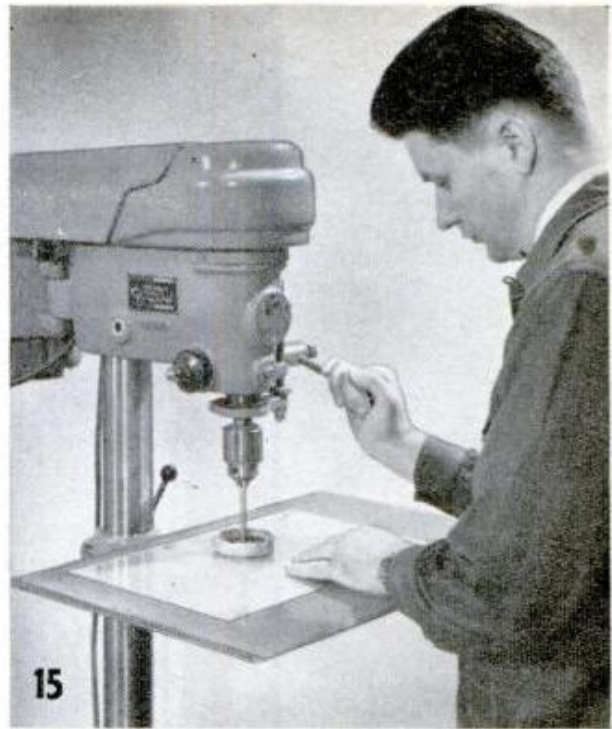
DRILLING HOLES through glass is done in a drill press, using suitable drill and mixture of abrasive and oil. Use slowest speed, lift drill frequently
