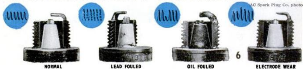
CONDITION OF USED SPARK PLUGS often provides clues leading to source of motor malfunctioning. Wave patterns in blue dots indicate engine performance as observed on screen of ACilloscope, spark-plug analyzer
