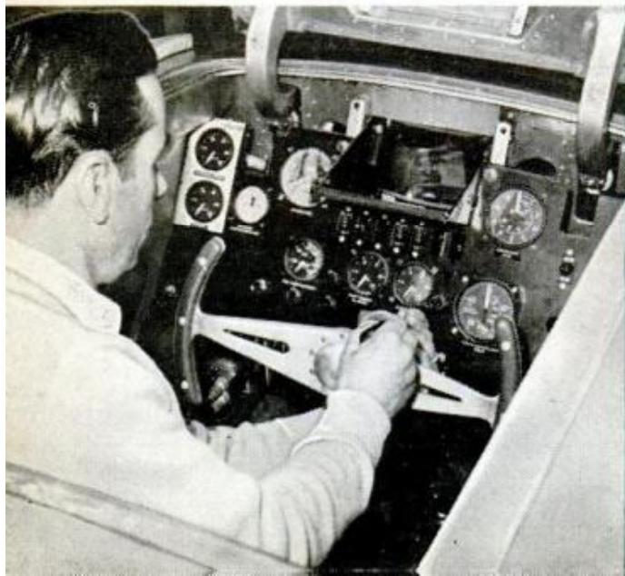
Optical system projects readings of Bluebird's speedometer and accelerometer as images that appear to be on track surface 100 yards ahead of car. Driver sees figures without moving eyes or changing their focus
