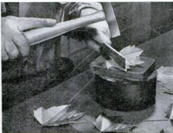
EMBOSSING OF LEAVES is done by striking knife-edge metal sharply while leaf is on hardwood block
