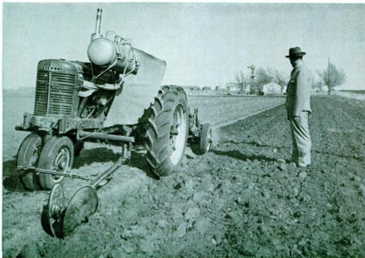
Guide disks follow furrow; if they leave furrow, an automatic ignition cutoff switch will stop tractor
