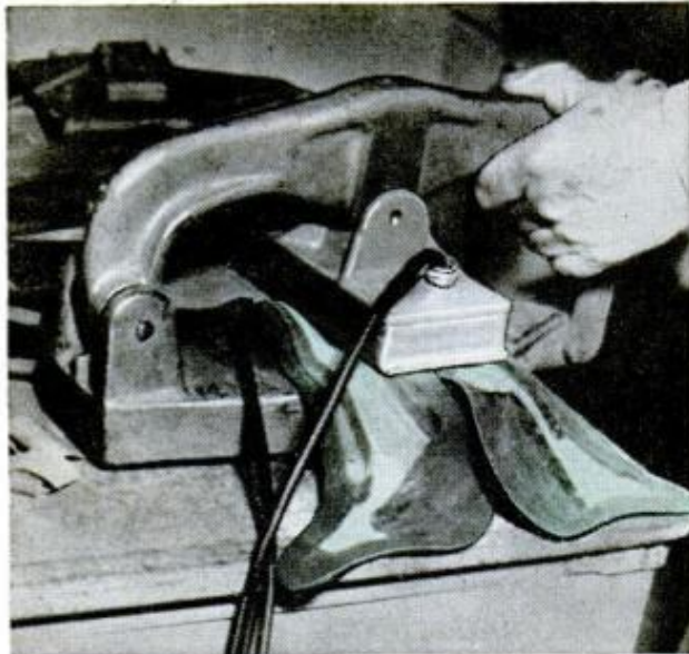
Vulcanizing takes about 15 minutes, and welds the nine cut-out sections into airtight shape. A short piece of quarter-inch tubing forms a simple valve
