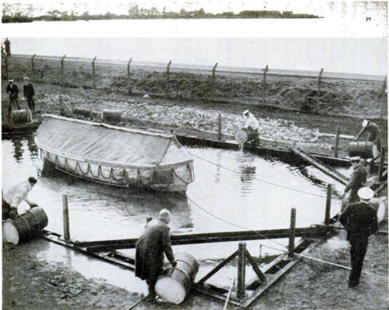
Duplicating the conditions around a burning tanker, personnel of the British Navy Damage Control School pour kerosene into the test tank. The volatile fuel produces a towering inferno below, a real trial by fire
