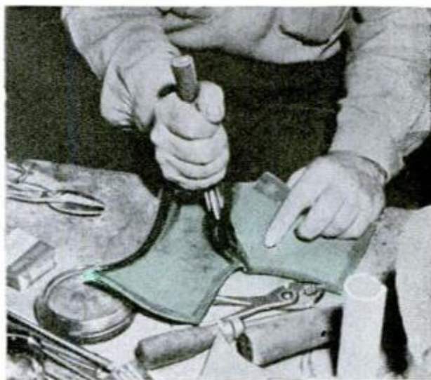
Step two—seam edges are buffed and spread with solvent, then vulcanized with thin raw rubber strips
