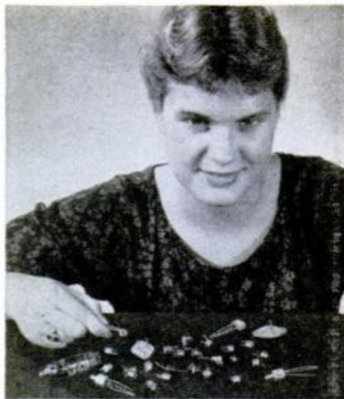
The transistors and diodes combined use less space than the only tube in the set
