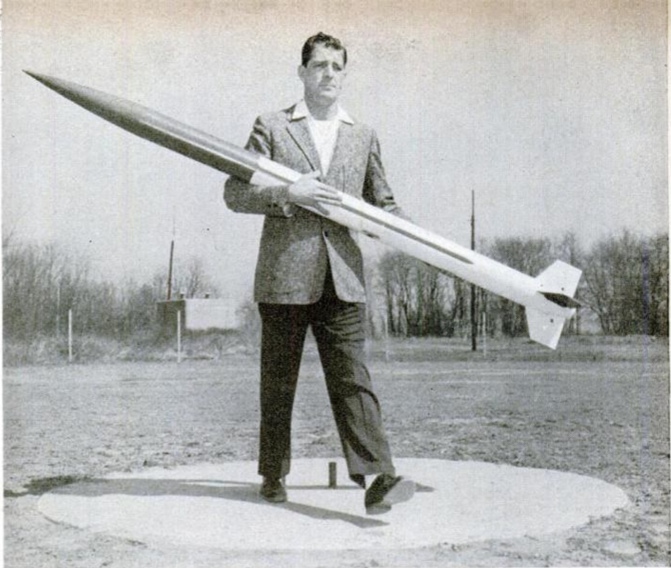
Atlantic Research Corporation builds the Arcas, a solid-propellant rocket, for low-cost experimental work
