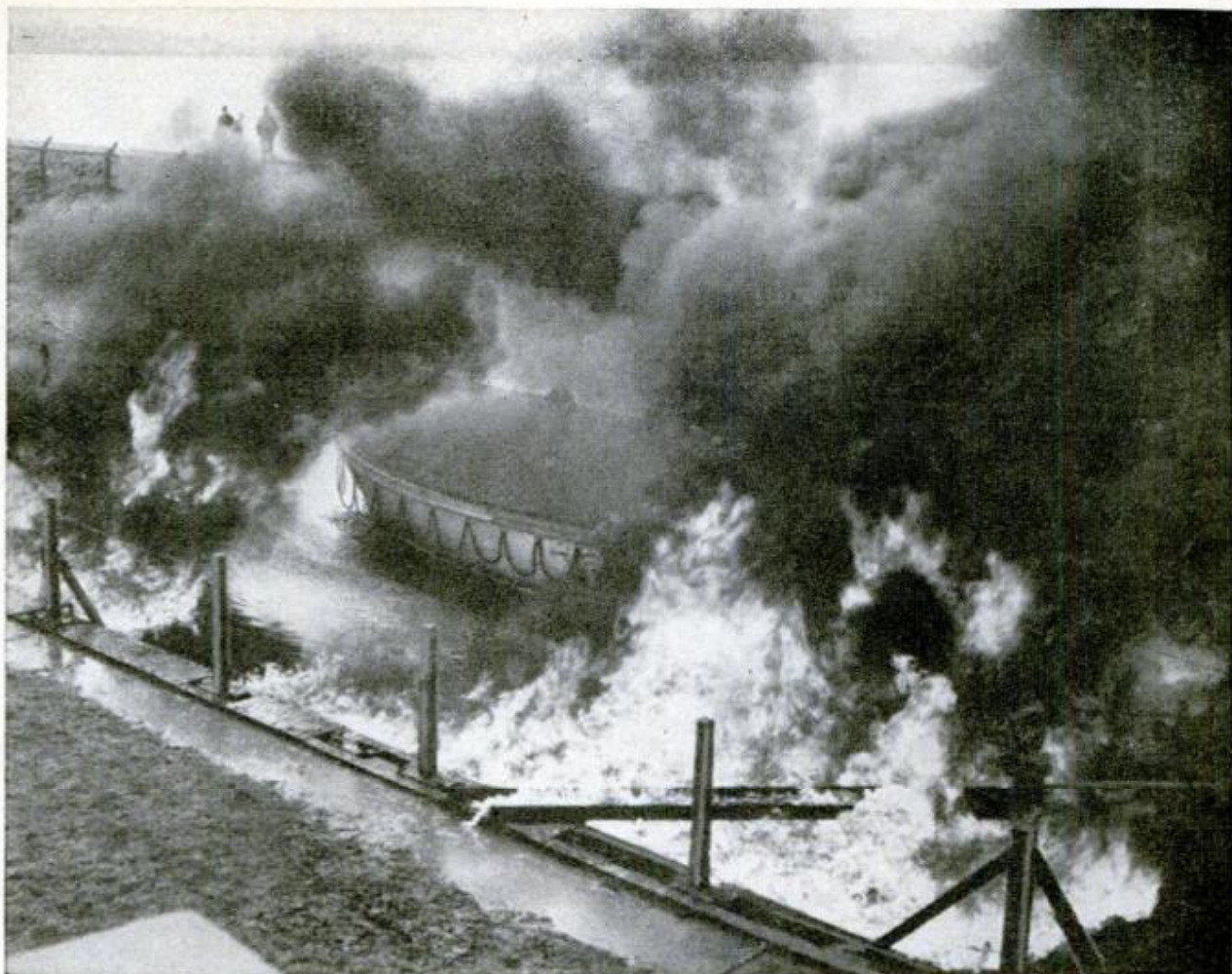
Barely visible through the smoke and flame, this aluminum lifeboat and its wet canvas cover withstood four minutes of terrible heat and emerged intact and floating with the only damage a hole in the bow
