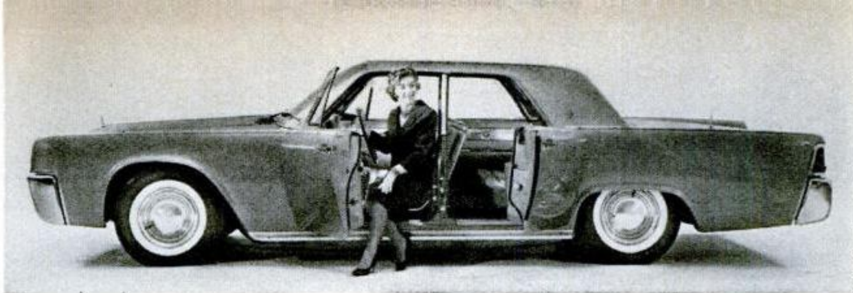
Profile of the '61 Lincoln Continental, above, shows its long hood, and deck contrasted to short roof area or "greenhouse." Rear view, below, left, has T-Bird look. Instrument panel, glove box, right, are wood
