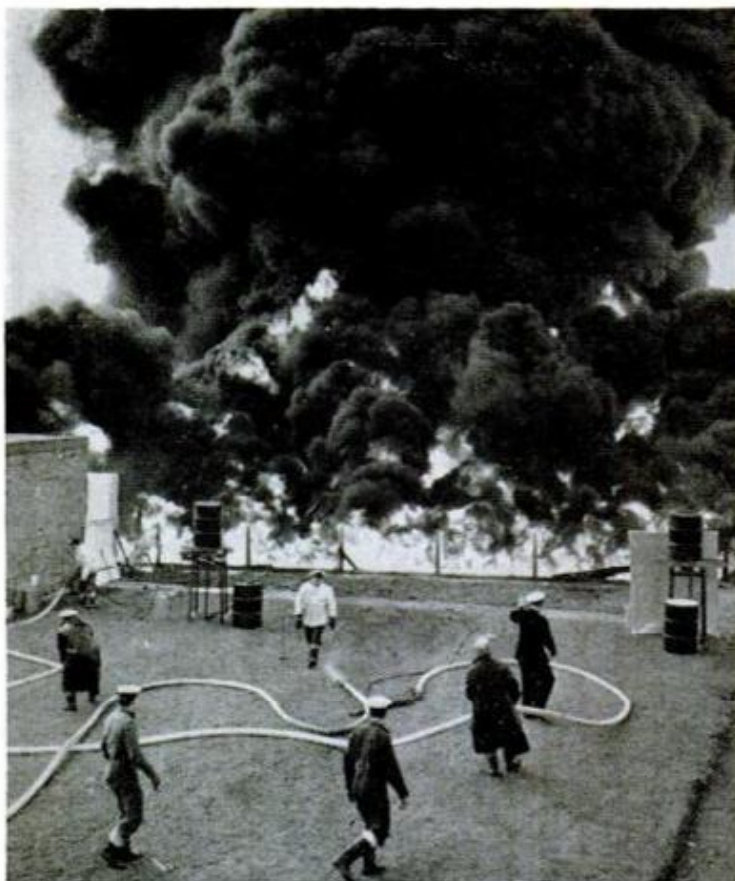
Duplicating the conditions around a burning tanker, personnel of the British Navy Damage Control School pour kerosene into the test tank. The volatile fuel produces a towering inferno below, a real trial by fire
