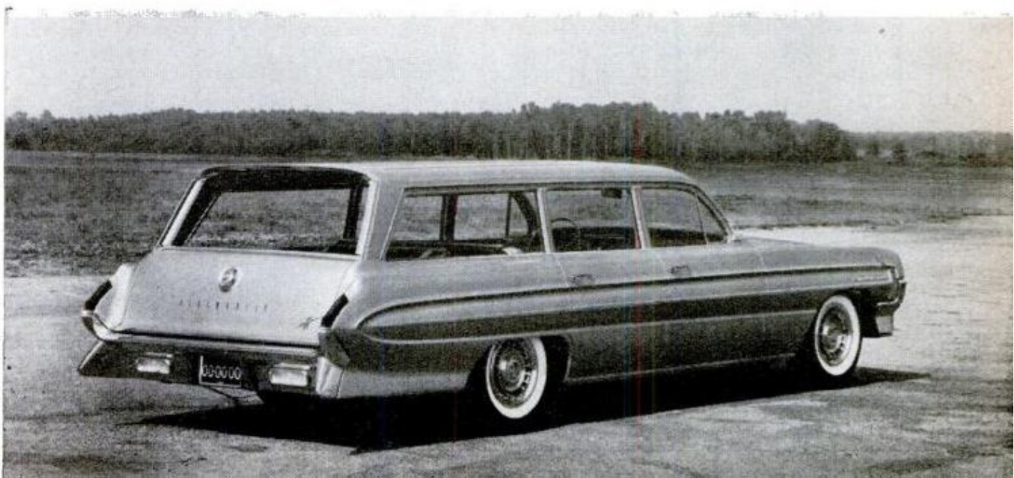
Rear treatment, above, shows down-curve of wide trunk lid on '61 Olds. Trunk has much more usable space than in previous models. Four-door station wagon, below, can be had with two or three seats
