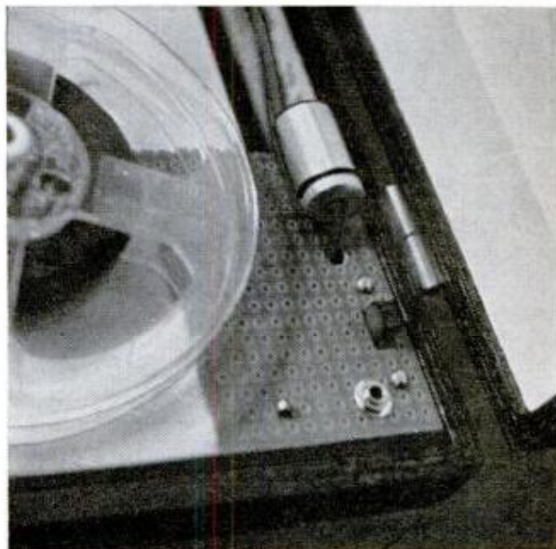
New control board is mounted to the top of tape recorder. Controls are accessible but out of the way
