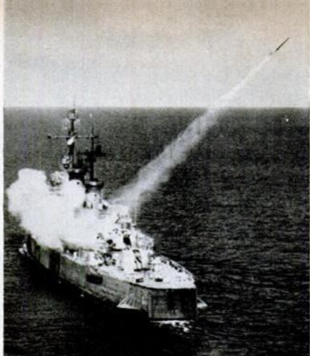
Fifteen-foot ASROC, with torpedo payload, is ready for loading into launcher aboard sub-chaser (left). At right, combination missile-torpedo is fired in tests off Florida Keys. Missile weighs 1000 pounds
