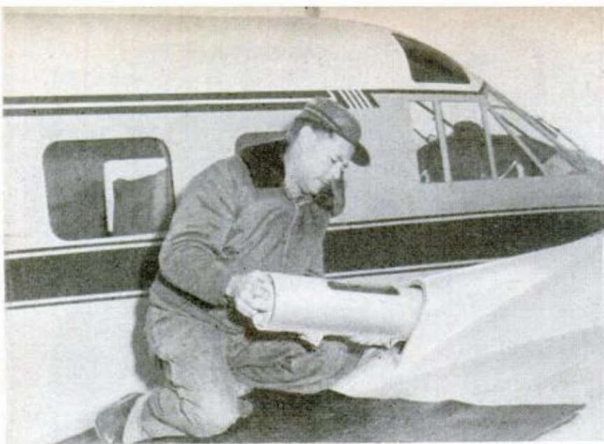
Two Aerojet Junior JATO units, in nacelles of Beechcraft Super 18 executive plane, yield 200 horsepower for 15 seconds
