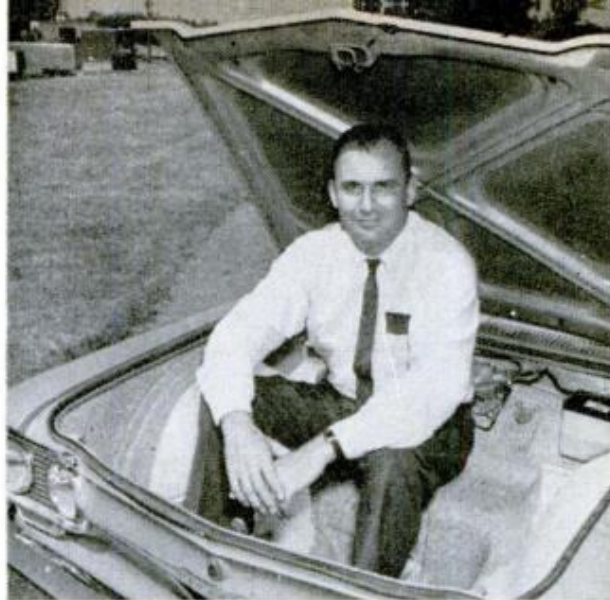
With tire removed and gas tank reshaped, Corvair's front trunk becomes much larger and more usable
