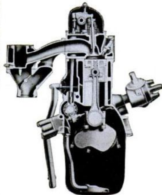
The new Lark two-door wagon, above, is one-inch lower, looks longer due to raised side trim. Regal hard-top, below, in profile shows new, flatter hood and rear deck. Cutaway, right, shows Lark's new OHV Six
