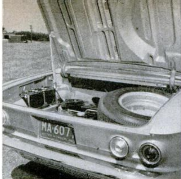
Relocating tire in engine compartment was made possible by eliminating large, central air cleaner
