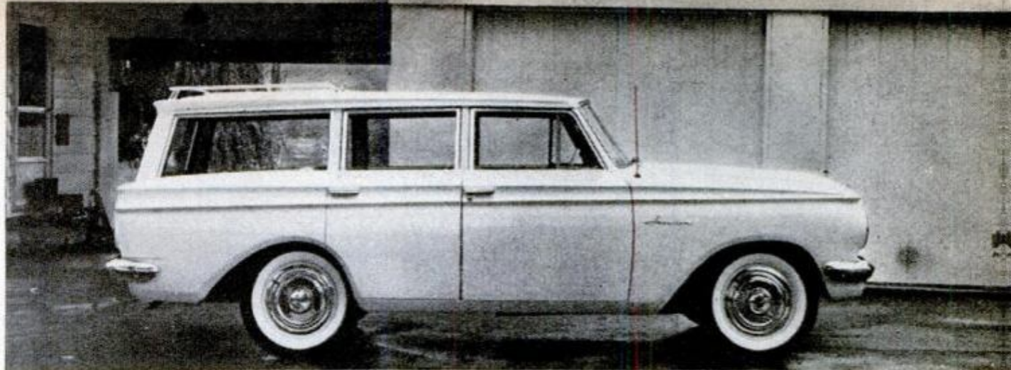
Rambler American four-door station wagon, a new body type for 1961, packs a lot of space on its 100-inch-wheelbase chassis. Area of glass and size of rear opening have been much increased for '61
