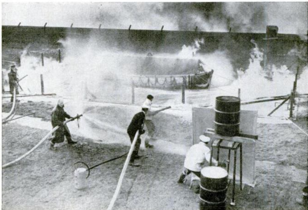
Barely visible through the smoke and flame, this aluminum lifeboat and its wet canvas cover withstood four minutes of terrible heat and emerged intact and floating with the only damage a hole in the bow
