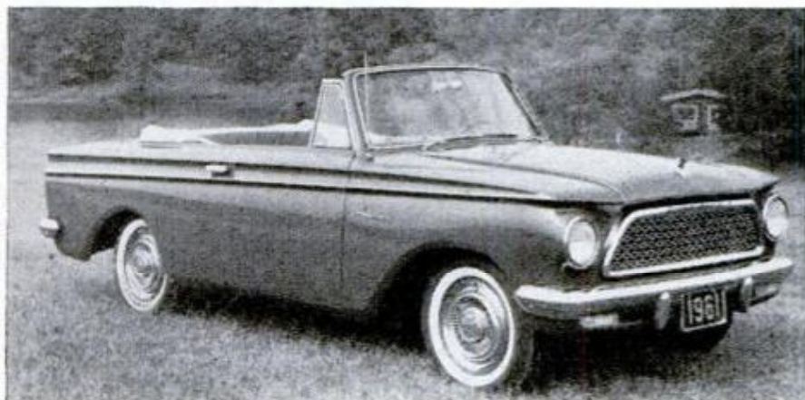
Five-passenger convertible, left, is brand new body for Rambler, has power-operated top, choice of 90 or 172-horsepower engines. Legroom in sedan, right, is adequate for six-footers with front seat fully back
