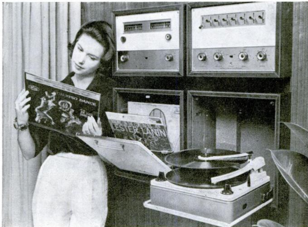
Turntable, enclosed in wall housing, pulls down to operating position. Record-storage cabinet matches phonograph panel, pulls down to expose records which are stored in the approved vertical position behind panel
