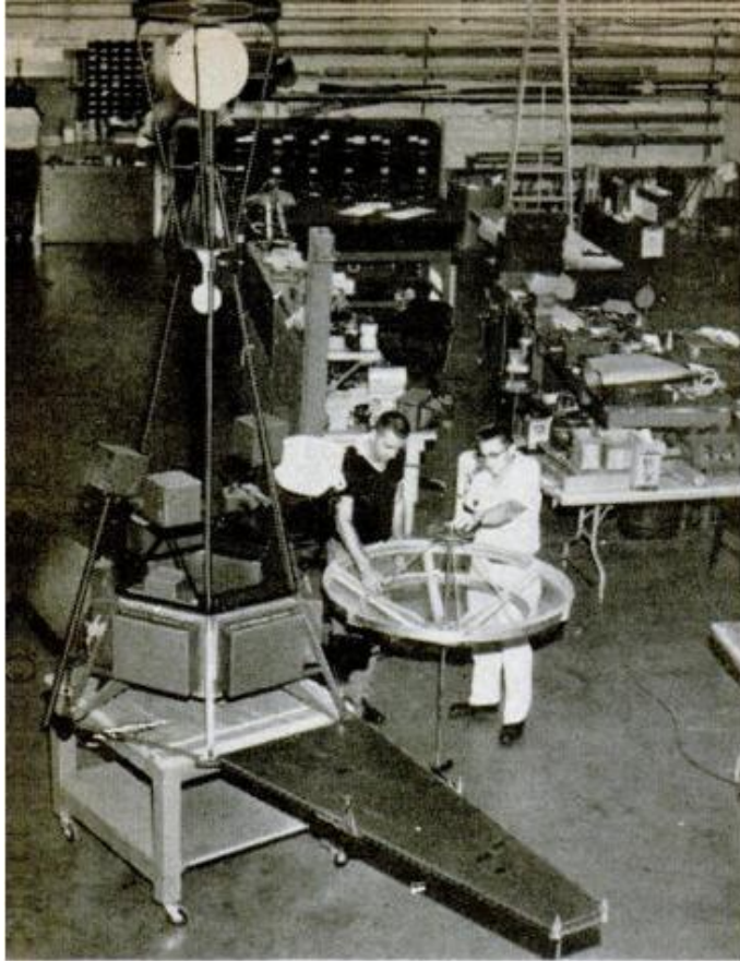
Mockup of Ranger One and Two spacecraft is studied at Jet Propulsion Laboratories (left). Diagram (above) shows instrumentation. Solar panels, folded up at launching, unfold in flight. Rangers Three, Four and Five will be modified to include Moon capsule
