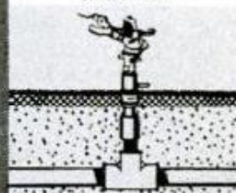
Sprinkler on self-closing lawn valve mounted on riser from underground pipe.
