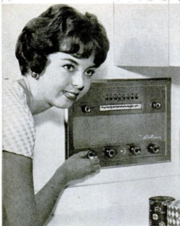
Integrated intercommunication system permits residents to interrogate callers and invite them to enter
