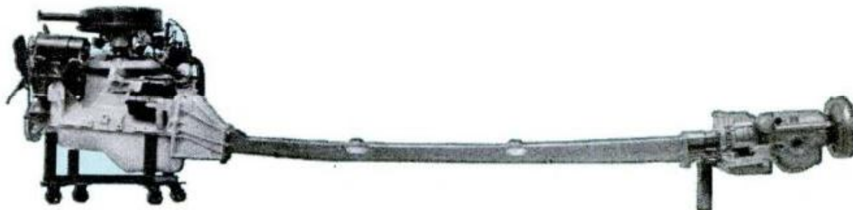
Tempest's power train with engine connected to transaxle by curved torsion bar shaft in tubular housing
