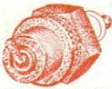
Fouled spark plug from an engine with badly worn bearings
