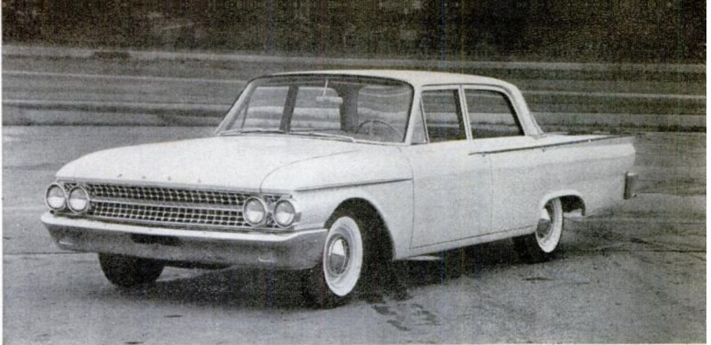
Fairlane above is plainest, lowest priced '61 Ford. Door handles are countersunk into the body panels
