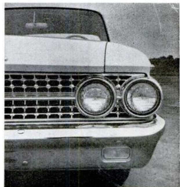
Beefier new bumper, more prominent headlamps and a simple, mesh-type grille mark front of '61 Ford
