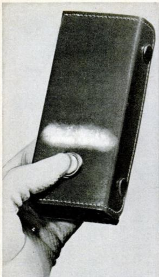
Radio-controlled garage-door operator in leather case can be carried easily. Pressing button raises door
