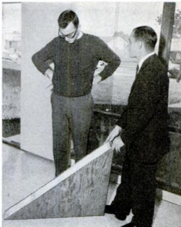
Basic building material of tomorrow probably will have plywood or other faces laminated to foam core
