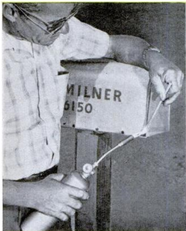
MOST METALS may be soldered by this new fluxless solder, including galvanized sheet metal mail box
