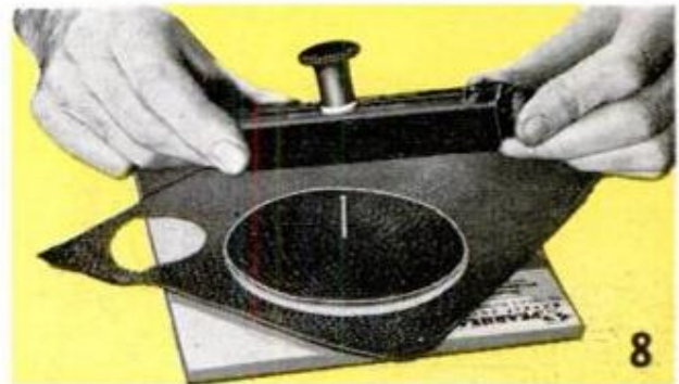
GASKET CUTTER does good work on materials such as leather, artificial leather, cardboard. Below, for true circles, perfect round openings, use lathe
