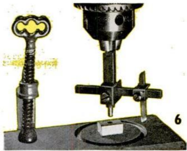
CIRCLE CUTTER on drill press will cut circles in hard-board, fiber, plastic, soft metals. Below, accessory circle jig in use on stationary jigsaw. Cuts true circle
