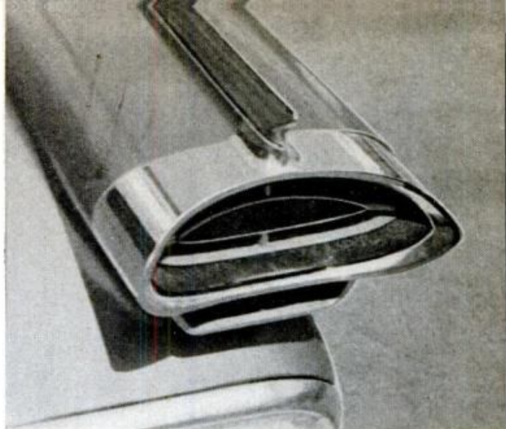
The hood or shroud may delight the stylists, but it not only narrows the angle through which the light is seen but causes eddies of air to deposit muddy spray onto the lens much more rapidly (1959 Olds)
