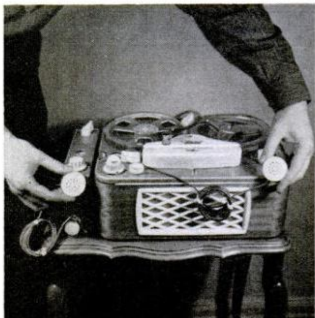
Left, RCA home tape machine plays RCA 3 3/4 i.p.s. tape cartridges. Below, Tandberg system boasts outrigger recording amplifier. This Norwegian unit has dual playback amplifiers and one built-in speaker which can be applied to either channel 1 or channel 2. The microphone for channel 2 record is plugged into the external recording amplifier
