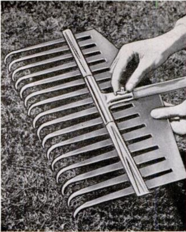
ADJUSTABLE RAKE sweeps leaves, loosens soil, rakes dead grass and spreads seed. It is set to perform any of these tasks by loosening a wing nut and moving the handle up or down, or sideways, to vary the tension on the tines and the position of the handle Braun Manufacturing Co., Inc., 1635 N. Kostner Ave., Chicago 39
