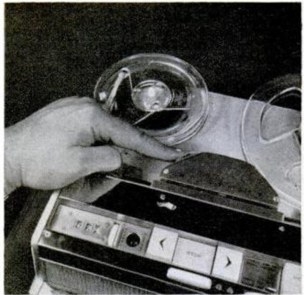
Many tape recorders have shift levers to select either half-track or quarter-track arrangement
