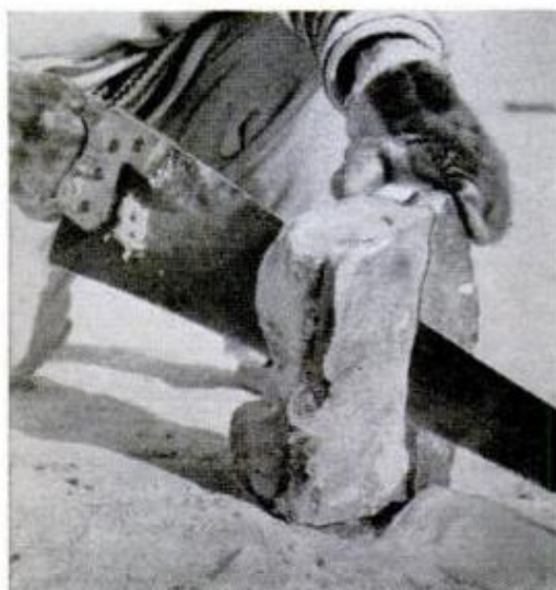
At the Povungnetuk quarry, members of the Sculptors' Society chop out pieces of soapstone. They pry it out with axes and ice chisels, cut it to shape with handsaws and hatchets, strange tools for such fine work
