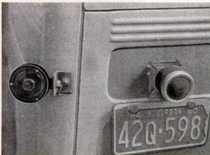
The tail lamp lens on Jeep, below left, is going to get much dirtier from eddy currents of spray than the outboard turn signal. Turn signal grouped with headlamp on this 1957 Plymouth, below right, is very difficult to see clearly when headlamp is on and can be dangerously confusing under certain conditions
