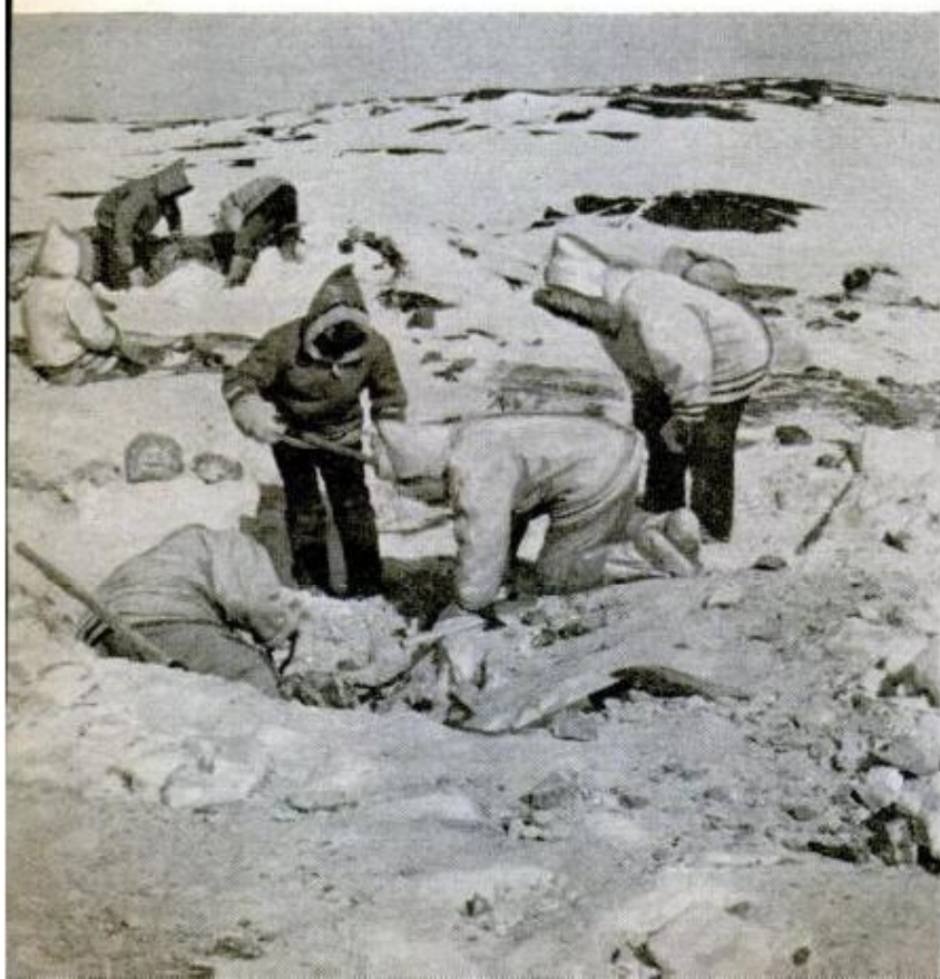
At the Povungnetuk quarry, members of the Sculptors' Society chop out pieces of soapstone. They pry it out with axes and ice chisels, cut it to shape with handsaws and hatchets, strange tools for such fine work
