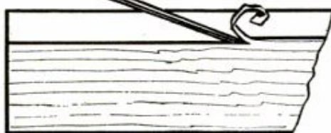
15 WHEN RABBET IS LONG, CHISEL IS HELD WITH BEVEL DOWN
