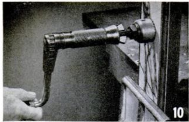
HOLE SAW cuts round openings in harder materials such as plastic-faced plywood, hardboard, metals
