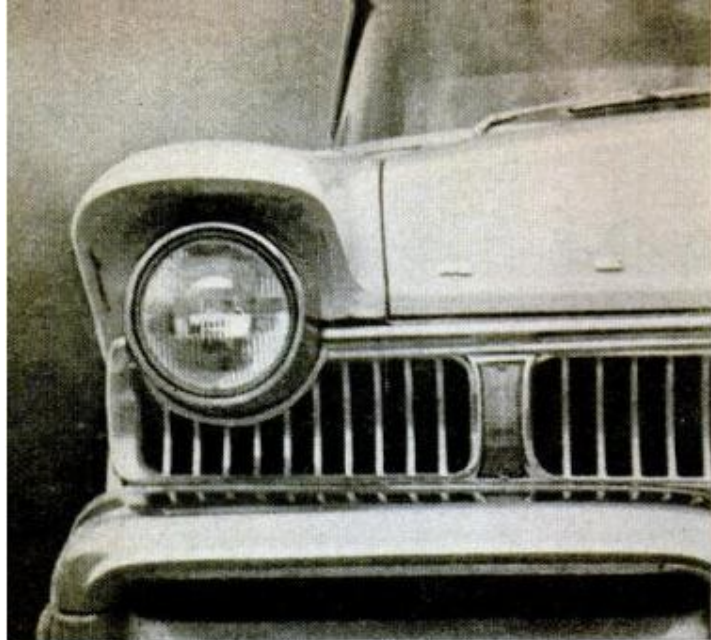
A poorly placed turn signal placement on this '57 Mercury. It is so far inboard that it can easily be hidden by a preceding car. It is also too small and viewers are distracted by much glittering chrome
