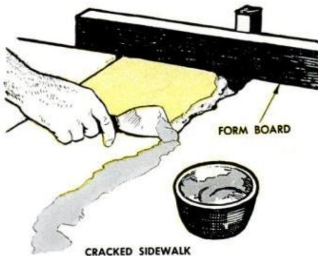
4. Board staked against sidewalk edge confines patching material to crack, resulting in neat repair
