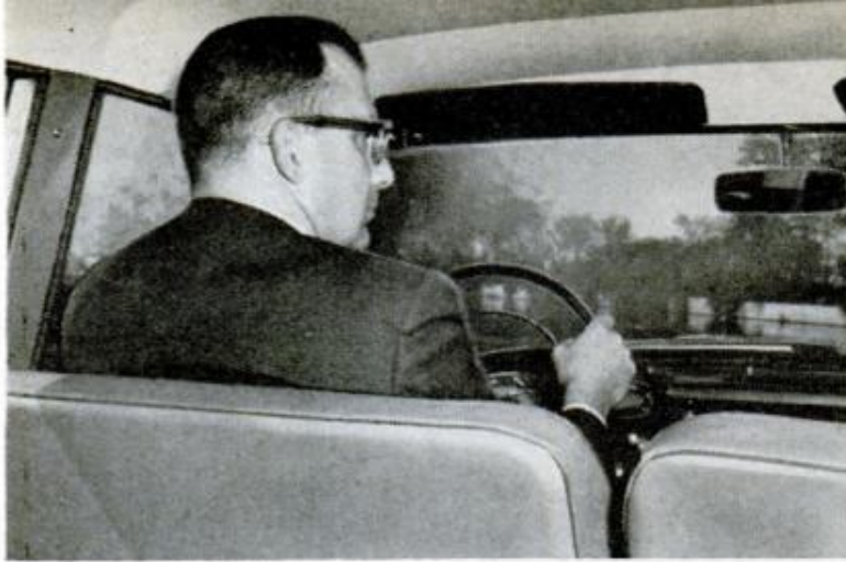
Rear-view mirror definitely blocks forward vision, left, for tall and average-height drivers. Low rear opening on wagon, right, limits loading capacity; 30-inch trash barrel can't be loaded upright
