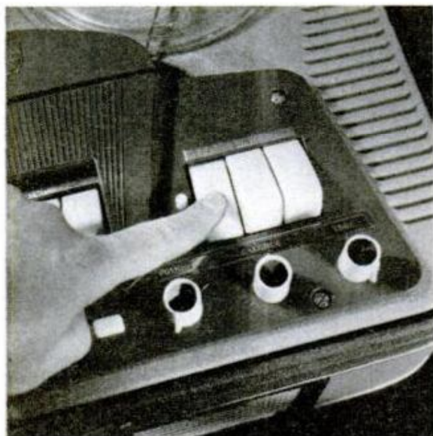
Three-speed machines, such as Norelco (above) and Stereo Record III, turn on and off by same switch that controls 1 7/8, 3 3/4 and 7 1/2-inch-per-second speeds
