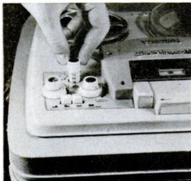
Three-speed machines, such as Norelco (above) and Stereo Record III, turn on and off by same switch that controls 1 7/8, 3 3/4 and 7 1/2-inch-per-second speeds
