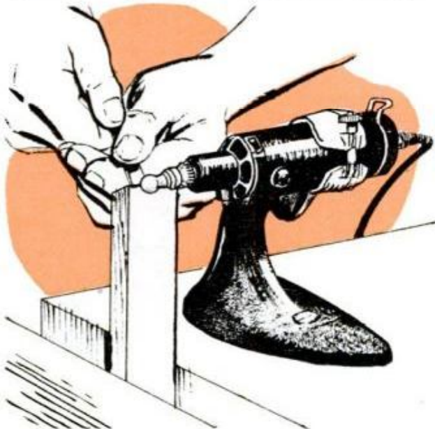
Modelmakers often have use for a midget speed lathe on which pencil-sized turnings can be made. Here's such a lathe in operation with improvised tool rest
