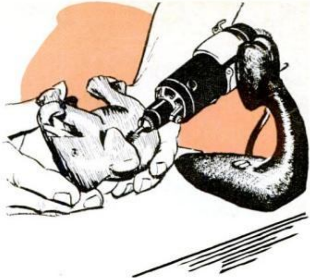
Here carving is being done freehand with grinder held in a fixture. Similar work also can be done with grinder held freehand and workpiece clamped to bench
