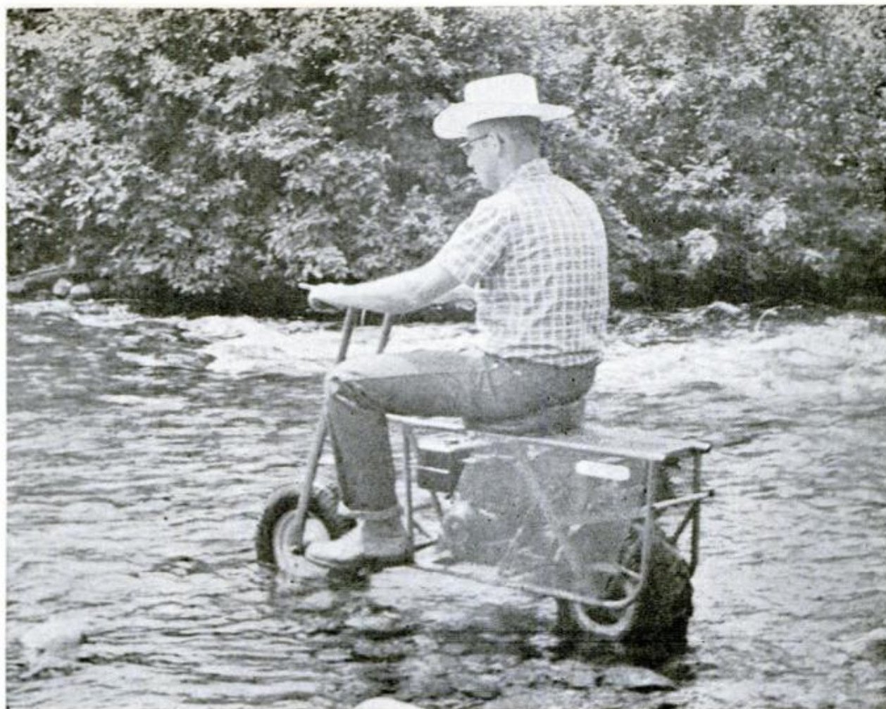
As much fun as a mountain goat (which it is named after), the go-anywhere scooter takes brooks in stride. The rear drive assembly is protected by the heavy mesh. Platform at the rear is designed for pack carrying
