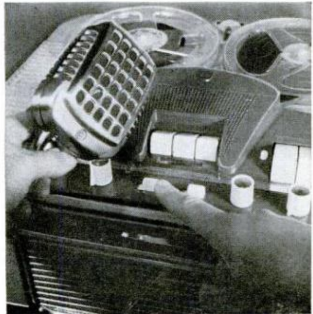
Dubbing switch on Norelco recorder permits narrative without erasing previously recorded background music
