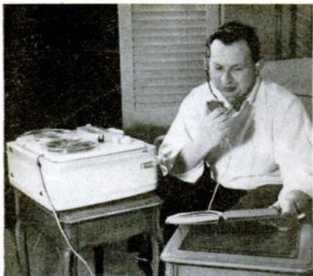
Recorders like Uher Stereo Record III permit you to record on track two while listening to track one
