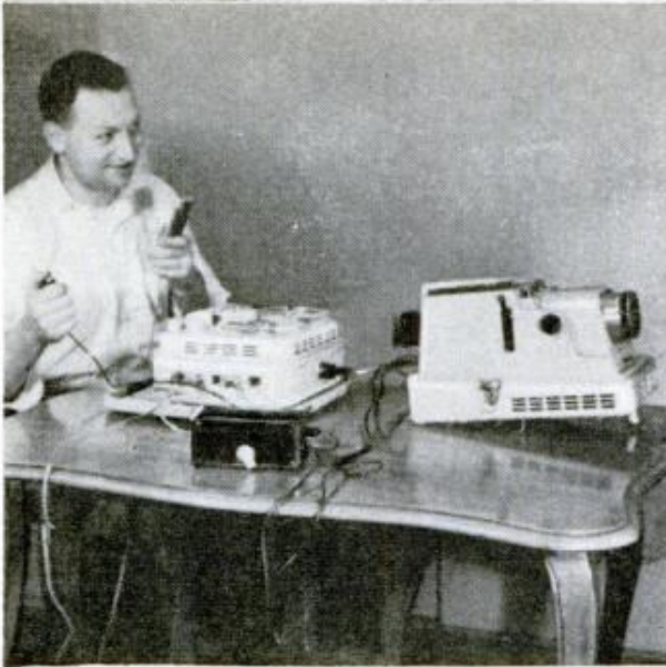
Uher Synchro-Akustomat (black box) puts inaudible tone on tape that actuates automatic slide changer
