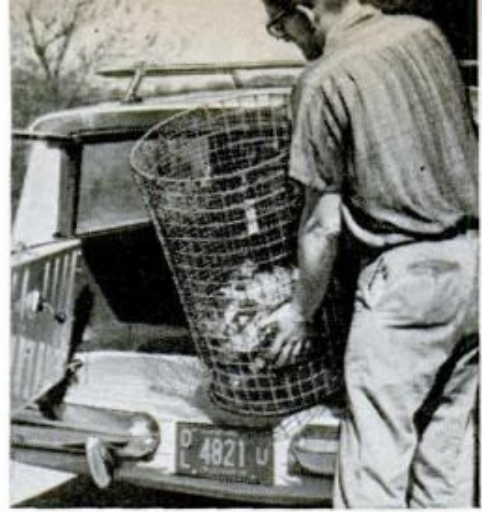
Rear-view mirror definitely blocks forward vision, left, for tall and average-height drivers. Low rear opening on wagon, right, limits loading capacity; 30-inch trash barrel can't be loaded upright
