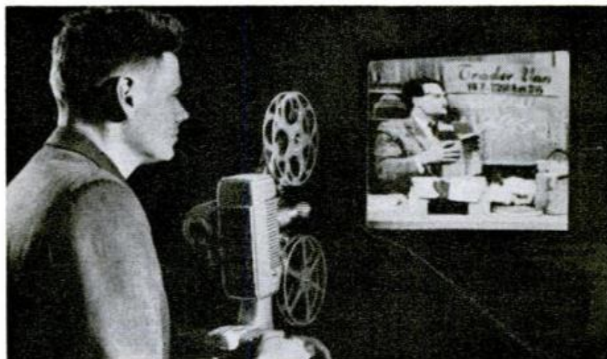
Above, Dr. Glenn uses his new thermoplastic system to record TV signal. Below, image reproduced from plastic instantaneously, without processing
