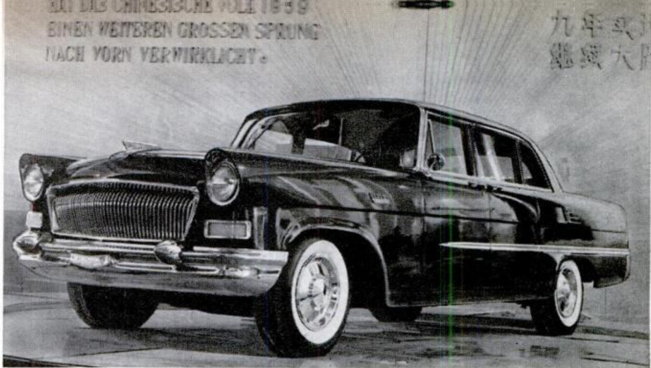
COMMUNIST CHINA'S first passenger car to show up at foreign exhibitions was displayed at the recent Leipzig Fair in East Germany. Called the "Red Flag," the big six-passenger sedan is powered by a V-8 engine developing 220 brake-horsepower at 4400 r.p.m. Length is 226 inches; wheelbase is 133.5 inches. It comes with automatic transmission, hydraulic-power steering, vacuum-assisted brakes and auto-tuning radio
