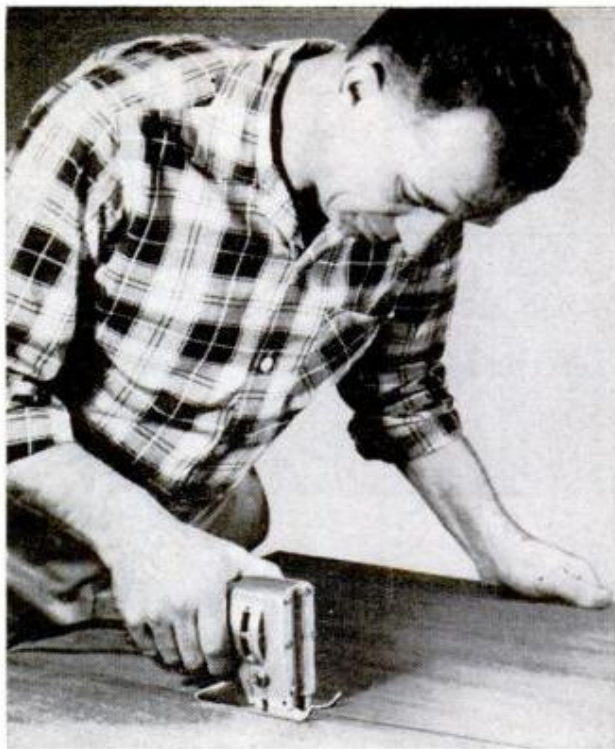
Curved pieces can be quickly sawed from the large sheets of plywood with a handy portable sabre saw
