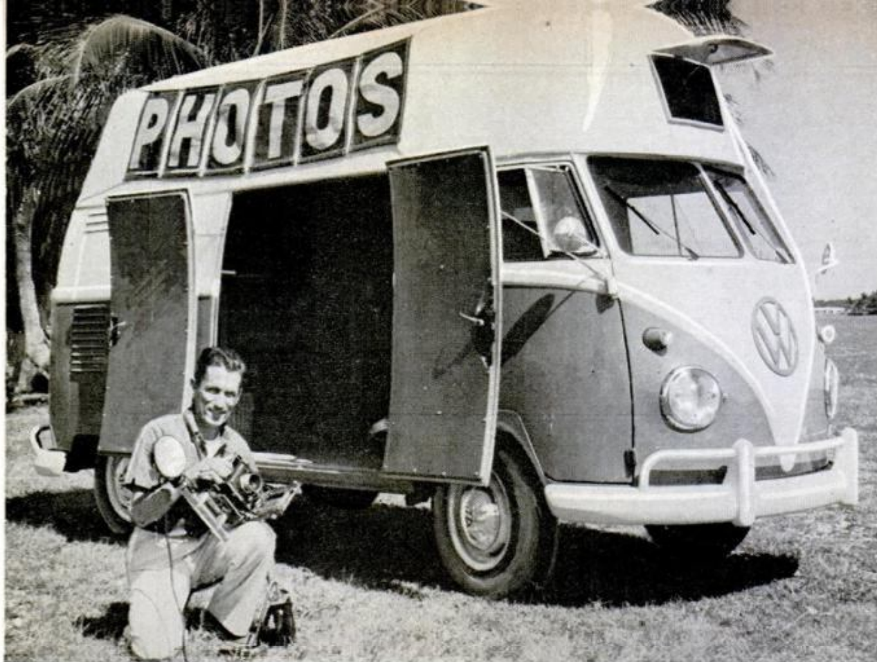
Photographer Wever raised the Volkswagen's roof to install a darkroom, painted it white to reflect heat
