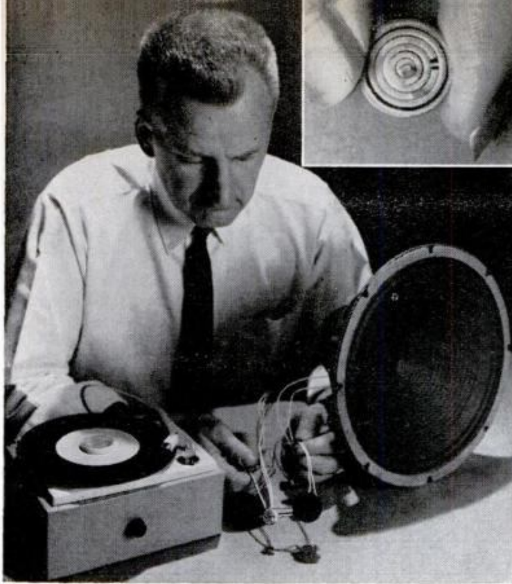
Button-like objects between turntable and speaker bear little resemblance to today's amplifiers and pre-amps., but perform the same jobs. Three of eight molecular electronics function blocks developed so far include (above, right) two-stage video amplifier, free-running multi vibrator and five-watt audio amplifier
