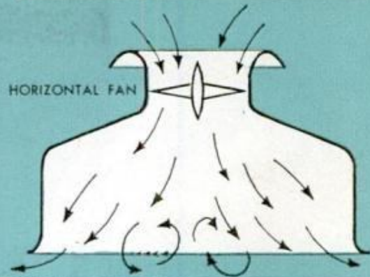
D PLENUM CHAMBER
