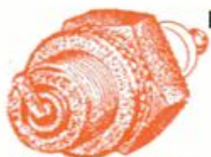
Fouled spark plug from an engine with badly worn bearings
