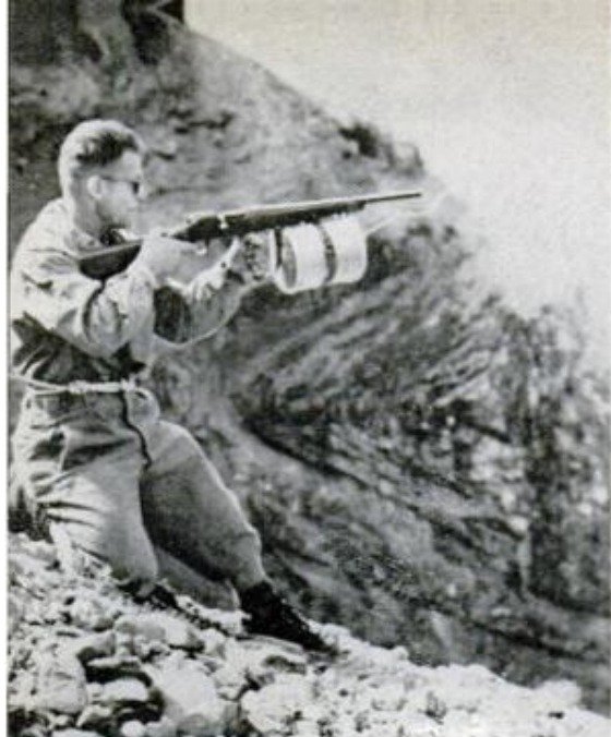
Rocket carries cable down to base
