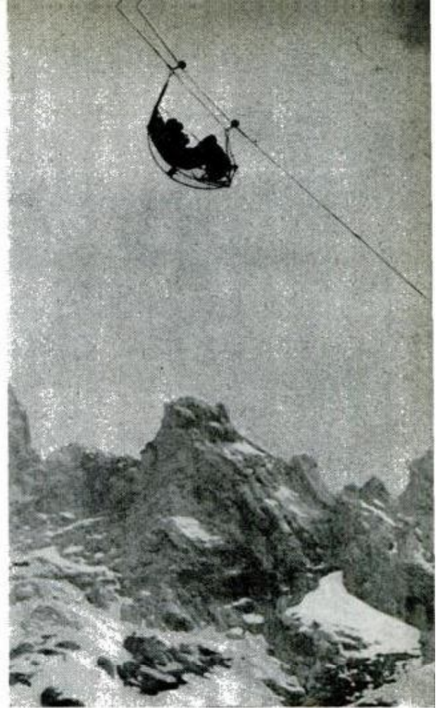
Volunteer goes into the chair, above, and down the mountain to safety. Thin cable has a tensile strength of 1800 pounds
