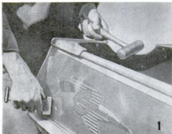
Above, first step in repairing gash in aluminum boat is to hammer metal back into original shape, using nylon hammer and heavy piece of metal as anvil
