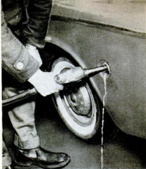
Above, many owners complain that the floor-mounted shift lever is awkward and that it interferes with center rider in front seat. Left, another complaint is that the fuel tank cannot be filled completely without spilling due to the horizontal intake pipe
