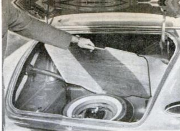
Above, trunk space is excellent in the Valiant as the spare tire is carried in a well in the floor. Note the horizontal gas filler pipe, left center. Right, dashboard is neat, although plastic frame around dials is extremely jazzy. Push buttons on left are for three-speed automatic transmission
