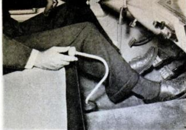
Above, many owners complain that the floor-mounted shift lever is awkward and that it interferes with center rider in front seat. Left, another complaint is that the fuel tank cannot be filled completely without spilling due to the horizontal intake pipe
