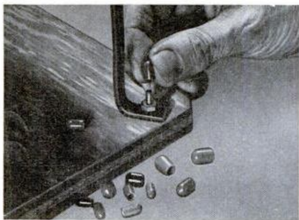
Tipped with colorful plastic caps, exposed ends of bolts have a finished look and caps offer protection
