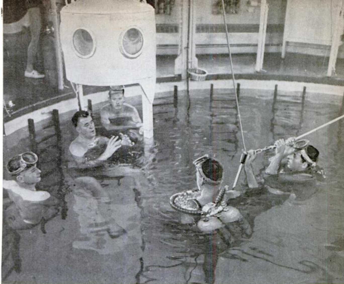
Divers at the Naval Diving Tank prepare to test flier's oxygen system to see if it will work underwater
