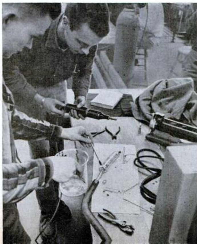
Testing for a tight seal with vacuum pump and testing coil
