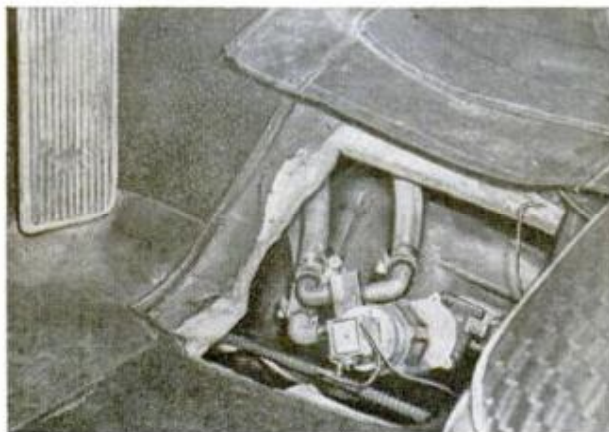
Antiskid unit is easily installed by gearing it to the speedometer drive mounted on the drive shaft
