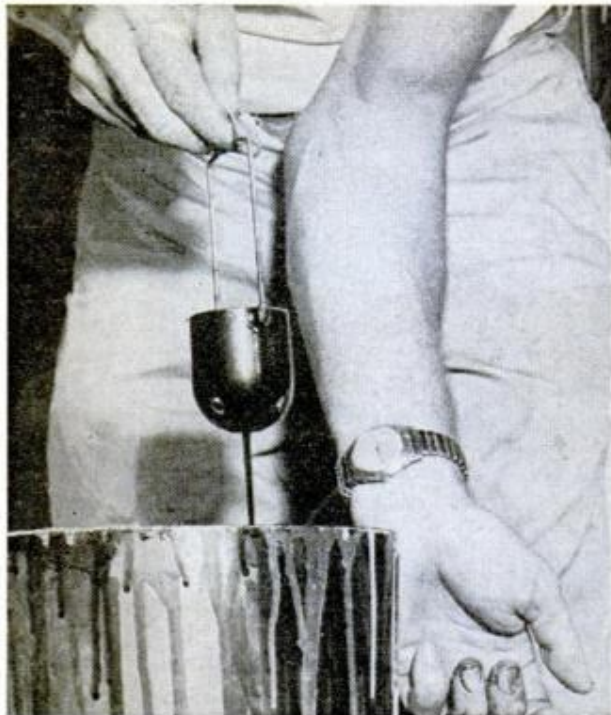
2. To attain the proper viscosity for the "flow-on" process, the fluid is passed through a viscometer. Its rate of flow through the cup is carefully timed
