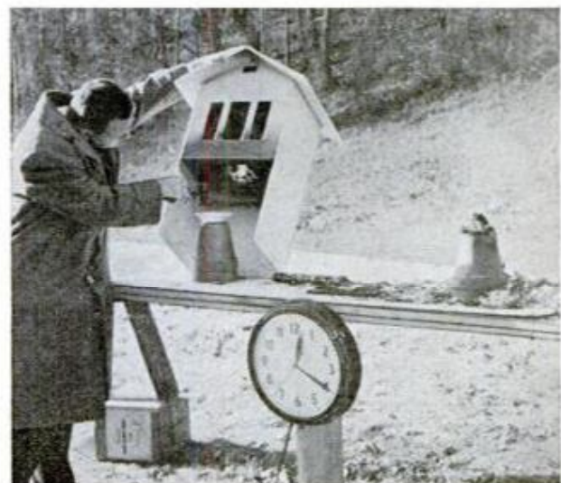
Below, after 20 min., the untreated house is completely consumed by flames. Treated house is scorched and has hole in floor where it was in direct contact with the fire but is otherwise intact and unharmed
