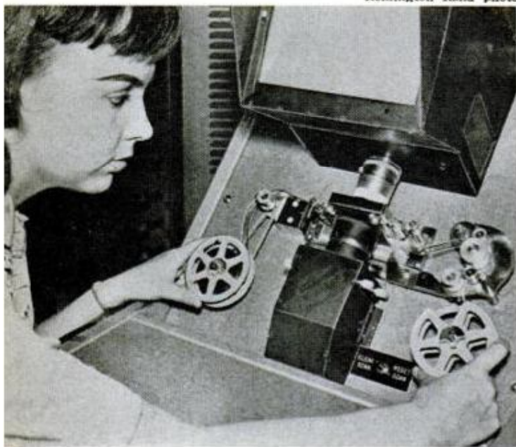
Electronic eye of FOSDIC scans each frame of microfilm. Below, operators prepare reel of the film
