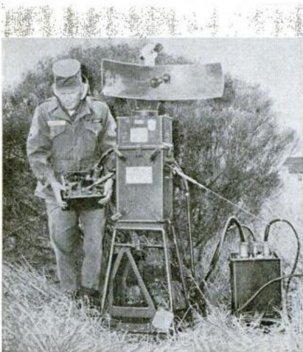
Medium-range field radar set detects moving objects, then tells its operator their distance and direction
