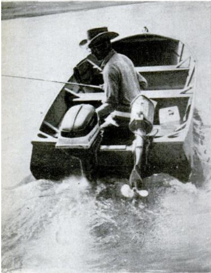
Author Tinsley, in his favorite fishing rig, runs out across Granite Shoals Lake in Texas with his aluminum boat and a 12-horsepower motor. When he's reached his spot, it's a simple matter to kill the big motor, drop in the troller, and ease quietly along the shoreline, casting with one hand and operating the small motor with the other when necessary. The motor in these photos is an Electric Sportsman; shown at far right are three other available motors. Another, not shown here, is the Minn-Kota Electric Troller
