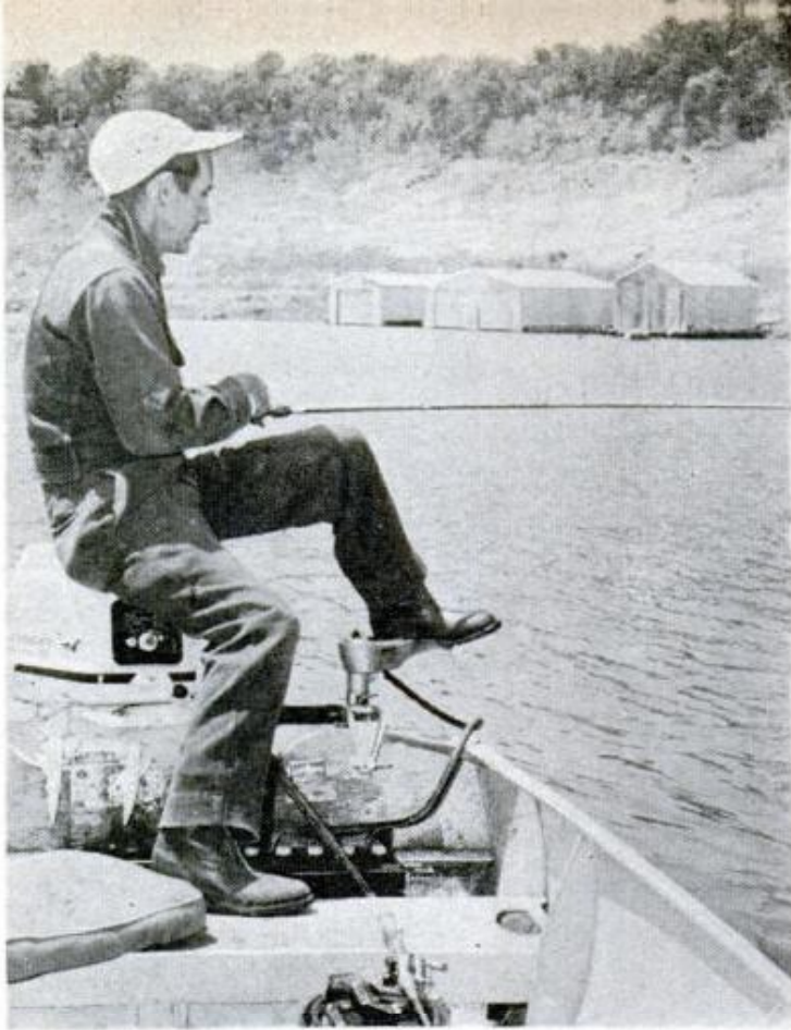
Two tricks with electric motors—above, sit on the motor and steer with one foot. Below, mount the motor on the bow (note footrests). But don't try either without a good, stable boat
