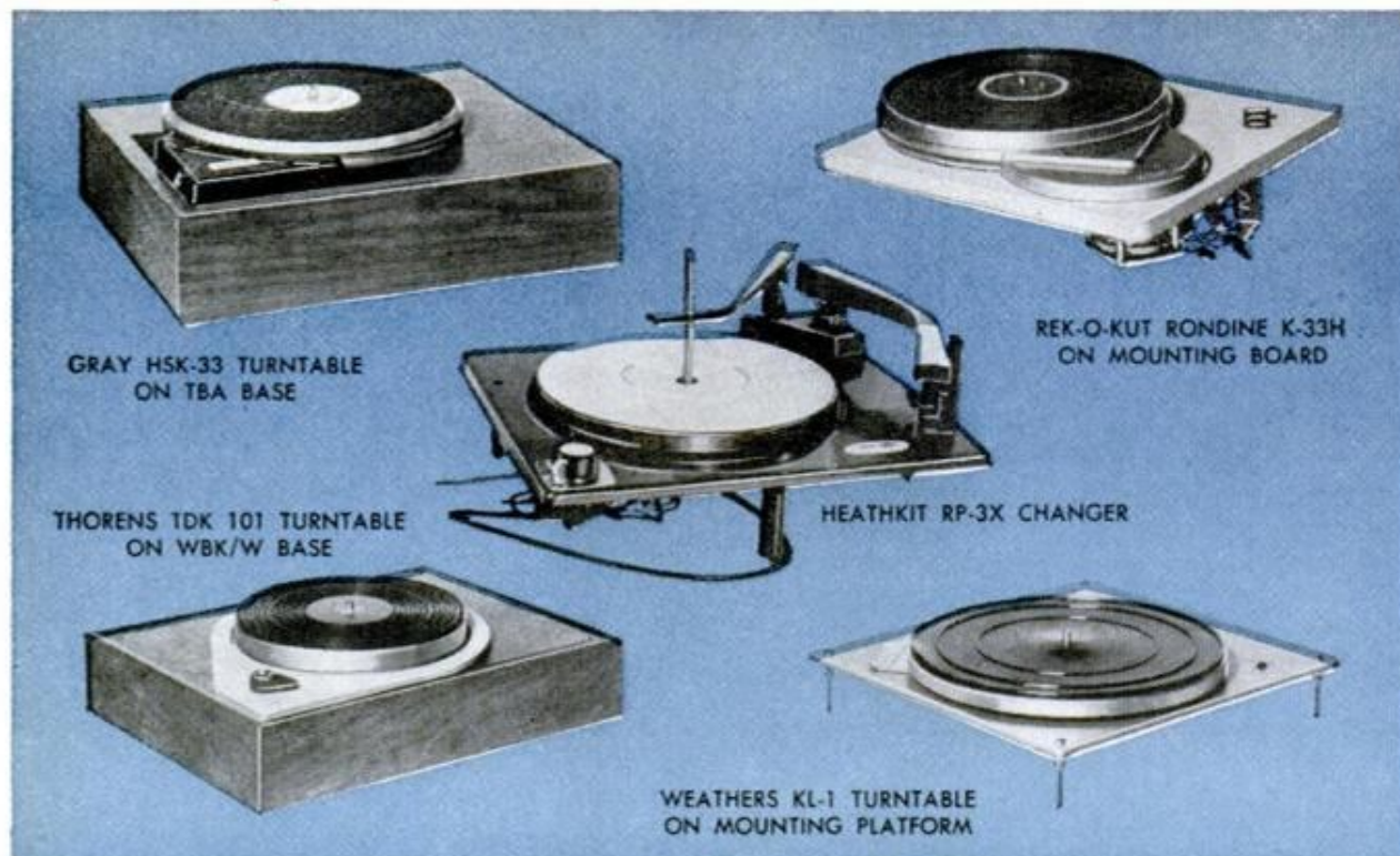
Kit-built turntables and record changer. The differences are measurable but audible variations are slight
