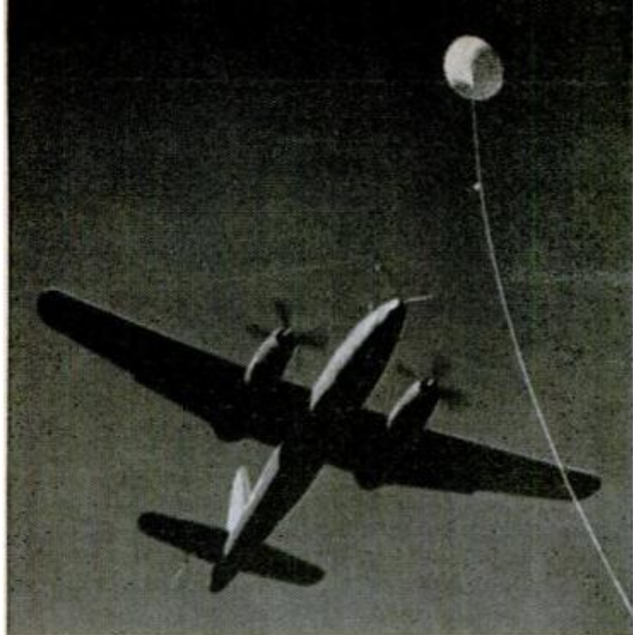
P2V Neptune patrol bomber grabs the pickup line at 500 feet and 125 knots. Pickup yoke is on its nose
