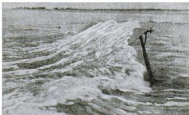
Breakwater model in surf shows wave-deflecting action
