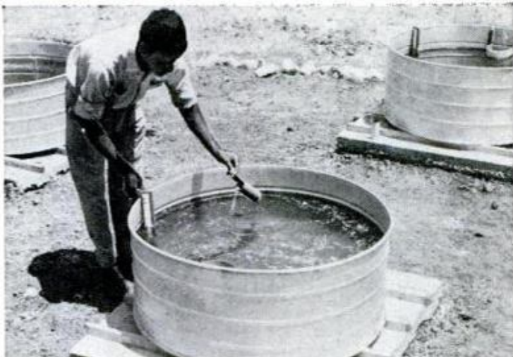
Measuring the flow of water in a river means half a day's work for members of Northern Rhodesia's hydrological section. Below, evaporation of water is calculated to learn the true capacity of a dam
