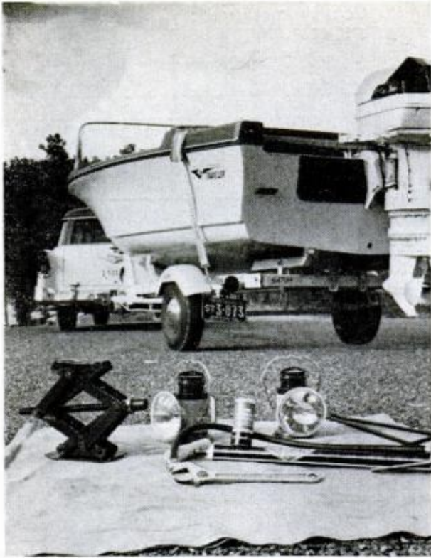
5. Scissors jack, tire-patching kit and pump, lanterns and wrench to tighten hitch are carried for emergencies
