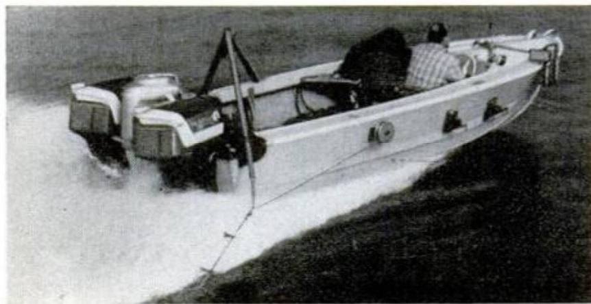
Unusual "sandwich" outboard motor arrangement drives the test boat at high speeds. Hooded operator reads instruments and makes test notes
