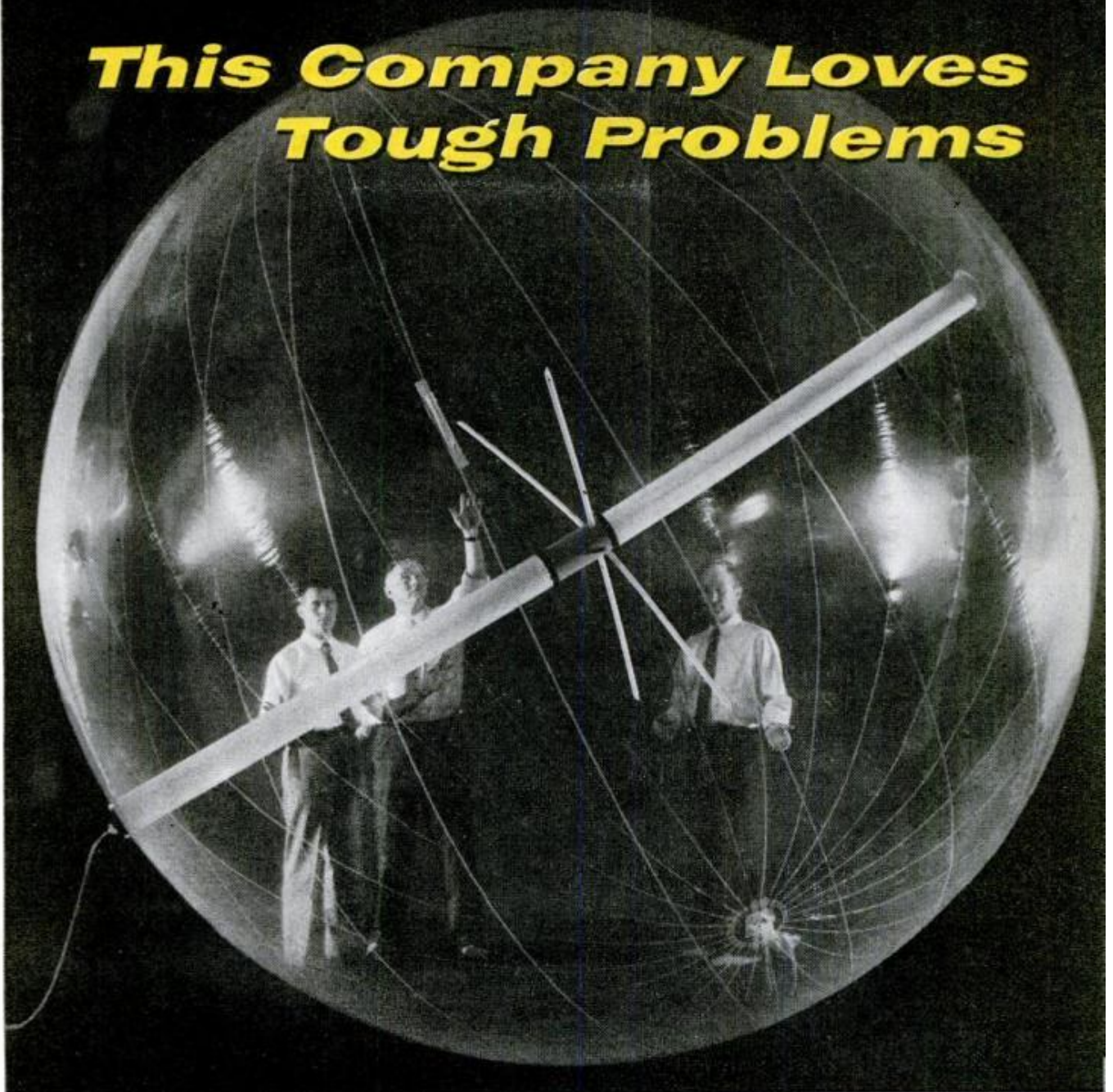
Balloon designed by ADL will shoot from a rocket to record density of atmosphere 300 miles above earth
