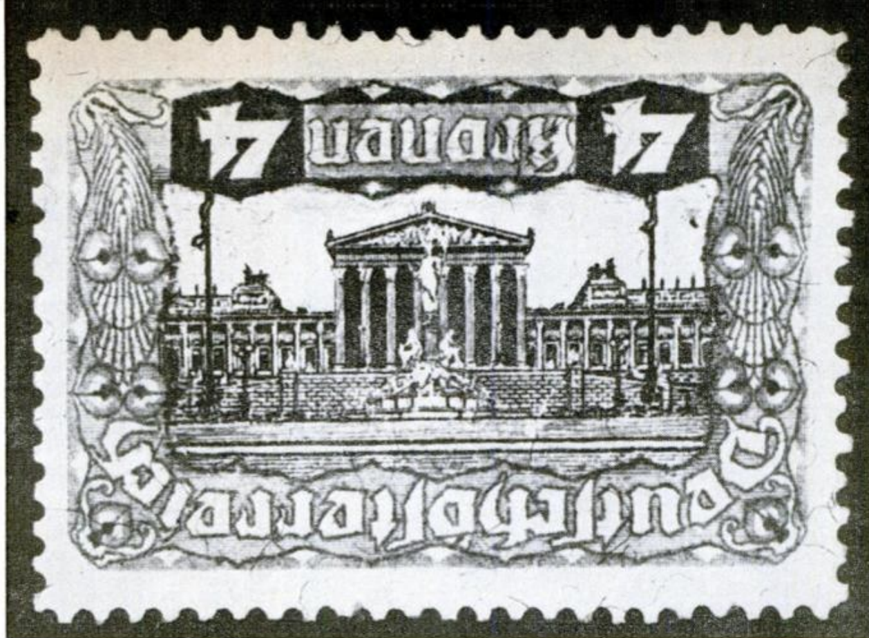
Radiograph of Austrian stamp shows center was removed and inverted. The adhesive used makes dark lines
