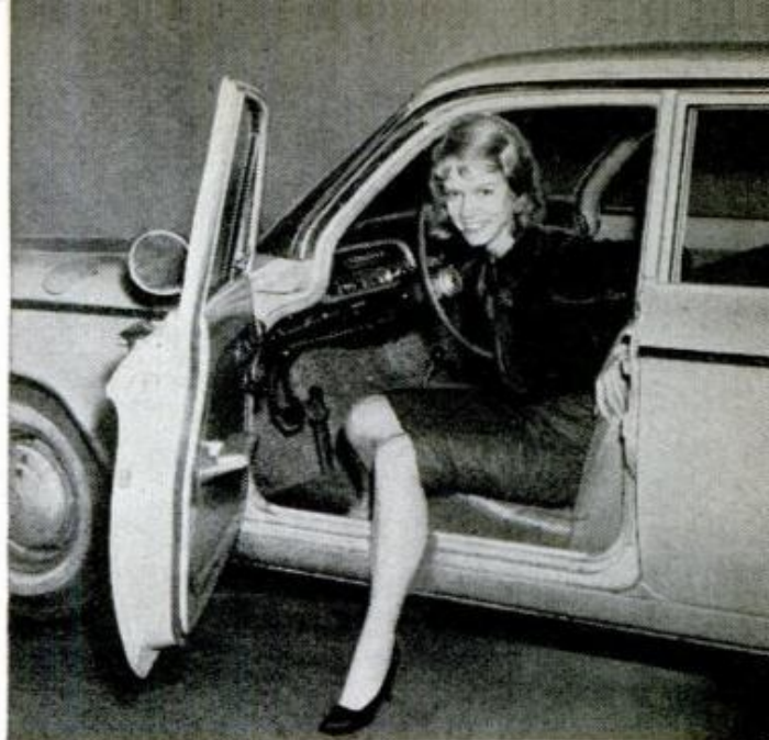
It is not easy to get in and out. Stepdown floor, low roof make entry and exit an art to be learned
