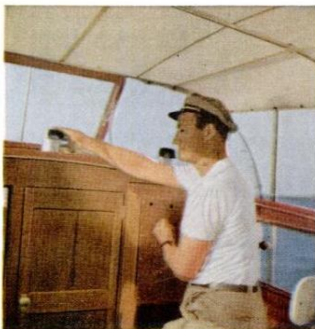
Author Wobeck sets compass monitor to the planned compass course to simplify navigation when the boat rolls at sea
