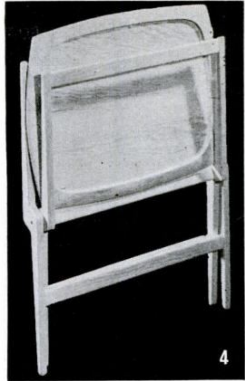
When table is folded, tray nests between upper halves of legs for compact storage
