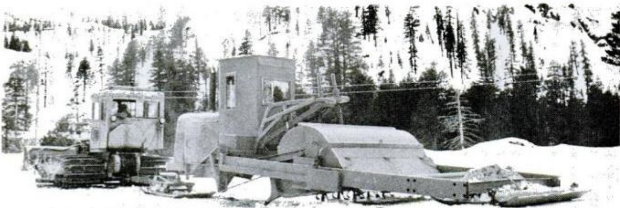
Giant snow roller weighs five tons empty, compacts snow in first step to allow other vehicles to operate. Snow planer, below, levels the rolled surface. Sawdust toppings varied from one to three inches in tests
