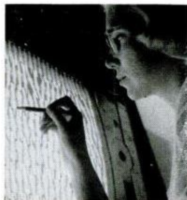
This X-ray check makes certain that the Conductaseal has bonded properly. It's one of 116 AC reliability tests.
