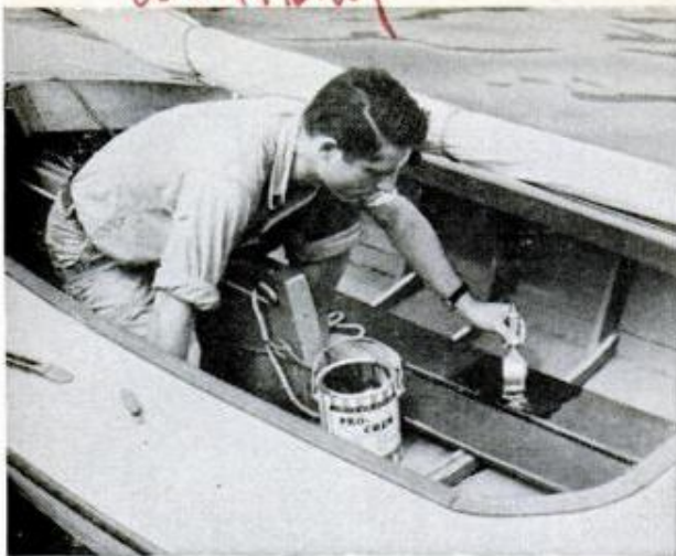
Liquid rubber brushed on boat floor boards provides non-skid, hard-wearing surface. To patch down-spout, coat repair area with liquid rubber, cover with screening when tacky and fill mesh with more coats
