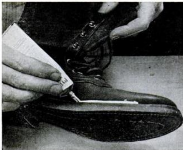
Bead of liquid rubber applied along seam between shoe sole and upper serves as waterproofing seal
