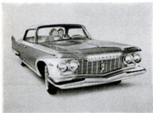
Body and frame are welded as one unit with Dura-Quiet Unibody construction.
