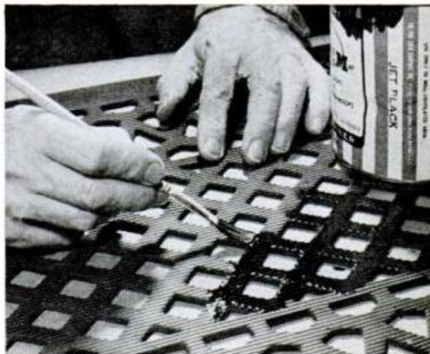
Coat of liquid rubber brushed on floor mat fills small cracks and cuts, giving it like-new appearance
