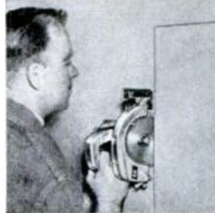
POCKET CUTS —Cuts openings quickly and easily in existing walls for windows, medicine cabinets, heat ducts, etc.
