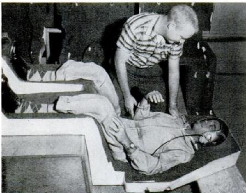
Each of the Astronauts has a foam-plastic acceleration couch moulded to his body. Here the fit of Shepard's couch is carefully checked by a flight surgeon
