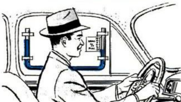
Performance meter is made by taping a transparent plastic tube to window and adding colored water
