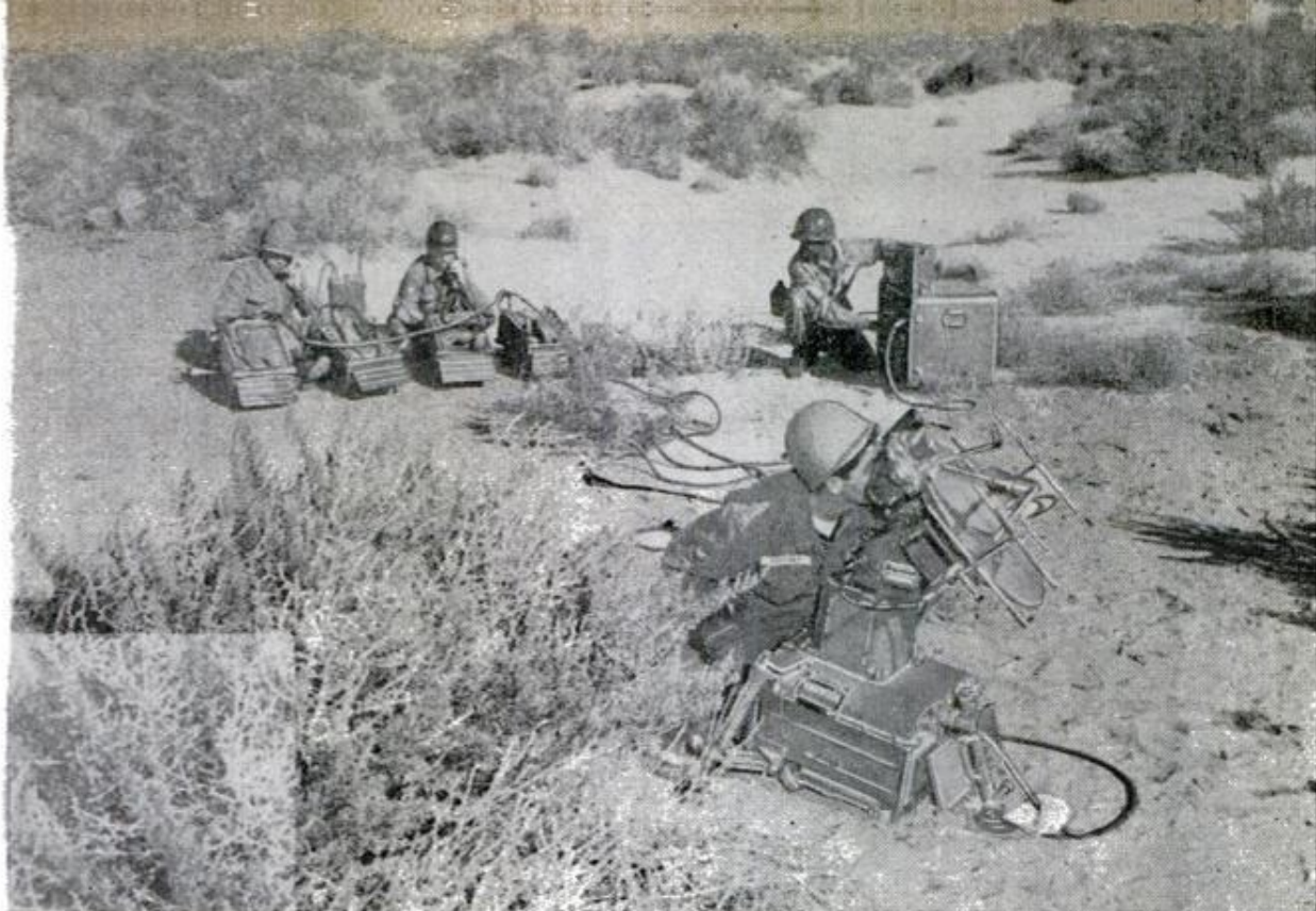
Troops guide Lacrosse missile with tracker and range finder. Tracker, right, leads missile to the target
