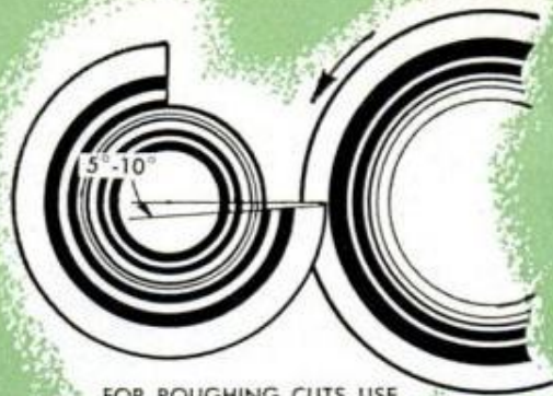
13 FOR ROUGHING CUTS USE TOP RAKE OF 5° TO 10°
