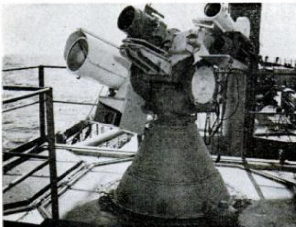
In poor weather, infrared equipment picks up the scorching missile cone as it streaks in from space
