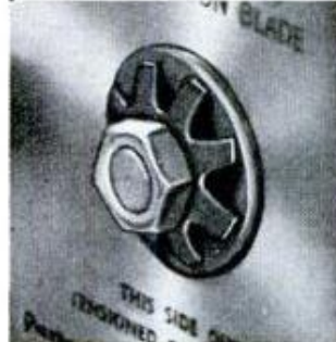
KICKPROOF CLUTCH —Automatically puts saw into "neutral" if it jams or pinches in the cut. Prevents kickback for all around safety.
