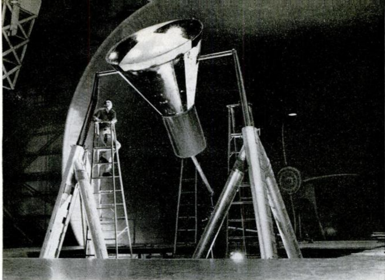
Model of the capsule is positioned in wind tunnel as part of the laboratory and free-flight testing program
