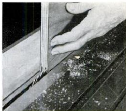
Careful setting of saw blade and rip fence makes cutting of tongues a simple matter
