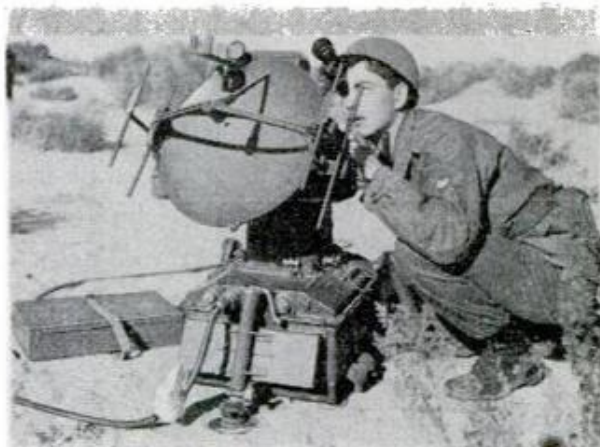
After initial blastoff, a Lacrosse missile (lower left) streaks to its target. Soldier at front line uses a portable range and direction finder (lower right) to measure accurately the exact distance to the target
