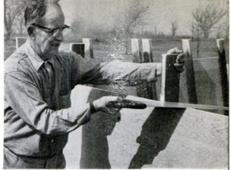
Waste ends of frame side members, plus bow and transom stiffeners, are sawed off even with top of planking. Side members are cut off at 4-deg. angle
