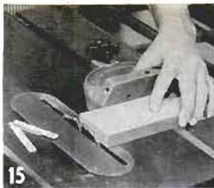
15 Run a test piece with shoulder \frac{1}{2} the work thickness. Use miter blade
