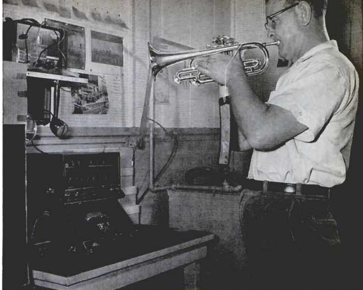
Each instrument is tested by a musician, who checks tones with an electronic device called a Stroboconn
