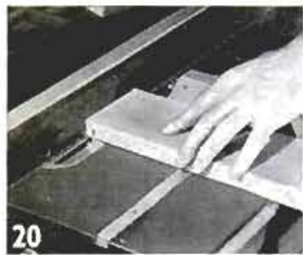
20 Make shoulder cut on end B, Fig. 14. Repeat on all ends marked B
