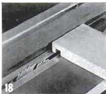
18 Follow with successive cuts to clear waste just beyond miter line
