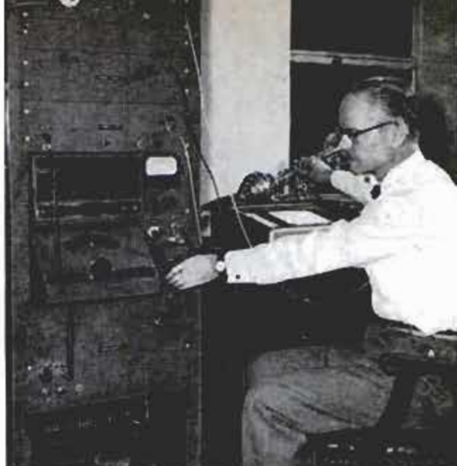
Dr. Earle Kent, Conn's research director, checks trumpet tone by attaching transducer to mouthpiece
