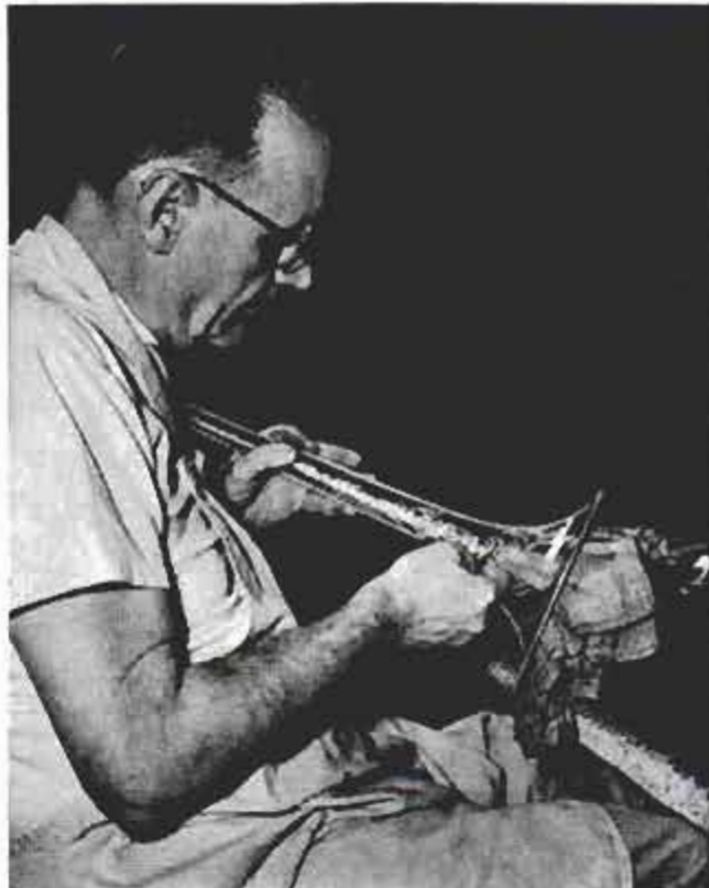
Engraving intricate, fancy lines on surface of instrument is one of jobs that still must be done by hand
