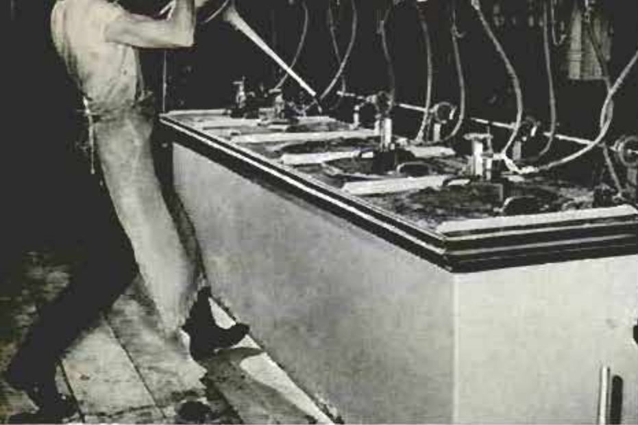
Electroformed tone chamber and bell unit of horn is yanked out of chemical vat, where copper was deposited on mandrel
