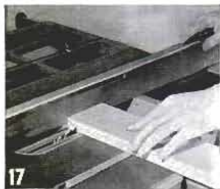
17 Beginning with end A, Fig. 14, make a shoulder cut with blade in waste
