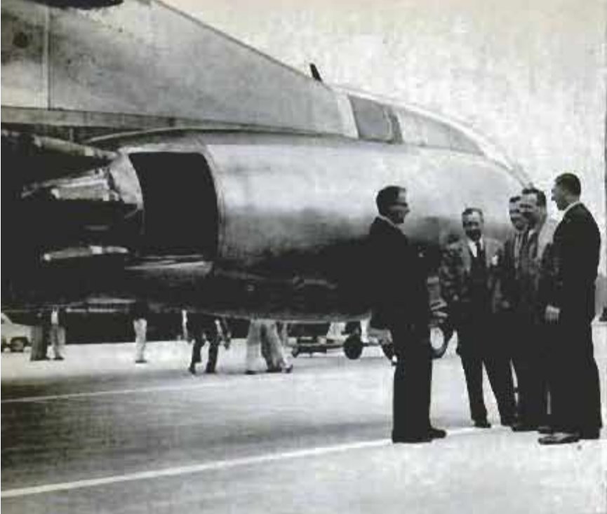
Turbofan engine on Boeing 707 has wide ducting to let extra air flow around engine. Turbofan, below, shows duct near end
