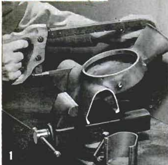
1 Select an old-type cleaner which will permit cutting away parts of main frame to form lugs for bolts
