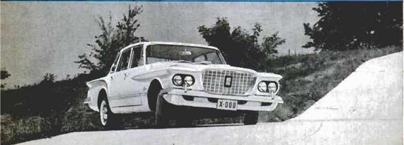
Below, despite a relatively soft ride, the Valiant corners flat and has virtually no pitch on bumps. Front suspension is by torsion bars
