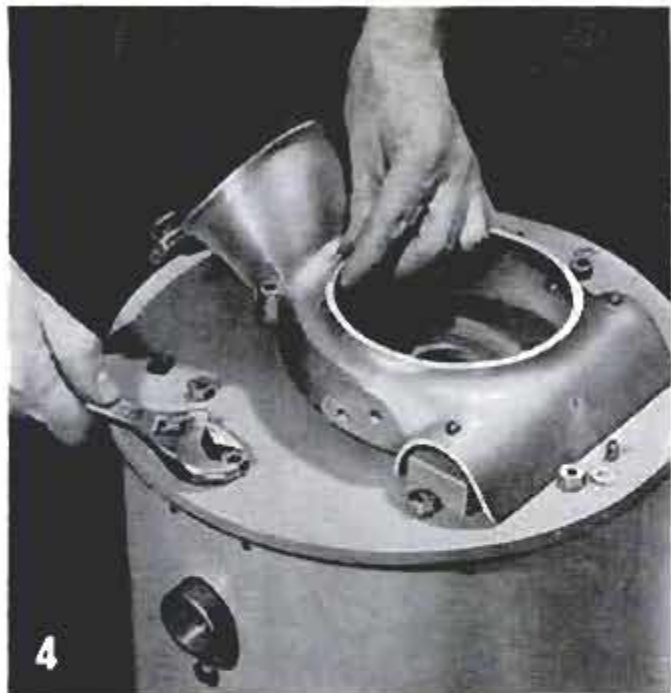
4 Plywood disks are bolted together to form rigid top. Note how cleaner-fan housing is attached to top
