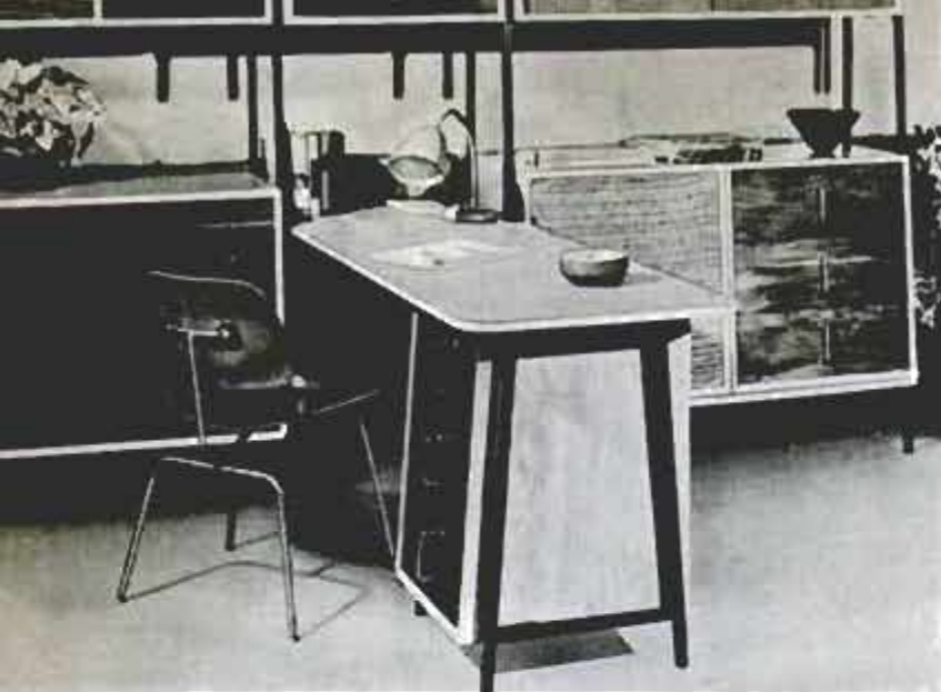
Wooden desk and cabinets built into framework of channel-type steel were made with wrench, hacksaw and woodworking tools
