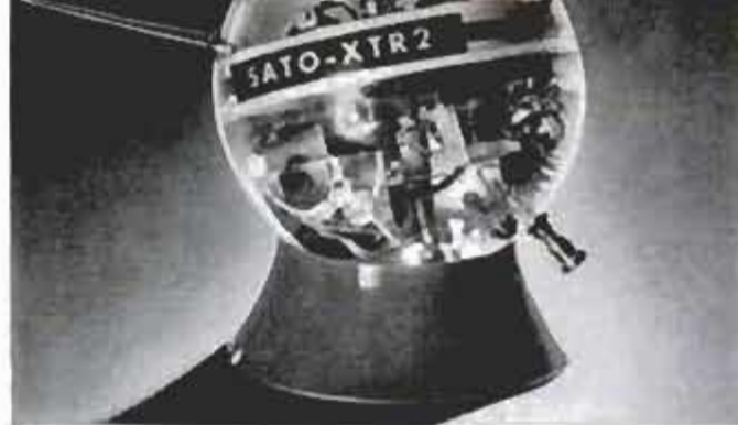
"SATELLITE" TRANSISTOR RADIO , above, sits on its desk-top stand or hangs by the antenna from a ceiling. The radio, enclosed in a transparent plastic ball, has two transistors. Earphones are supplied The Brownlee Company, P. O. Box 636, Yucaipa, Calif.
