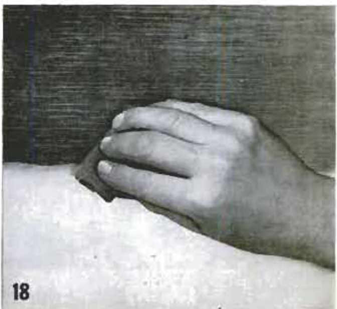
Below, wiping off filler applied over dark toner
