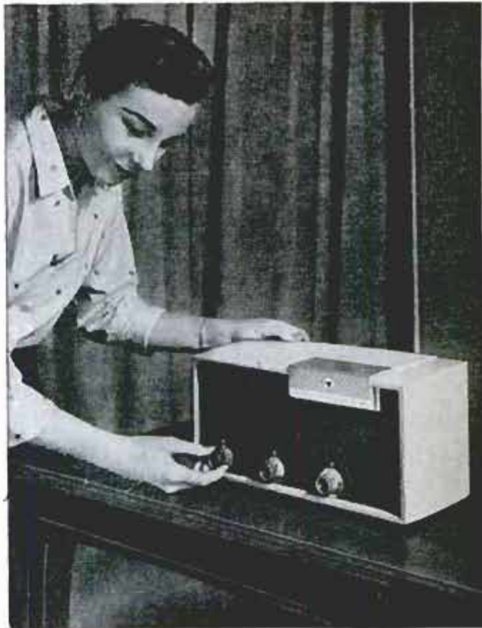
Telemeter attachment sitting atop TV set adds three optional pay-TV channels to regular free TV fare
