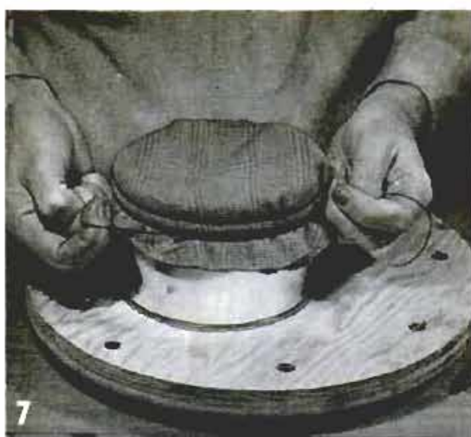
Air is drawn through cloth and cleaner bag to filter out fine dust, prevent it from entering fan housing
