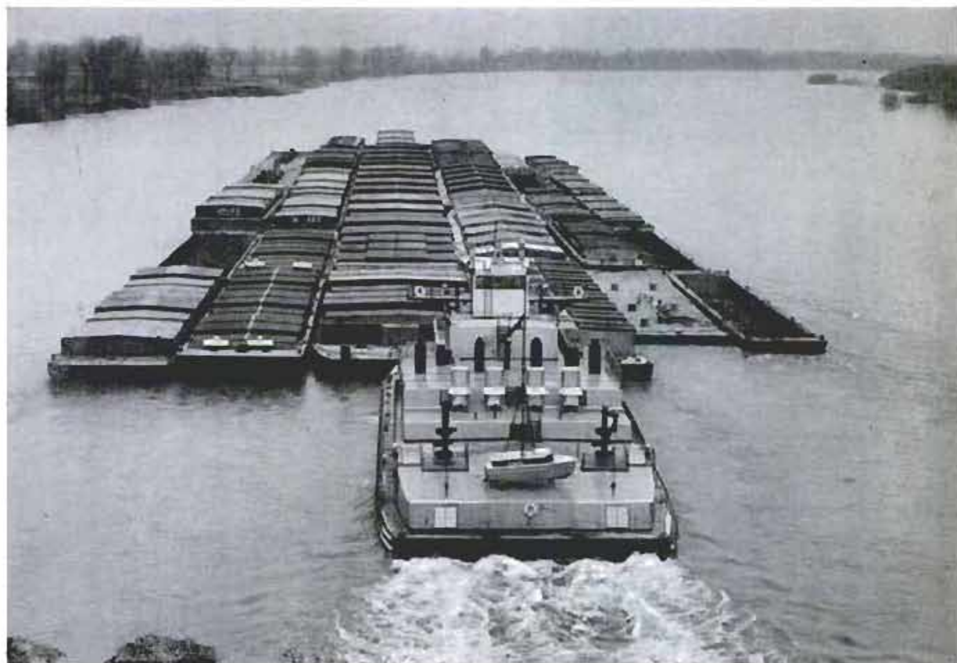
Captain Jesse Marks, above, heads upriver with a 30-barge tow. Though river boatmen stopped towing and started pushing cargoes a hundred years ago, the words "tow" and "towboat" are still used on the river
