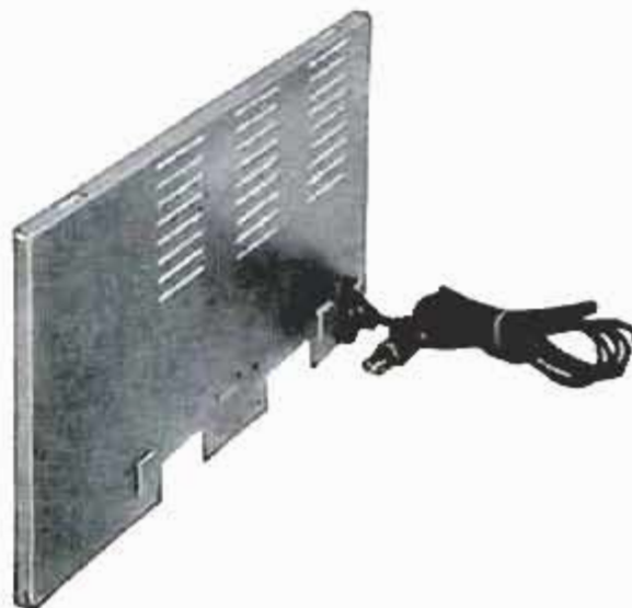
Coin box which fits inside Telemeter doubles as tape recorder; automatically records code numbers of all purchased programs
