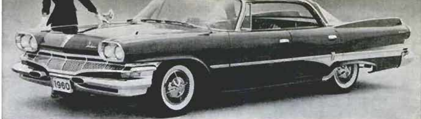
Above, the Dart has a Dodge look, but front and rear-end treatments are distinctive. Wheelbase is 118 inches. The bigger Dodge, below, is on a 122-inch wheelbase. Both series have jet-tube rear fenders, big taillights
