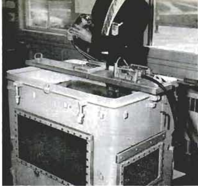
Louis Padberg inspects spark gap he places in 1200-pound water tank to make underwater sparks
