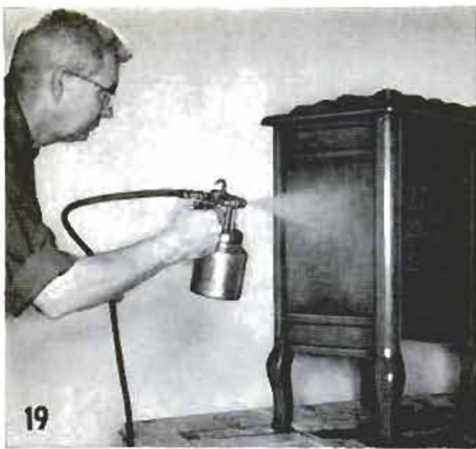
Lacquer is best sprayed on. Work should be mounted on turntable in a spray booth, or taken outdoors
