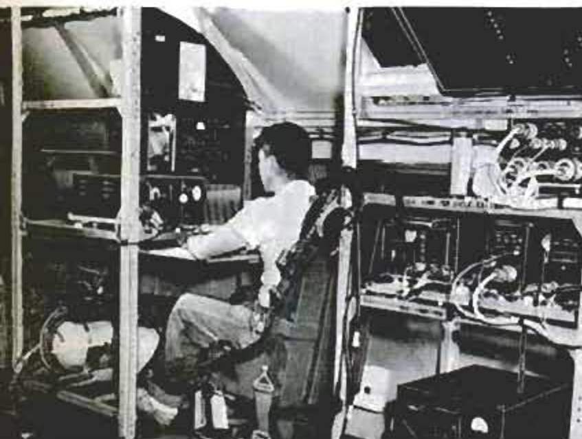
Easily assembled stairway and catwalk above illustrate versatility of lightweight steel. Below is electronic rack developed by Wright Air Development Center for test planes. Idea has saved base $500,000 annually in modification time
