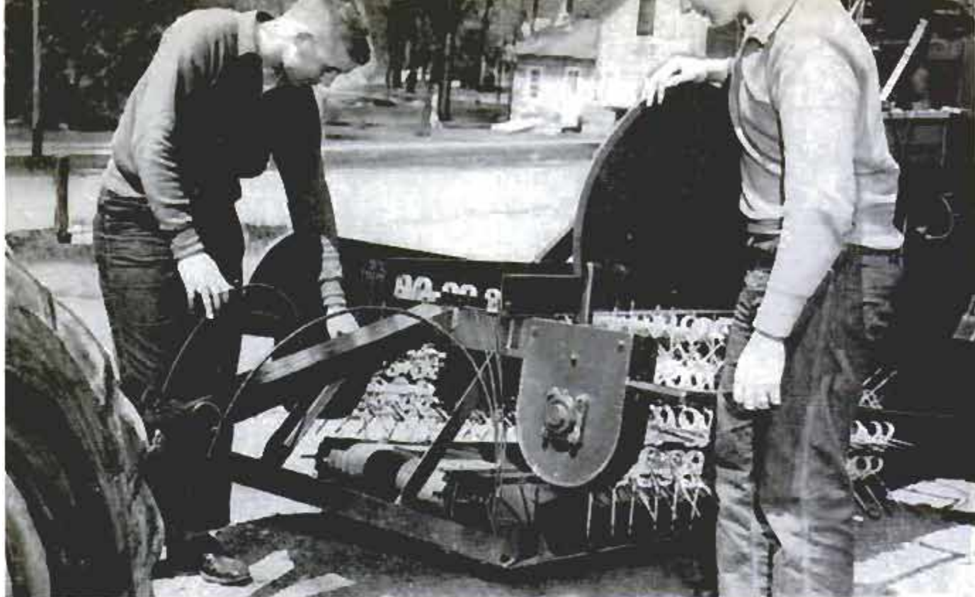
Steel fingers strip the entire bean plant onto a conveyor belt; a blower removes the leaves and stems
