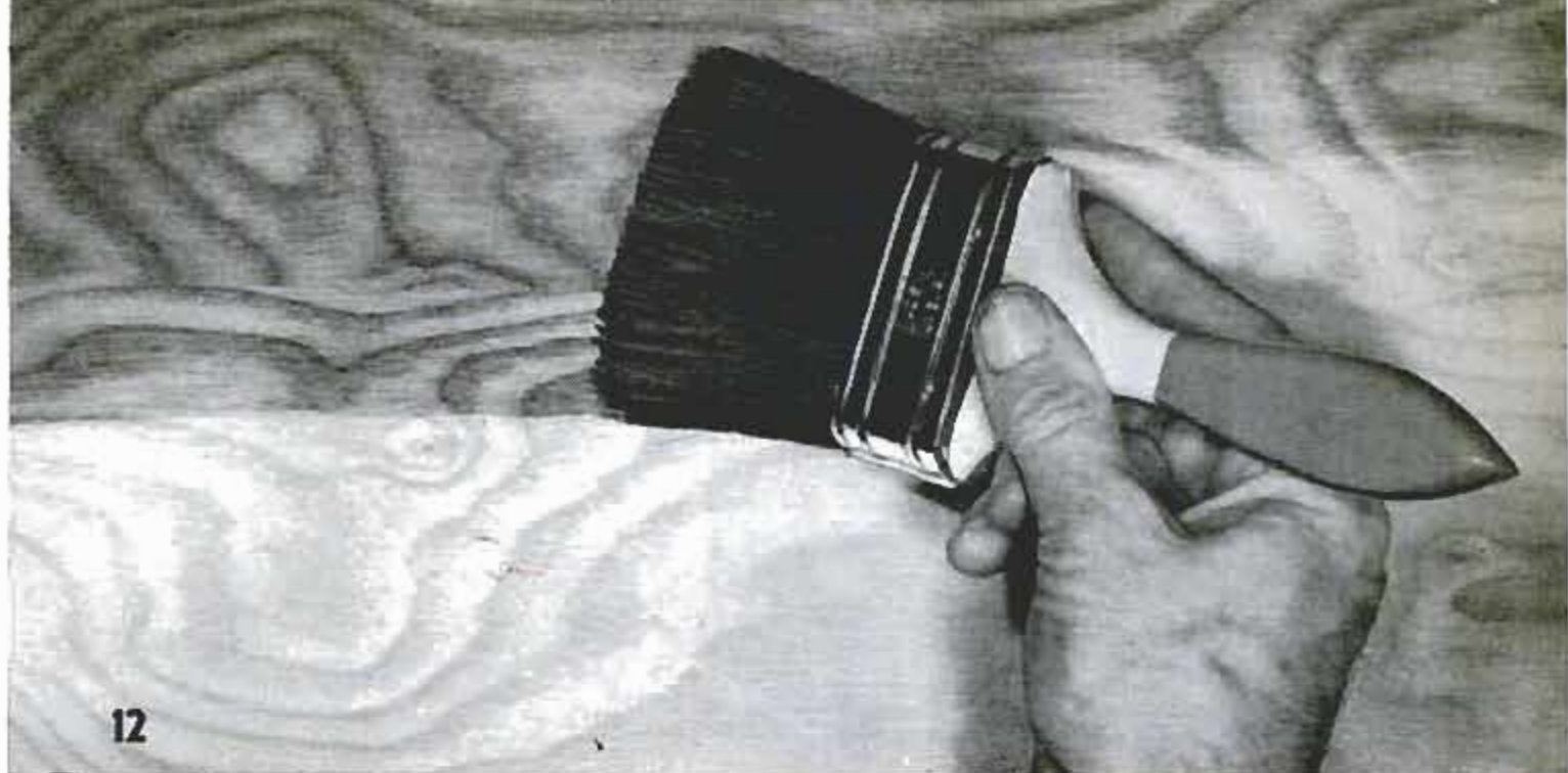
Staining or toning tends to add color beauty to wood and, in some cases, helps accentuate the grain
