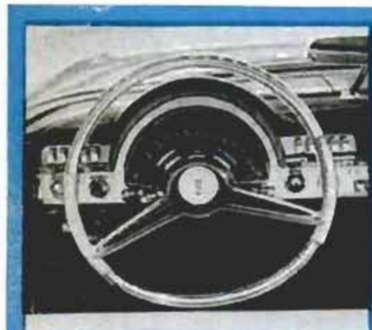
Above, Windsor two-door hardtop. New Yorker models have slightly different grille. Below, new dash has glarefree electroluminescent lighting. Push buttons (for transmission and heater) are mounted horizontally
