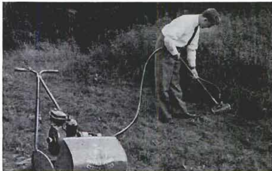
Left, flexible shaft powers the hedge trimmer. Right, rotary tiller is lightweight and easy to handle
