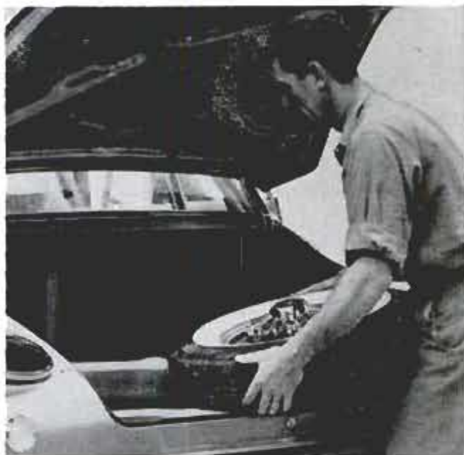
Rear end of the Valiant. Spare fits in a floor well. Trunk lid slopes down sharply from window to bumper
