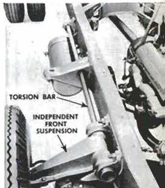
Left, light-duty rear suspension. Note frame kickup. Right, heavy-duty front suspension with torsion bars
