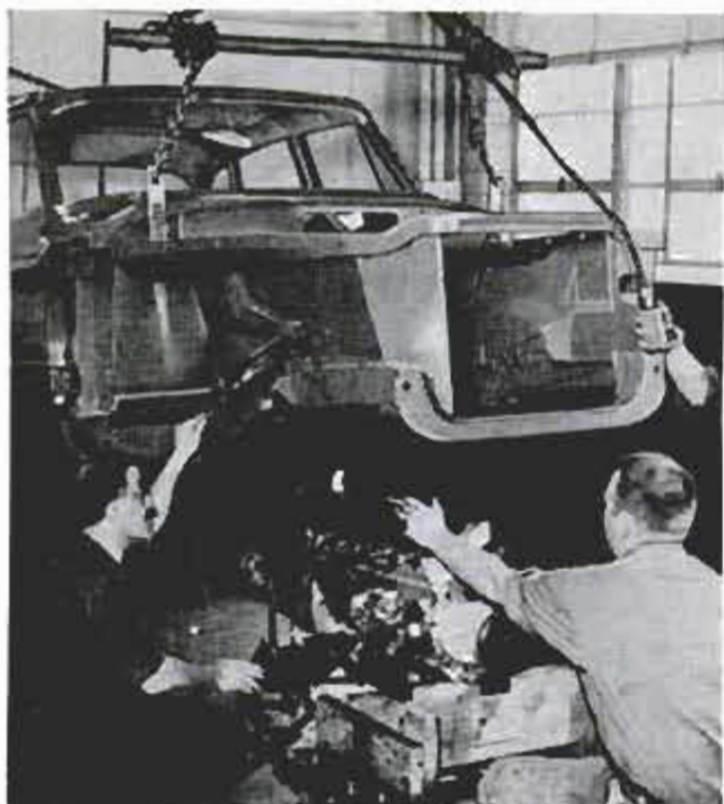
Valiant's unit body has no frame, the welded sheet metal providing the structure. Front fenders bolt on
