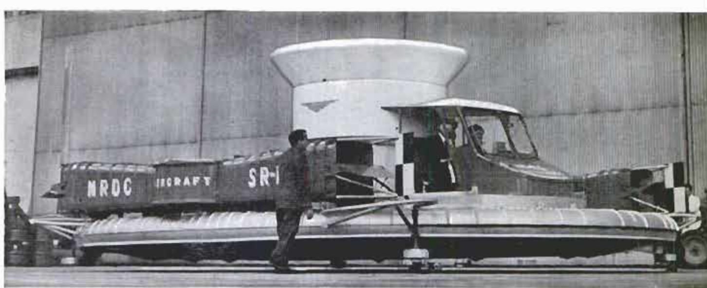
Saunders-Roe "Hovercraft" is 30 feet long, 24 feet wide, weighs 3½ tons and has passed its flight tests
