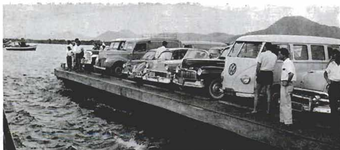
Ferry across Santos harbor docks sideways to allow the whole load of cars to drive ashore at once
