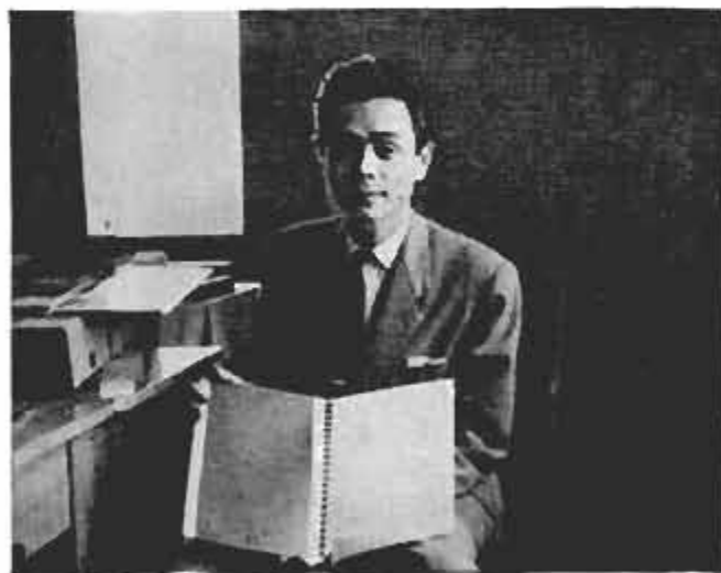
Sheets in album have pictures on one side, recording on other. Sheets are removed and played by machine
