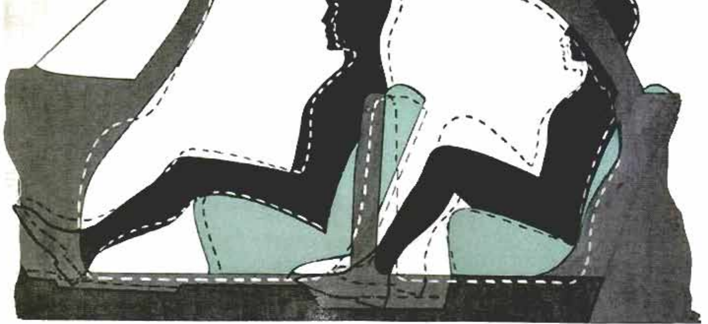
Above, dotted lines show last year's body, solid lines this year's. Deep footwells increase room and the narrower posts and roof make entry easier. Below, plastic figure is used to test out a 1960 Dodge front seat
