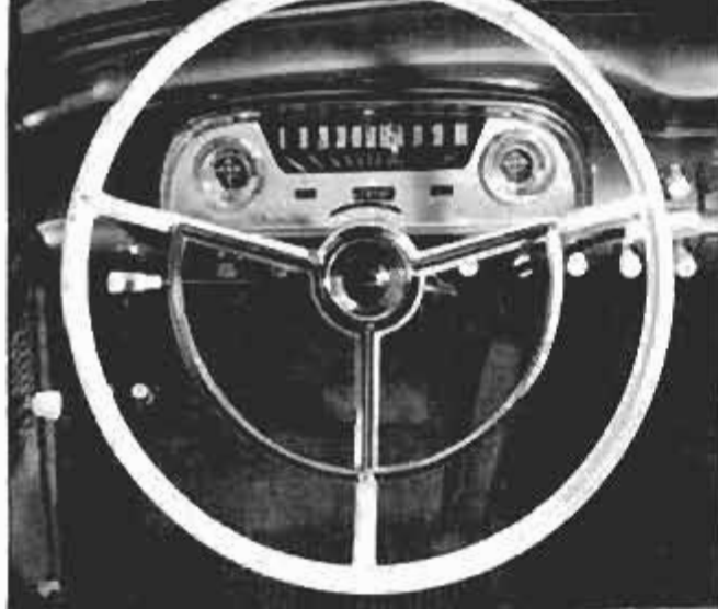
Instruments are well planned. Gas and temperature gauges are needles, the others are warning lights
