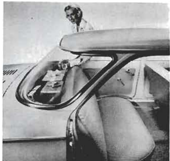
Gas-tank filler pipe is in left front fender. Tank is under the floorpan. Below, there's more luggage space behind the rear seat. Note amount of leg room
