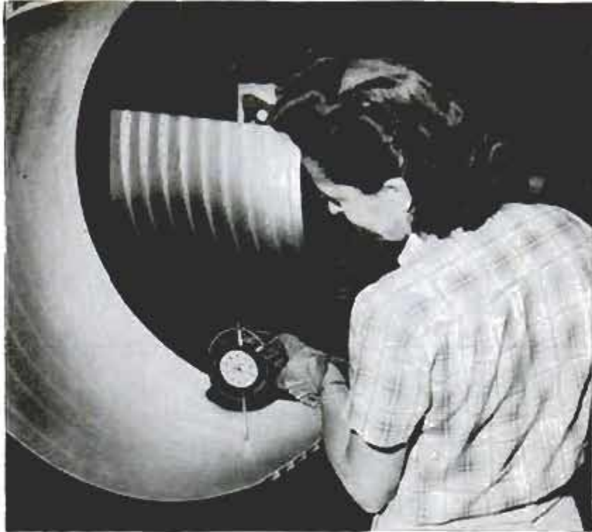
Left, examples of electrolytic drilling and recessing in superhard metals. Cord shows how hole was drilled in from surface and out on adjacent side. Right, micrometer is used to check thickness after chem-milling
