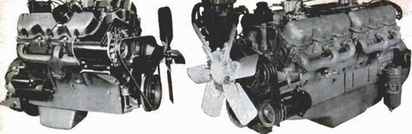
Left, the 305-cubic-inch V6, smallest of the line. Right, the 702-inch V12, made by tandemming two V6s
