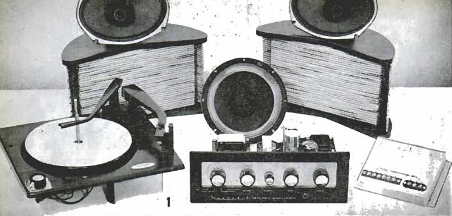
Electronic components of kit, Fig. 1, include preassembled record changer with stereo cartridge, parts for amplifier and speaker network, and 3-unit speaker system. Under-chassis views of amplifier and speaker network, Fig. 2, illustrate wiring simplicity made possible by new 2-in-1 amplifier circuit
