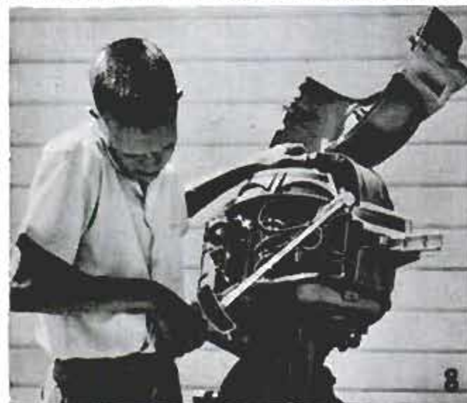
Below, use torque wrench to tighten cylinder-head bolts; be careful not to exceed recommended pressure
