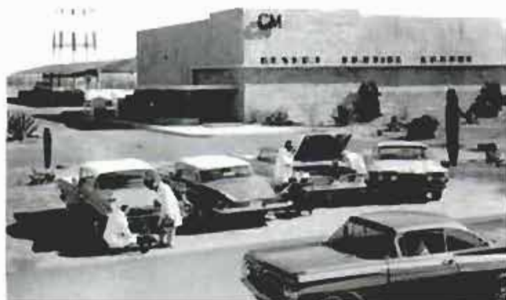
The GM Desert Proving Grounds simulate the most severe summer conditions. At the same time, other parts of the country are chosen to reproduce winter and extreme altitude conditions.
