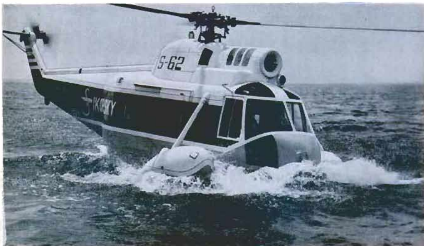
The hull of this turbine-driven amphibious whirlybird, unveiled this year, weighs less than the land type
