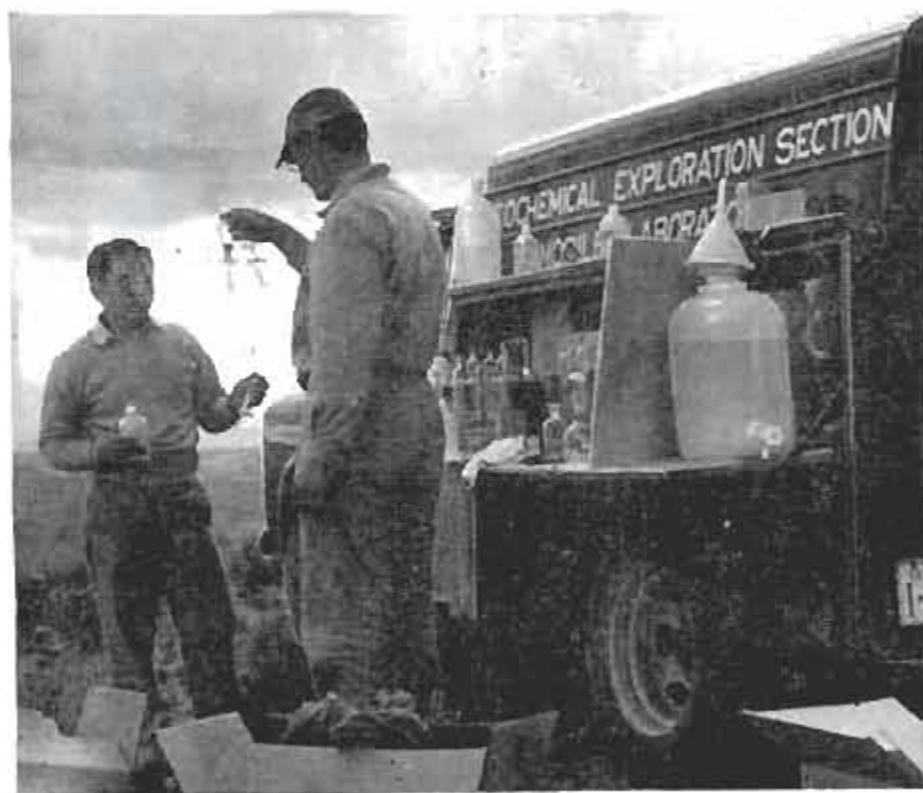
To identify an unknown metal found in a sample, U.S.G.S. teams compare the color of the sample with standard reagent
