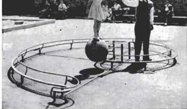
Girl can easily balance herself on wooden ball, since it can move only backward and forward while following spiral rail
