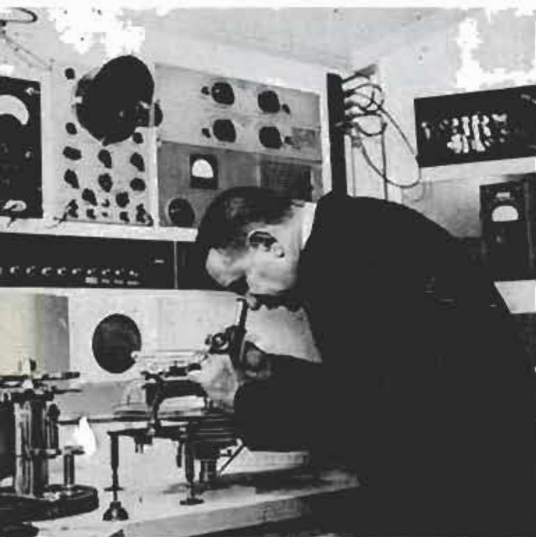
Scott uses microscope to see that grooves are cut correctly on test record made in his home studio
