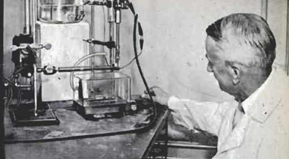
Early laboratory setup for electrolytic milling. Work is rotated by geared motor under glass "tool" at right side of apparatus
