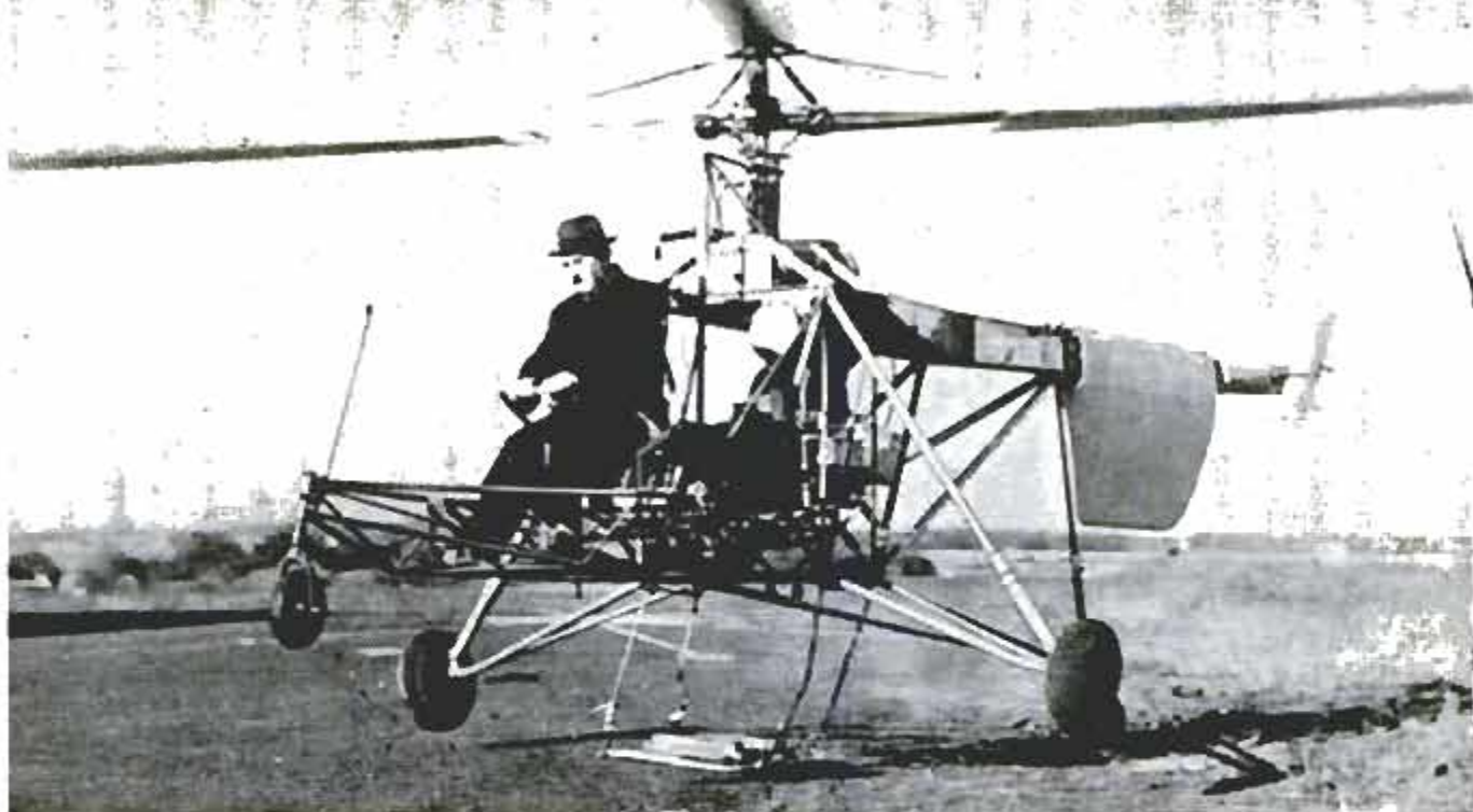
First serious bid for vertical flight was the VS-300, shown above still anchored to the ground for safety
