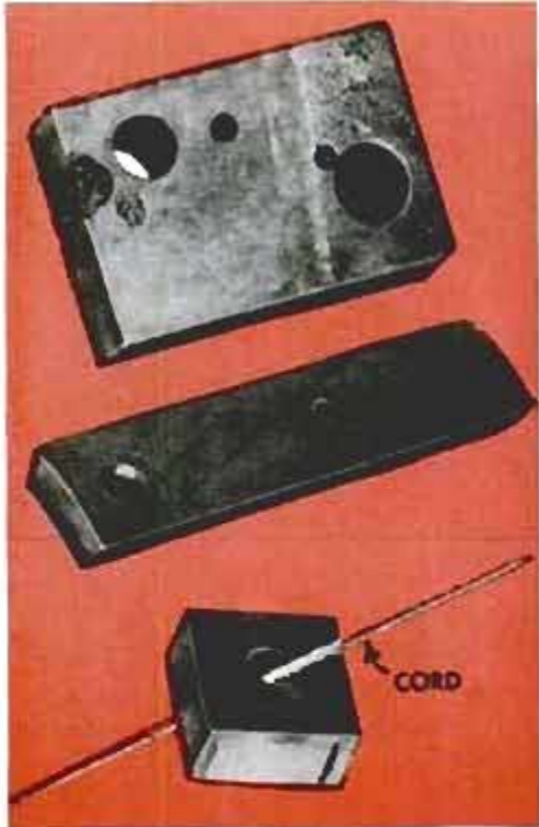
Left, examples of electrolytic drilling and recessing in superhard metals. Cord shows how hole was drilled in from surface and out on adjacent side. Right, micrometer is used to check thickness after chem-milling
