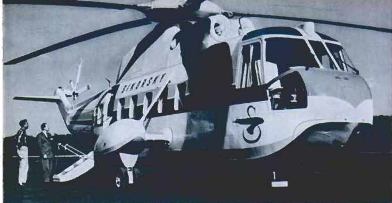
Full-size model shows what 1960 travelers can expect. The S-61 gas-turbine craft will carry 25 passengers
