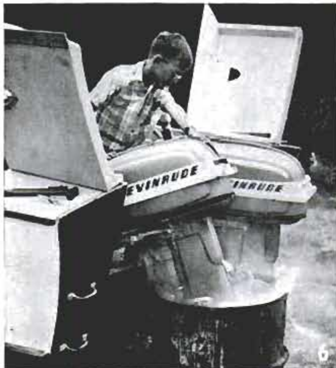
Above, to clear salt water from motors, run them in drum of fresh water while still mounted on transom
