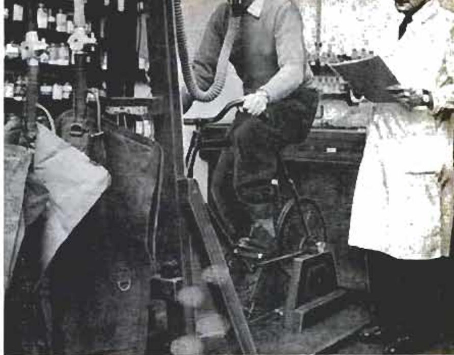
Dr. W. R. Wilkie (on machine) helps aviation scientists test amount of horsepower man can produce and for how long
