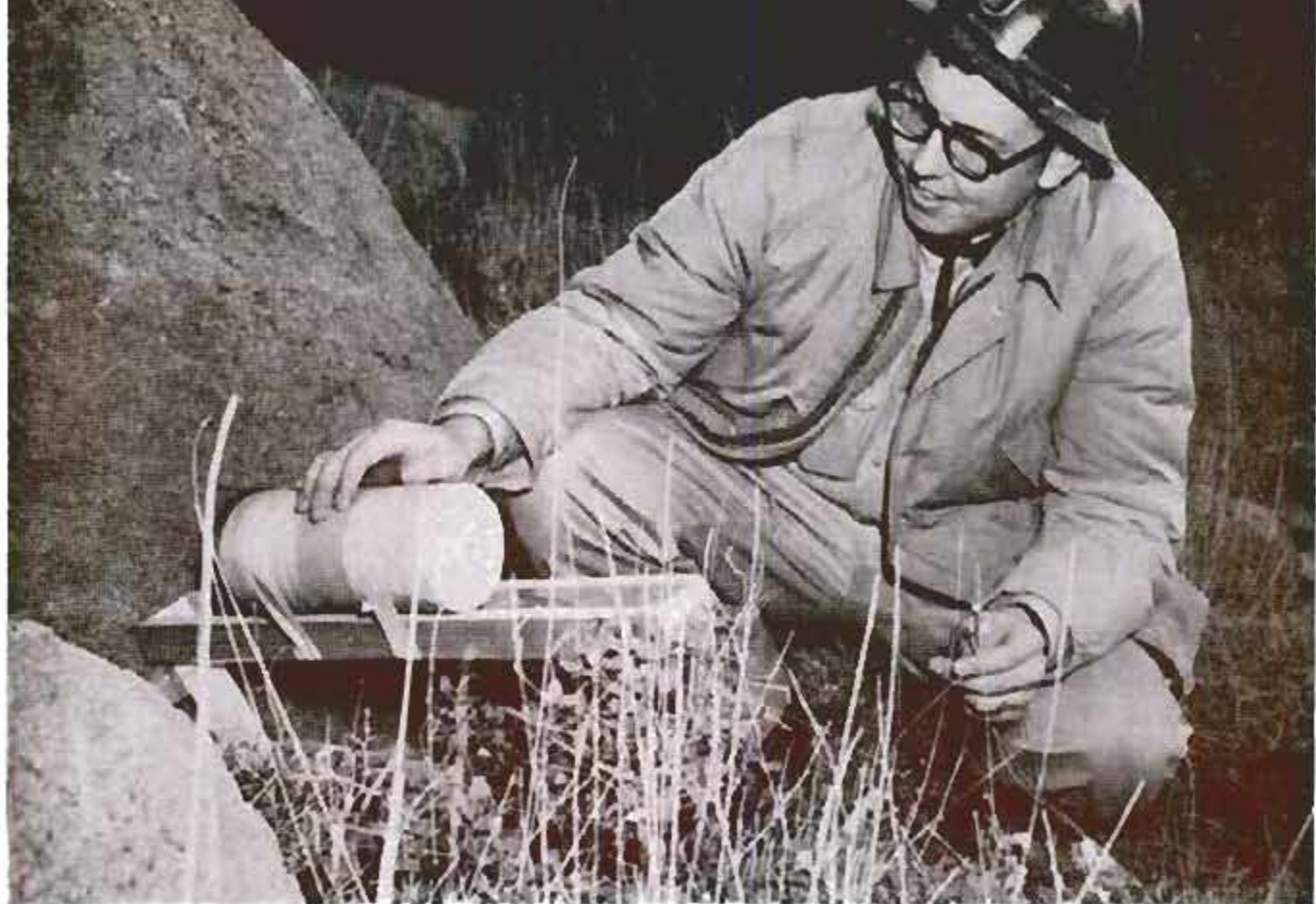
Dr. Carl Austin prepares to set off shaped charge that uses bazooka firing principle to drill into hard rock
