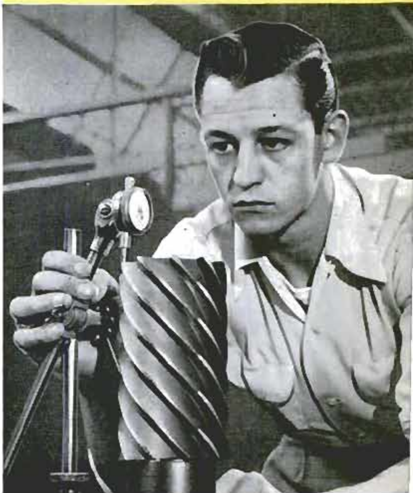
Slab-milling cutter, a sort of planing mill for metal, is checked for clearance on its heavy-duty roughing teeth. Grinders keep edges sharp to hairline tolerances
