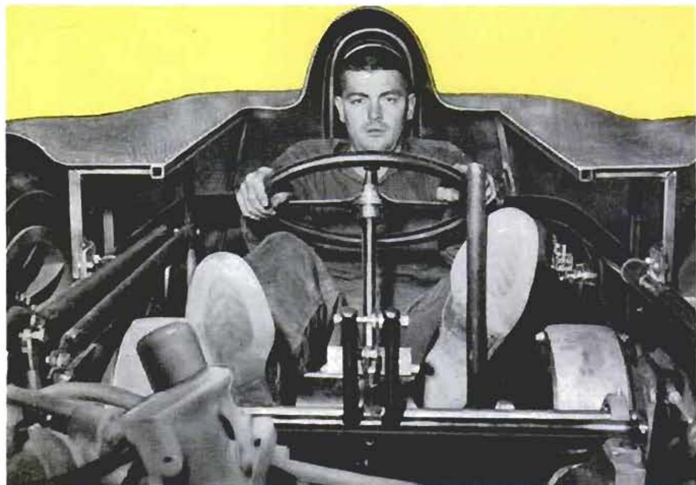
Thompson sits far aft, his legs resting atop the rear axle, his eyes just an inch above the top body line
