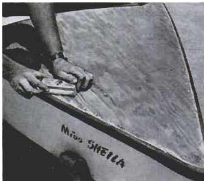
2. Above, hardened putty is sanded flush with deck. Remaining depressions are puttied and sanded again
