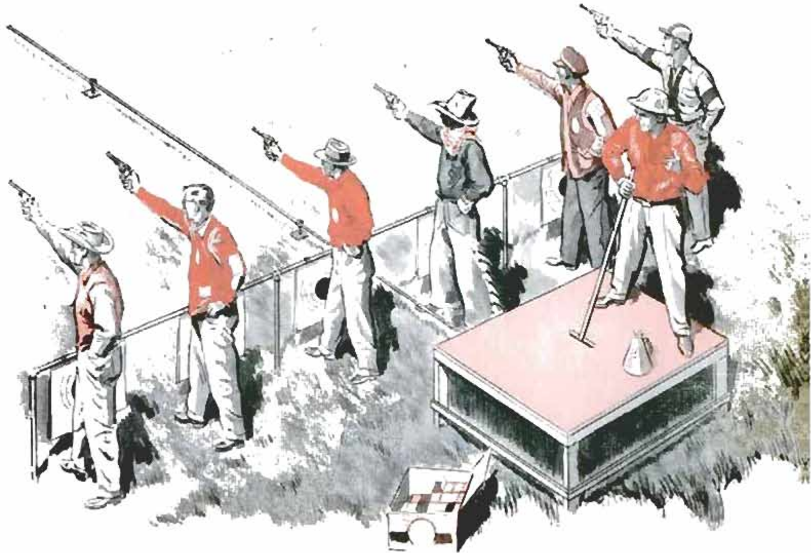
Erected in a row in front of an earth bunker, the sections of the rack, each of which contains three target holders, are bolted end to end between supporting posts. Standard paper targets slip into the holders
