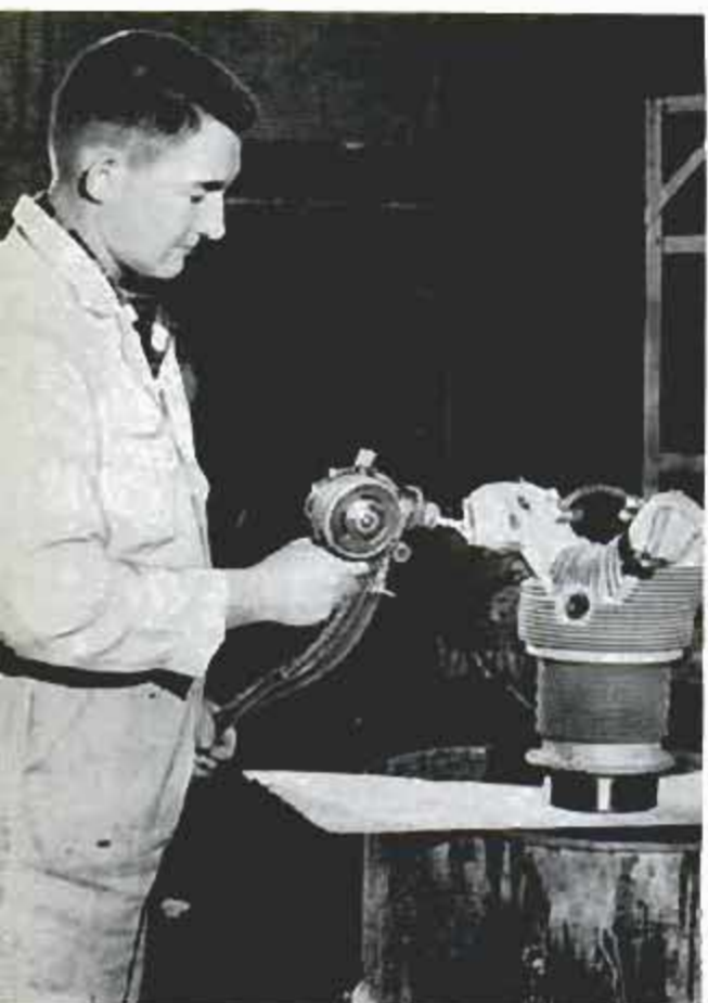
Another brainstorm led way to preventing corrosion, by spraying molten zinc-aluminum alloy on planes with a metalizing gun
