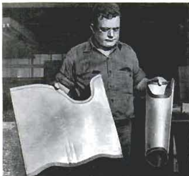
At left, inventor Alvie Twiss shows freshly cut and stitched legging. Finished product is in other hand
