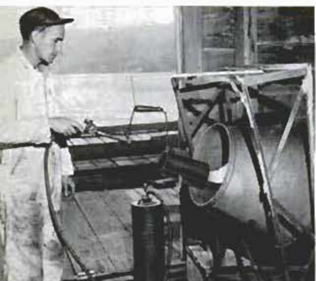
Sand for sand-blasting comes from a nearby glacier. Too moist, it is fed into a cement mixer and dried with a weed-burner
