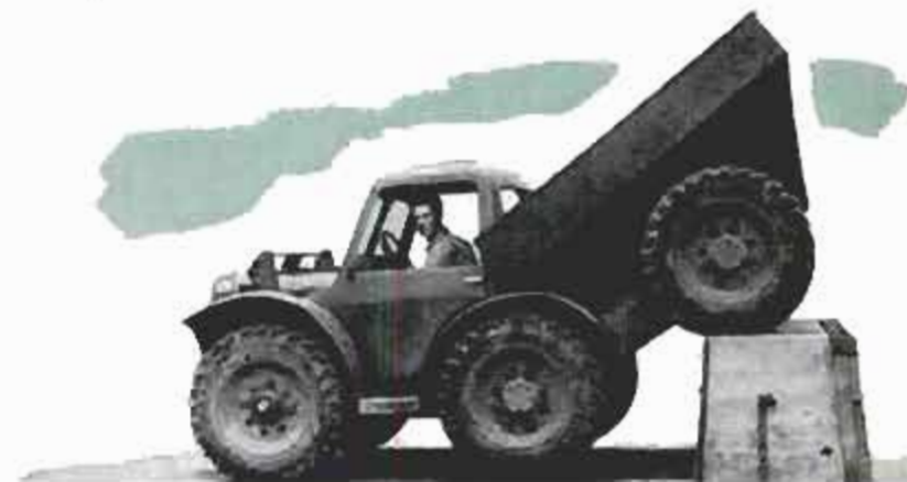
Center wheels drive the truck forward until front wheels touch down, then center wheels can be lowered and the truck is over
