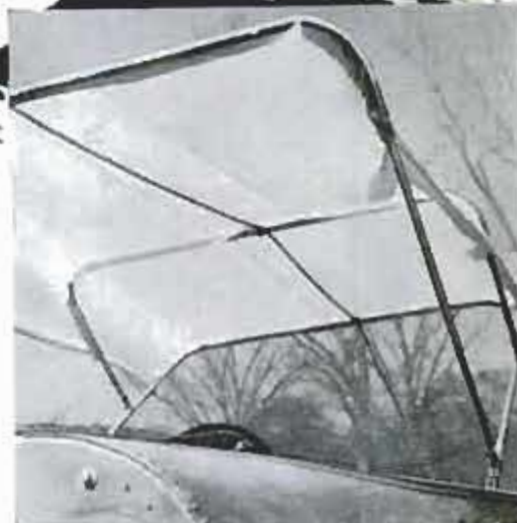
4. Rope knotted to each frame at center holds them in position while canvas is fitted on frames and pinned in place temporarily
