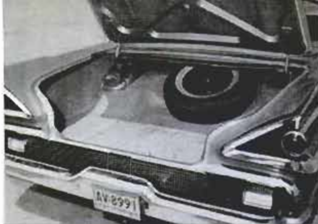
Mercury makes its trunk space more accessible by mounting the rarely used spare tire forward
