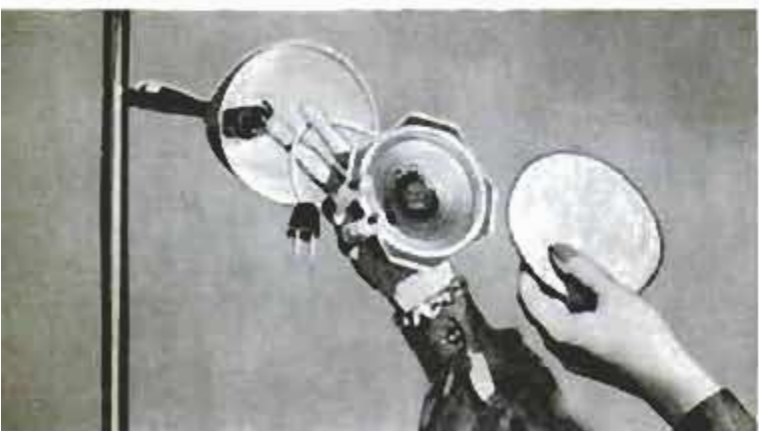
Adapter plug, speaker and grille-cloth assembly replace light bulb. Friction holds parts in place
