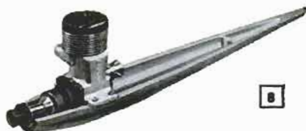
Along with a control unit, here are the two additional parts you must buy—a racing-type engine and a magnesium pan to which engine is bolted. Mounting holes drilled, then tapped in
