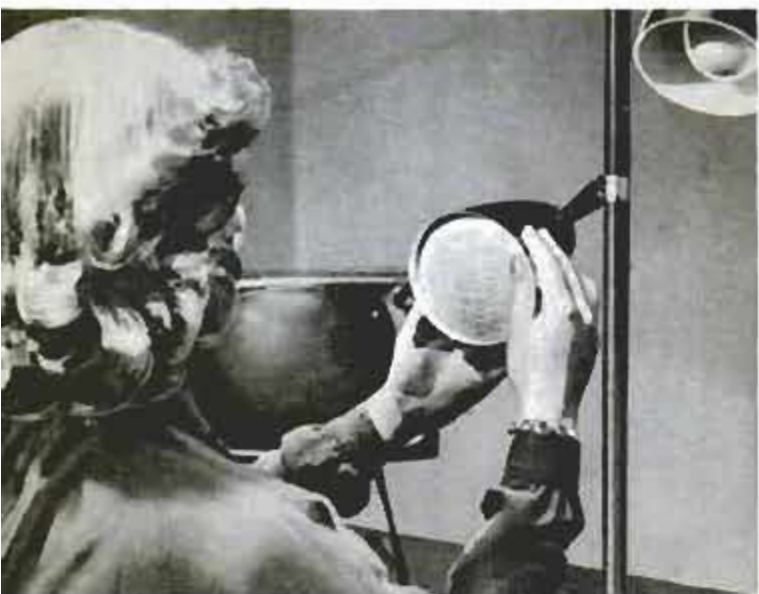
Concealed in pole-lamp "bullet," speaker permits personal TV listening without headphone discomforts
