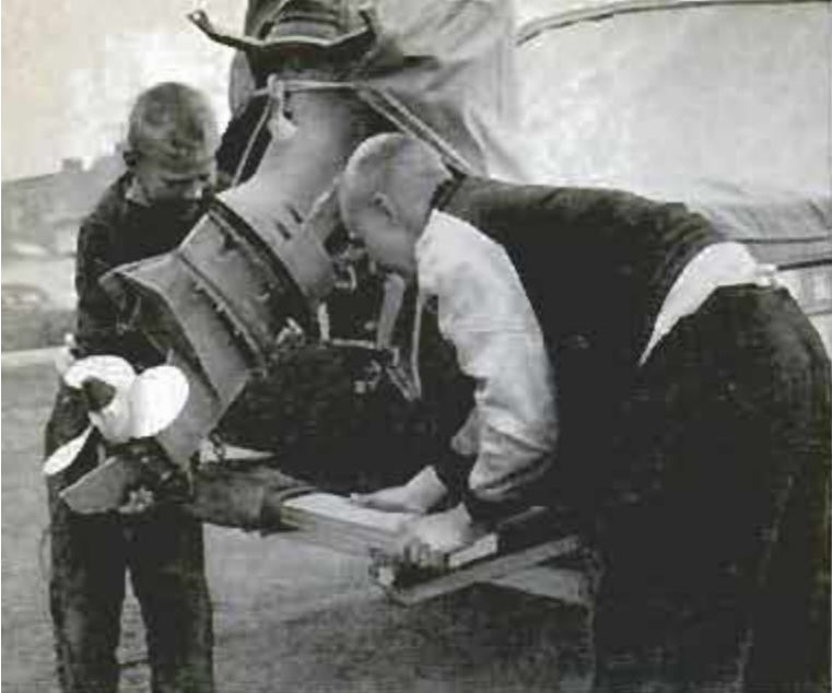
When the propeller started to scrape on ruts in road-repair area, Harry stopped at next wilderness village and built a tilt brace from a two by four
