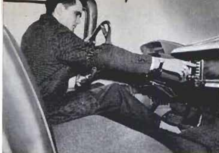
High on the complaint list is the hard-to-reach location of the radio, caused by the forward position of the dash
