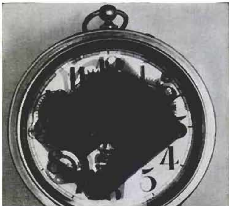
Inner parts of alarm clock black out the hands in this photoradiograph, but all the numbers are visible
