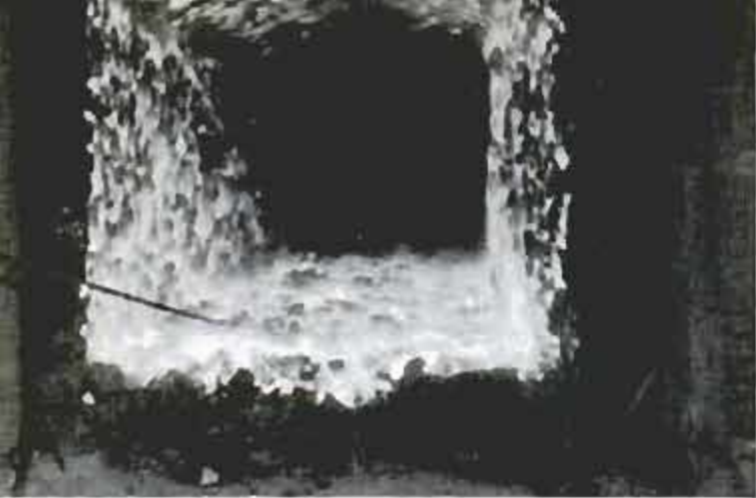
Coal fire burns brightly inside experimental mine. The fire was one of nine started deliberately to test the new "foam plug" technique. Six of the fires were controlled by the foam, three of them were not
