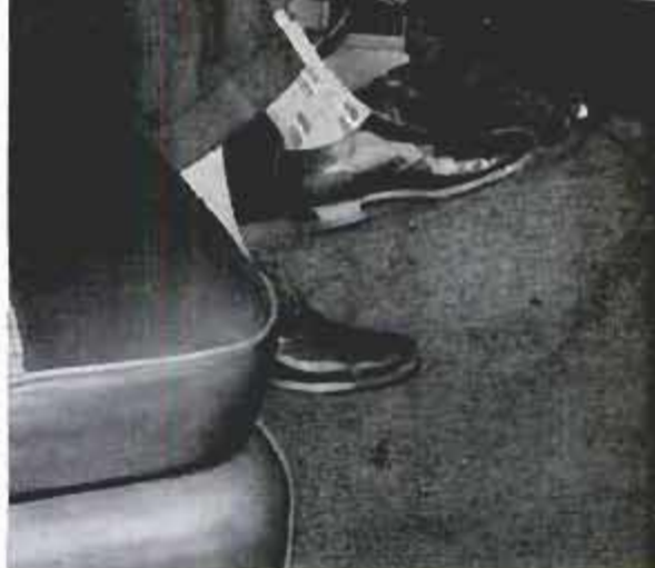
Mercury's lower front-seat floor hump provides the center passenger with sufficient legroom
