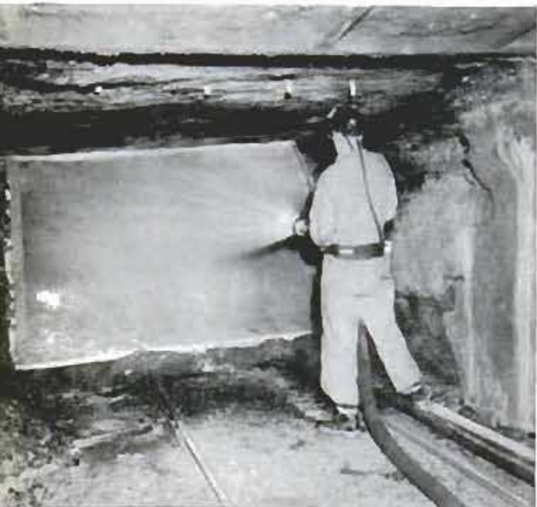
Far from the fire, a researcher sprays bubble-making solution across a net. Large "plug" of bubbles forms, which is carried to the fire by ventilating current
