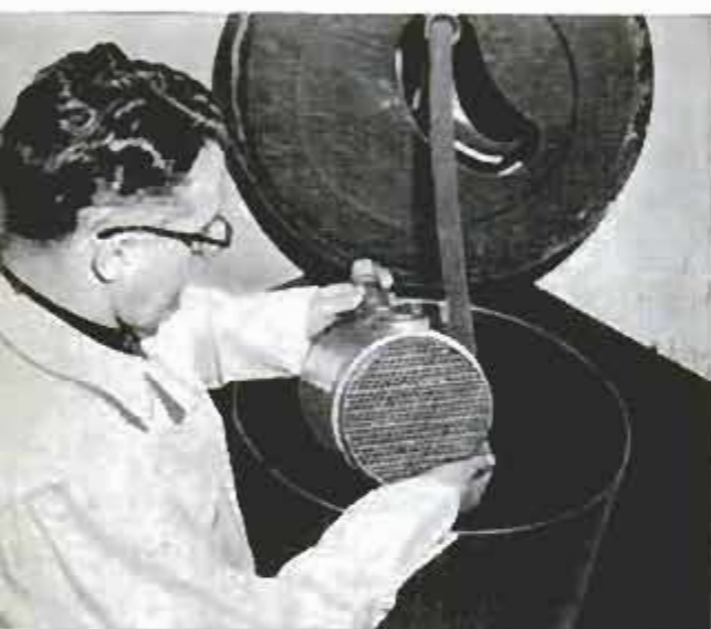
ACA's oil coolers are cleaned in, of all things, a washing machine. The machine runs cleaning fluid throughout the cooler
