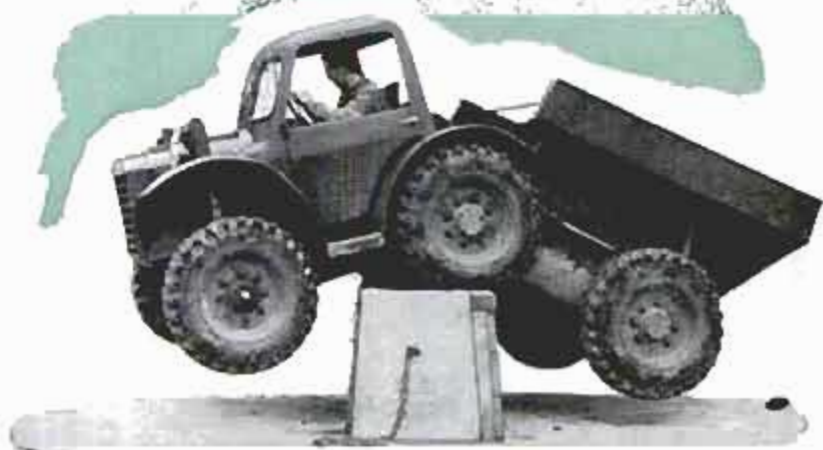
With front wheels up on top of the wall, the rear wheels push forward and the center axle is arched to support the weight
