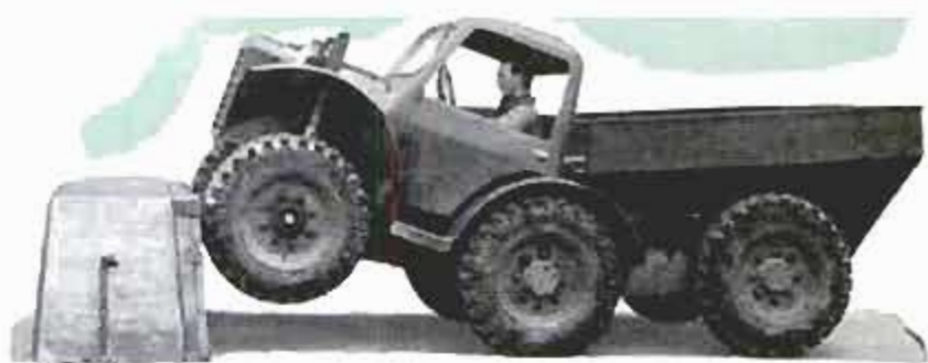
As the truck approaches the wall, the driver raises the front axle by means of the hydraulic jacks (visible behind fender)
