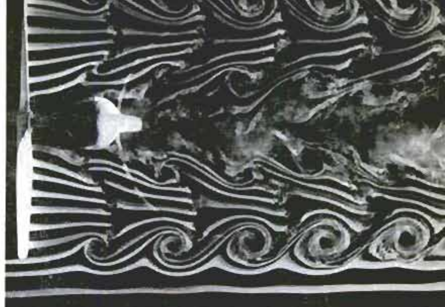
Here a model of a plane propeller is turning at 4080 revolutions per minute. The smoke shows a highly organized pattern, proving that distinct whorls are formed, and pattern is endlessly and precisely repeated as propeller moves through the air
