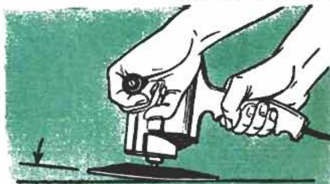
HOLD AT SLIGHT ANGLE FOR SMOOTH CUT
