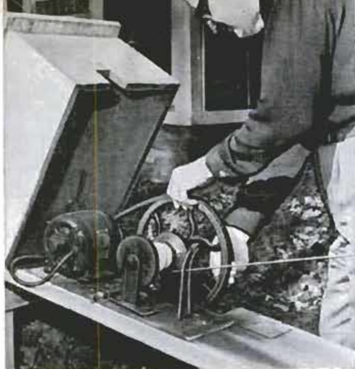
Electric motor belted to the flywheel of an old sewing machine winds up a line to pull locomotive up the track
