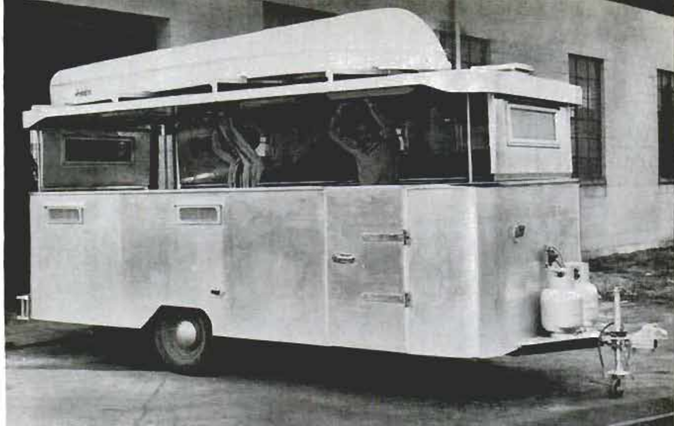
Upper-wall sections fold against the roof, which then is lowered to form the compact road unit shown below
