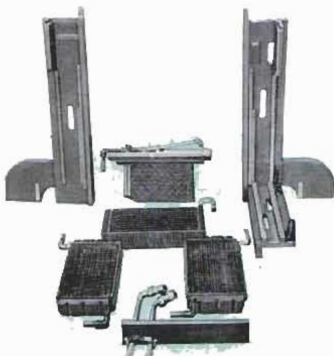
Below, connections are made between radiators with garden hose, copper tubing, and pipe where necessary. Components shown at left, before assembly
