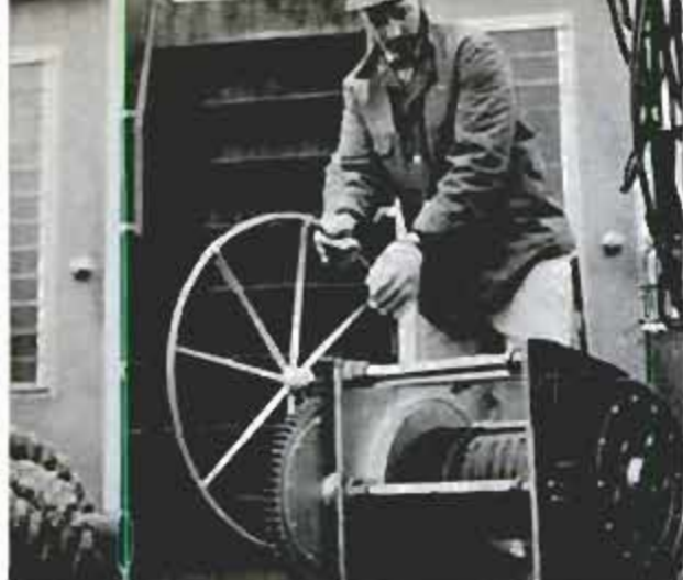
Winches made of old tractor parts take up slack in the Robert L. 's towing cables
