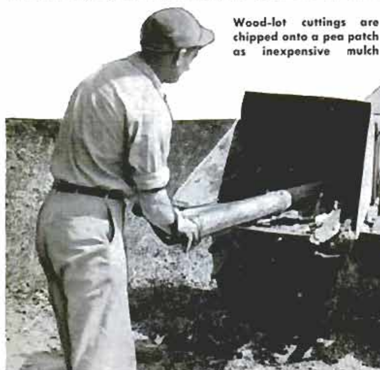
New chipping machines will turn out chips of any size. Operator can make adjustments to the machine, or select different blades
