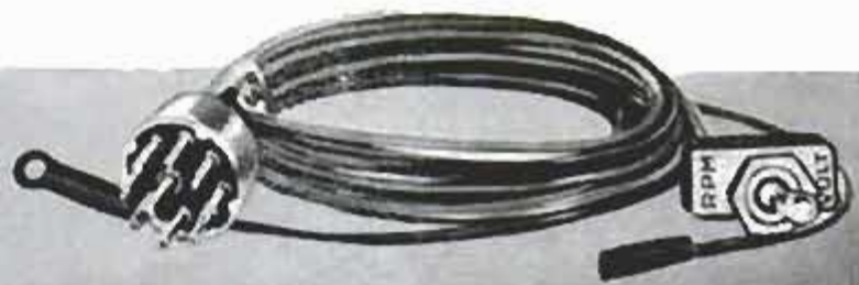
2. "Voltack" tachometer has voltmeter included in head with ignition-impulse detector. Flipping switch one way shows engine r.p.m., flipping it other way shows voltage output of battery to check its condition
