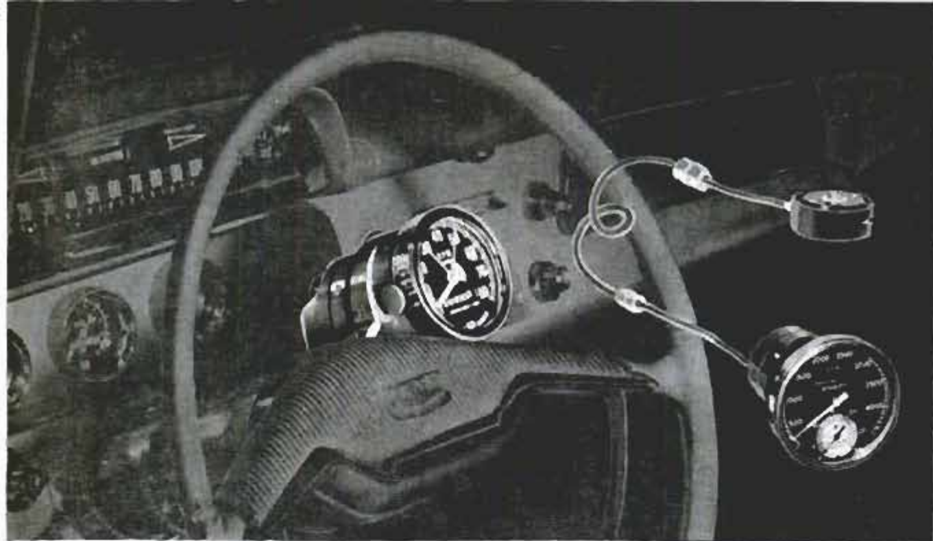
1. Sending switch for Stewart-Warner tachometer fits between distributor and cap, wire leads to head
