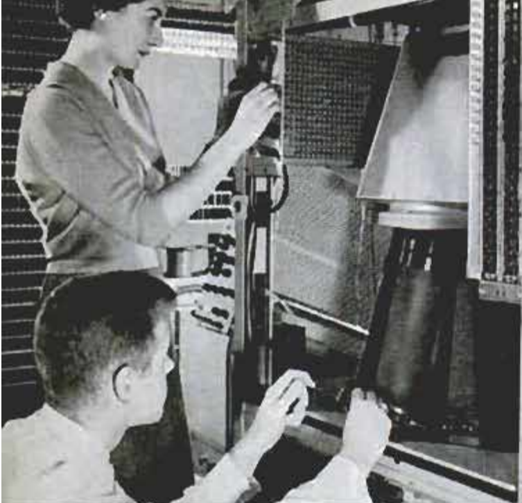
"Flying Spot Store" prototype for electronic telephone exchange is vertically mounted unit shown here
