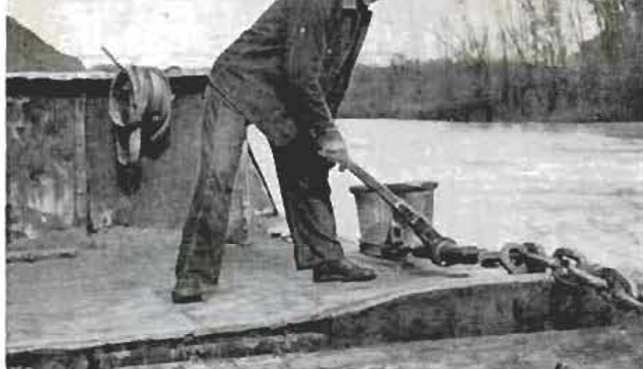
Sharp corners in the narrow river keep crewmen busy adjusting tow slack. Adjustment is made by slackening or tightening a ratchet coupling on chain between the boat and the barge
