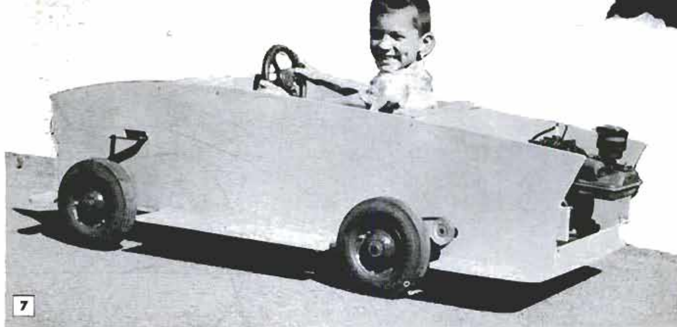
Your anxious youngster can drive the car before the body is constructed, or body simply can be omitted
