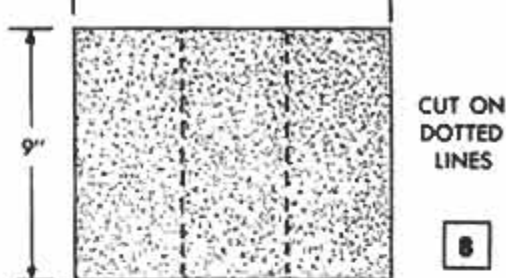
SHEETS FOR PAD SANDER CUT FROM 9" x 11" ABRASIVE SHEET
