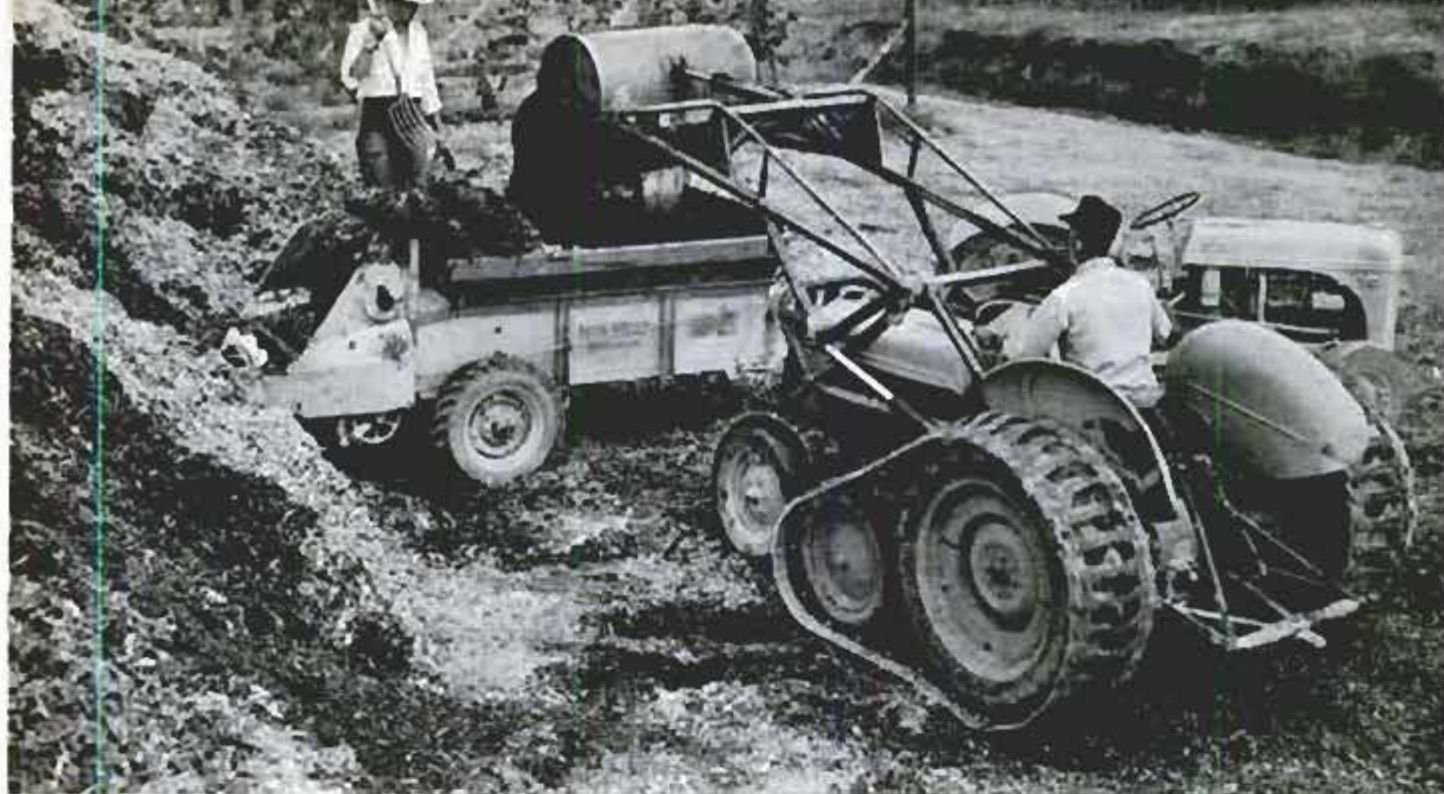
Front-end loader digs into a huge pile of chips and drops them into a spreader to mulch a grape plot
