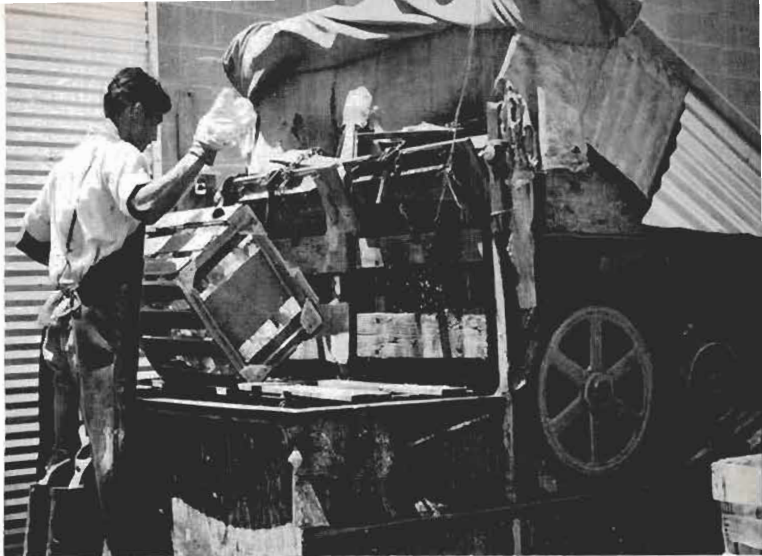
Powered by electric motors, this machine bathes jugs in solution of wetting agents, caustics and solvents
