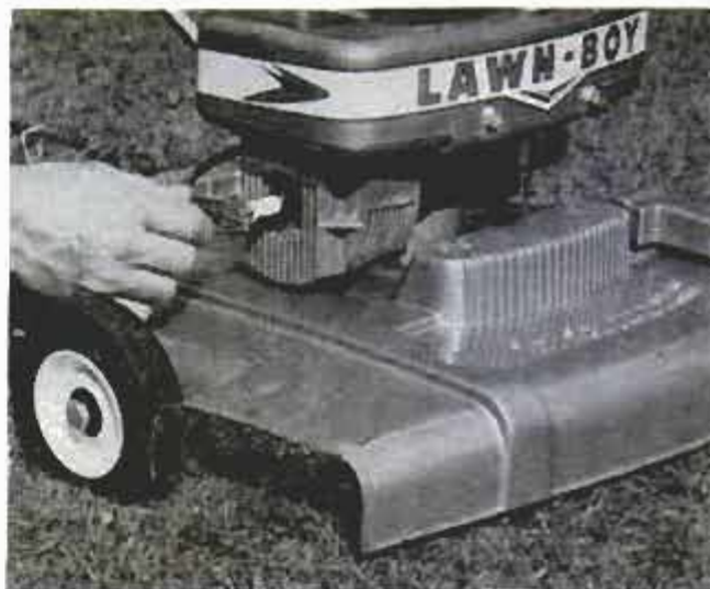
Play it safe and always remove lead wire from spark plug before ever touching blade of rotary mower
