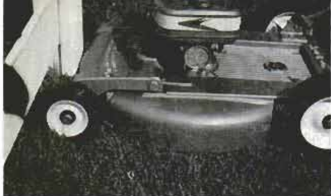
Front-trim feature on most rotary mowers permits trimming to within fraction of inch of post, tree
