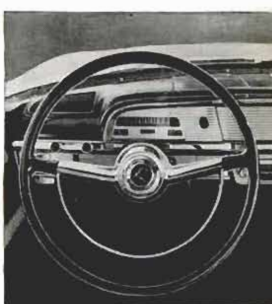
Dash instruments are very small and simple. Speedometer scale has numerals jammed together in central 30-to-70 section where speed information is most valuable. Charts at left show gasoline mileage claimed by owners
