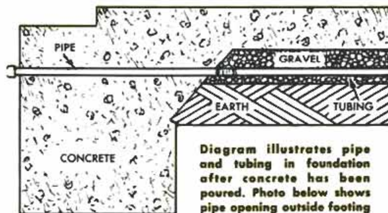
View above shows installation of pipe in gravel fill
