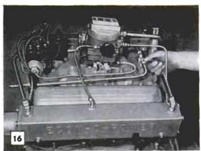
Tubes connected to cover plate discharge water into exhaust pipes to cool them and silence exhaust noise
