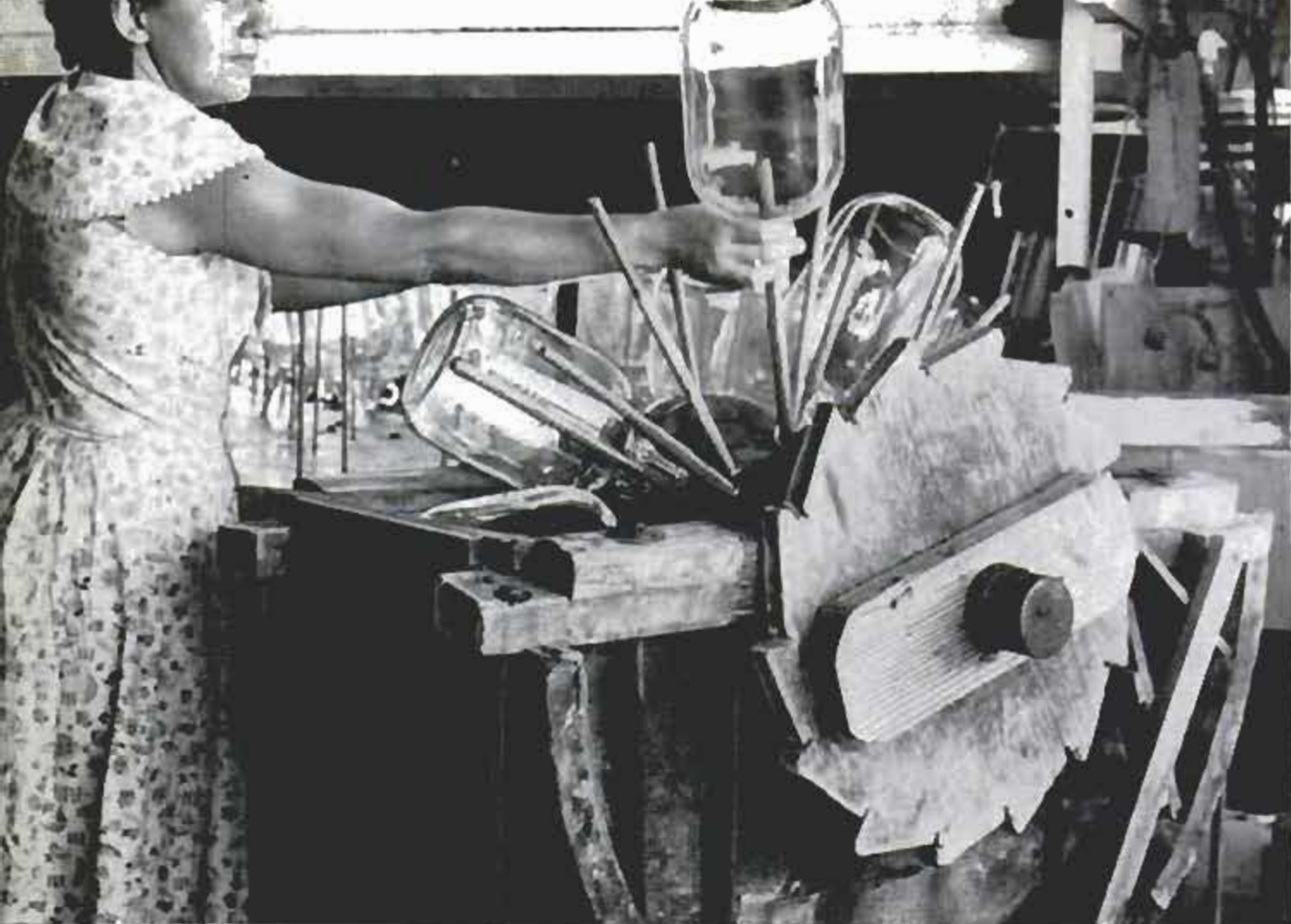
When ordinary laundering doesn't do the job, jug is placed on machine that immerses it in muriatic acid
