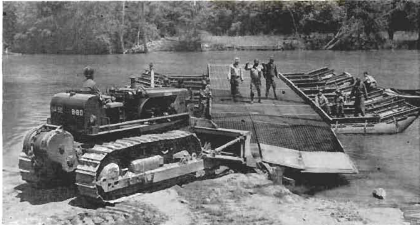
Graduate of school, assigned to 5th Engineer Battalion, pushes stranded pontoon-bridge section off pilings. He will then maneuver his International Harvester TD-18 aboard and float across to other side of river.
