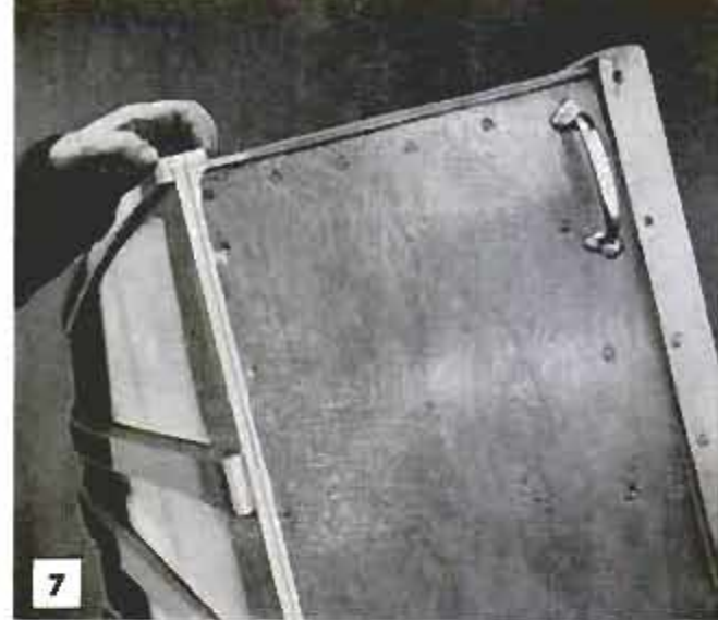
7 Chine-molding strip cut from 1 x 2-in. oak, protects chine from damage, can be easily replaced if broken
