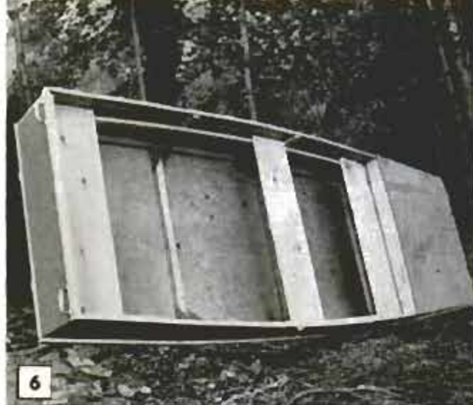
6 Window lifts that are through-bolted to upper corners of transom and bow, serve as carrying handles
