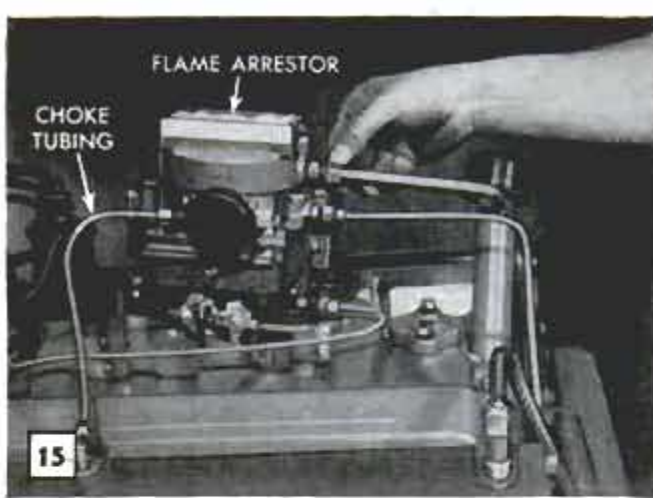
Flame arrestor removes smoke and fumes from engine compartment, provides ventilation for crankcase
