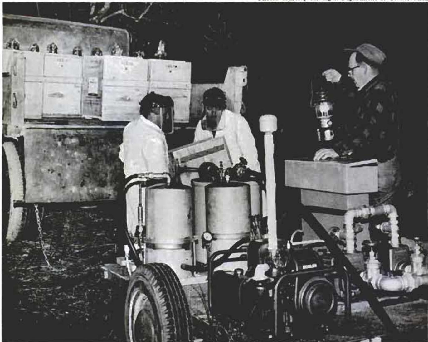
Portable fluid-proportioning machine meters the lamprey poison through a perforated pipe on stream bed
