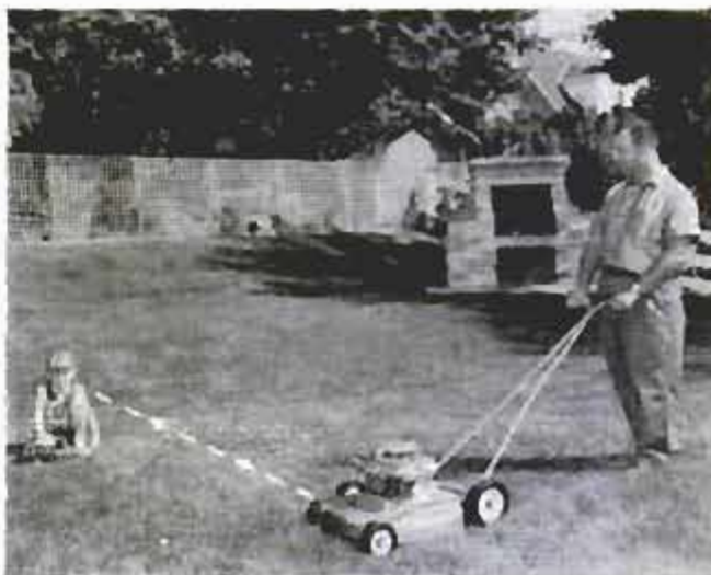
Don't let child or other person be in direct path of discharge chute—they could be hit by flying object
