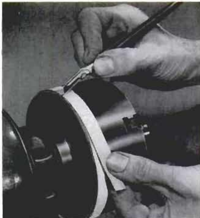
To make a true butt joint, wrap paper strip once around chuck body and cut through both thicknesses
