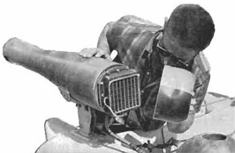
Jet, shown here with cover off, generates temperatures up to 2300 degrees. Below, Pearson adjusts the master gas valve
