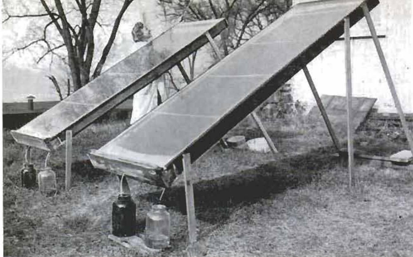
Another kind of solar still, under tilted glass, consists of sandwich of wicks and condensation layers
