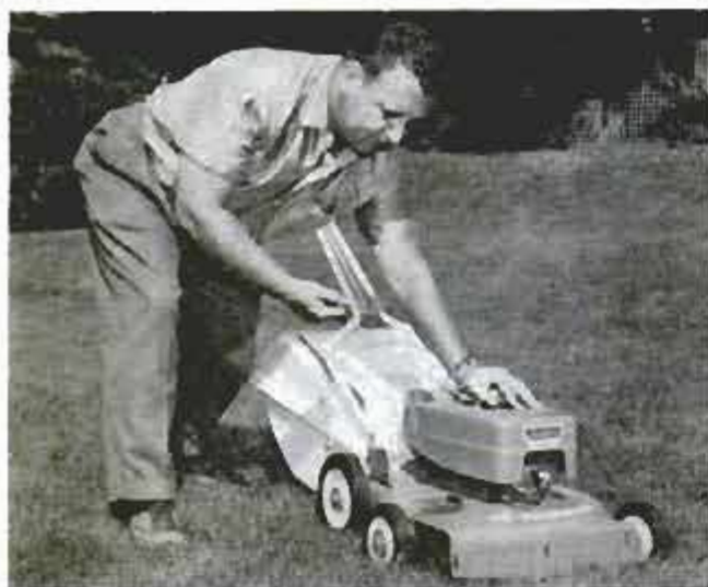
Safe position for starting mower with rewind starter is to brace self with hand on starter housing
