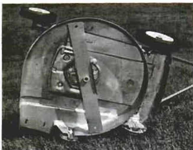
Above, underside view of deck shows typical bar-type blade. Note smooth channeling of underdeck. Below, disk-type rotary-mower blade has four reversible blades, giving greater number of cutting edges
