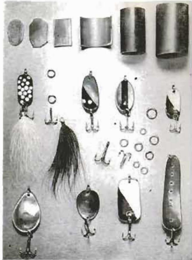
Spoons can be handmade from scraps of metal and a few simple accessories such as split rings and hooks
