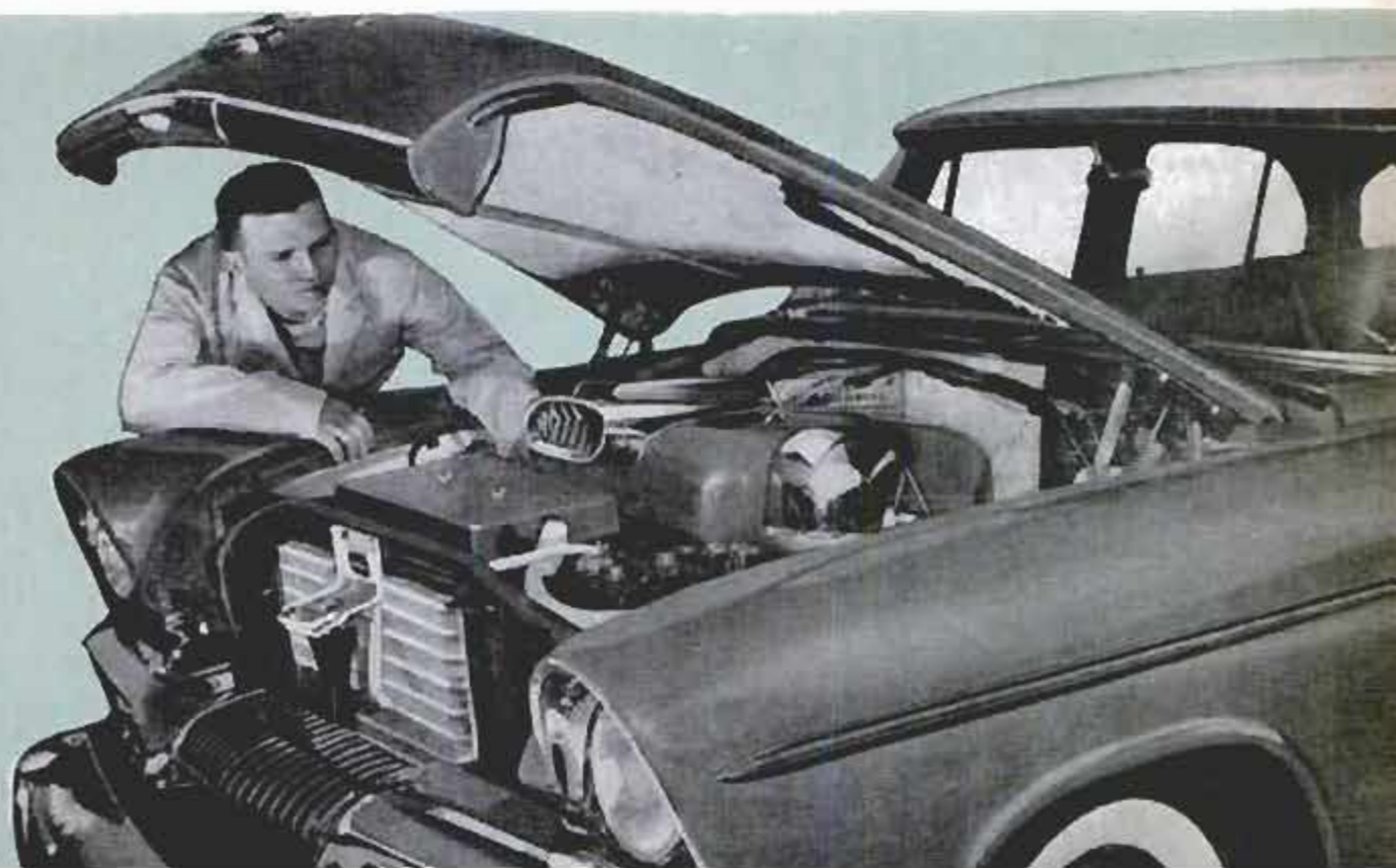
Soundproofed hood covers the compact gas turbine which powered the Plymouth in its virtually nonstop run
