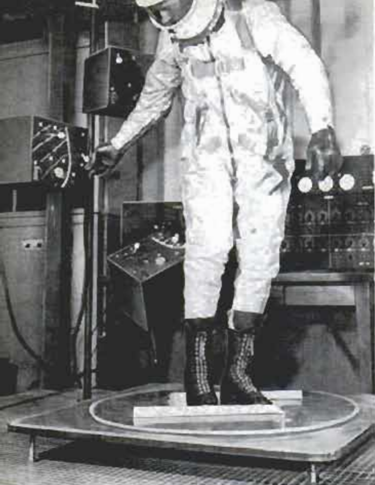
Test subject, standing on disk, literally floats on cushion of compressed air as he tries to flip switch
