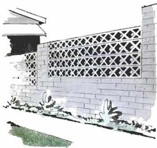
Attractive masonry wall combines regular 4-in. concrete building blocks with ornamental criss-cross ones Courtesy National Concrete Masonry Association
