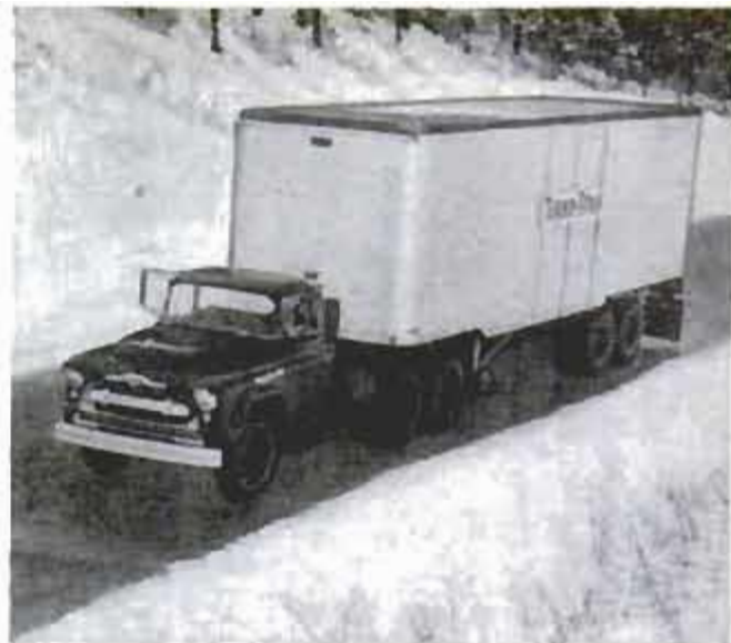
Chevrolet turbine-powered truck has excellent hill-climbing ability, low maintenance, burns cheap fuels
