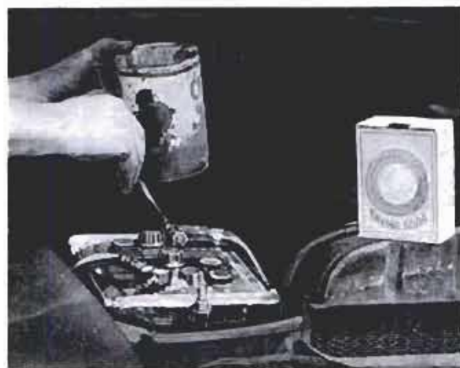
Fig. 5. Above, assure maximum efficiency from a battery by washing top with solution of baking soda and water, then rinsing thoroughly with clear water
