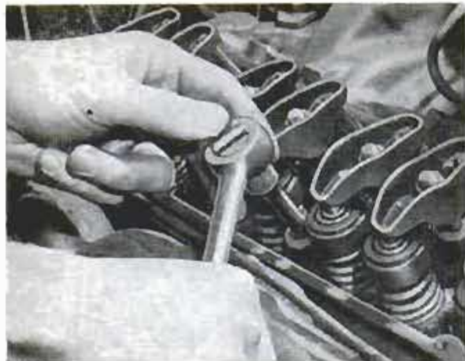
Fig. 9. Tighten up the head bolts, beginning at center and working toward each end. If torque wrench is not available, just "snug up" firmly on each bolt
