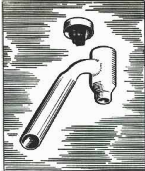
Fig. 3. Crankcase-breather pipes, such as this one, on inline engines should be removed and cleaned thoroughly
