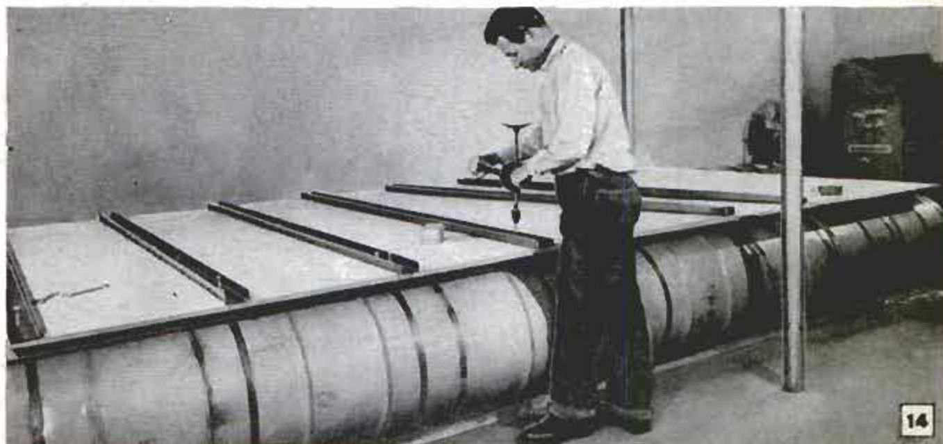
Beams are positioned on deck, spaced as required so that holes for deck bolts can be drilled accurately
