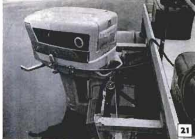
Above, control cables must have enough slack in them to avoid binding on sharp turns. Below, hoist makes easy work of lifting heavy motor from dock to boat
