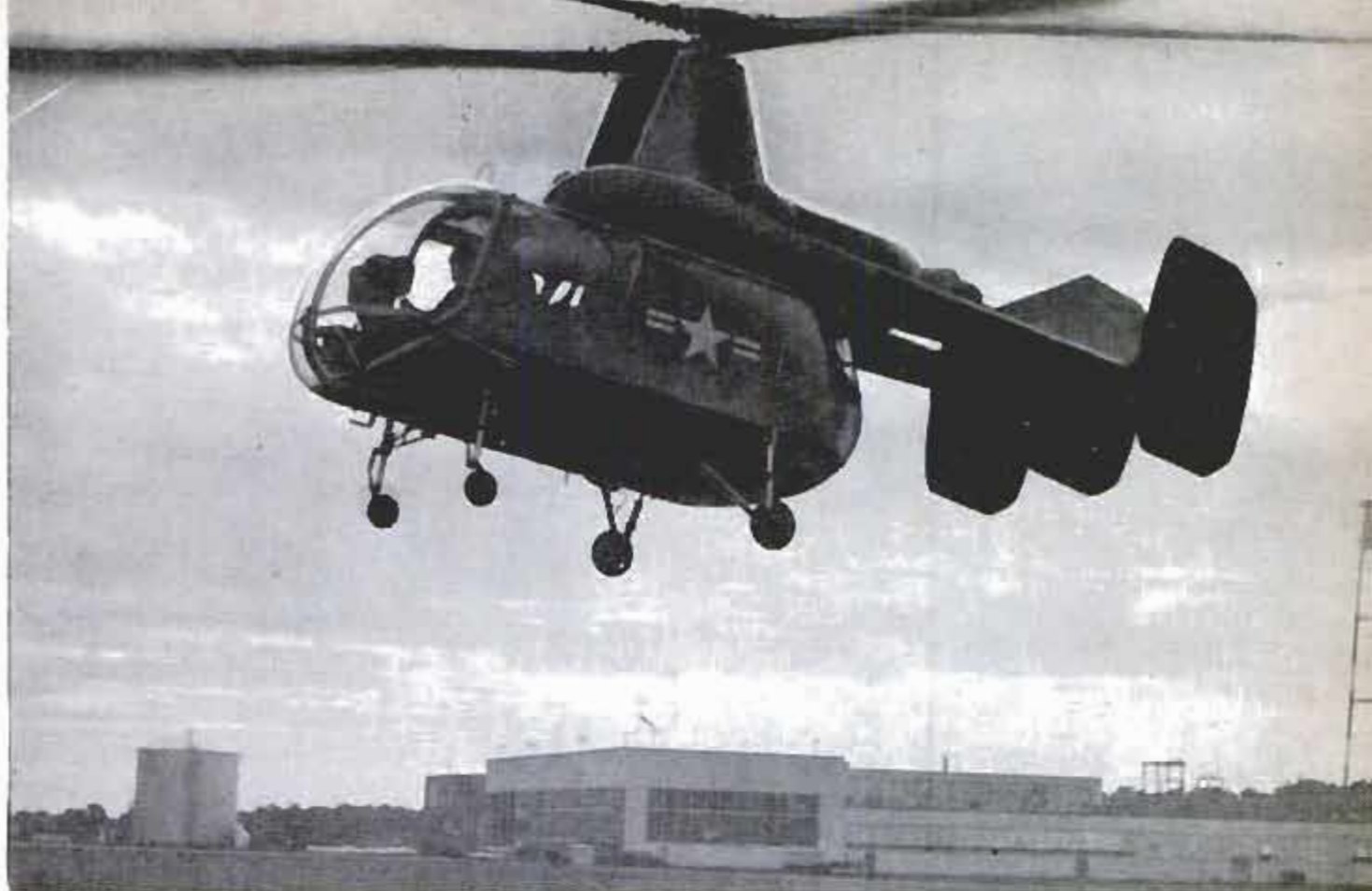
Kaman helicopter has 825-horsepower gas-turbine engine. A turboprop version of engine has 960 horsepower
