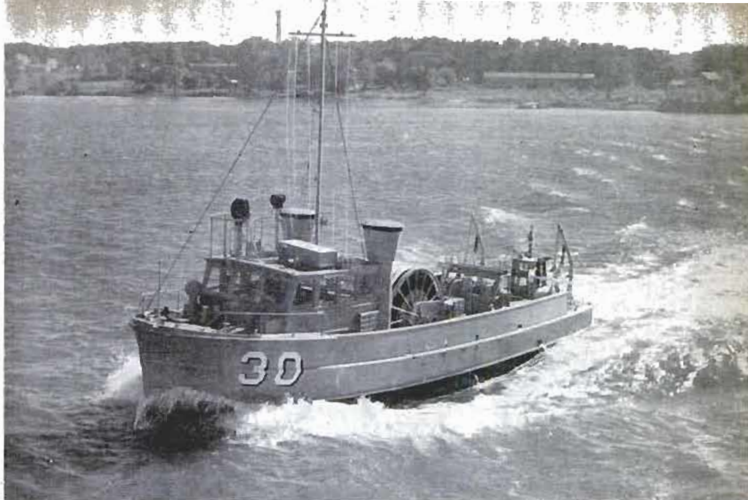
Two compact 500-horsepower engines produce the large amounts of electricity required by a minesweeper
