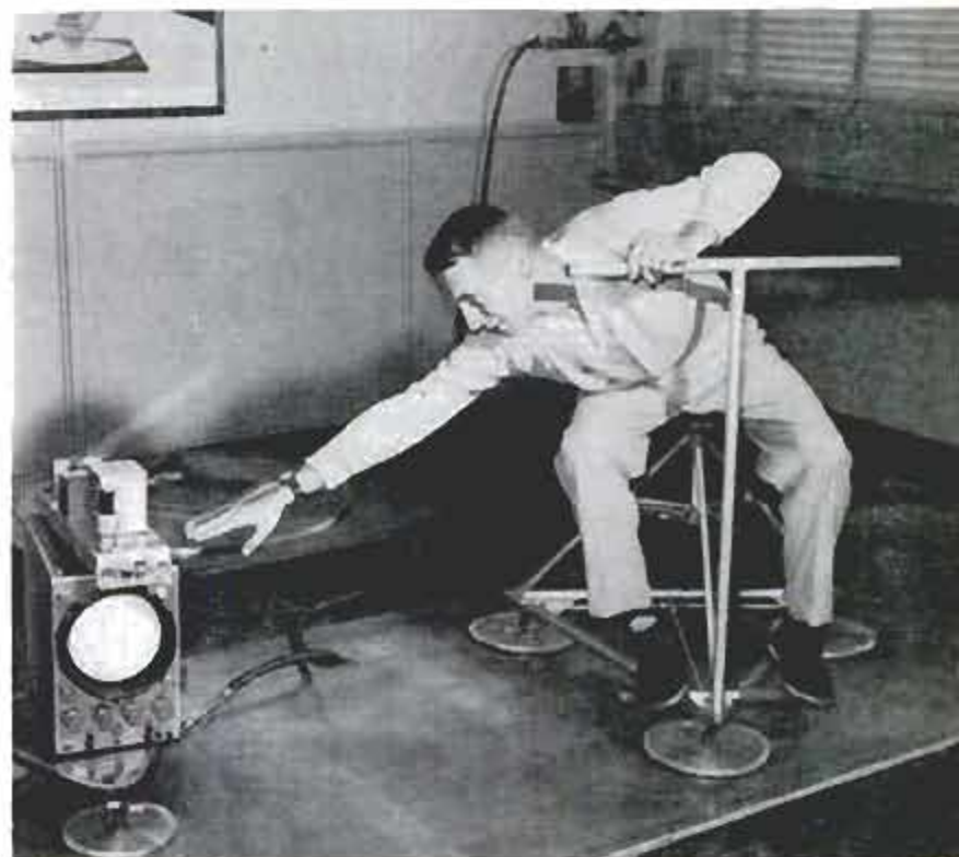
In this experiment, the subject rides a frictionless "tricycle." Framework is mounted on three disks with tiny holes in them, and electronic gear is mounted on similar disks. Compressed air is forced through holes to float the equipment. When subject tries to remove tube, he and electronic gear glide apart
