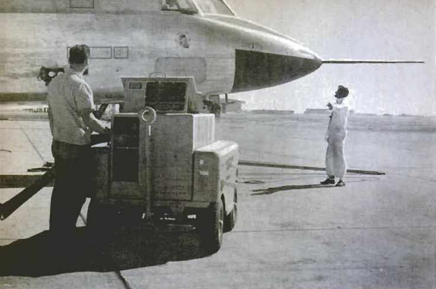
Gas-turbine ground unit starts a B-66 by spinning the jet engine with air taken from the unit's compressor
