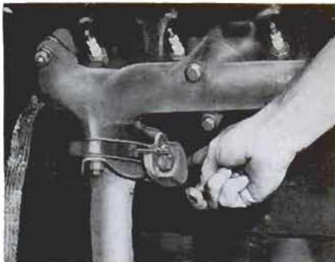
Fig. 10. If heat-riser valve on exhaust manifold does not work freely, pour penetrating oil on shaft, work valve back and forth until it will rotate easily
