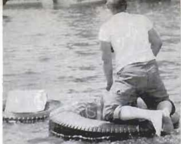
Simplest boat of all was two truck tires tied together. Motor was mounted on a crossbar inside one tire. Skipper just missed dunking in water
