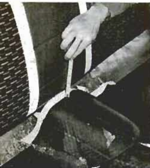
Tunnel under center of rear seat allows about one inch of padding
