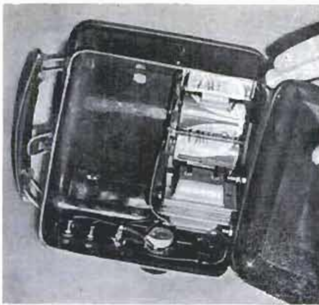
Electric stethoscope fits neatly inside child's metal lunch box that has handle for easy carrying
