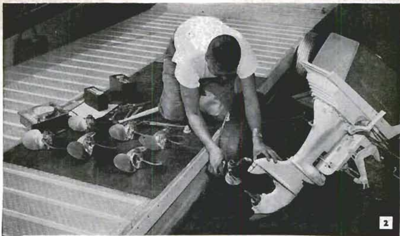
Several propellers, each having slightly different pitch, diameter or blade characteristics, are test-driven to determine the one that will give best over-all performance for given motor, hull, type of service and load
