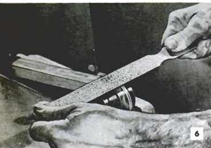
Above, tungsten-carbide grains are cutting edges of this new tool. Below, perforations in metal form cutting edges of this tool. Cuts in any direction
