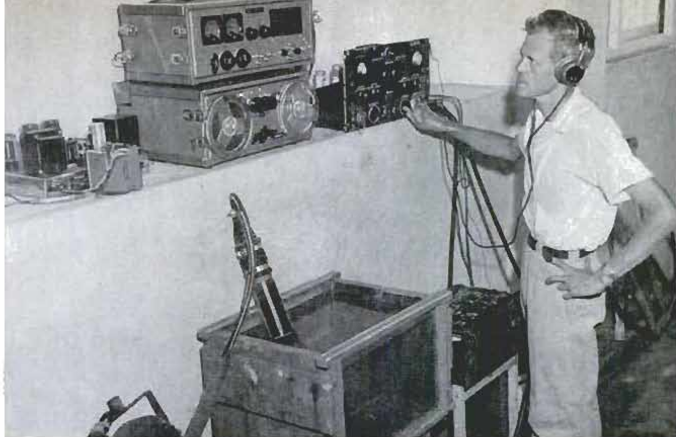
Hydrophone in aquarium detects fish chatter, which Dr. James Moulton, above, amplifies and records on tape
