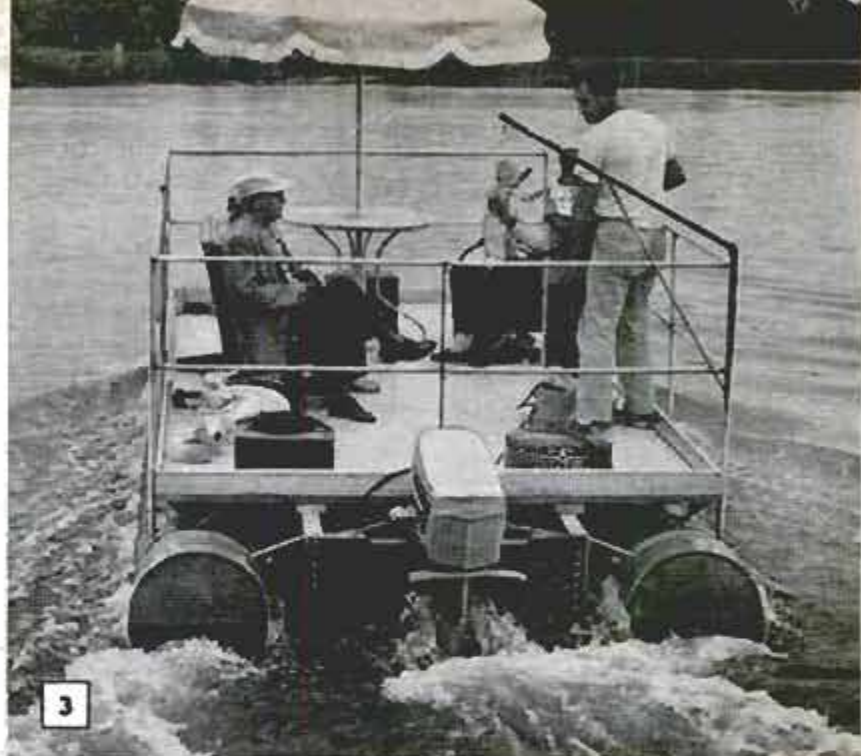
Above, typical of pontoon boats, PM boat appeals to all ages and is easily handled by means of remote controls mounted on steering station
