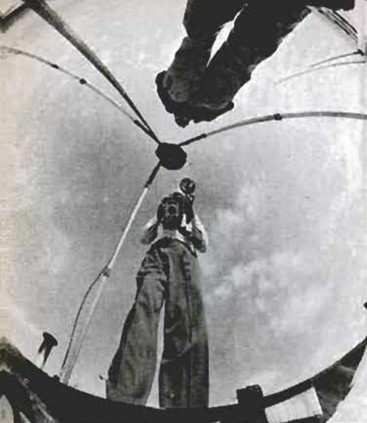
Silvered hemisphere is used as wide-angle lens for pictures of sky. Camera records cloud conditions
