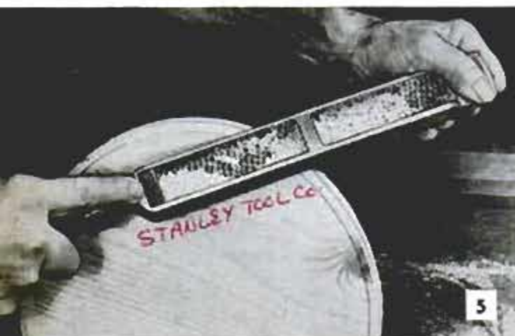
This new tool is handled like a rasp, cuts very fast and smooth in woods, plastic, nonferrous metals
