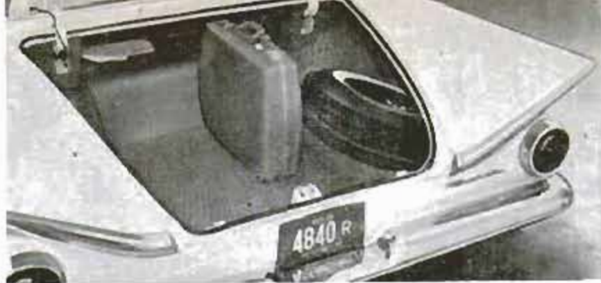
Trunk is ample, but deck slants so sharply to rear that two-suiter case must be placed in extreme forward position to allow lid to close
