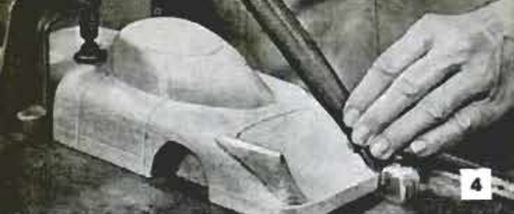
No other hand tool quite equals a rasp for finishing contoured shapes of models in wood and plastic
