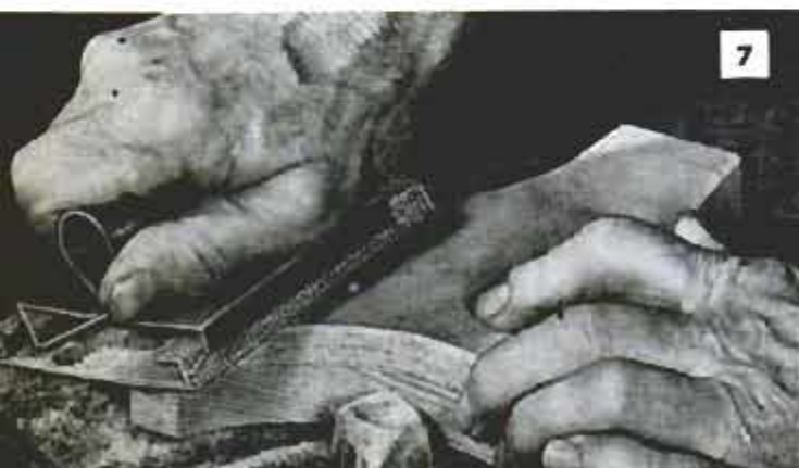
Above, tungsten-carbide grains are cutting edges of this new tool. Below, perforations in metal form cutting edges of this tool. Cuts in any direction
