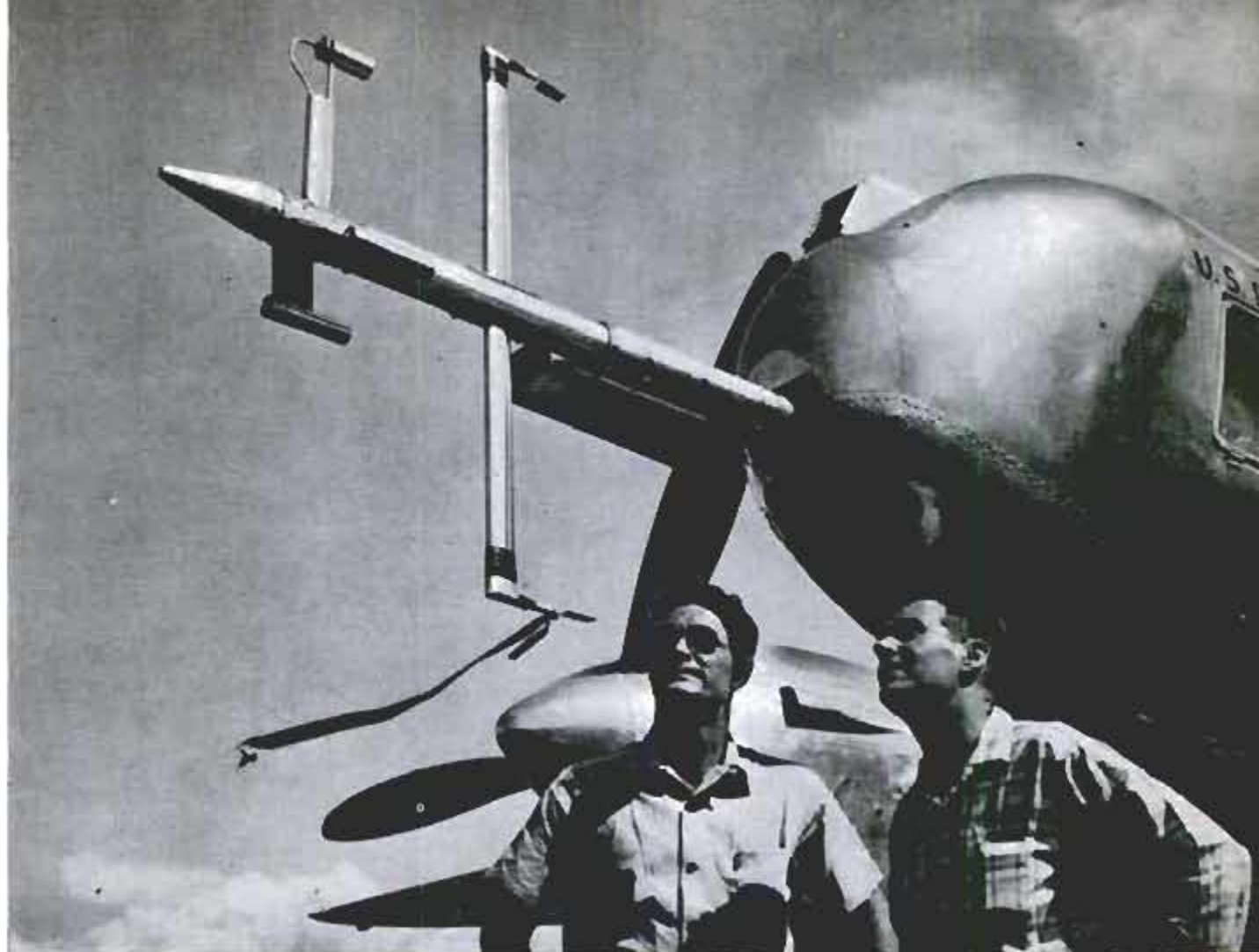
P-38 airplane, with special weather instruments mounted on probe, is used in studies of thunderstorms
