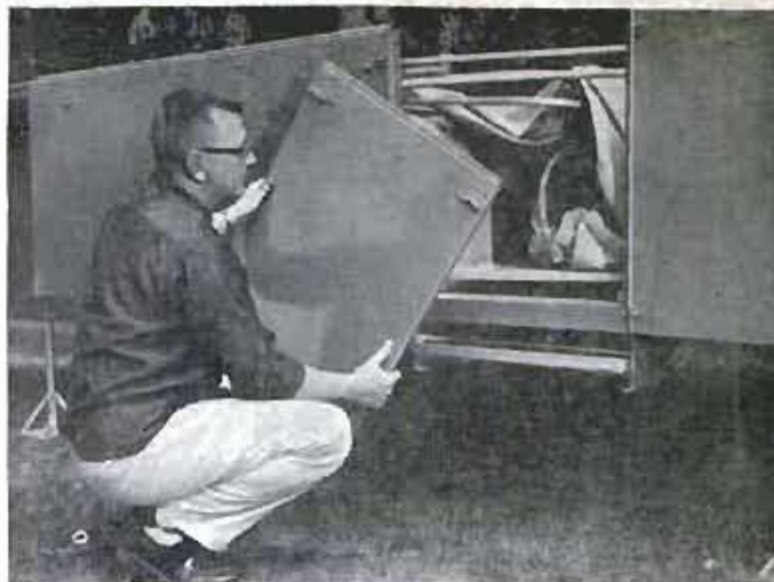
Separate removable panel closes regular door opening in side of trailer body when en route. Notice retractable commercial trailer step below opening. Step can be box and stowed inside
