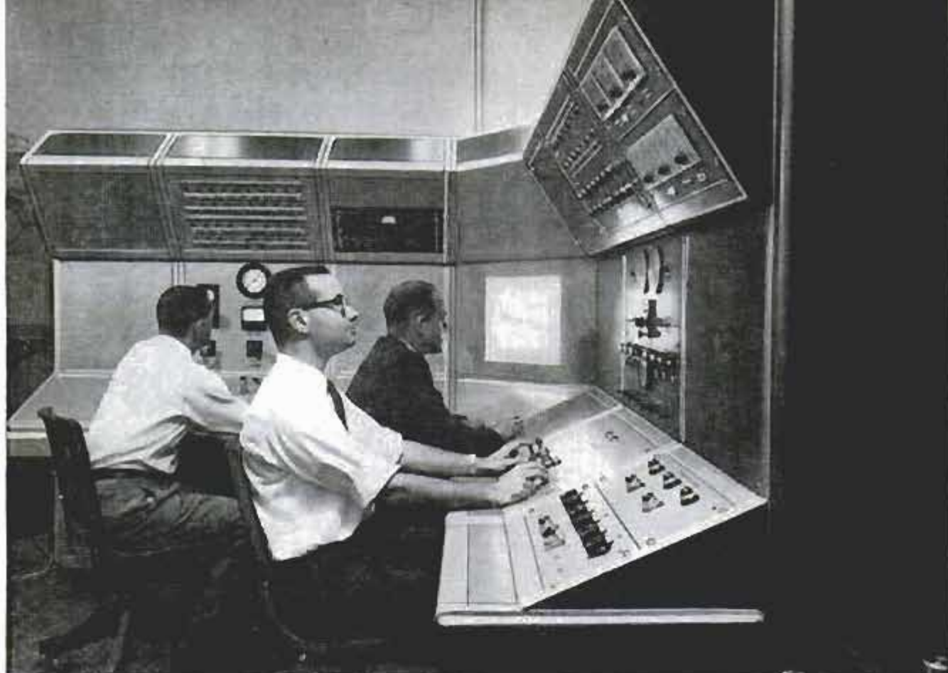
This is the control console during a test blow. The model airplane is viewed on the screen in the center
