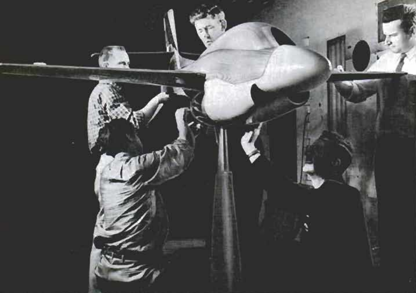
Low-speed models like this one of the T2J jet trainer are built of wood and plastic on a metal frame
