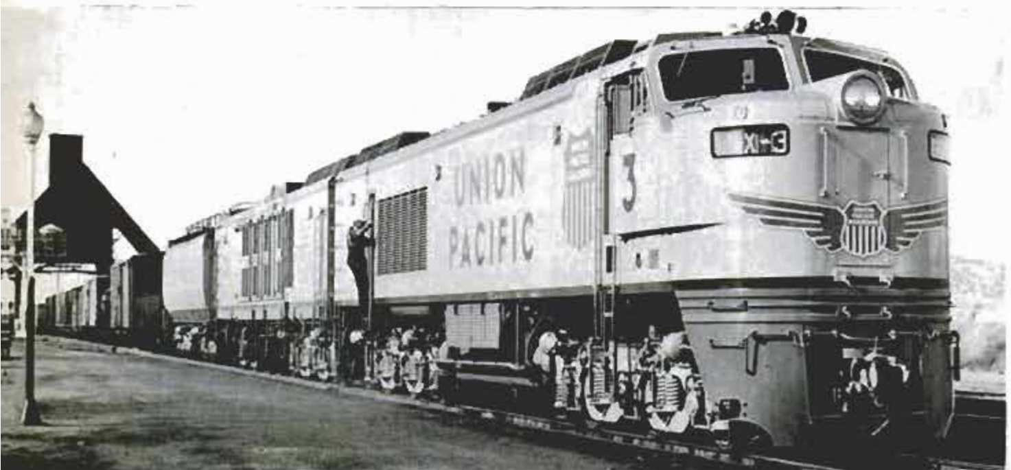
Union Pacific's first successful gas-turbine locomotive (above) has been in service several years; it has 4500 horsepower. Below, new 8500-horsepower turbine makes a stop at Evanston, Wyo., for change of crew
