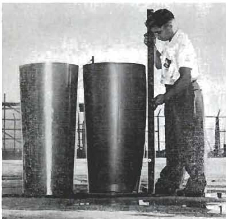
Above, cone is placed in die. Below, finished curved section of tank is shown alongside straight-walled original cone blank
