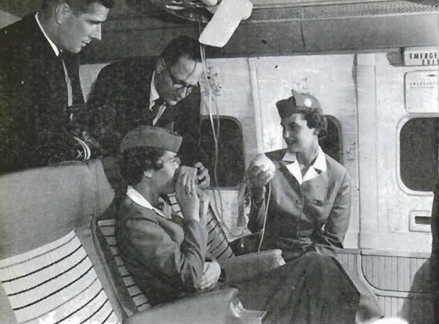
If decompression should occur, individual oxygen masks automatically drop down in front of passenger seats
