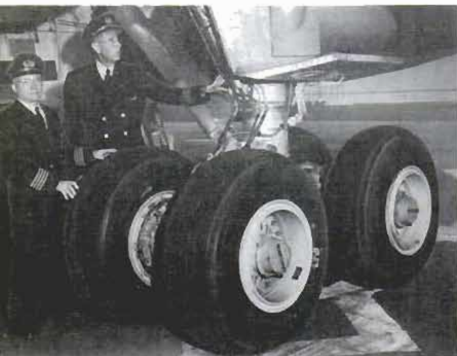
Author (right) and Captain Bittner, one of first pilots to take jet training, study four wheels on one unit of landing gear
