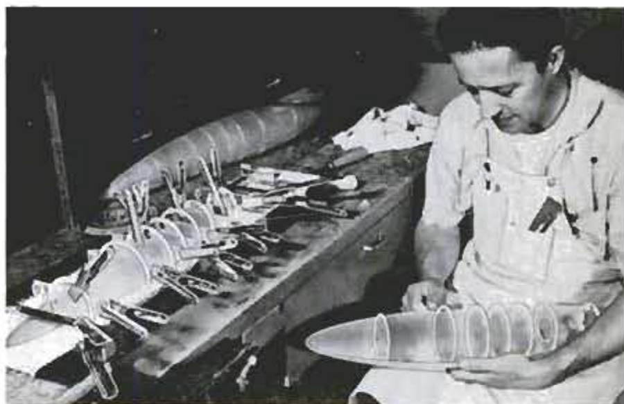
Halfway through construction, a flutter model of a fuel drop-tank has the fragile delicacy of a cocoon. On the workbench, behind a model drying in the mold, is a finished one. It is made of glass fabric stretched over thin plastic bulkheads
