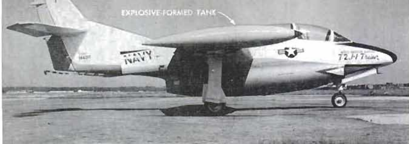
Wing-tip tank for North American's T2J jet trainer is formed by exploding charge inside of special die
