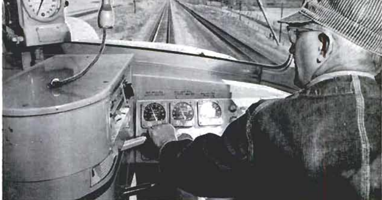
Engineer E.R.G. Pope is about to start train by moving throttle handle back. Three gauges show air pressure in reservoir and part of brake system. Dial at upper left alongside whistle cord is the speedometer
