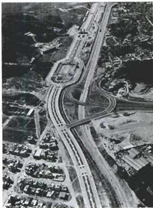
Complicated but efficient cloverleaf serves traffic entering Caracas from section of Pan-American Highway
