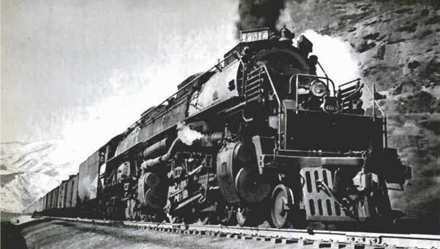
Big Boy — one of the class of most powerful steam engines ever built; it has a rating of 6000 horsepower
