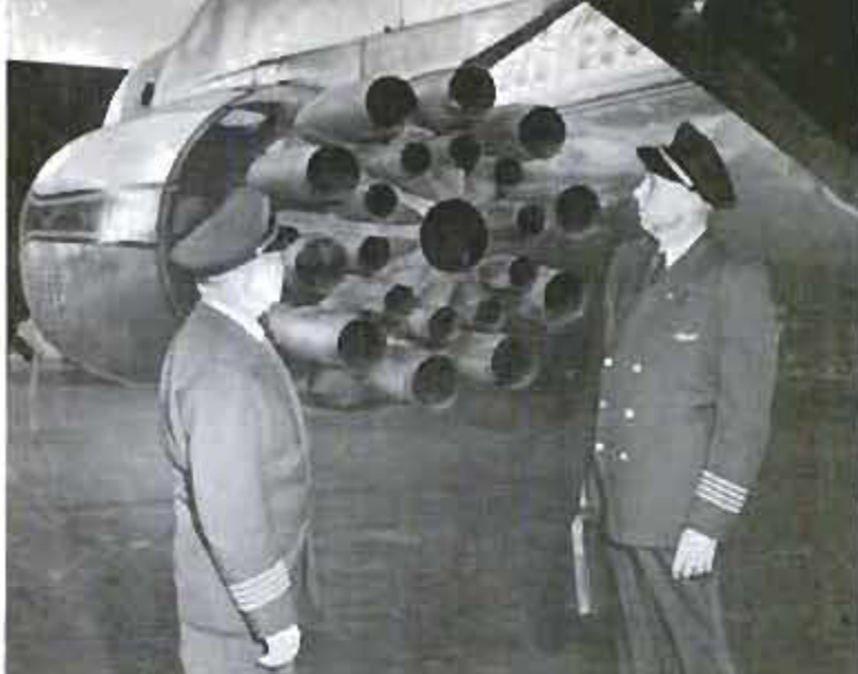
Noise suppressors on each engine materially reduce amount of noise reaching the ground during the takeoff run and climb
