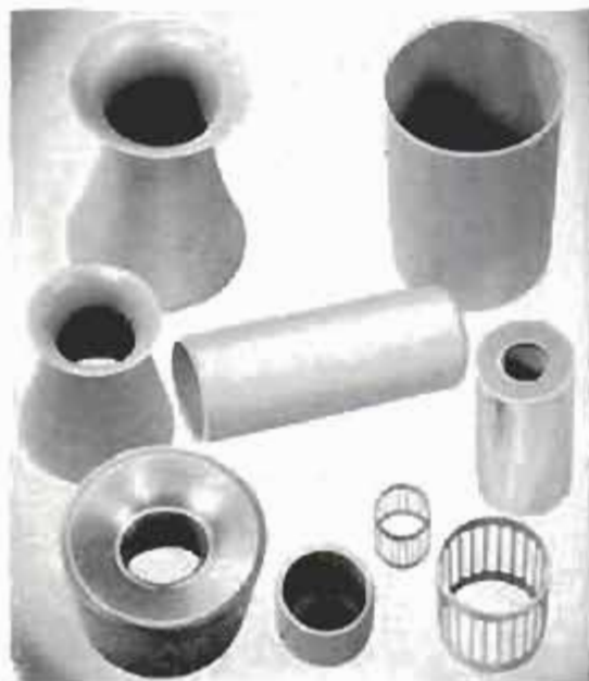
Rocket nozzles, nozzle liners, crucibles and vacuum-tube-grid cages, below left, are among products fabricated or coated with torch. Photo to the right shows stainless-steel coat being applied to aluminum plate
