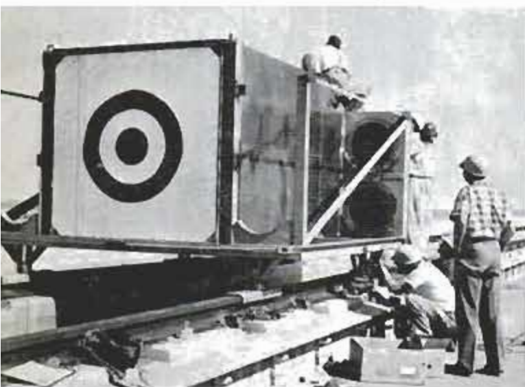
Special target sled was built for the experiment. Its rocket motors develop 200,000 pounds of thrust
