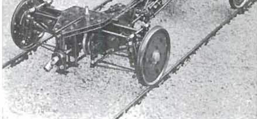
Here a vehicle's undercarriage and chassis-drive system, complete with differential, is ready for testing before elaborate scale model is made
