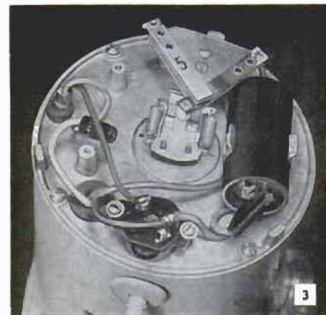
Below, centrifugal governor is spring-loaded device at center, internal switch is V-shaped object above it. Cylinder is capacitor, overload switch is below
