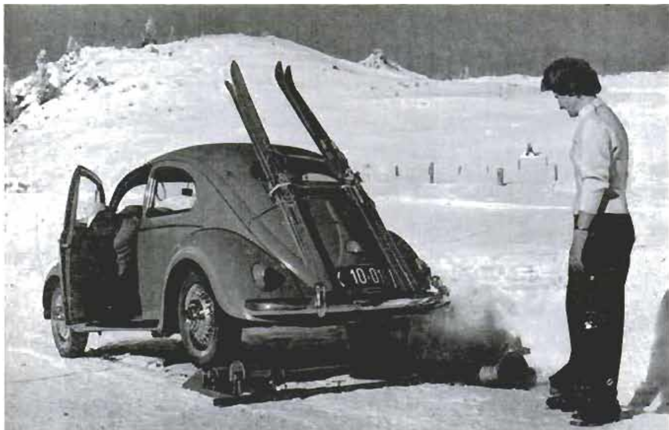
The rear wheels of the ski-lift-driving automobile rest on cylinders placed at each end of the rotating shaft
