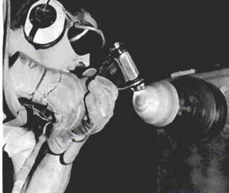
Nose cone for a missile, above, is given a heat-resistant tungsten coating with Plasma Arc Torch which harnesses highest temperatures used in industry, up to 30,000 degrees Fahrenheit. Diagram below shows how torch applies surfacing material
