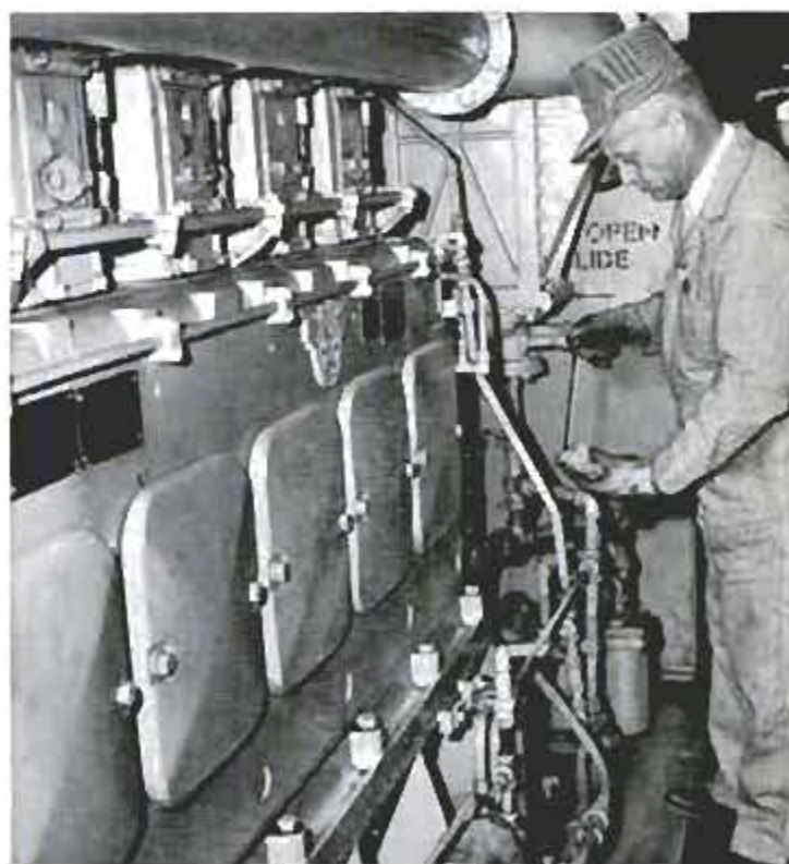
Alberts checks level of oil in diesel auxiliary; engine keeps up pressure for the brakes
