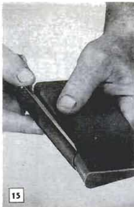
It's permissible to sharpen outside gouge on side of wheel as in Fig. 14. Figs. 15, 16 picture two methods of finishing inside gouge. In the first, Fig. 15, gouge is moved, stone is stationary. In Fig. 16, stone is moved
