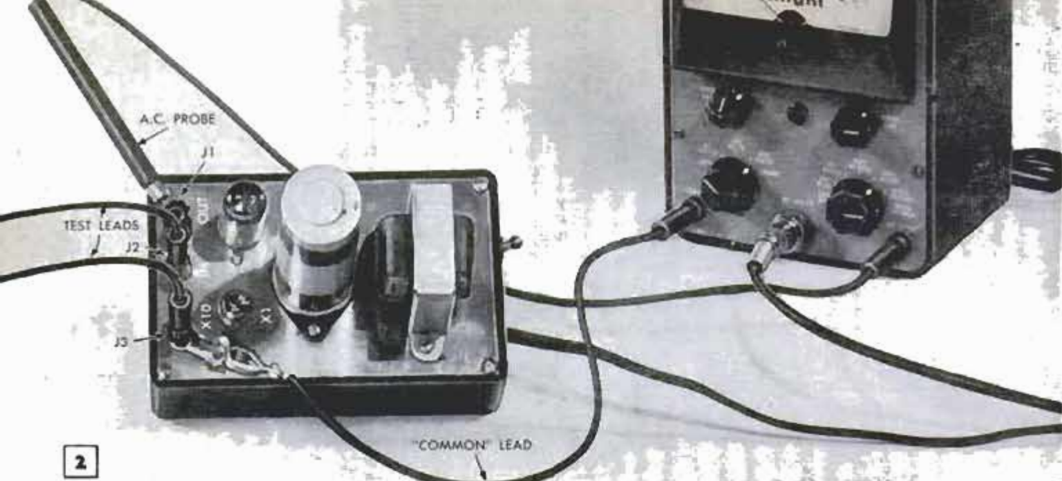
Preamplifier is connected between signal source and VTVOM. Signal is measured with separate test leads
