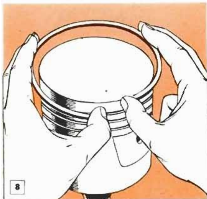
8 Above, twisting ring as shown, when installing it on the piston, will completely destroy its effectiveness
