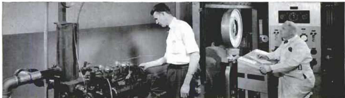
• Dynamometer tests determine the effect of carburation on maximum power output of a GM car engine. Carburetor design is matched to the specific requirements of each GM engine.
