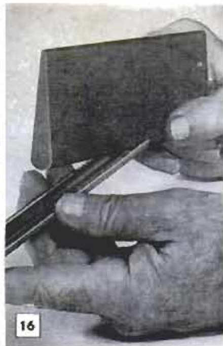
It's permissible to sharpen outside gouge on side of wheel as in Fig. 14. Figs. 15, 16 picture two methods of finishing inside gouge. In the first, Fig. 15, gouge is moved, stone is stationary. In Fig. 16, stone is moved
