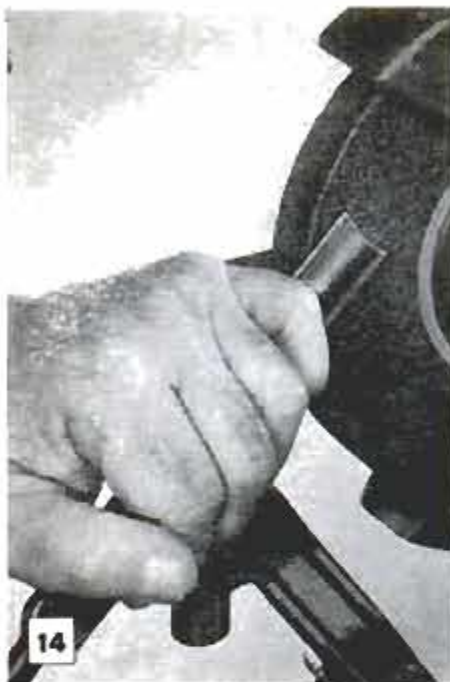
It's permissible to sharpen outside gouge on side of wheel as in Fig. 14. Figs. 15, 16 picture two methods of finishing inside gouge. In the first, Fig. 15, gouge is moved, stone is stationary. In Fig. 16, stone is moved
