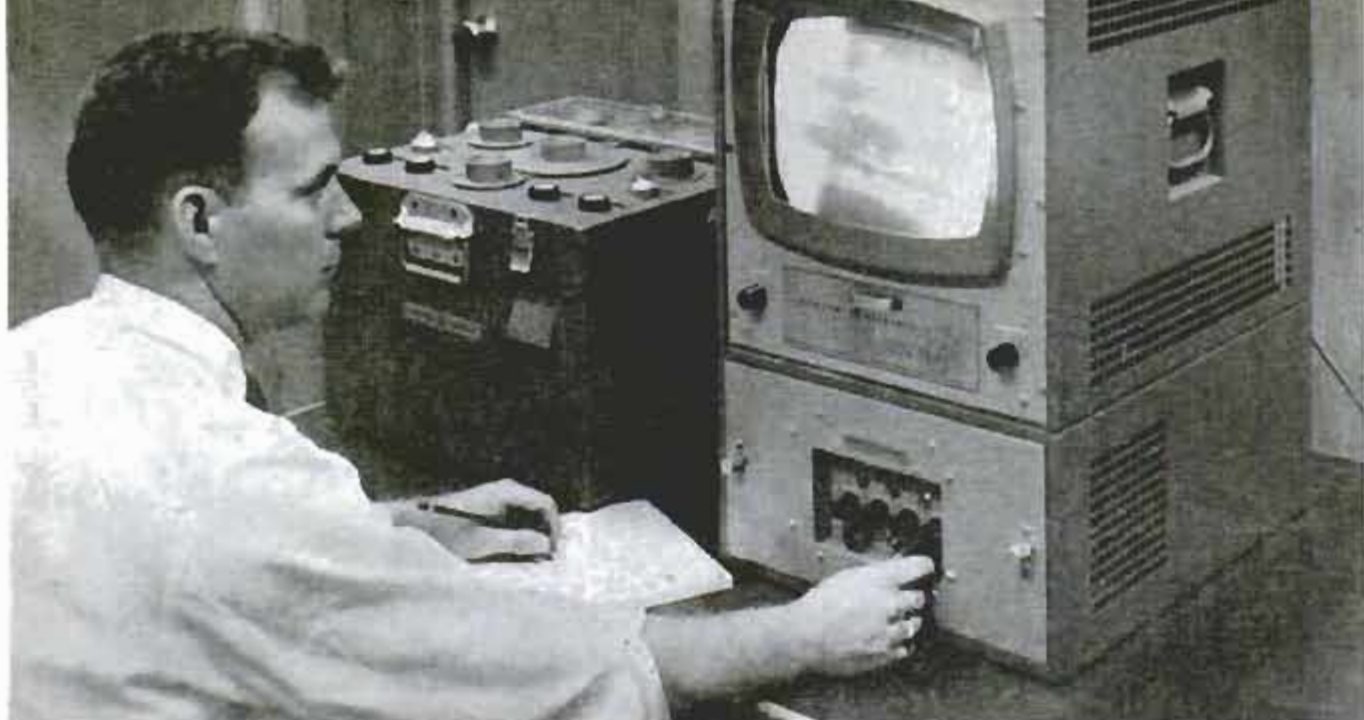
Operator, seated at a remote television monitor, watches X-ray images of parts passing down assembly line
