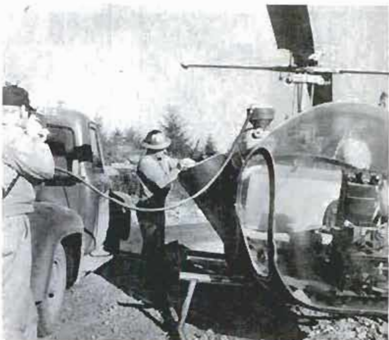
Seed tanks are behind helicopter's "eye." Below, slinger throws seed in 90-foot swath at the rate of one acre in 15 seconds
