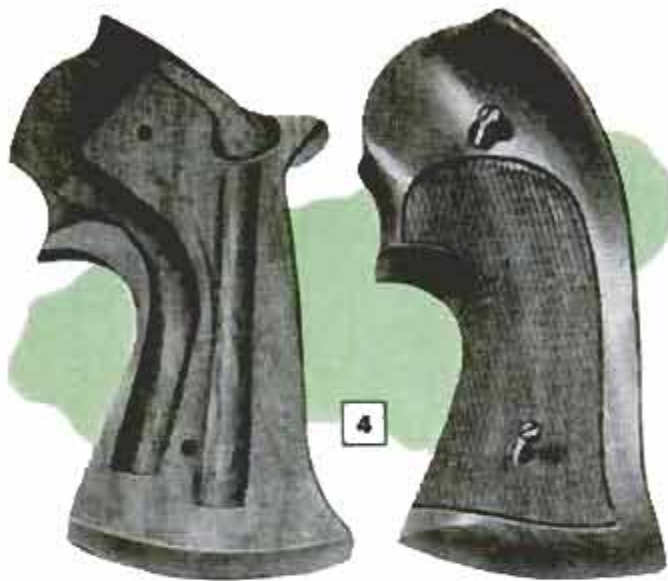
Above, left and right halves of stock are carefully grooved to provide tight fit when bolted together on tang of gun. Right, heavy gun requires custom-made holster of stiff leather bound with heavy thongs
