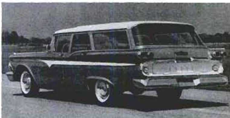
Villager wagon comes as two or three-seat model. Weight distribution on wagons is 50-50, giving good traction on ice or snow
