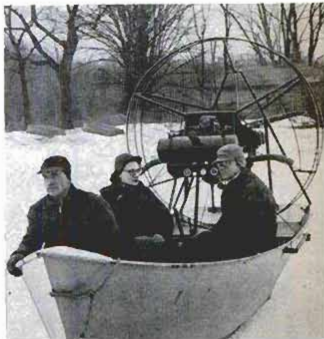
Another type of sled boat powered by airplane engine has runners under metal hull
