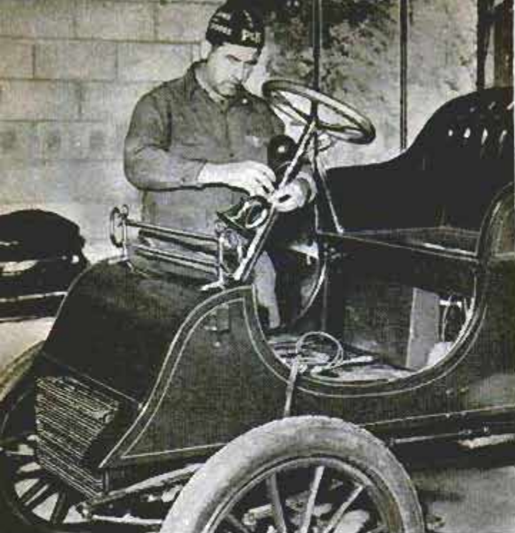
One of Davis' assistants, Roger Gallidan, attaches horn to steering column of a 1903 Model A Ford
