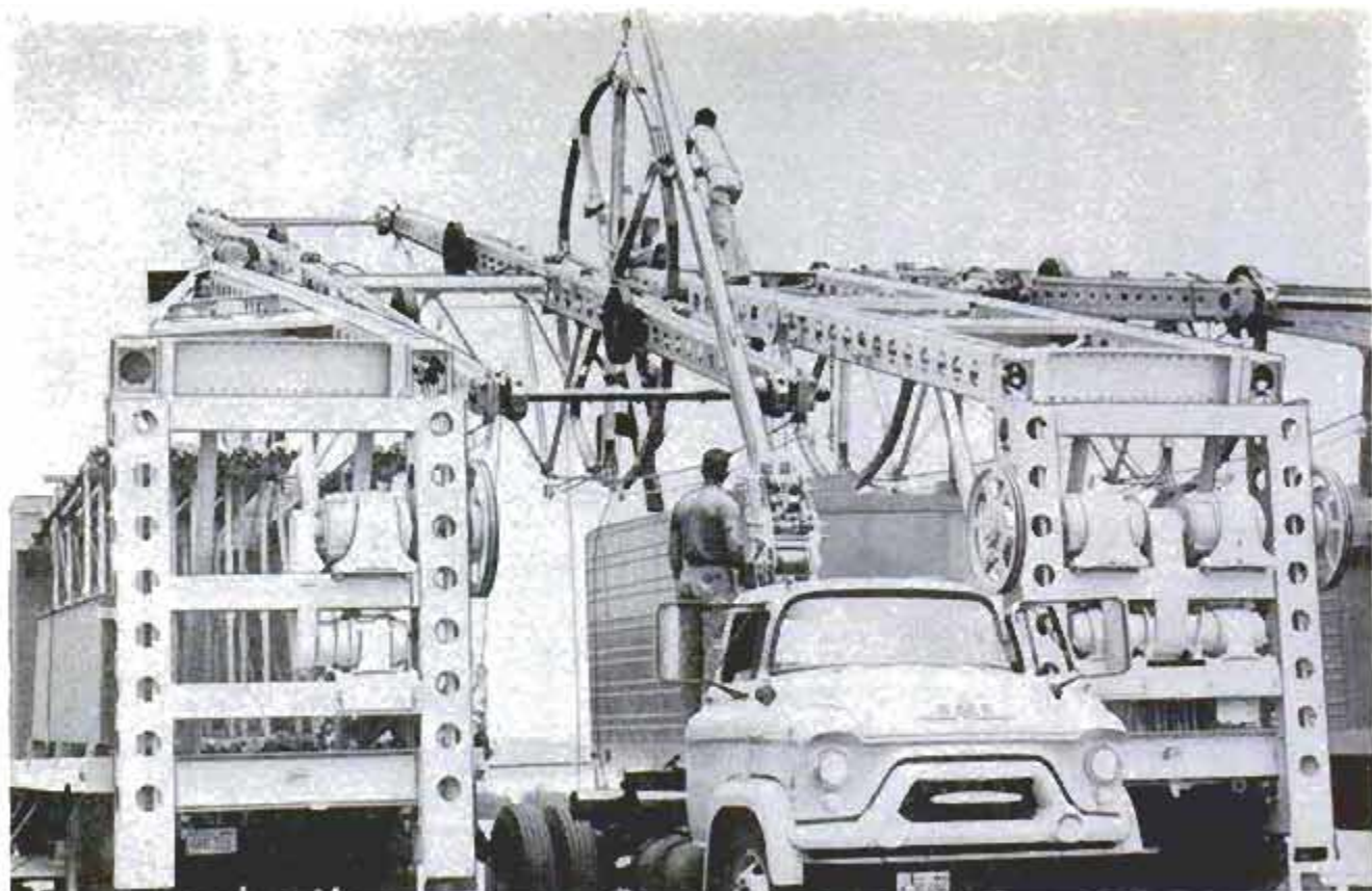
Partially unloaded, the big wheel starts to go up. A minimum of 70 kilowatts is needed to operate unit
