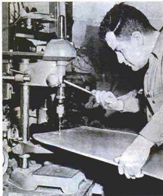
Holes are drilled in flat aluminum sheet that will become new rear fender for 1906 model Pope-Toledo
