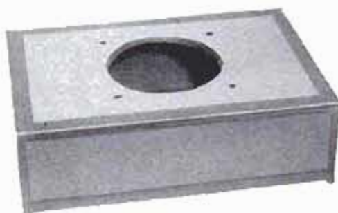
Cigar box forms theater base. Previously prepared speaker is mounted from below with screws and nuts
