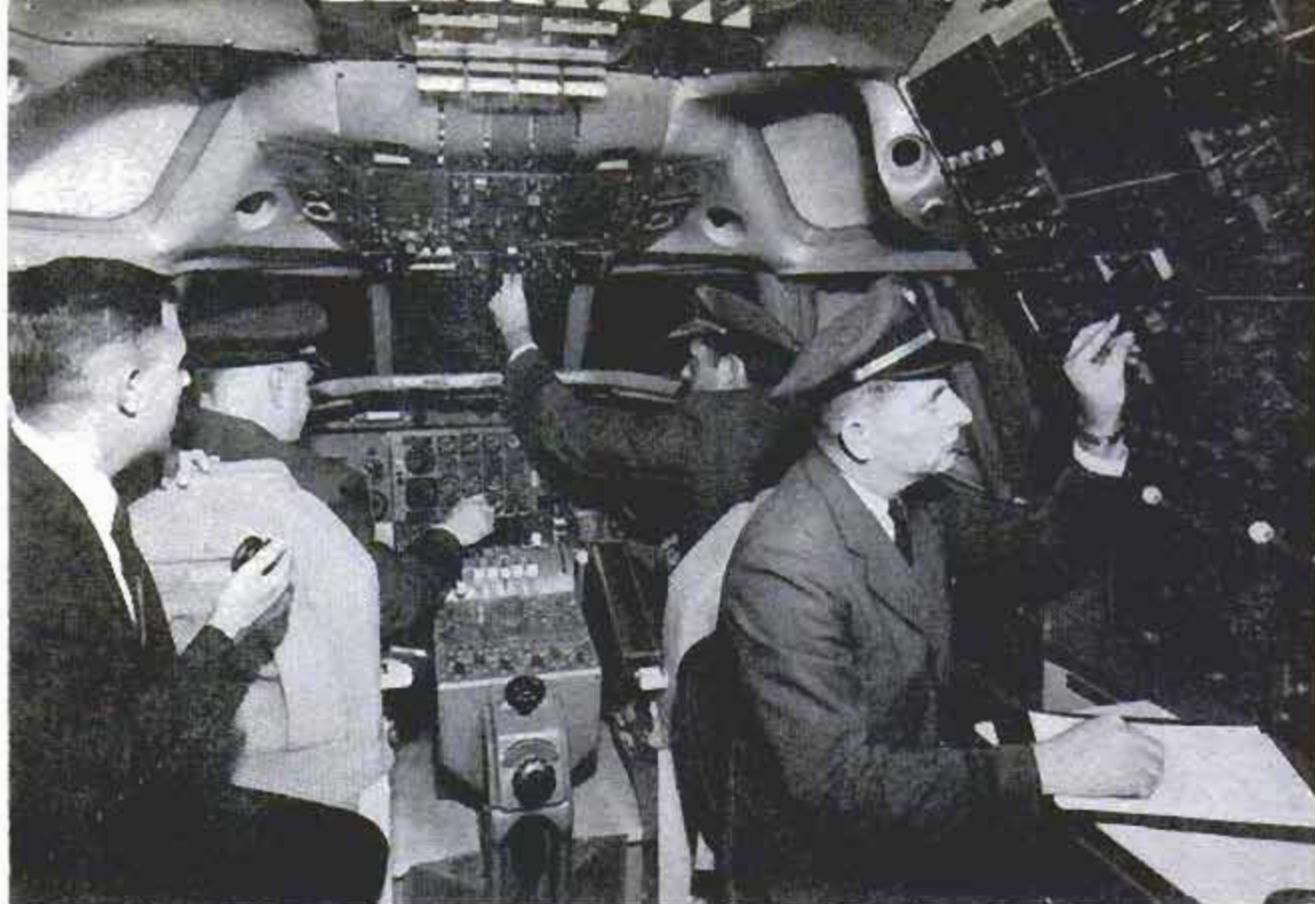
Simulator is a detailed replica of the DC-8 jetliner cockpit, with identical instruments and flight controls
