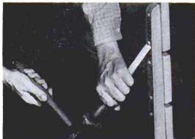
Above, screws through underside cleats hold front and back members. Below, screws holding backboards to legs are capped with plugs, trimmed flush
