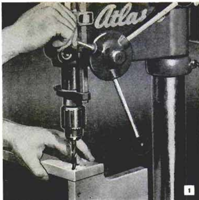
Primary purpose of a drill press is drilling holes of various diameters in wood and metal but it is adaptable to other jobs
