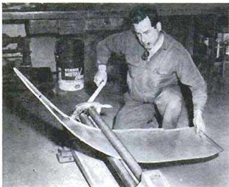
Flat aluminum sheet, above, is being curved into a rear fender. Below, the crankshaft is being removed from 1906 Locomobile
