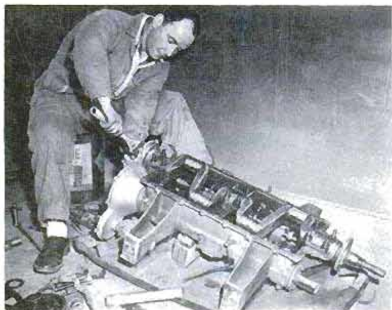
Flat aluminum sheet, above, is being curved into a rear fender. Below, the crankshaft is being removed from 1906 Locomobile
