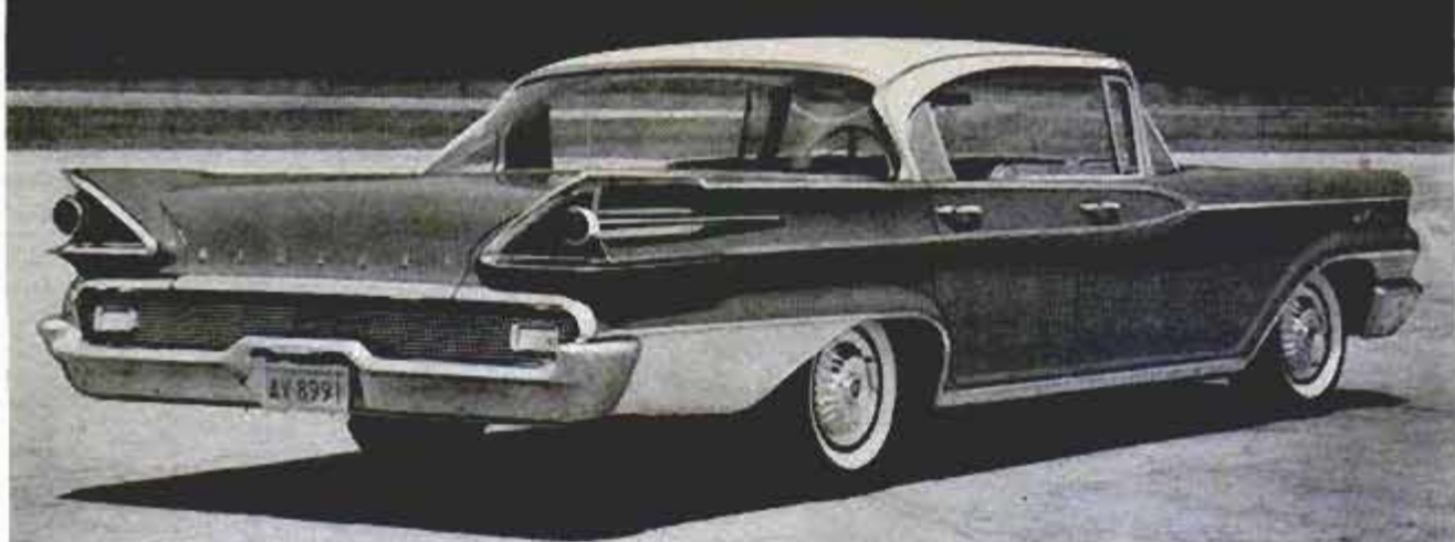
Park Lane models, like this four-door hardtop, have a distinctive "torch" mounted in rear-fender cavity
