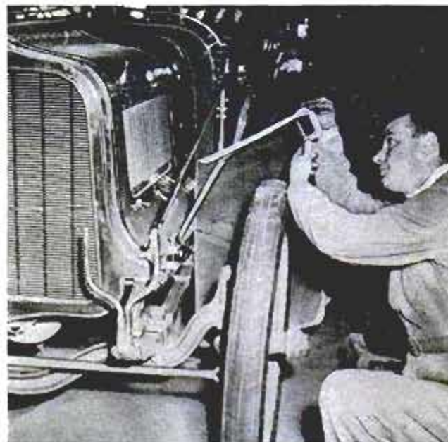
New aluminum fender is clamped into position on antique car. Some fenders are shaped from sheet steel
