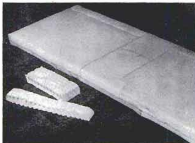
Above, after frame is sprung with No-Sag springs, springs are covered with denim. Below, foam-rubber scraps, cemented together, form built-up cushion pads
