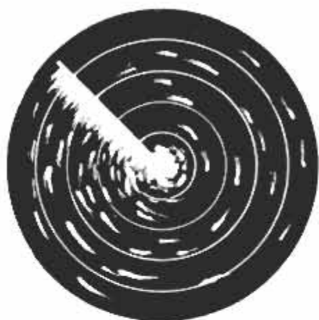
Terminal radar now in use shows only direction and distance of planes by blips on the black viewing screen
