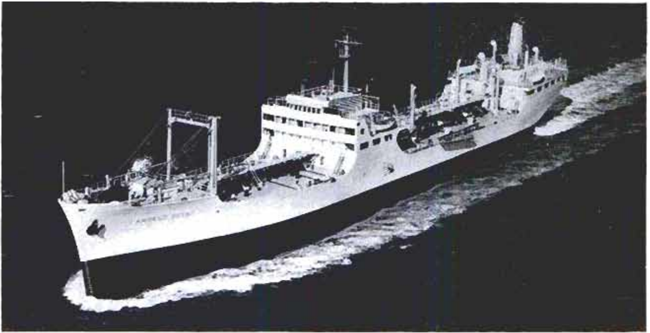
This 530-foot wine tanker, Angelo Petri , is the first ship of its kind under U. S. flag. It has 26 vats
