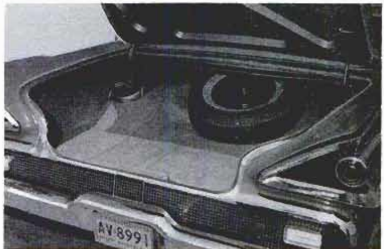
Spare mounts forward to increase handy-to-get-at trunk area. After all, when did you last need a spare? Below, frame cross-member over rear axle is curved heavy-gauge sheet metal instead of box girder. It is lighter, stronger, requires less height
