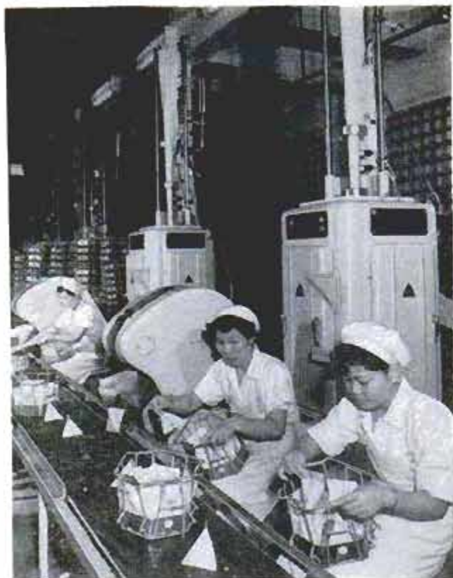
Machines that make milk containers from rolls of coated paper are behind workers in Japanese dairy
