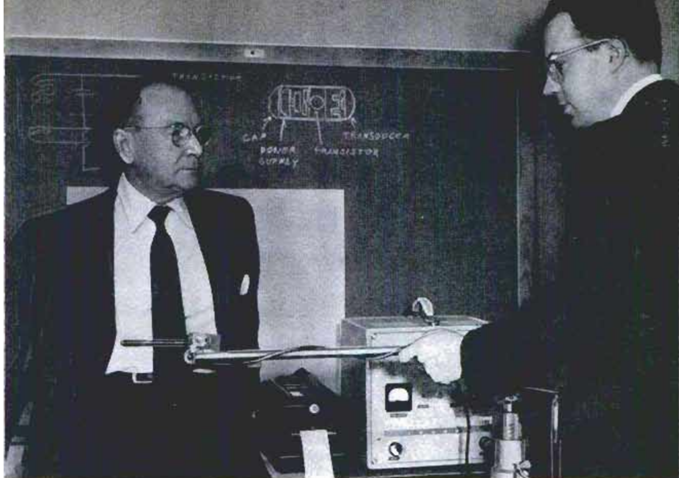
Scientists show how medical information broadcast by "radio pill" inside patient is picked up with antenna
