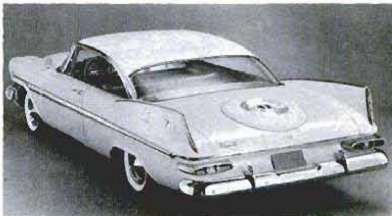
Available at extra cost is a dummy spare-tire cover that is embossed on the trunk lid. The canted tailfins are new also
