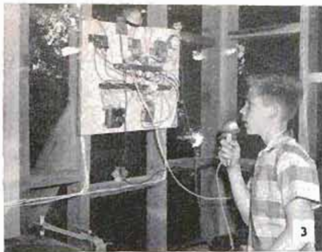
Santa speaks through hidden microphone and speaker. Peephole in nearby garage lets operator observe passersby to extend friendly personal greeting
