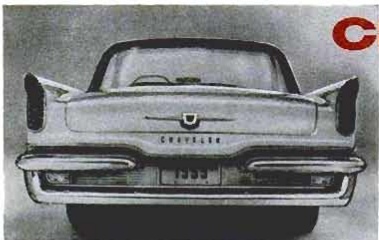
Completely fresh is the rear-end styling. Bumper is more massive this year and has a recessed anodized-aluminum insert
