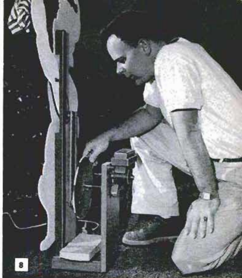
Back view of Mrs. Santa Claus shows how drive rod attached to motor-driven eccentric provides a gently waving movement to arm holding handkerchief
