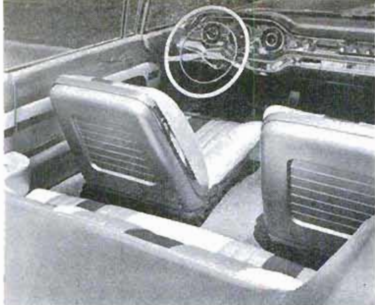
Bonneville convertible has bucket seats in front, stylishly contoured. Wide dash shroud eliminates windshield reflections
