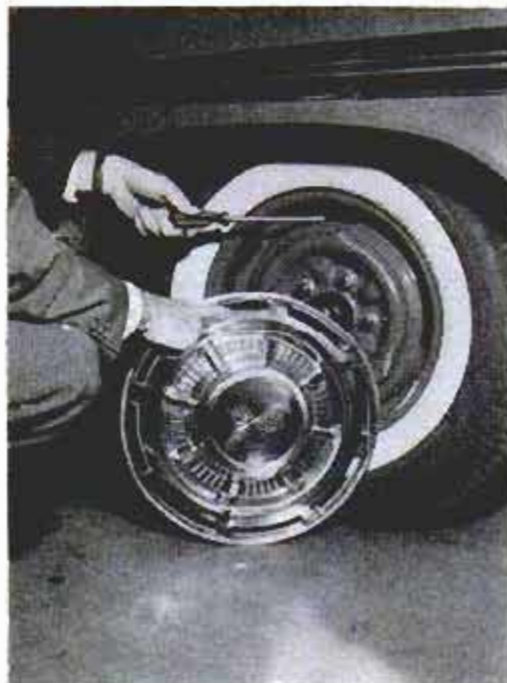
Slots in the wheels and extra-cost wheel covers create a flow of air to cool brakes
