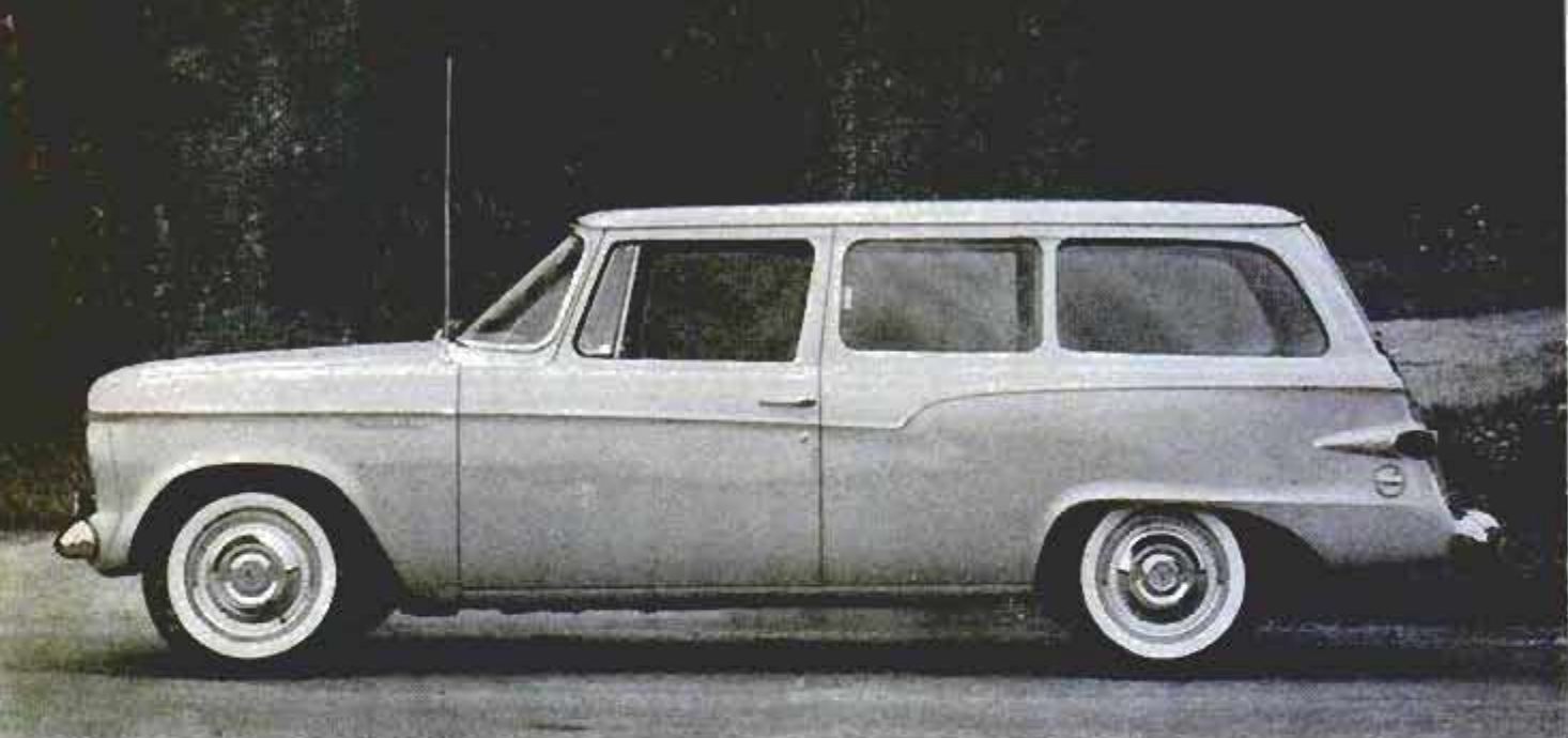
Station wagon has 113-inch wheelbase, 184.5-inch over-all length. Other models share 108.5-inch wheelbase
