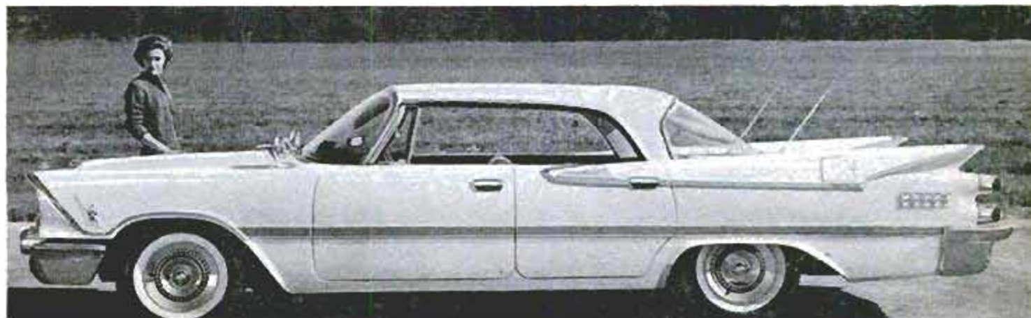
Four-door hardtops have a new stepped roof which is slightly higher in the rear for more interior room
