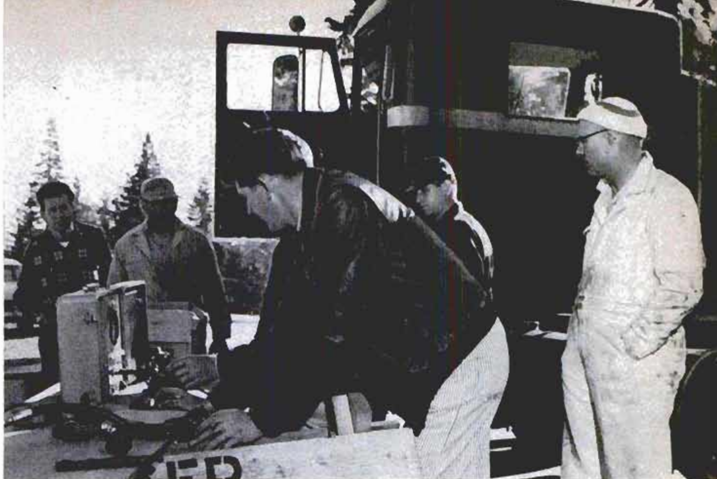
Inspectors use special apparatus to check transmission time for the air to reach farthest brakes on big truck
