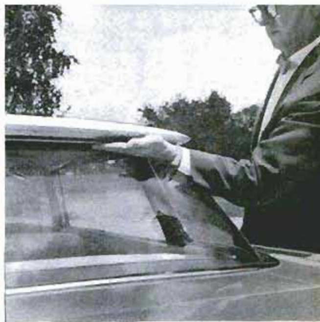
Roof of four-door hardtop extends beyond the tremendous wrap-around rear glass
