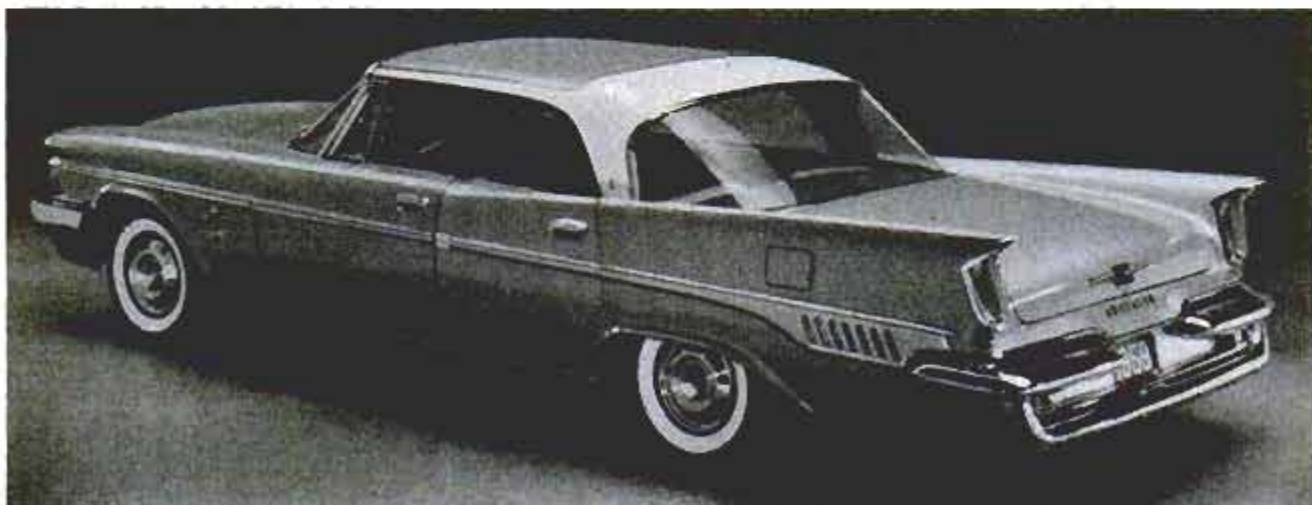
Above, top is smaller than bottom half of wheel, allowing it to be positioned higher for more legroom without blocking vision. Below, rear of hardtop roof is stepped up for added room
