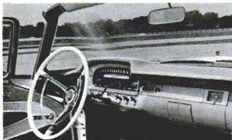
Ford continues its neat, uncluttered dash, but has replaced the curved shroud with a straight one like the rest of the industry
