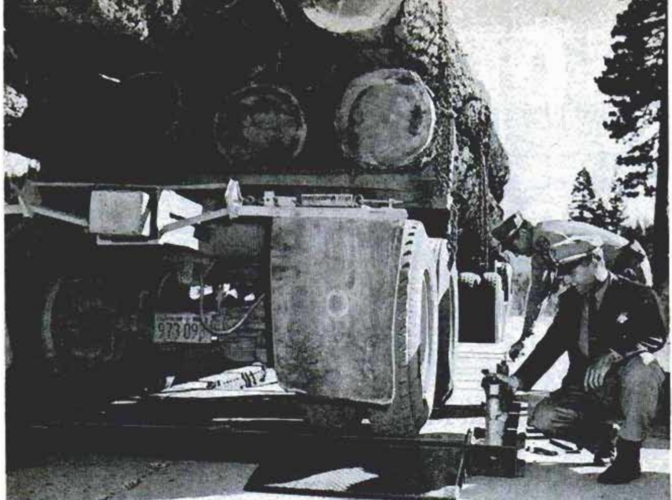
Highway patrol officers check weight of load on each axle of huge log carrier during "round up" at Dunsmuir
