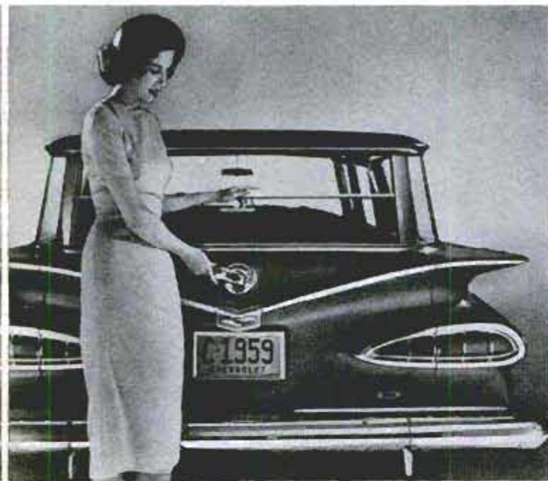
Station wagons have no upper tailgate. Glass winds down into lower half of door manually or electrically (option)
