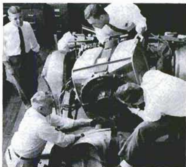
Big gas-turbine engine mounts in the rear. Actually, this is simply the wooden mockup being tried for size
