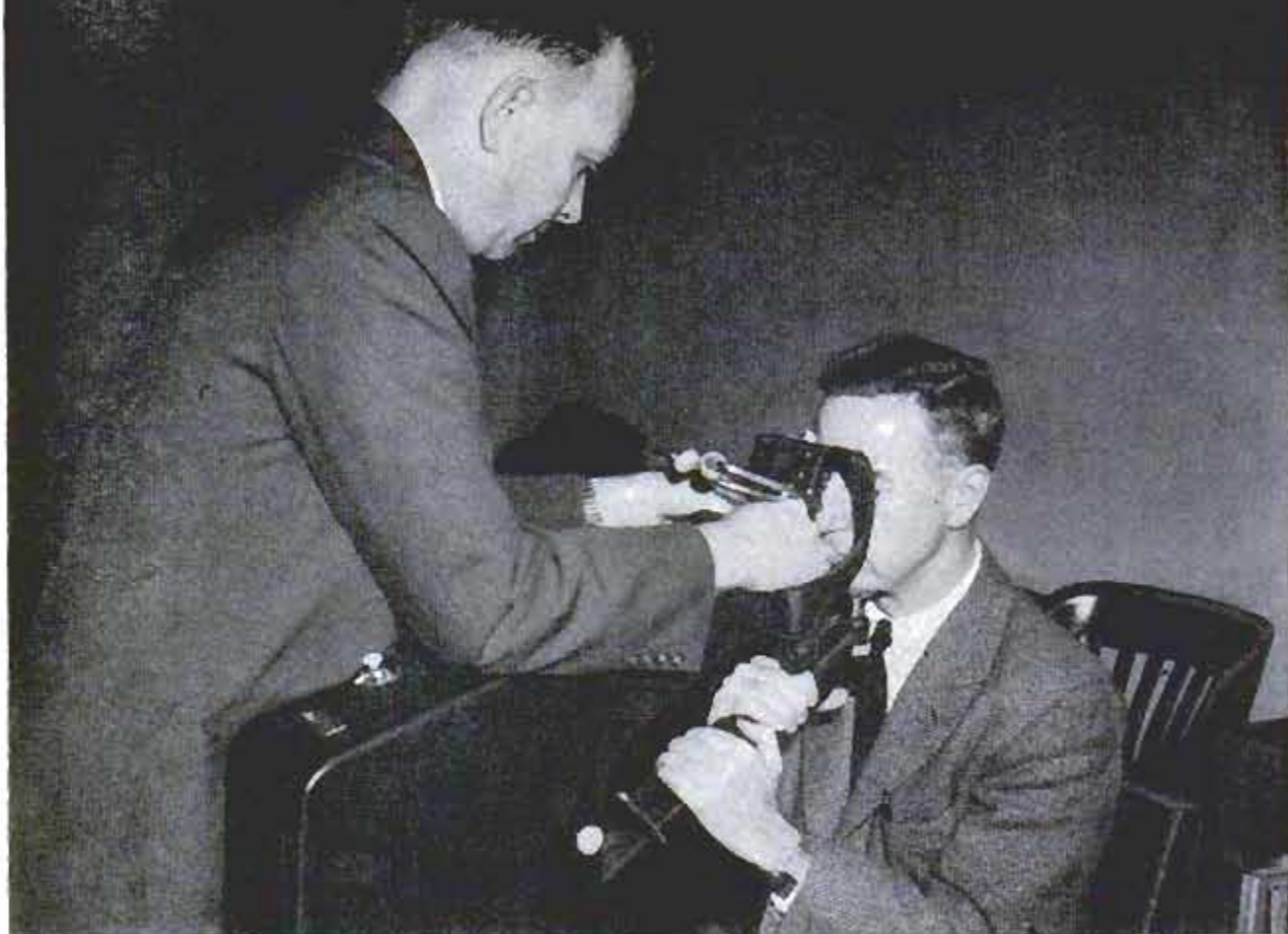
Pattern of pauses and backtracks on film, at right, is traced by the light reflected from reader's eyes as he looks into the ophthalmograph, above
