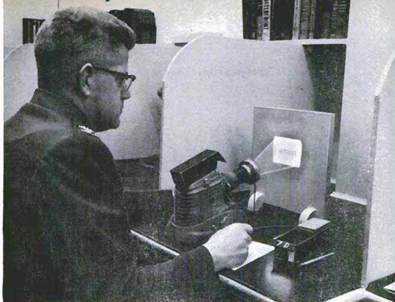
Tachistoscope flashes row of numbers for fraction of a second, then observer writes down digits he saw
