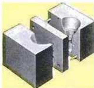
1-DIE WITH MATCH PLATE BETWEEN HALVES
