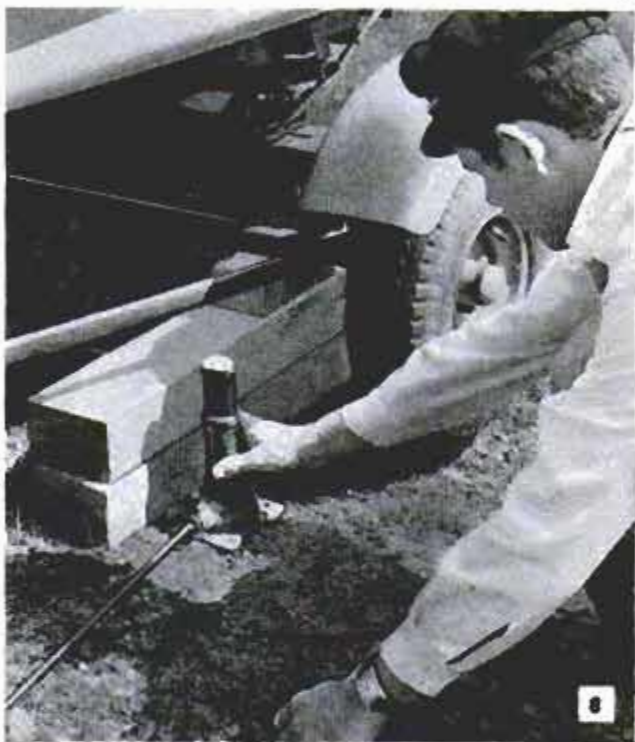
When boat is stored on trailer, it's a good idea to block up axles and tongue to take weight off tires
