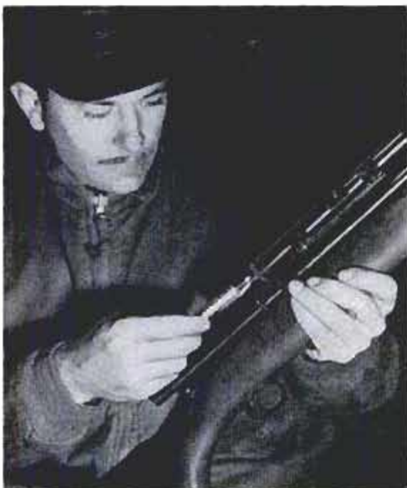
Drug darts are fired from air gun which has steel tubing barrel to fit darts
