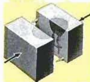
3-MERCURY FROZEN AND MATCH PLATE REMOVED
