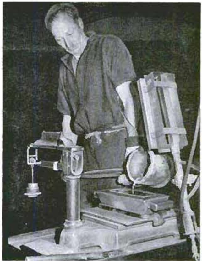
Gold concentrate is cast into rough bars for trip to the refinery, where impurities will be removed
