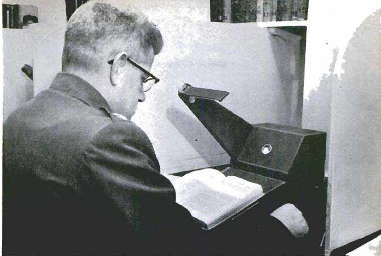
Reading pacer projects a band of light which moves from top to bottom of the page the officer is reading
