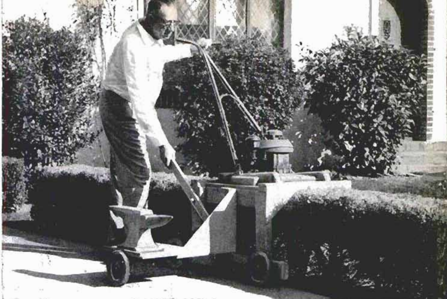
Trimming a 375-foot hedge by hand required six hours, but rotary-mower rig does the job in five minutes
