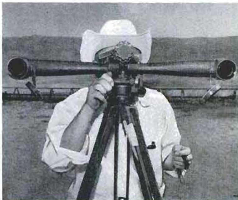
Tracking-team member sights falling rocket and records bearing. Location of the buried rocket can be found by triangulation
