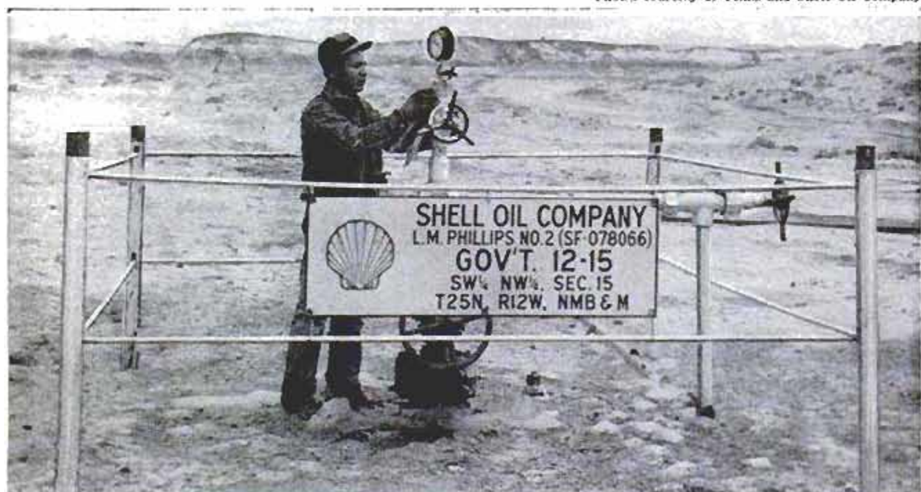
Once well begins to flow, drilling rig is dismantled and moved. A small fence is erected around wellhead Photos courtesy of Texas and Shell Oil Company
