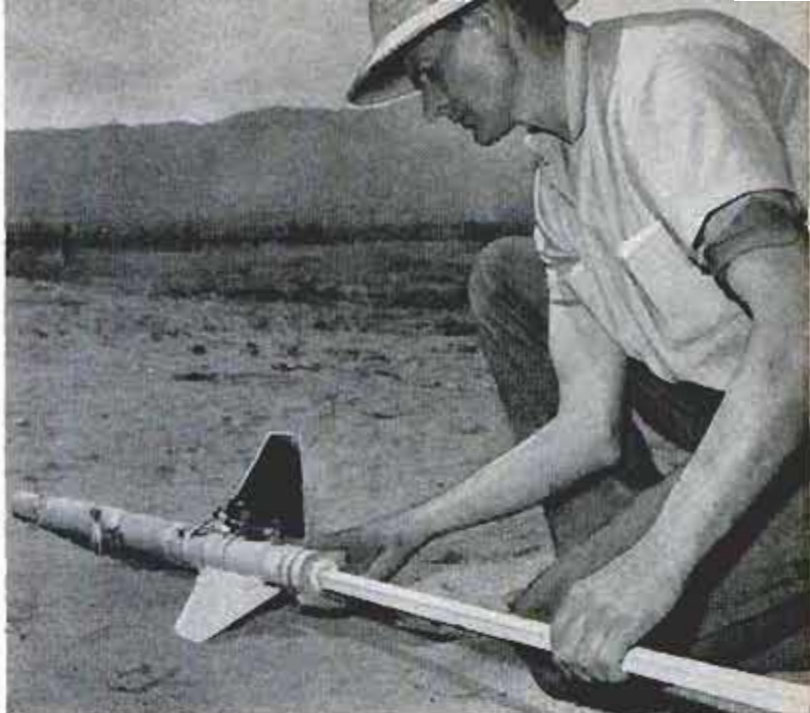
Full safety precautions are observed during the critical period when the solid fuel is tamped into place
