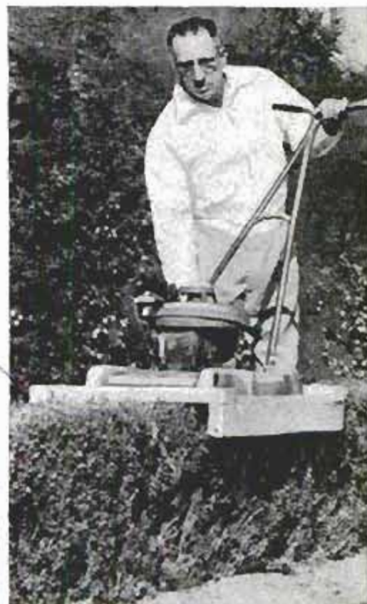
Trimming a 375-foot hedge by hand required six hours, but rotary-mower rig does the job in five minutes
