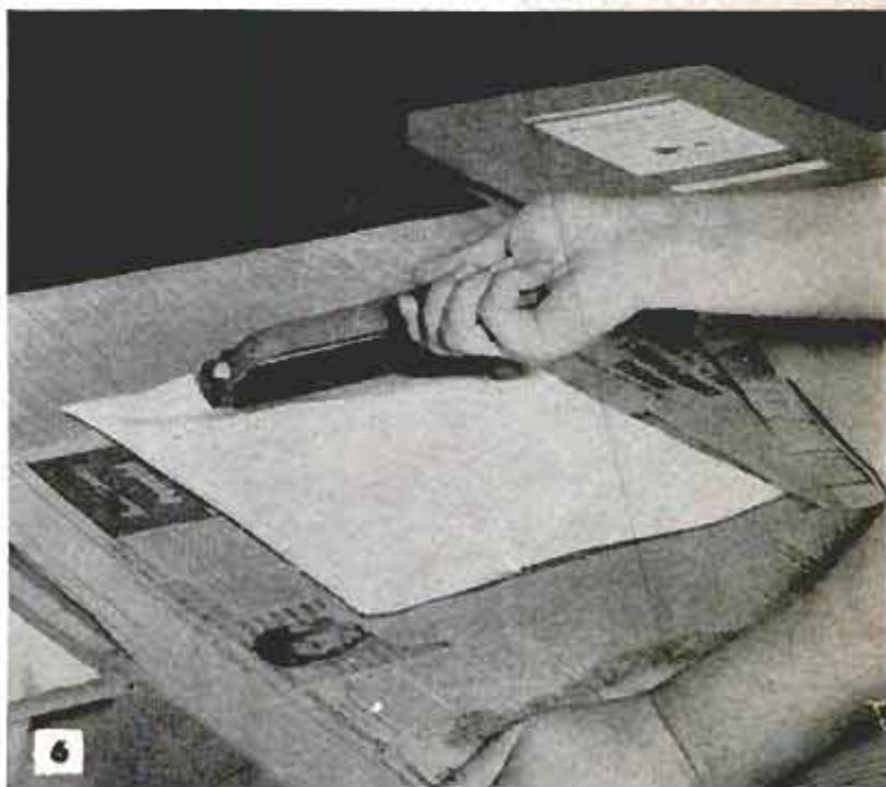
Above, pressure is applied to print-exposure box to keep all areas of slightly curved surface of book page in contact with it. Fig. 6. Pad of newspapers absorbs water rolled from negative-positive "sandwich"
