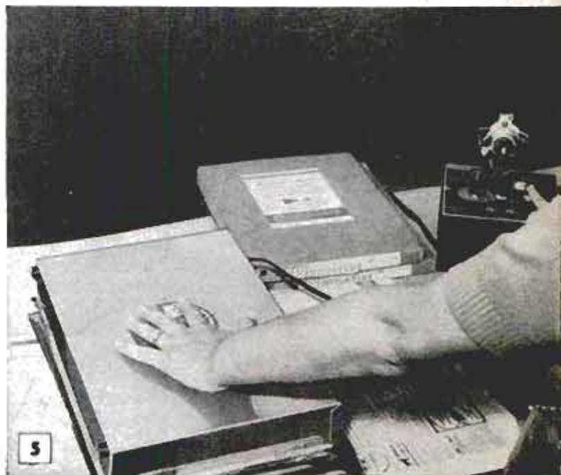
Above, pressure is applied to print-exposure box to keep all areas of slightly curved surface of book page in contact with it. Fig. 6. Pad of newspapers absorbs water rolled from negative-positive "sandwich"
