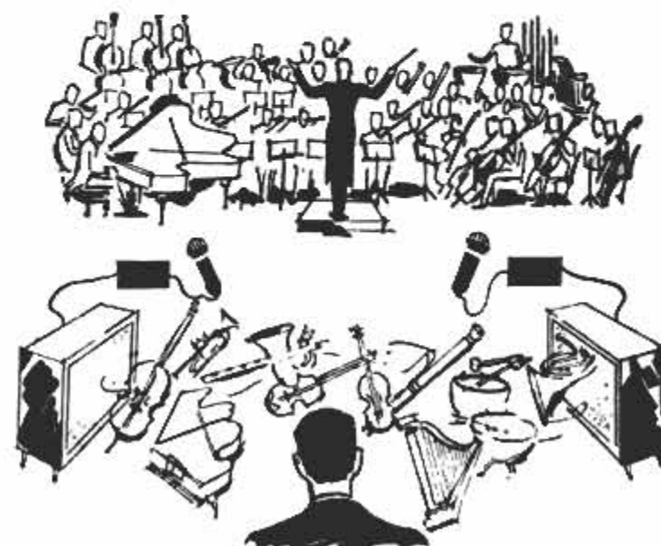
Fig. 2, above. When two microphone signals are mixed in one amplifier and reproduced by two speakers, the resultant sound is still a point source but seems to come from a position midway between the speakers. Fig. 3, below. True stereo reproduction requires two separate, independent sound channels
