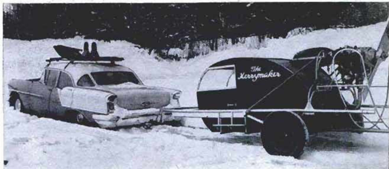
Above, with runners on auto-top carrier and wheels on the hubs of the Merrymaker, the snowmobile is trailered to new location. Below are shown details
