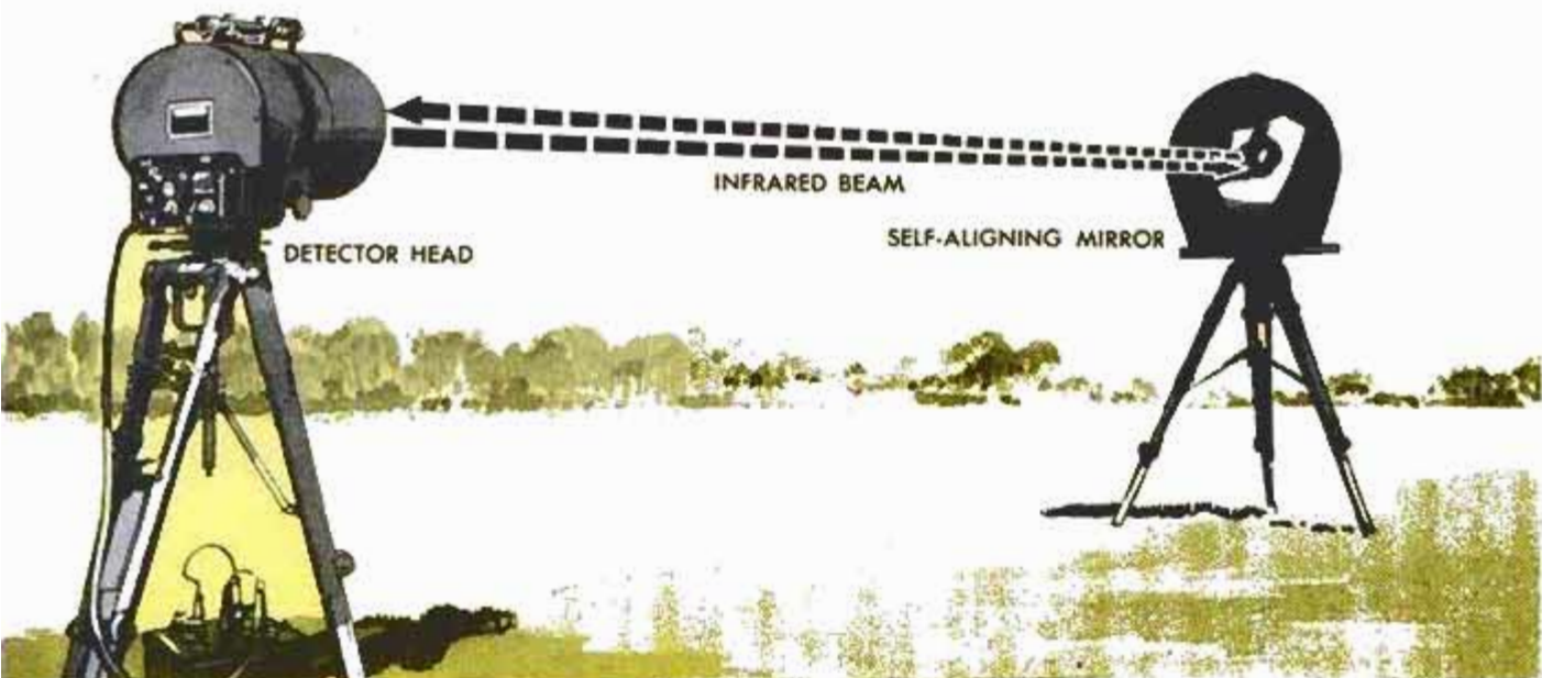
Detector transmits infrared beam, analyzes reflected beam, trips alarm if certain chemicals are detected
