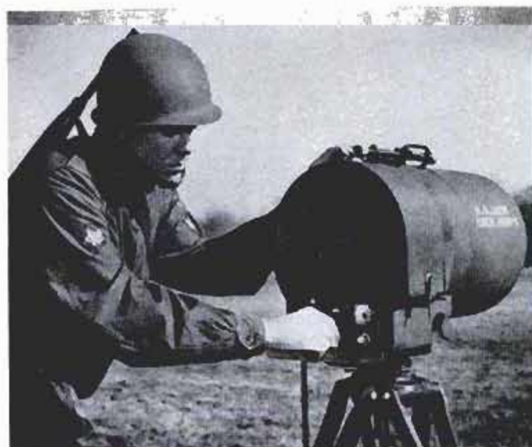
Detector transmits infrared beam, analyzes reflected beam, trips alarm if certain chemicals are detected
