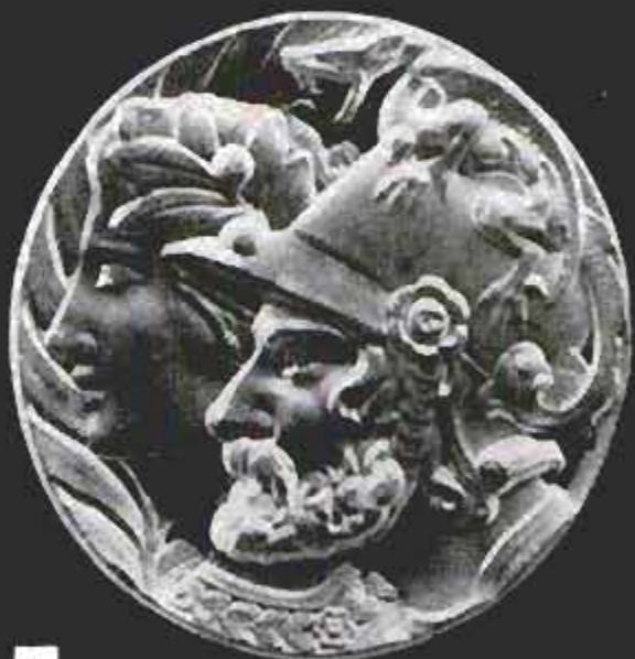
Relief work cut into glass with ultrasonic impact grinder. Note accuracy of extremely intricate detail
