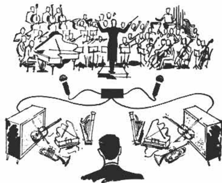
Fig. 2, above. When two microphone signals are mixed in one amplifier and reproduced by two speakers, the resultant sound is still a point source but seems to come from a position midway between the speakers. Fig. 3, below. True stereo reproduction requires two separate, independent sound channels
