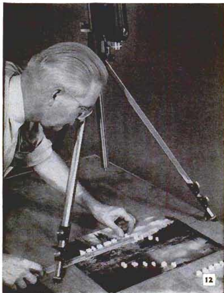
Fig. 12, to simulate letter movement, sequence of single-frame exposures of each are made as title is assembled
