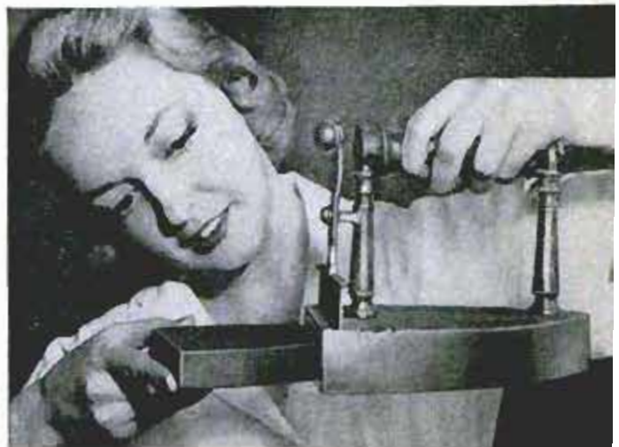
Above, center, balance-type scales were used in most country homes for checking weight of small items such as butter fresh from the mold, proportions of medicinal herbs. Object being weighed is placed on one tray, counterweight on other
