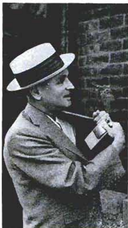
Left, radio-paging device buzzes to signal that phone call is being held. Right, operator sends out signal
