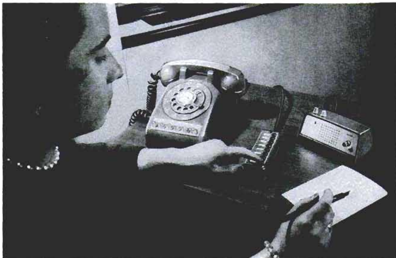
Operator of speaker-phone can set up a conference between remote and local stations by extra push buttons
