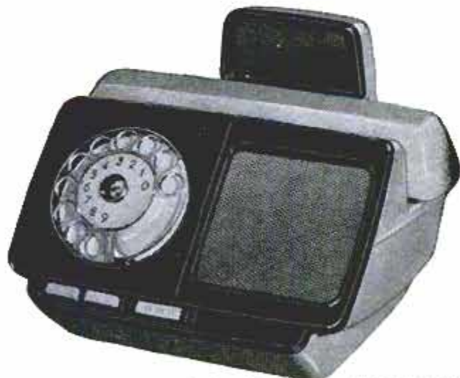
American-Swedish News Exchange photo Swedish WeGo-Phone has small loudspeaker beside dial so individuals or groups can talk back and forth
