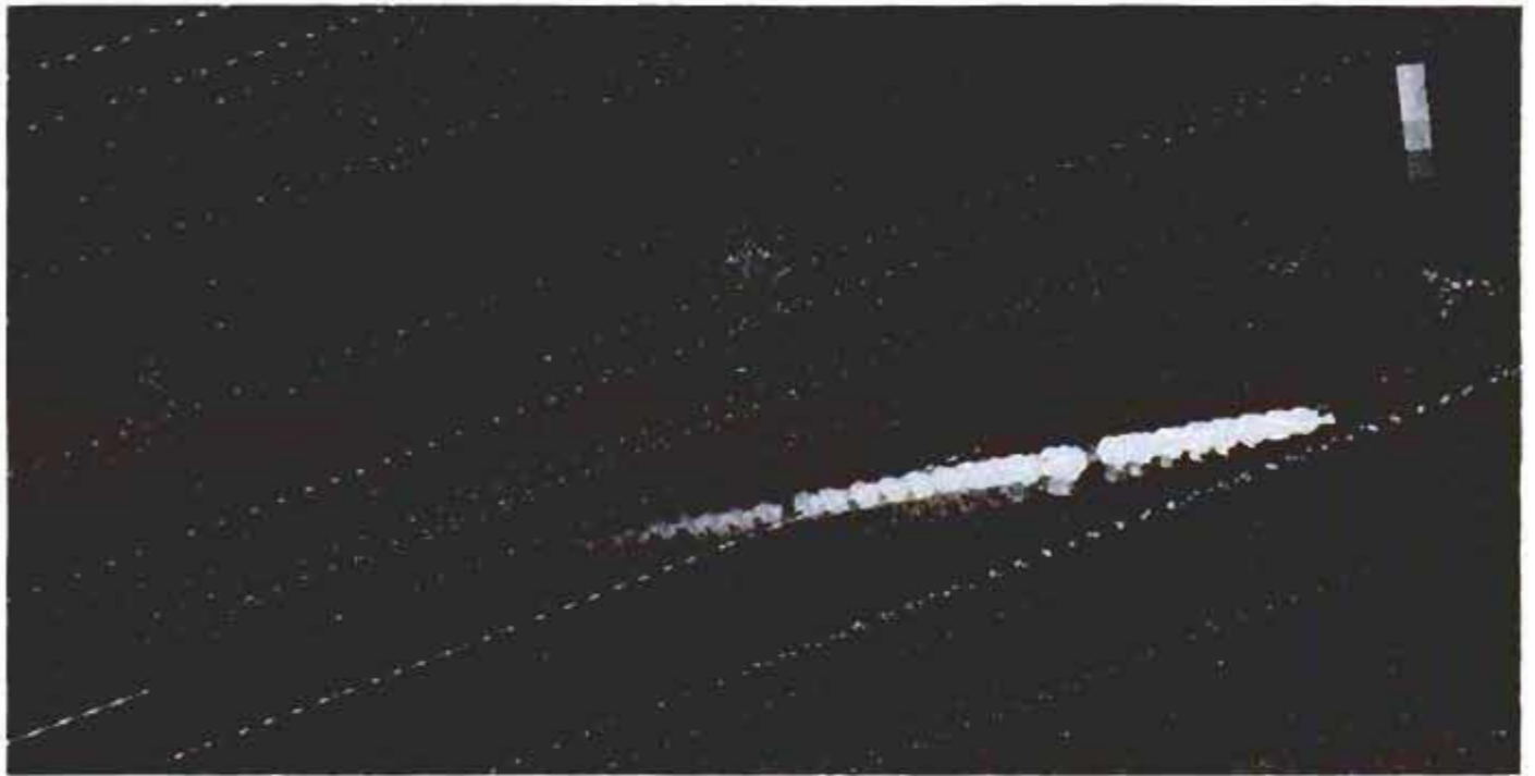
Multiple-exposure photo of radiation glow when released nitric oxide merged with free atoms of oxygen
