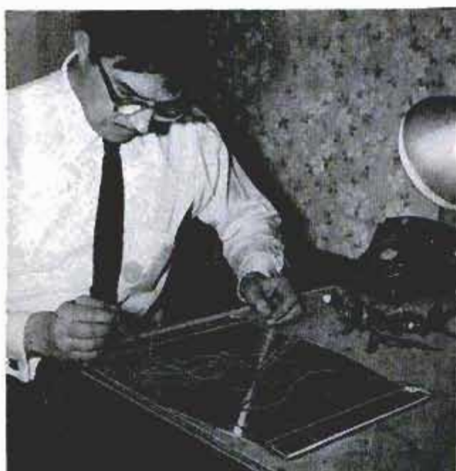
Hoffman technician cements in place the 20 solar cells which will operate a clock in Palm Springs, Calif. Sunlight powers the clock 24 hours a day
