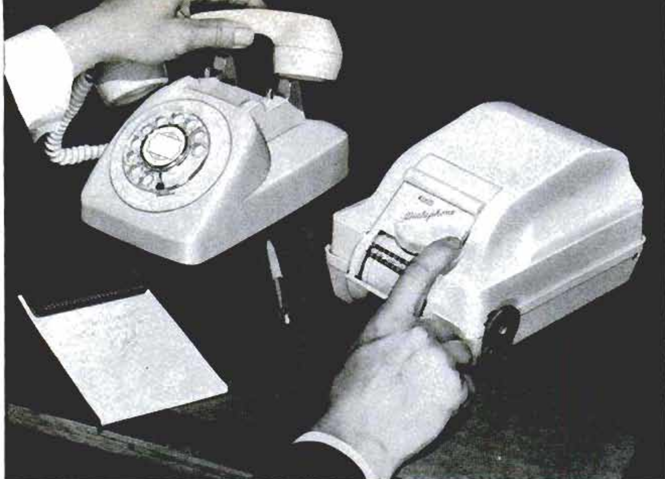
Caller turns knob on Dialaphone to name of person or company and perforated tape automatically makes call
