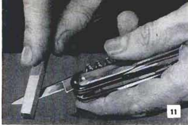
For a fine edge on a pocket-knife blade use a hard abrasive stick. Unless the edge is nicked or otherwise damaged, honing with the stick will suffice
