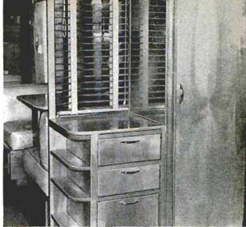
Venetian blind used as room break is left open for passage of light and air, closed for privacy. When not needed, the blind is raised up out of the way
