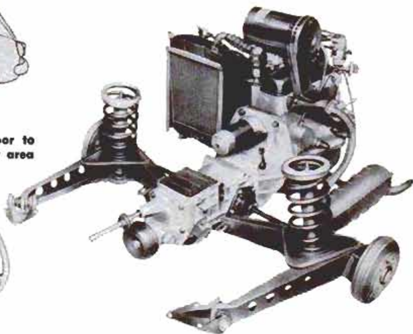
Illustrated here as an example of unconventional design, the Multipla has integral construction without a frame. These elements of the running gear attach directly to the unit body. All four wheels are independently sprung and the car, although very small, has excellent roadholding and a reasonable amount of comfort under most conditions
