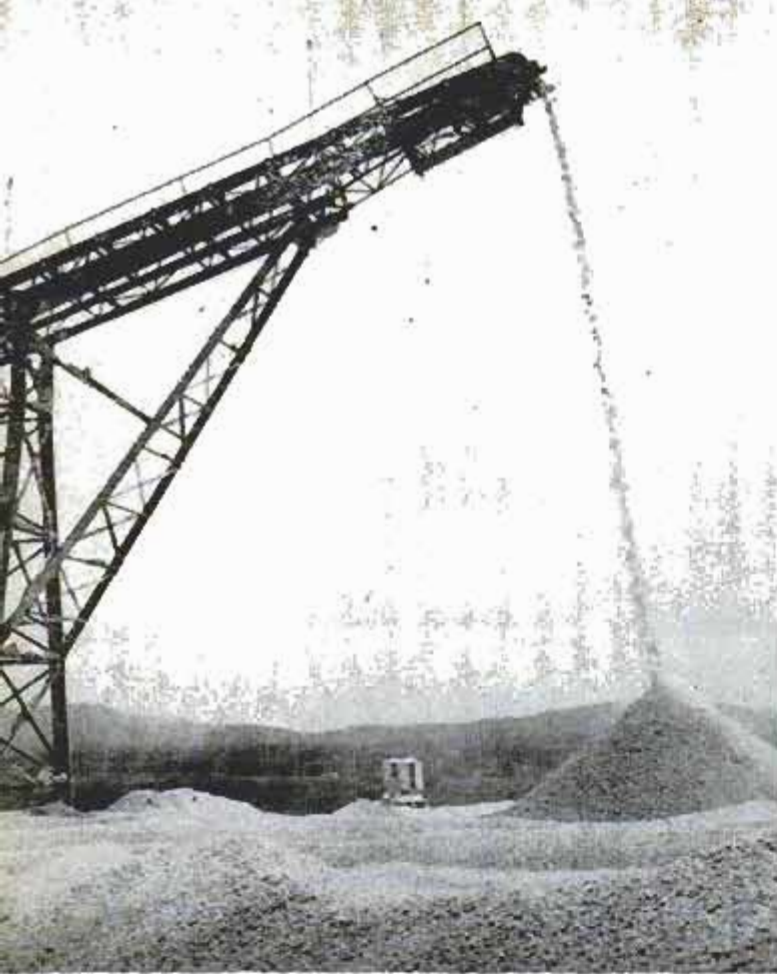
After the ore is mined in the form of huge boulders, it goes to a rock crusher. Pounded into gravel, it flows up a feed chute which drops it in a huge pile. Ore then is ready for shipment to processing plant
