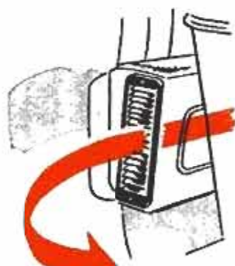
LINCOLN CLEVERLY USES ITS FRONT-DOOR ARMREST AS A DUCT TO PIPE HEAT INTO BACK SEAT
