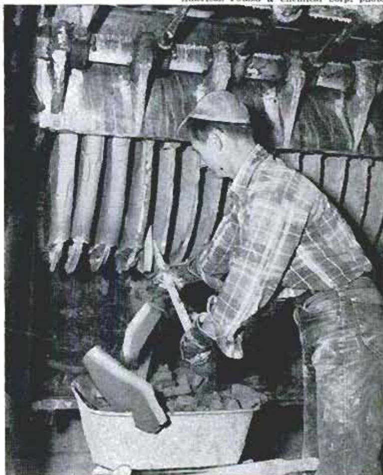
Workman removes cakes of lithium concentrate from filters American Potash & Chemical Corp. photo
