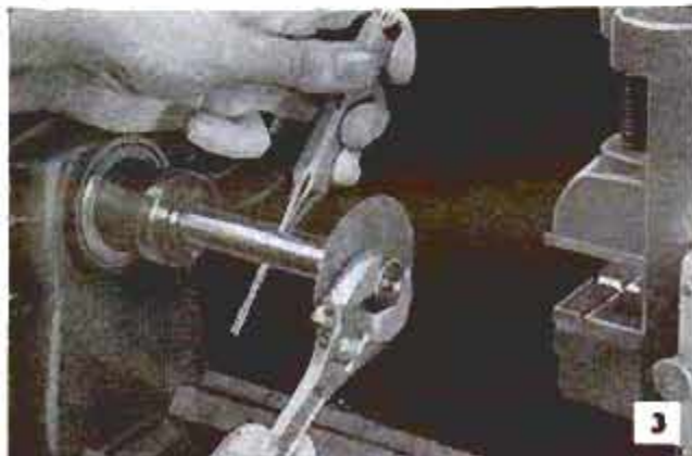
Arbor can be driven from lathe-spindle by collet chuck or by adapter having a No. 1 or 2 Morse taper. Note use of pin punch when loosening the arbor nut
