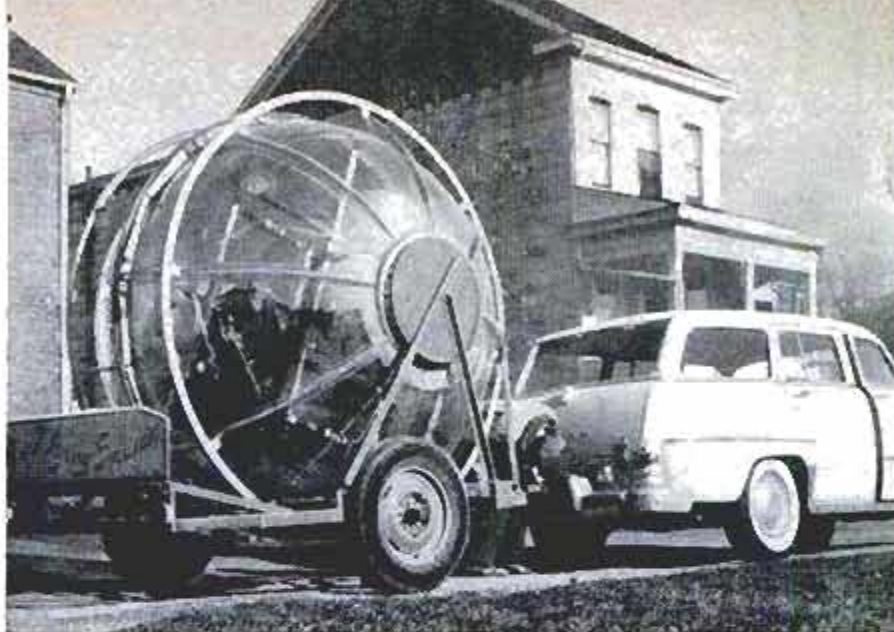
Sphere can be rolled onto its special trailer which has ramplike track
