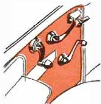
CADILLAC'S FRONT DOOR HAS A CLUTTER OF HANDLES, NOT ALL OF WHICH ARE WELL POSITIONED
