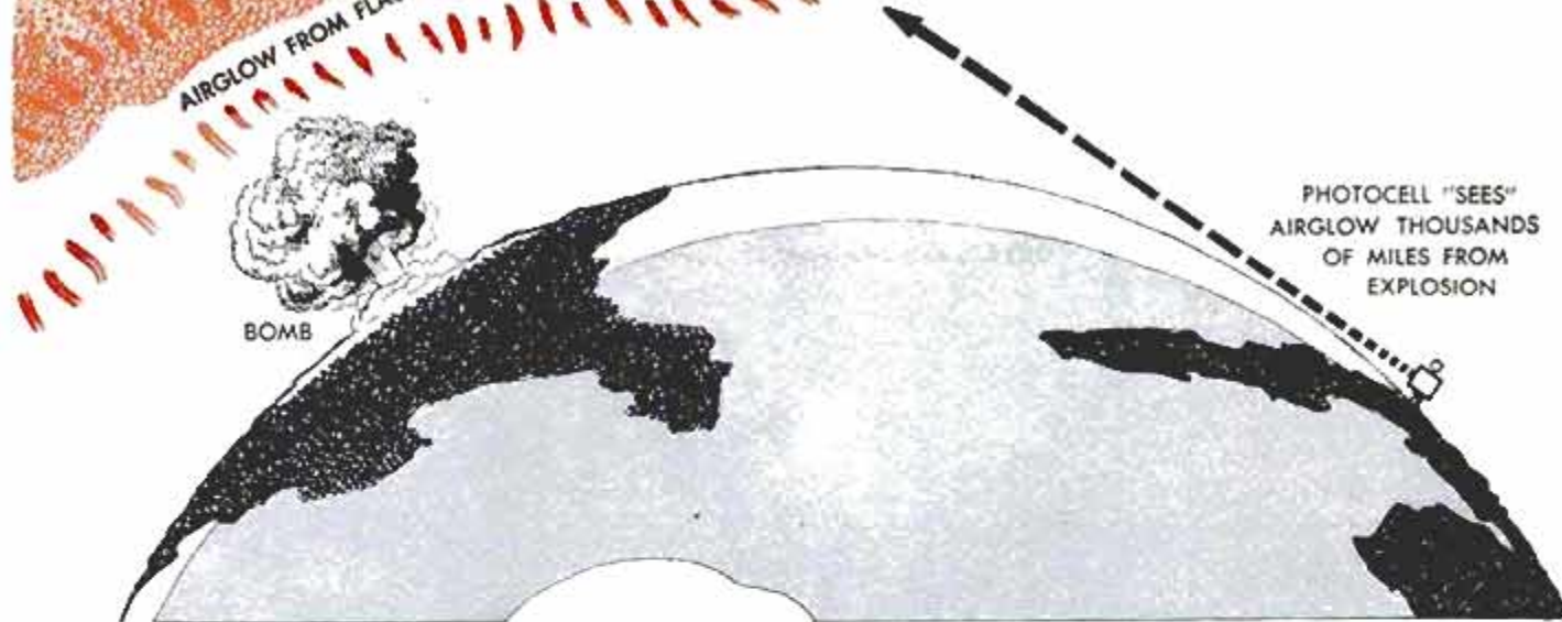
Thermal radiation from a bomb excites air particles, causing a glow that can be "seen" by photocells
