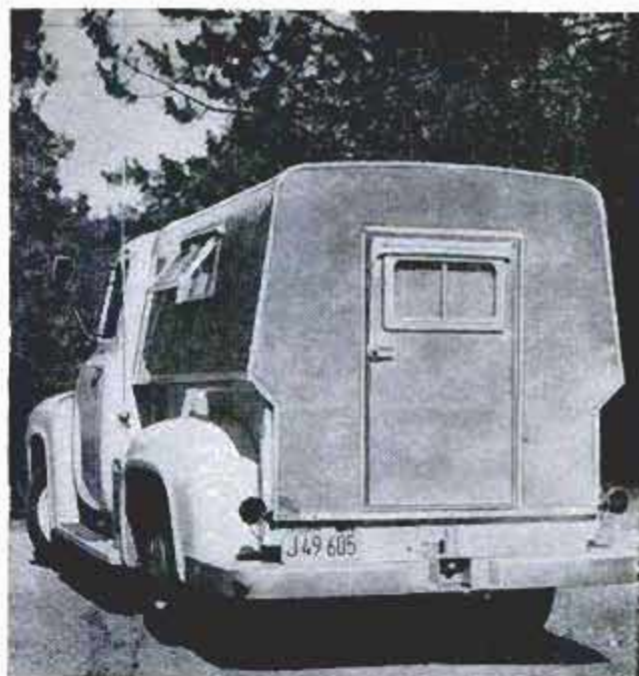
All-aluminum exterior of shelter cab reduces maintenance problems and helps to keep interior cool
