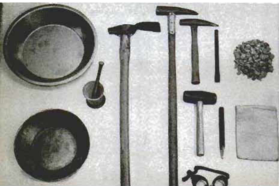
Tools for prospecting include large and medium-size pans, steel mortar and pestle, picks, chisels, chip samples and goggles
