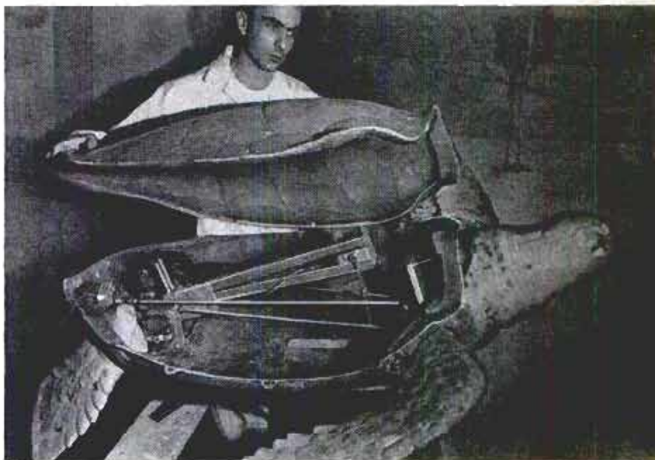
Above is a turtle with its upper shell removed, showing the body's mechanical organs. Below, motions of a manta ray and giant turtle are tested. The manta's movements are created in its wing tips by puppet wires leading from the trolley. The turtle's head and flippers are moved by internal motors
