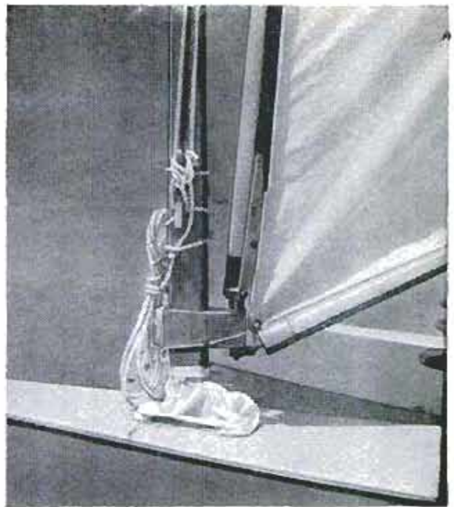
Gooseneck fastened to mast has fittings for attaching boom and lower end of gaff for lateen-type sail
