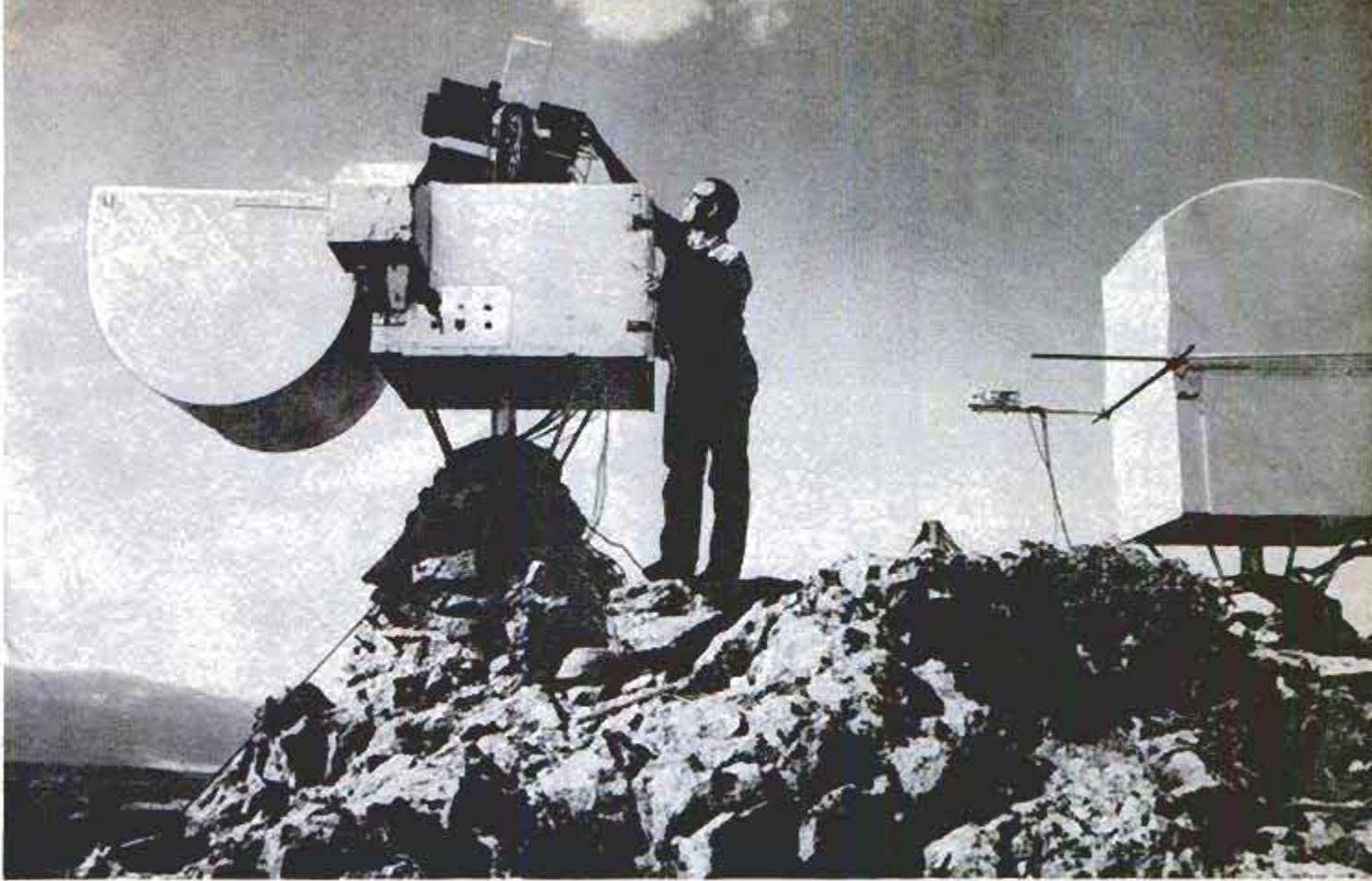
Instrument on Colorado mountaintop measures airglow, caused by a chemical process in the upper atmosphere
