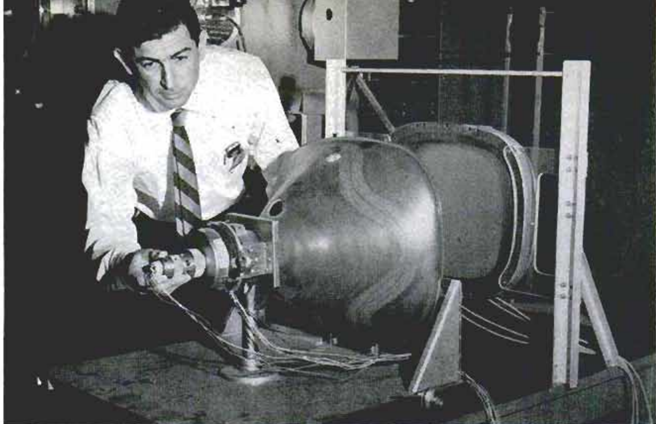
Components of TV receiver are installed in vacuum chamber, where tubes work well with glass covers removed
