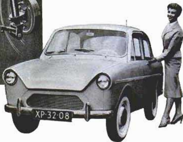
Front suspension has low-slung transverse leaf spring. Shocks and kingpins are combined. Turn-circle diameter: A tiny 28 feet
