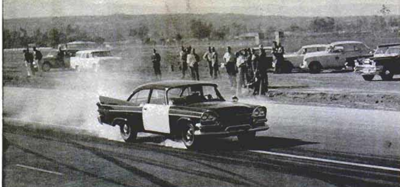
Smoke pours from tires as California state trooper puts test car in a panic stop from 60 miles per hour
