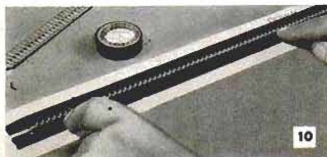
Above is shown method of modifying tank treads so they are more flexible. Original connector link on end of each tread is removed. Below, brass screws in control-box lid press on spring battery contacts
