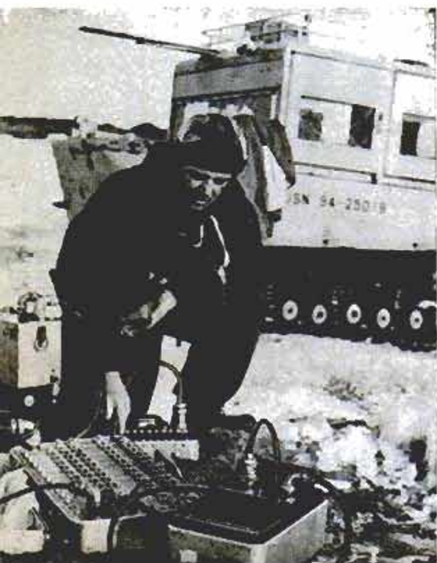
Seismic recorder is used in Antarctica to determine thickness of the ice by bouncing sound waves off underlying rock. Diagram shows research indicating Antarctica may be group of islands
