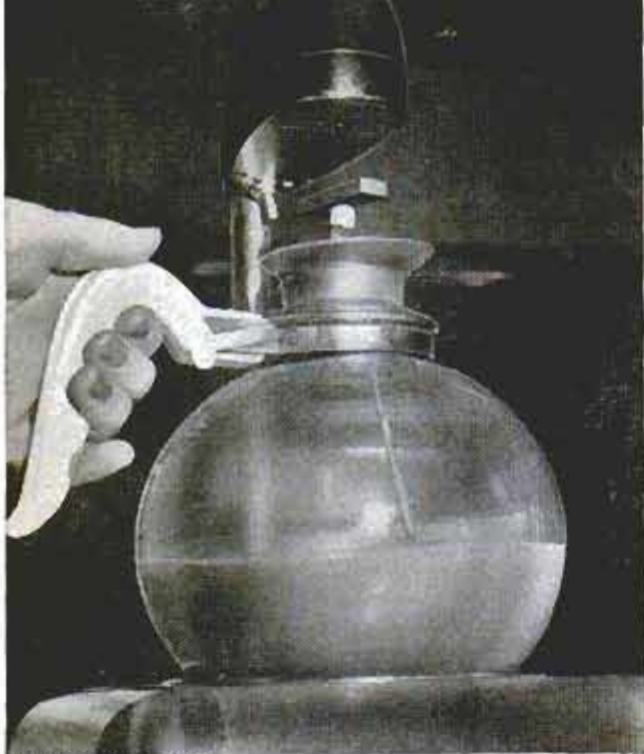
Krim-Ko Corp. photo Motor-driven magnet in housing atop Silex turns stainless-steel paddles to agitate pot of chocolate
