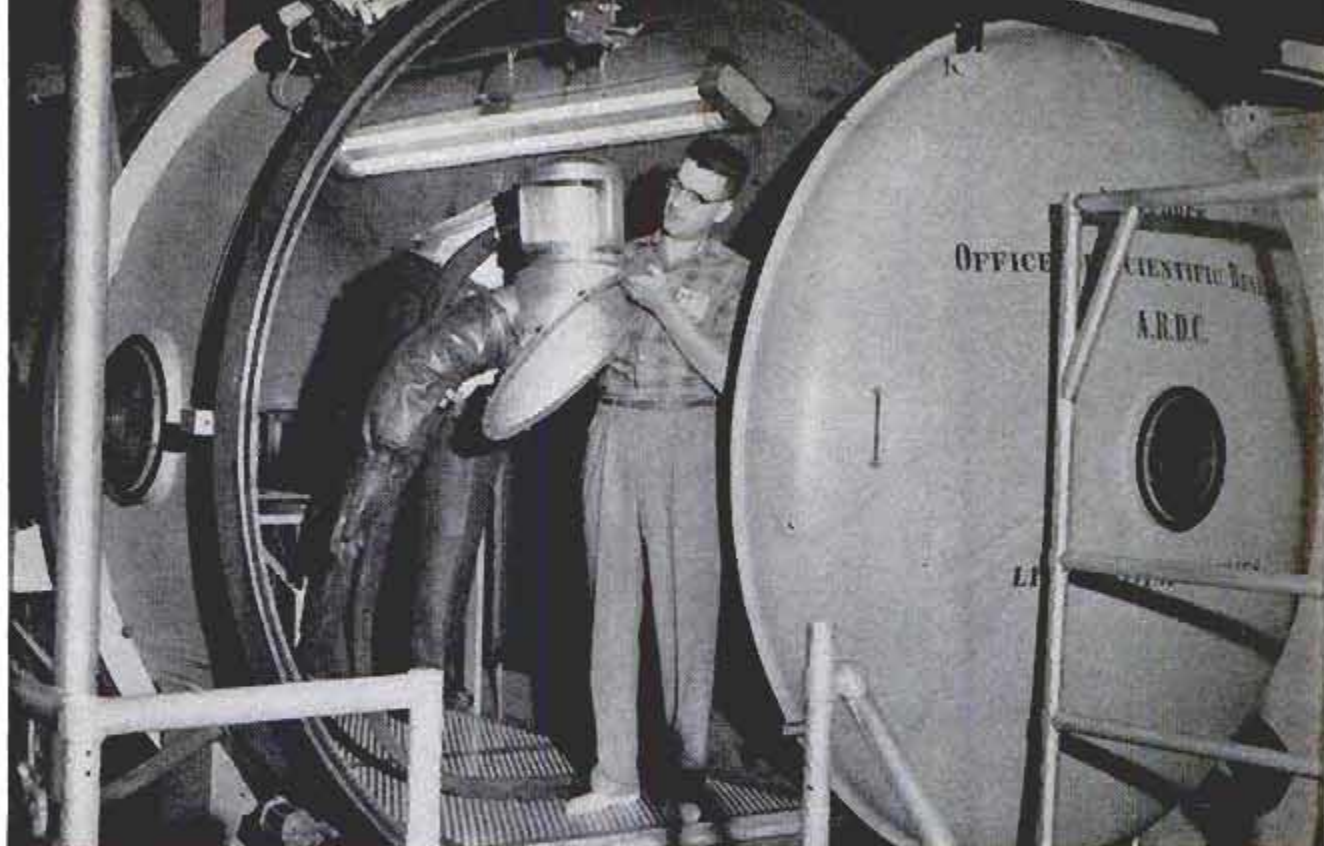
Door of chamber rolls aside. Pumps in chamber remove all but one of every 18,000 molecules of air inside
