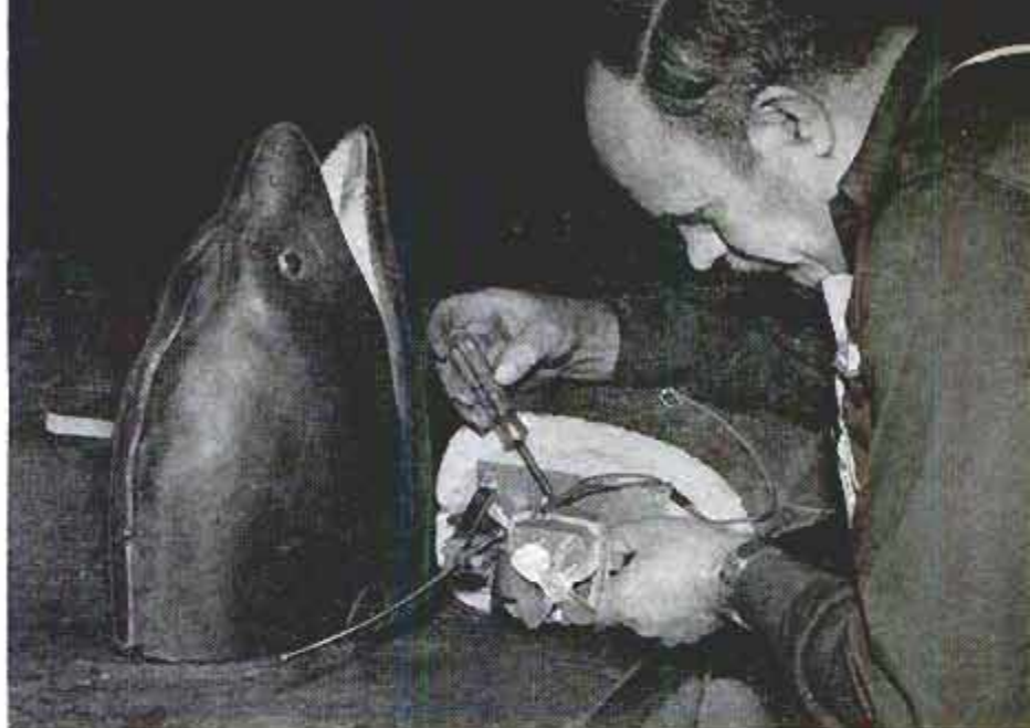
An internal electric motor lends sinuous motions to the body of this big moray eel, composed of rubberlike sponge plastic
