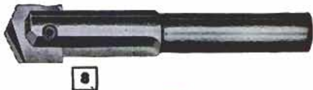
8. SPADE DRILL for hard-to-machine metals comes with replaceable blades and provision for circulating coolants through shank. Wide range of sizes available Robert H. Clark Co., 9330 Santa Monica Blvd., Beverly Hills, Calif.
