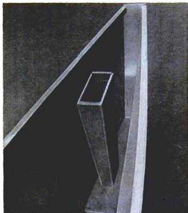
Below, mast trunk is glued in step-block cutout. Later, the top is nailed to deck beams and decking
