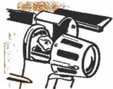
STYLISTS SEEM TO FEEL THAT GAS-TANK FILLER TUBES ARE INDECENT AND MUST BE HIDDEN. OLDSMOBILE HIDES IT IN THE LEFT TAIL-LIGHT ASSEMBLY.
