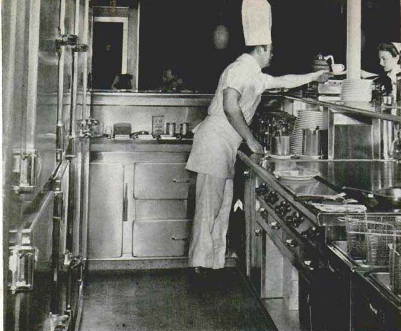
Chef stands before push-button console of electric griddle. In foreground are electric deep-fat fryers
