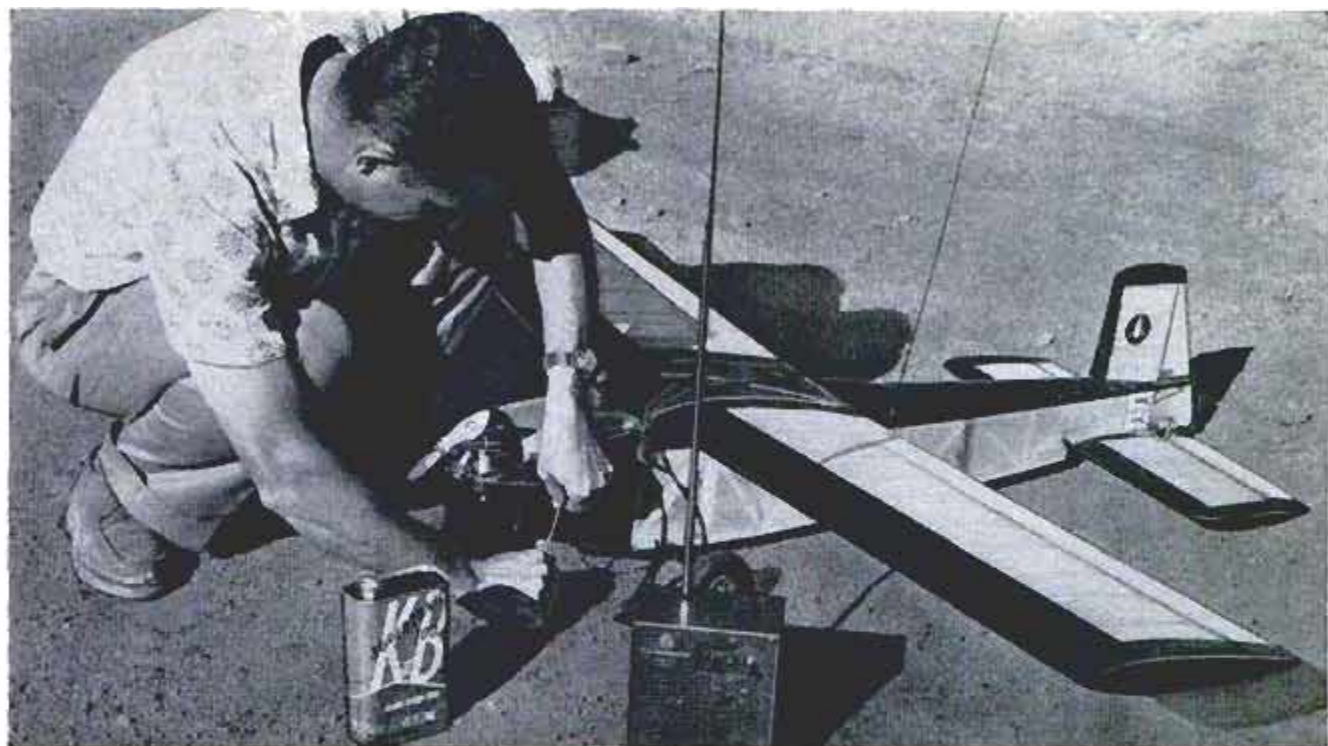
After fueling and starting the engine, owner uses radio to put model through any maneuver of full-size plane
