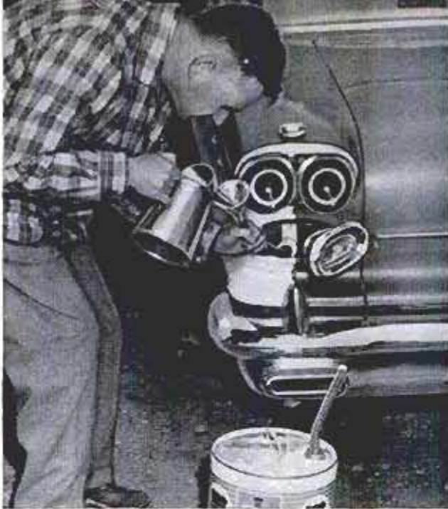
If you run out of gas, you need a long hose to pour into tank. Flexible spout on can is not long enough
