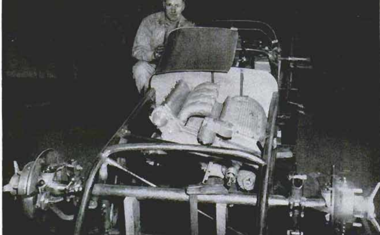
Its Offy engine horizontal, the Quinn Epperly car retains the solid front axle, unlike the Kurtis car below
