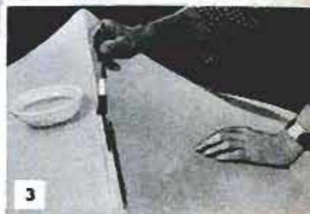
Fig. 3. Epoxy-resin mixture is flowed into deep scratches on keel of hull with small paintbrush. Several coats are required
