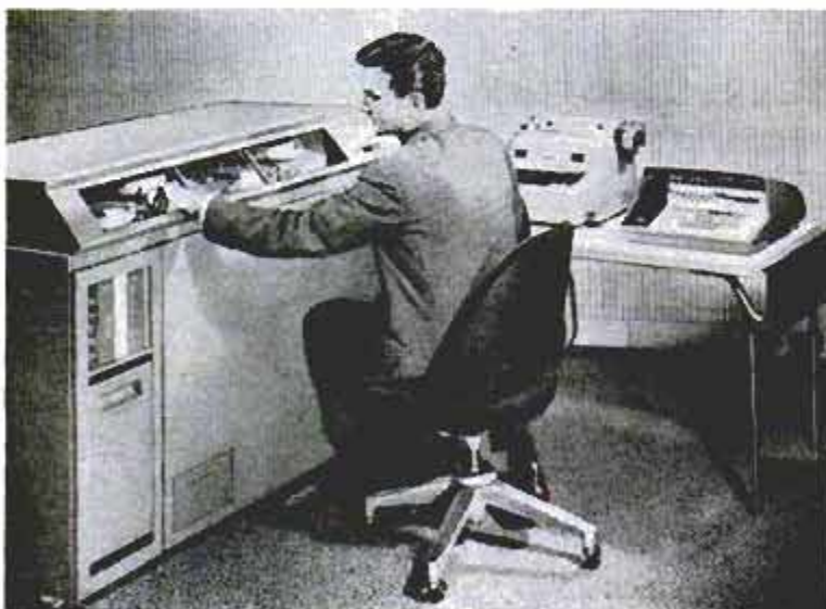
Operator checks IBM desk-side machine that solves many problems now handled by big computers. Typewriter gives answers
