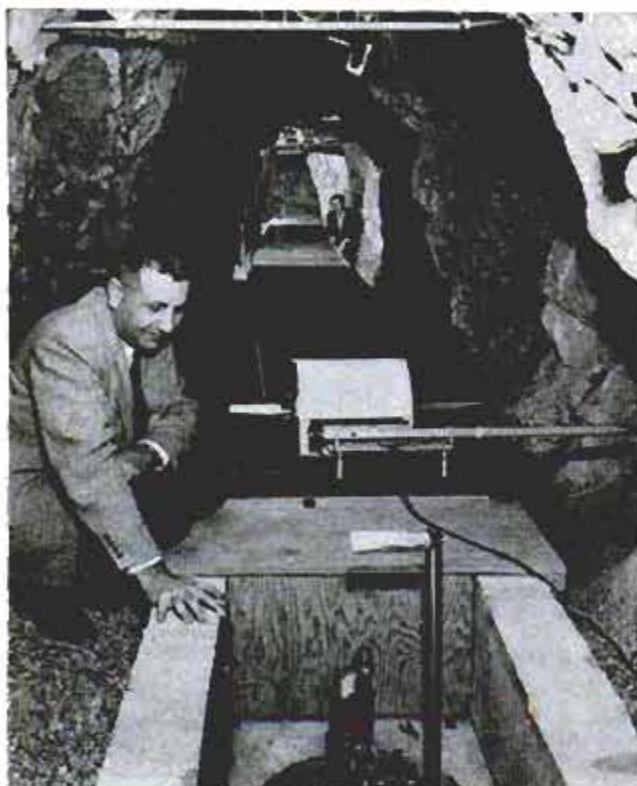
Strain seismograph in tunnel 25 miles from San Andreas fault detects slight pressure on earth's crust
