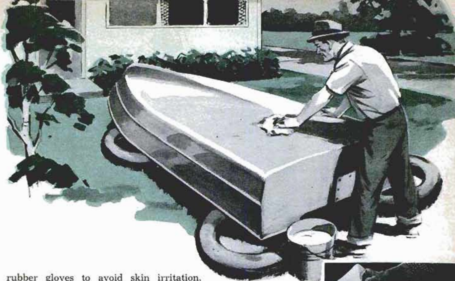
Fig. 3. Epoxy-resin mixture is flowed into deep scratches on keel of hull with small paintbrush. Several coats are required
