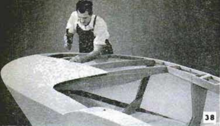
FRONT AND REAR SEATS ARE SIMILAR IN CONSTRUCTION. NOTE ARC ON BACK OF REAR SEAT, FRONT SEAT HELD IN POSITION WITH ANGLE BRACKETS AND WING NUTS AND BOLTS. REAR SEAT MOVABLE TO ALLOW ACCESS TO STORAGE SPACES UNDER STERN DECK. DISTANCE FROM FRONT SEAT BACK TO DASH 27" TO 30" AS DESIRED
