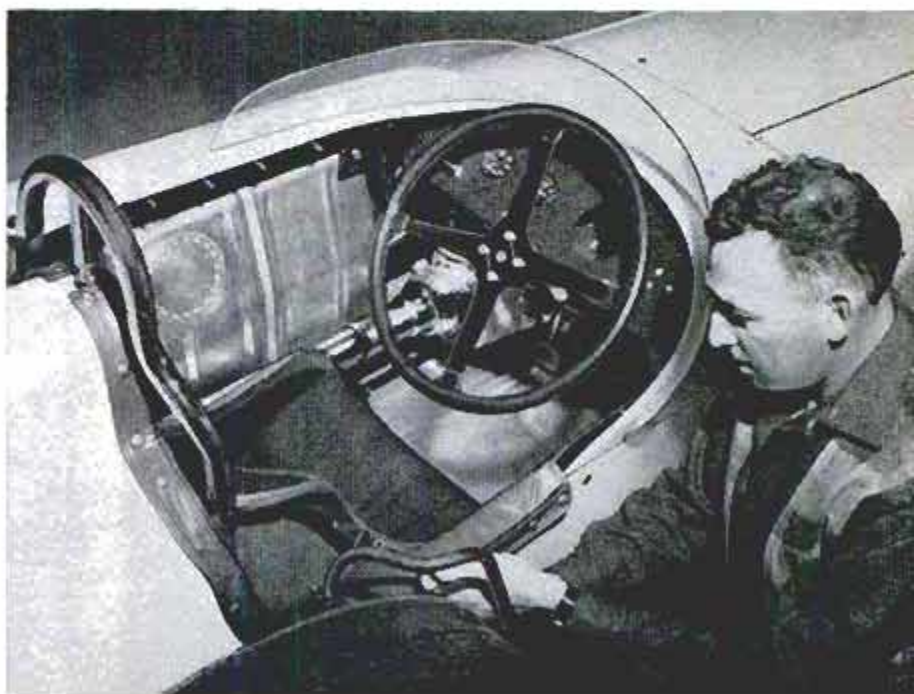
Author Salih fits a guard on car to keep driver's elbow from accidentally hitting rear tire. Note the driveshaft location
