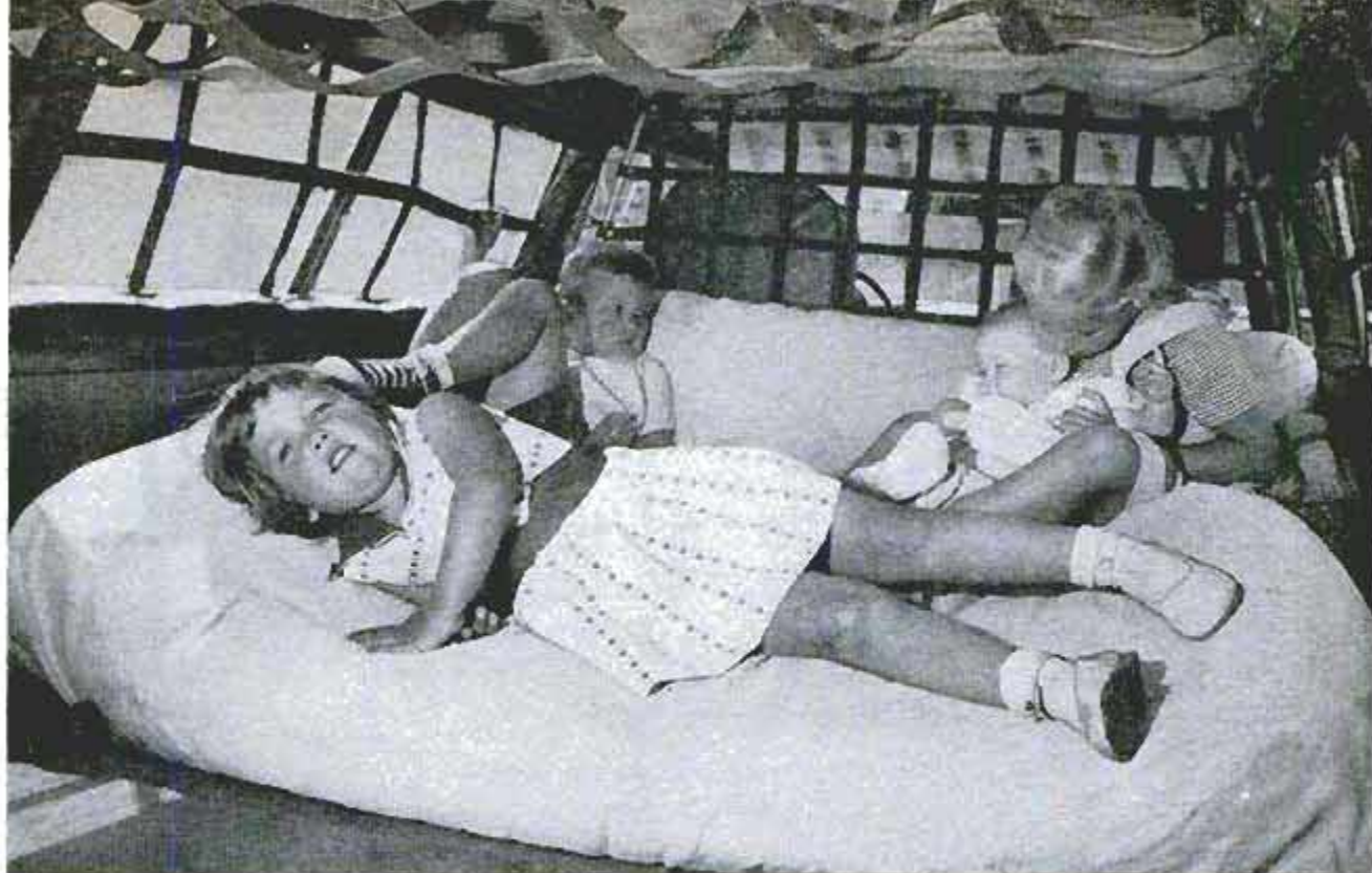
Children play in the back seat, surrounded by safety nets. All the interior surfaces have been padded
