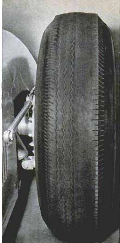
Tread is not for traction but to indicate wear. Drivers would like no grooves at all
