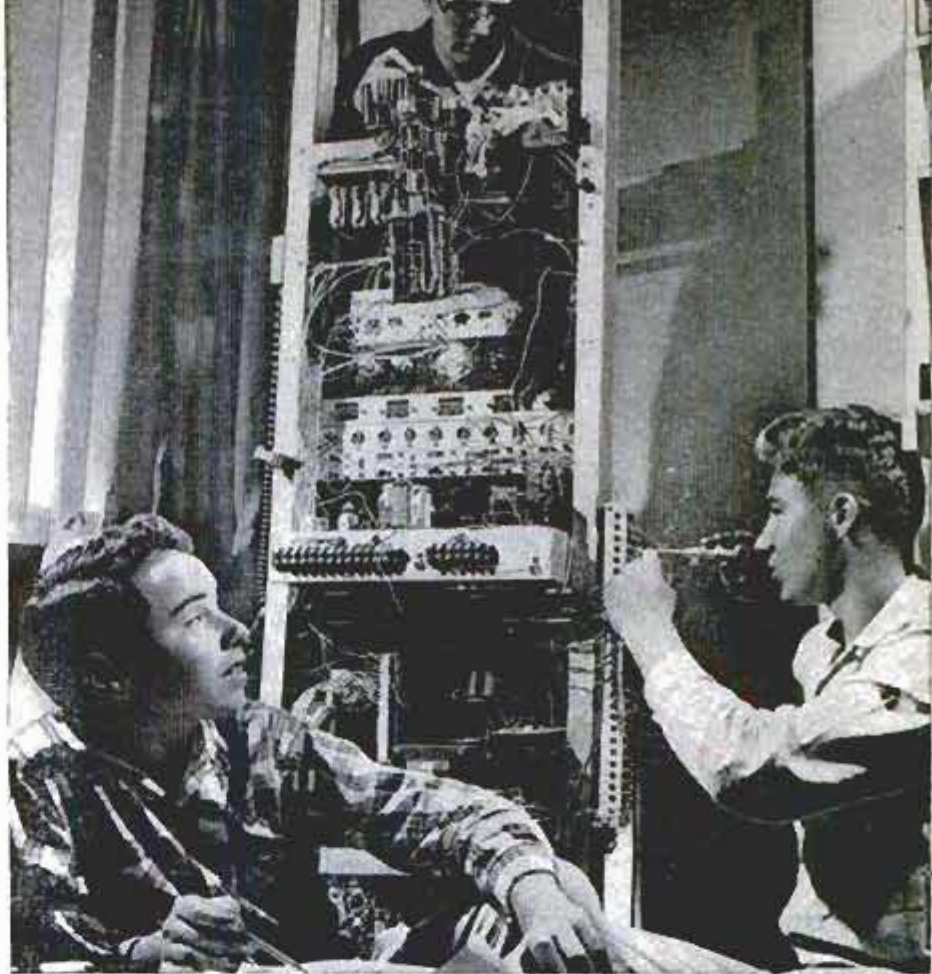
Growing pains: Circuits in switchboard must be rewired to handle a new subscriber. Switchboard limits number of phones
