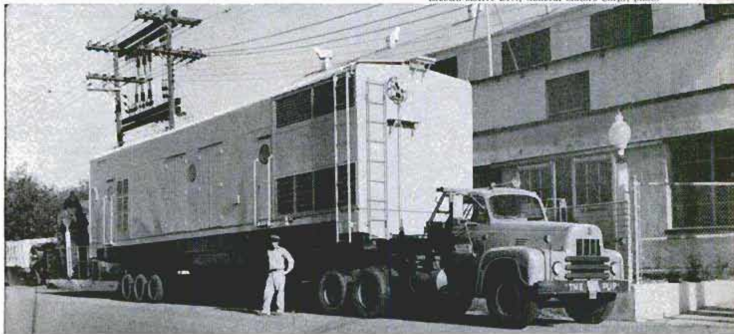
Massive 1000-kilowatt mobile generator of the West Texas Utilities Company can relieve a central station
