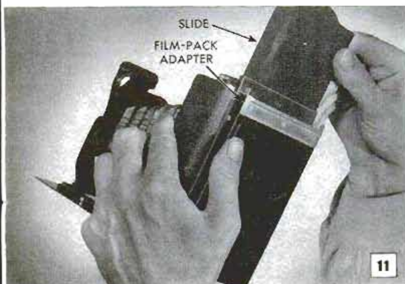
Fig. 11, film pack must fit snugly in adapter on camera and accept and permit withdrawal of slide without entry of light that would damage film
