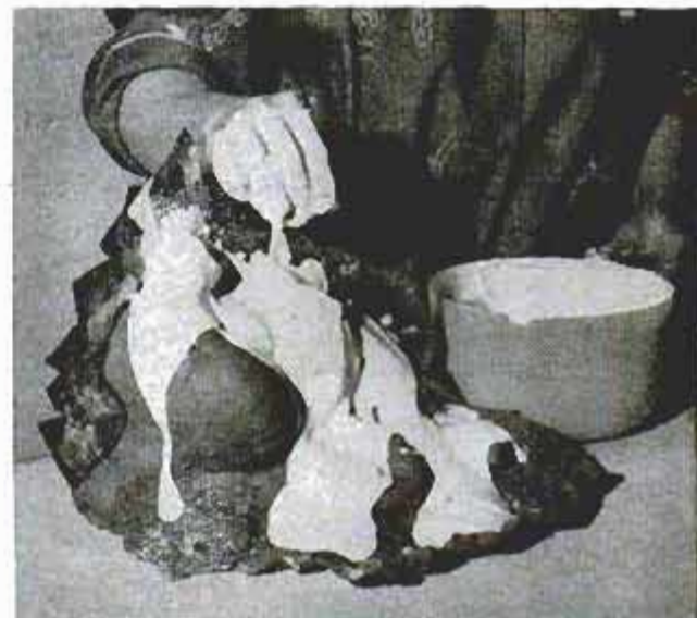
Each side of clay face is cast separately. Enough plaster of paris is added to form 2-in.-thick layer
