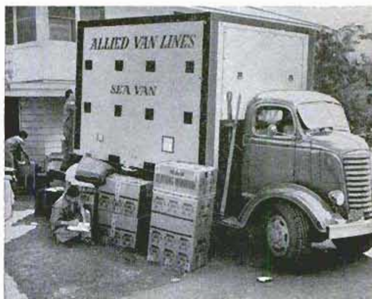
Piggyback Sea Van rides flat-bed truck and will be deposited in hold of a ship for trip overseas. One van can hold contents of a four-room home. Exterior is plywood
