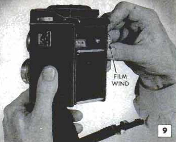
Above, film-wind knob should move forward only without binding or excessive play. Parts that come in contact with film must be smooth and free of rust
