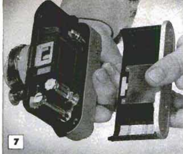
Loose-fitting camera back should be checked for light leaks that may be caused by missing or tightly compacted yarn packing in grooves in camera body
