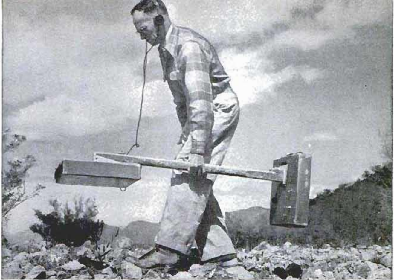
Closing in on elusive particles from outer space. Dr. Nininger uses a mine detector to find meteorites
