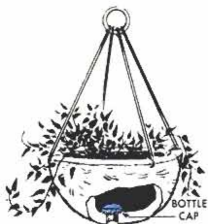
HANGING PLANTER is coconut half-shell with bottle cap over drain hole drilled in bottom
