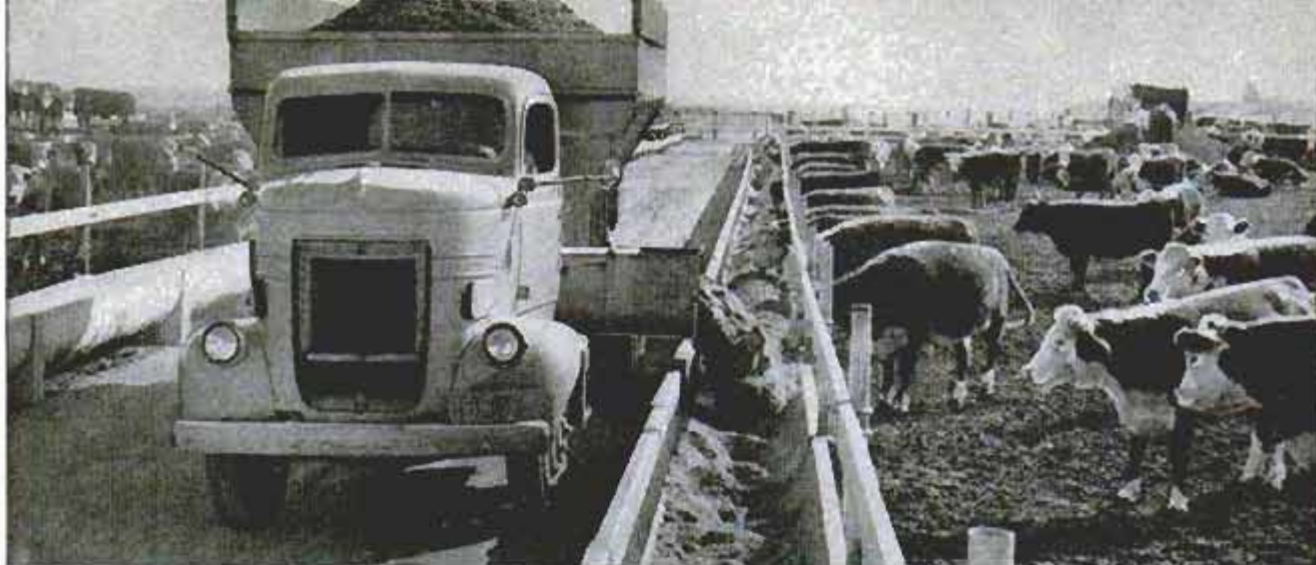
Another method of feed delivery makes use of trucks equipped with augers that empty feed into yard troughs
