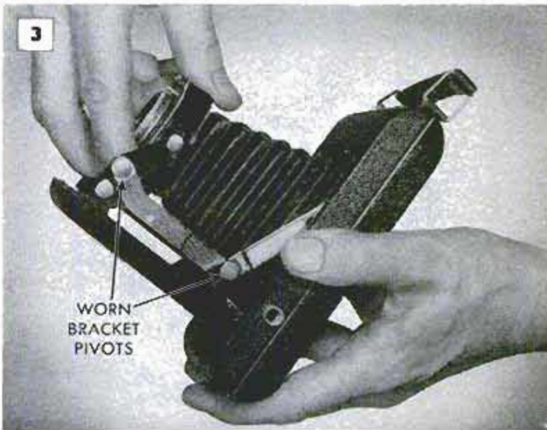
Below, worn bracket pivots or bent brackets that hold lensboard in required position may cause lens misalignment and make accurate focusing impossible
