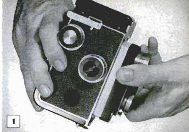
Above, condition of focusing mechanism of twin-lens reflex camera is determined by noting amount of play found in members of movable lensboard
