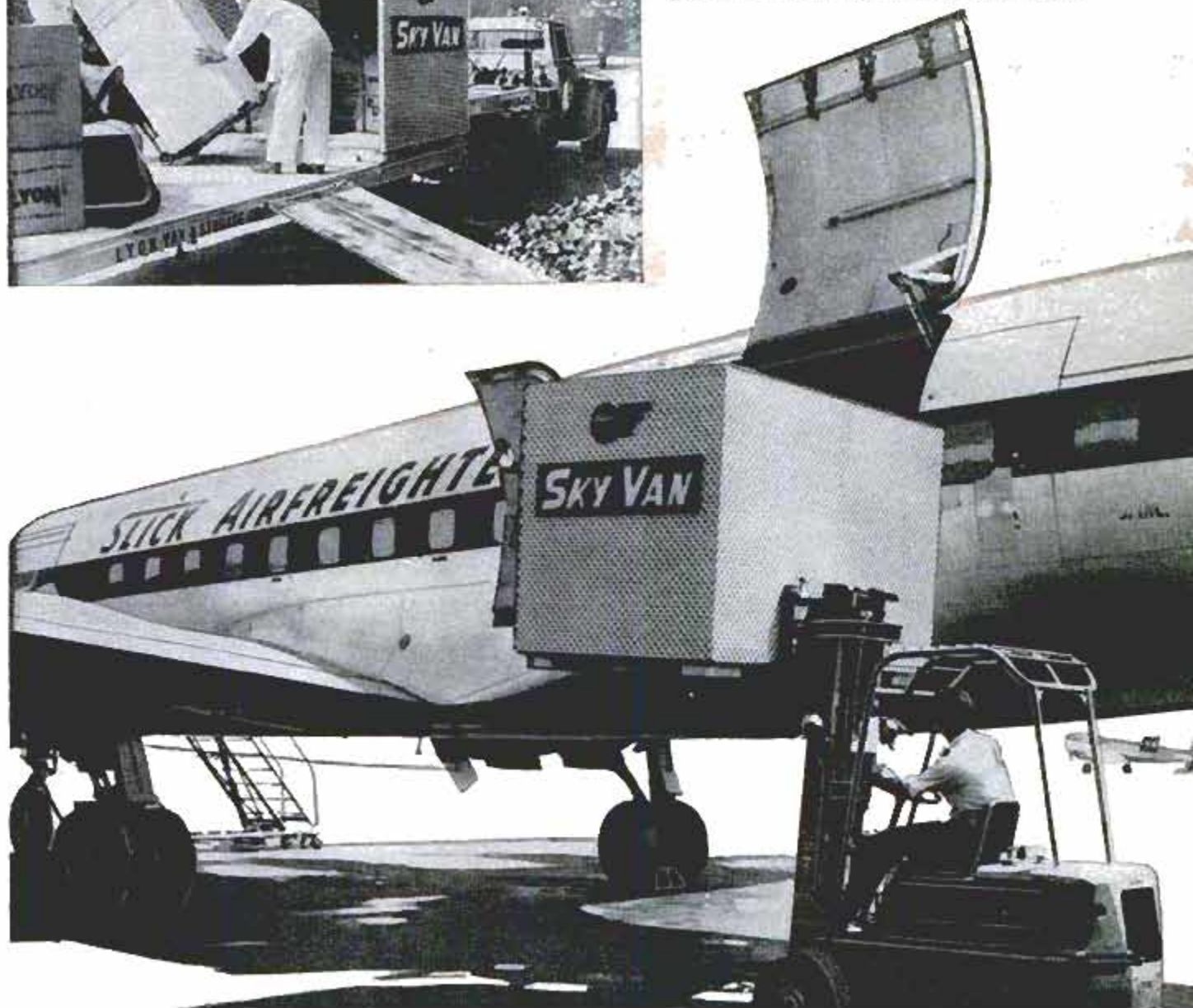
Sky Vans are packed on flat-bed truck at home of family (left) then taken to airport and loaded by fork lift to freighter
