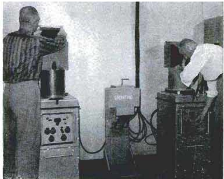
Cameras supplied by weather bureau are mounted on radarscopes to make a photo record of any rainfall within 100 miles
