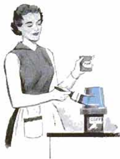
FLOWERPOT placed on coffee can for painting, can be rotated without touching pot for fast smudge-free paint job
