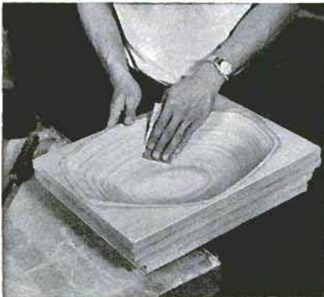
Next he sands it smooth. Later, he raises the grain by soaking the bowl in water and sands it again
