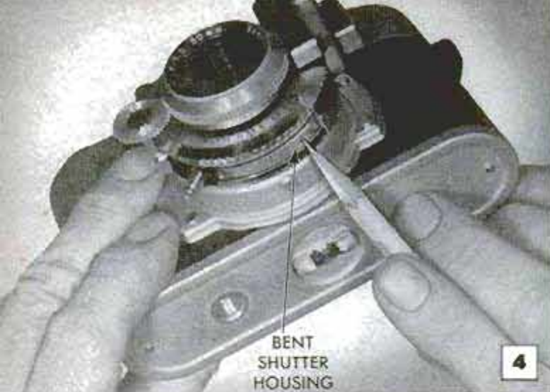
Above, this camera has been dropped on hard surface, resulting in severe damage to shutter housing and attached mechanisms making the shutter inoperative
