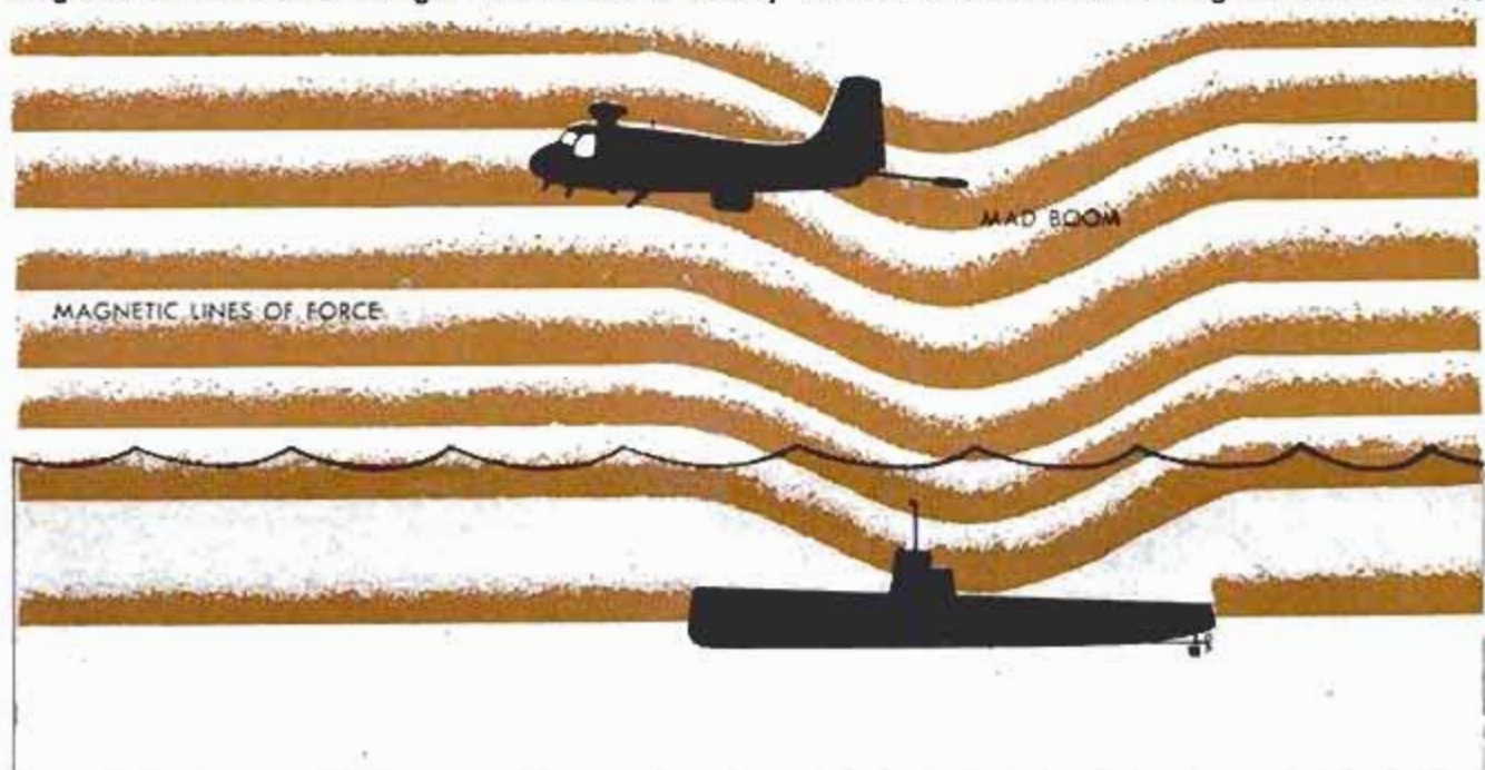
Magnetic airborne detection gear shows sub is nearby because of disturbance of magnetic lines of force
