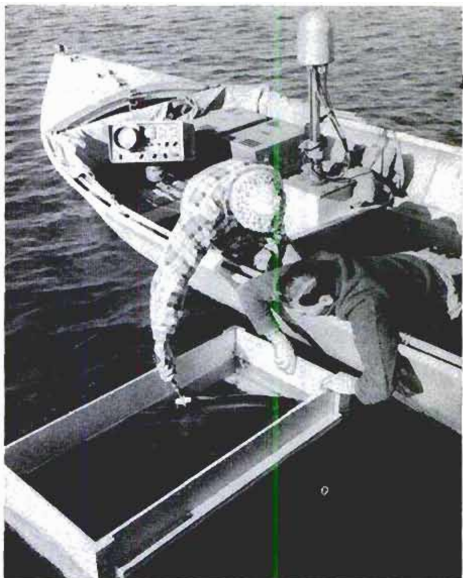
Salmon are tagged in 30 seconds inside a trap. Tag is attached by a "hog ring." Aboard boat is automatic sonic tracking-ranging receiver
