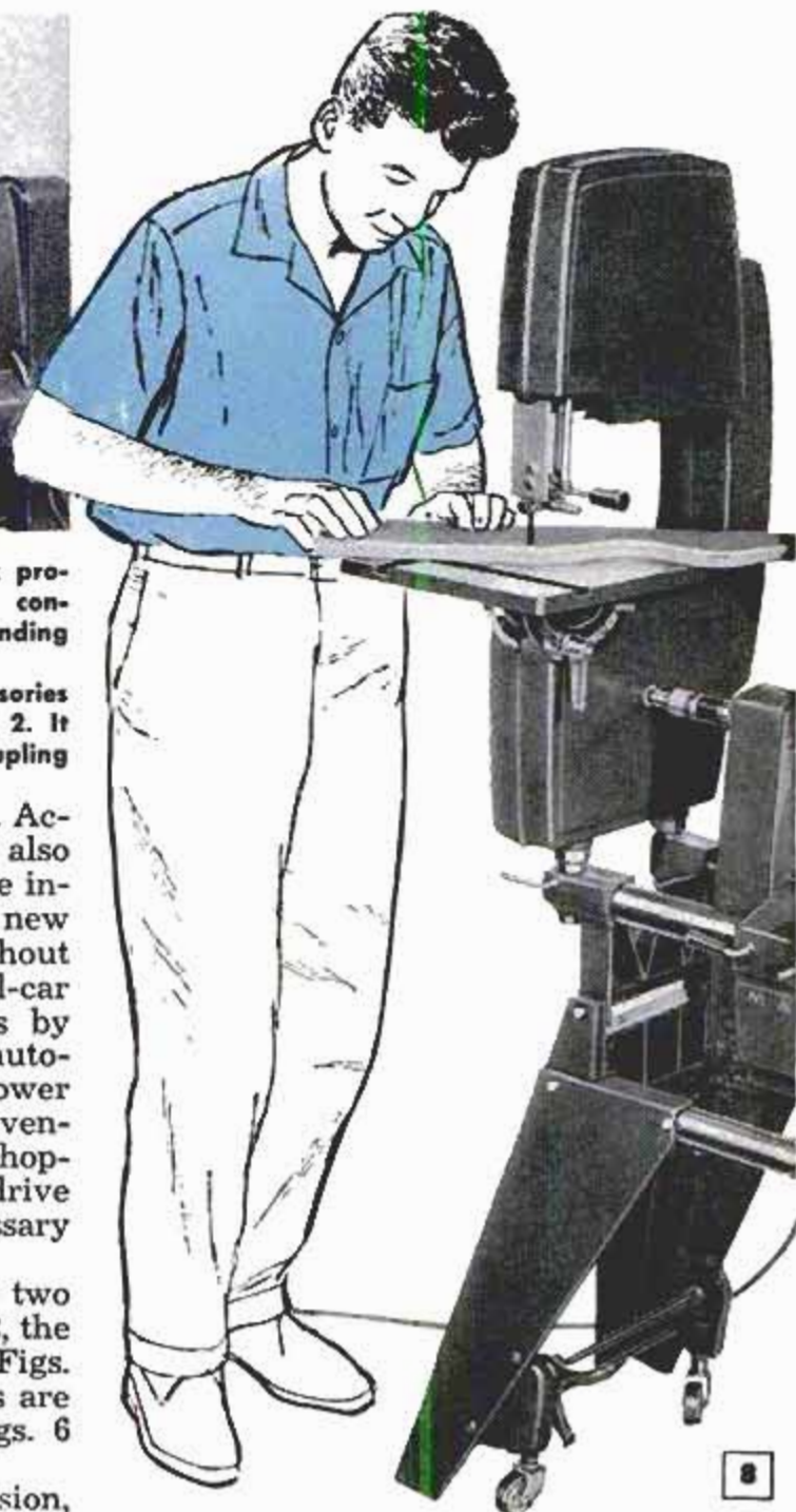
Desired speed is dialed on Mark 5. An expandable pulley on motor shaft is widened or narrowed by dial mechanism to increase or decrease pulley dia.
