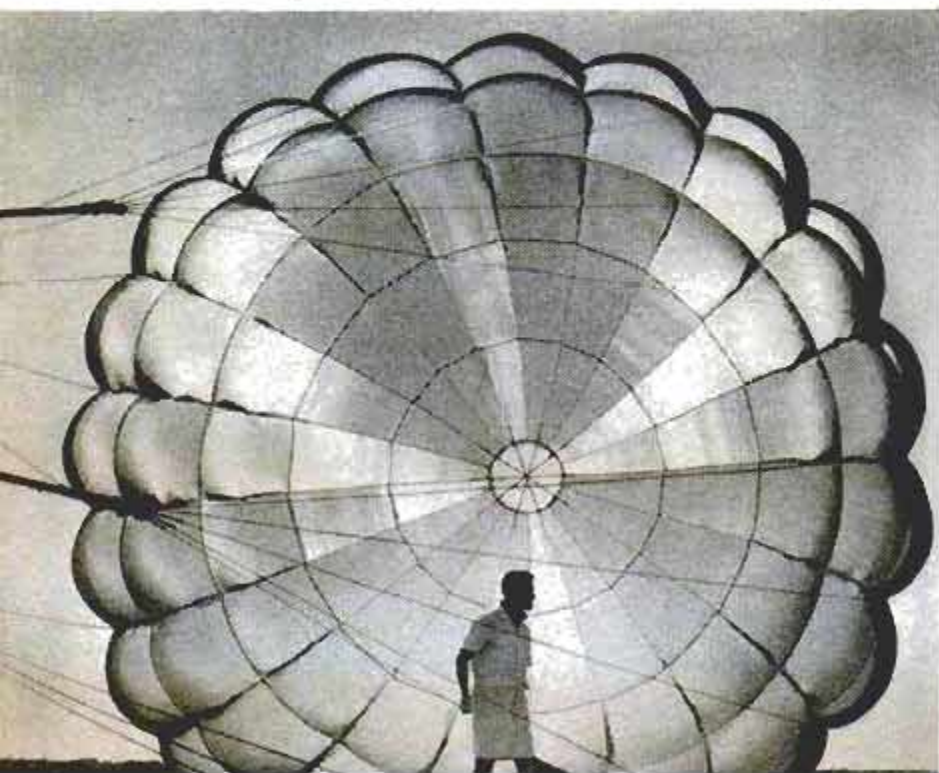
Multicell parachute canopy developed by Jalbert will carry 35 to 40 percent greater load than a conventional parachute
