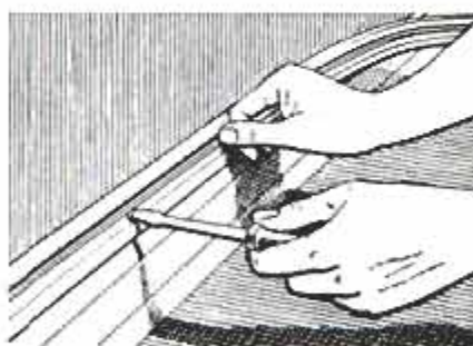
2 Remove old outlet strip
