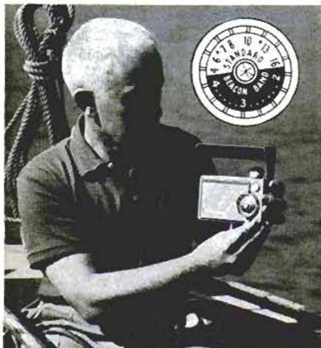
Fig. 1. Motorola's Weatherama, a transistorized portable covering beacon and standard broadcast bands
