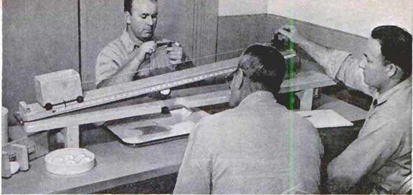
Egg-breaking machine tests shell's strength. Researchers discovered that Terramycin makes shells stronger
