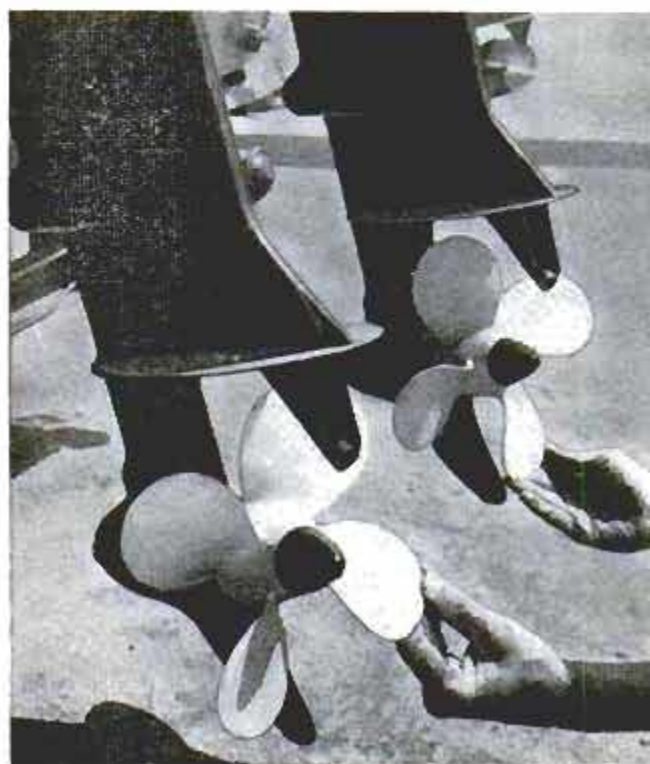
Fig. 1. Make visual inspection of propellers. Nicks, dents or bent blades might cause excessive vibration
