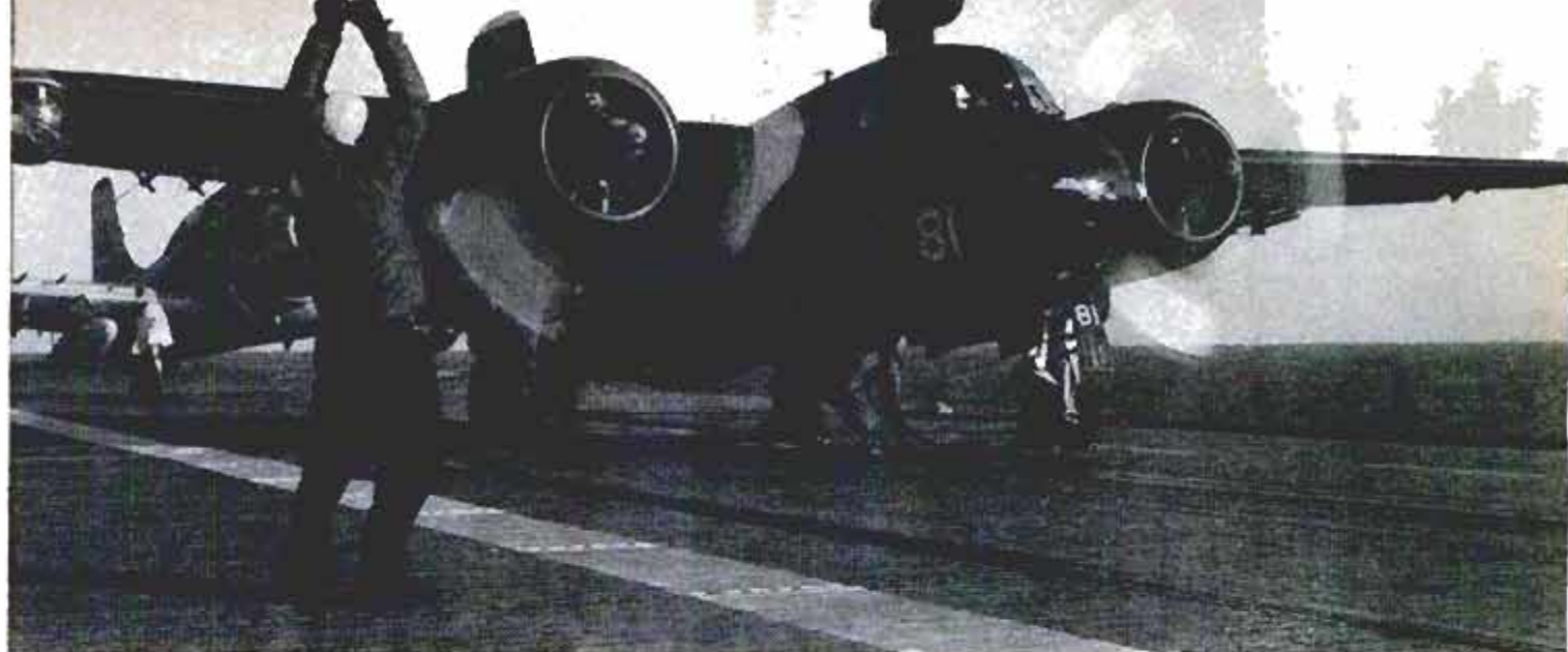
Plane director positions Tracker for take-off from a carrier. Practice rockets are visible under the wings
