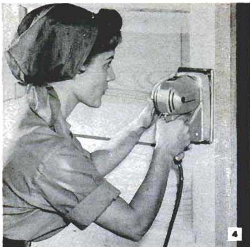
Above, pad sander works just as effectively on a vertical surface as on horizontal table top. Below, while not all-inclusive, the table lists and describes abrasives suited to pad sanders
