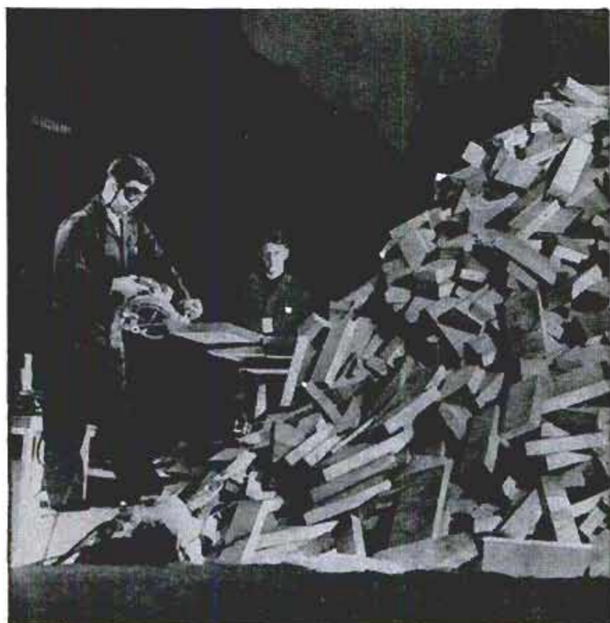
Test runs through the night. After 24 hours, saw was still going strong. It was then put on laboratory testing machine to continue test* for 6 more days and nights.
