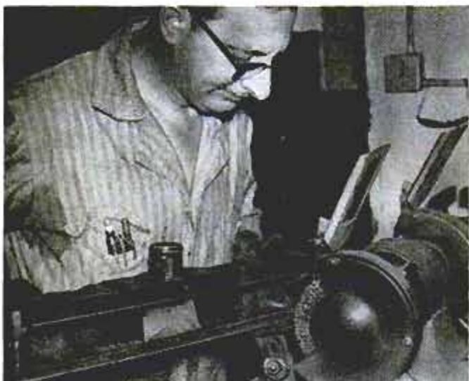
Edges of upper and lower tanks are wire-brushed to remove rust, dirt and scale to assure complete tinning in preparation for soldering them to new core
