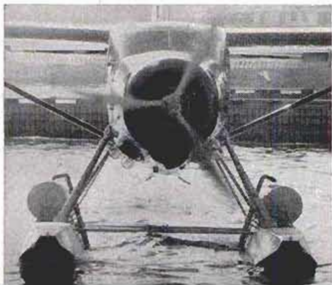
Canadian Otter aircraft sprays water from pontoon tanks, above, during test at Sault Ste. Marie. Refill pipes force water into tanks as plane taxis
