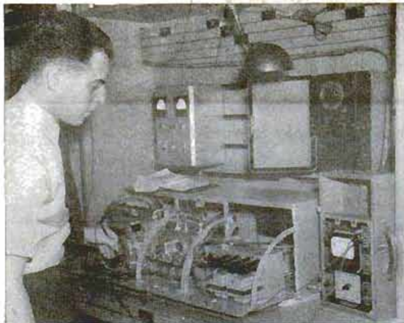
Engineer checks an experimental model of a new electronic alarm system designed for a bank vault. These alarm systems are so sensitive they are activated by the slightest sound
