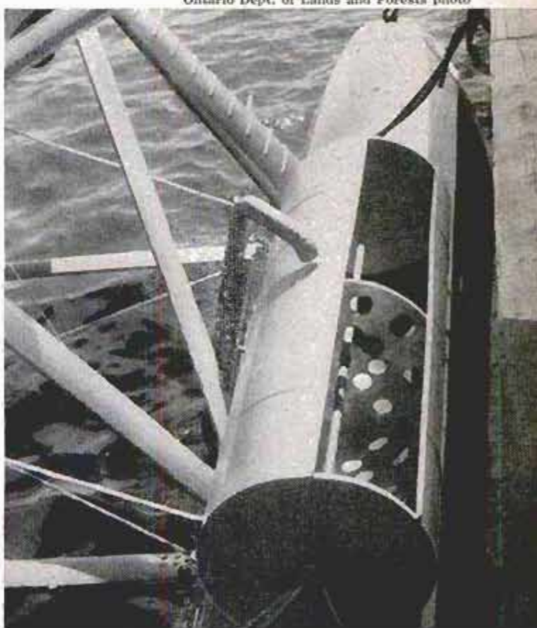
Canadian Otter aircraft sprays water from pontoon tanks, above, during test at Sault Ste. Marie. Refill pipes force water into tanks as plane taxis
