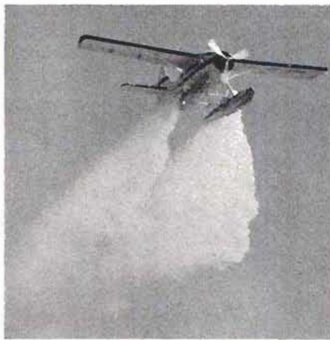
Canadian Otter aircraft sprays water from pontoon tanks, above, during test at Sault Ste. Marie. Refill pipes force water into tanks as plane taxis
