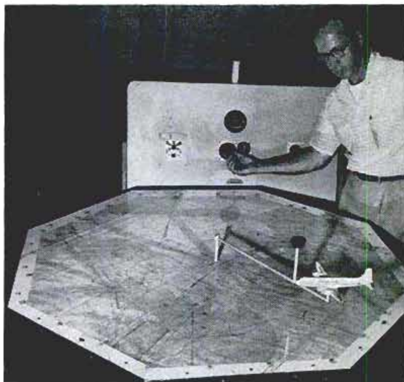
Model of aircraft on the swinging arm demonstrates the VOR (very high frequency omnirange) radio-navigation system
