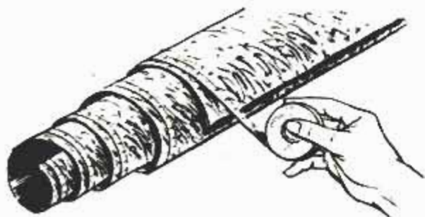
UNROLLING A PIECE OF LINOLEUM to measure it is unnecessary if it is pulled out to spiral one end as above. This exposes the turns of rolled linoleum so that a tape can be used for measuring it
