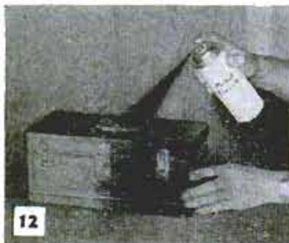
Figs. 12 and 13, flat surfaces are painted by starting at near end, allowing overspray to drift forward on work not yet coated. Fig. 14, cold paint is warmed by placing can in a pan of 90 to 100-deg. water
