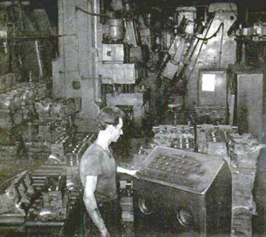
Russian factories have fine equipment. This is an automatic transfer line for machining cylinder blocks at Moskvitch plant
