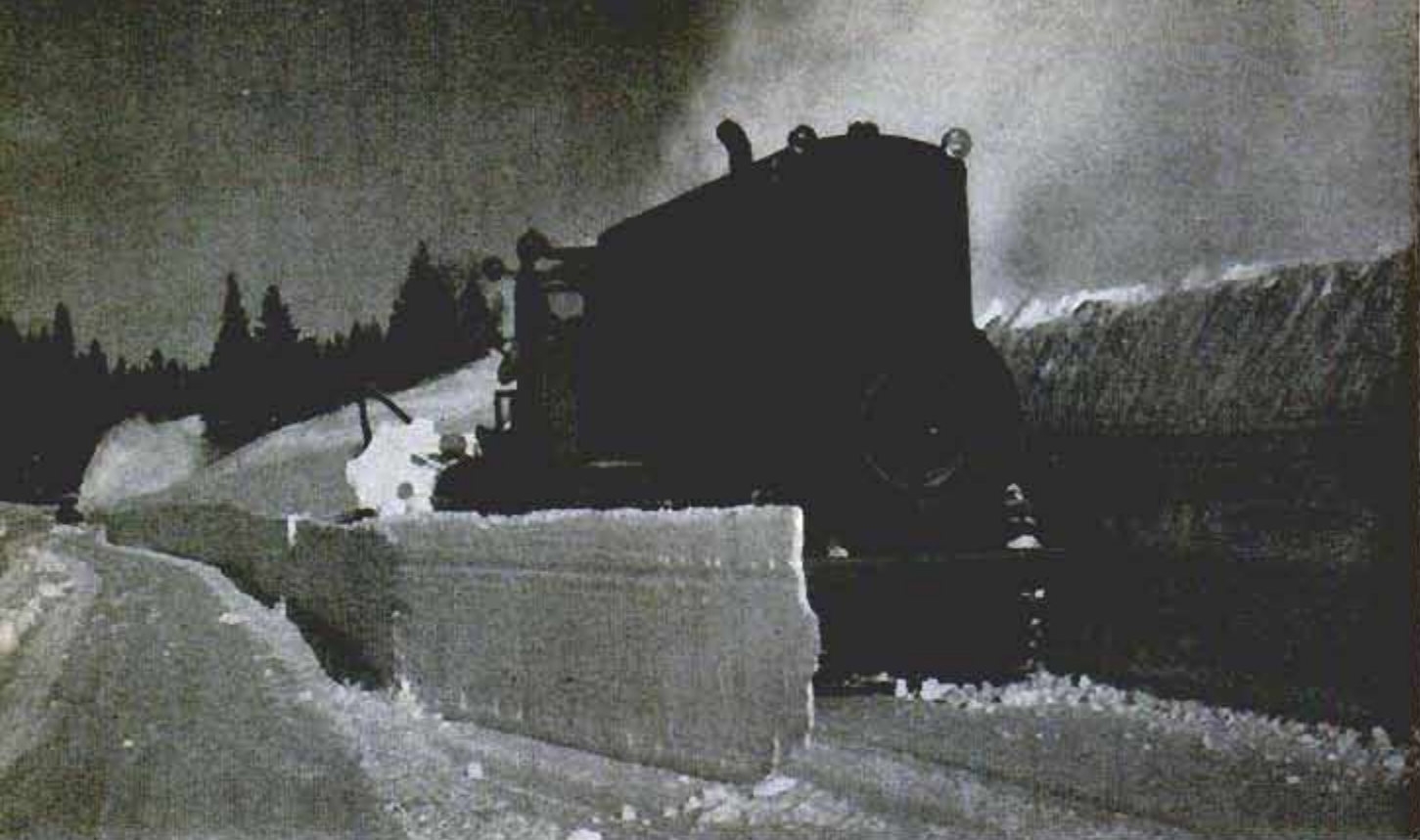
Rotary plows working in parallel paths to open highway after a storm produce strange wafers of packed snow
