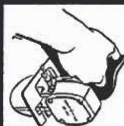
Plunge cuts without drilled hole
