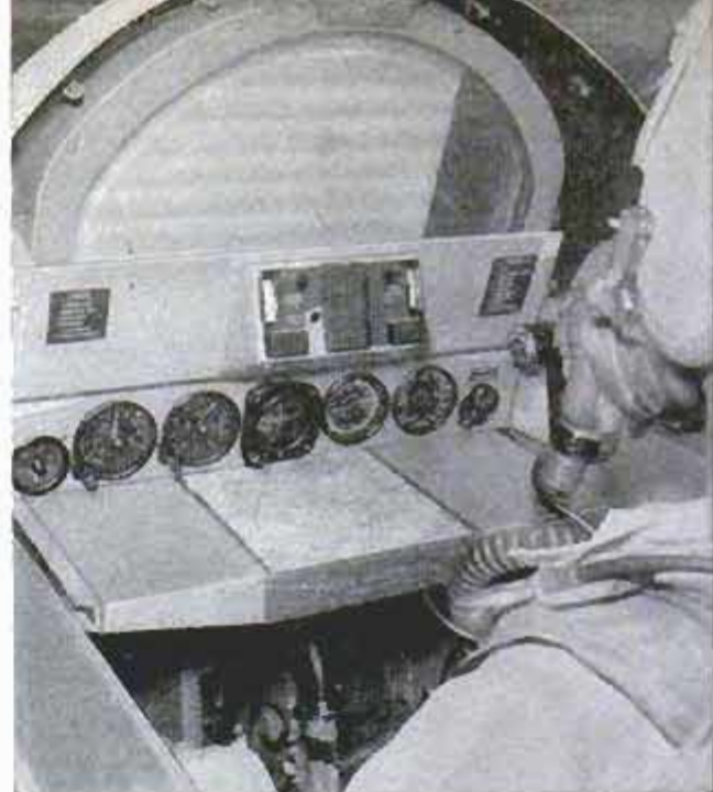
Used in airplane cockpit, picture of area in which pilot is flying appears on TV tube in front of him
