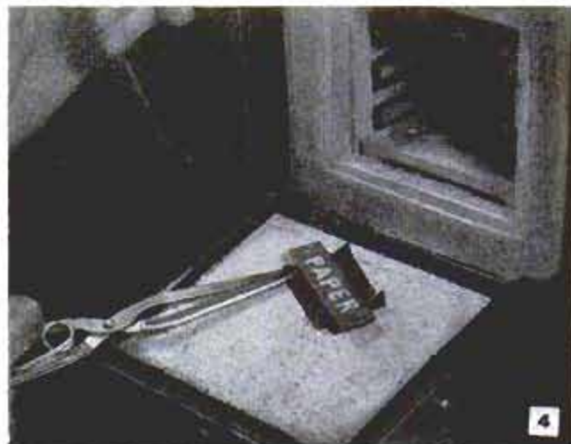
Finally, firing hardens last coat of enamel of contrasting color and attractive sign is ready for use
