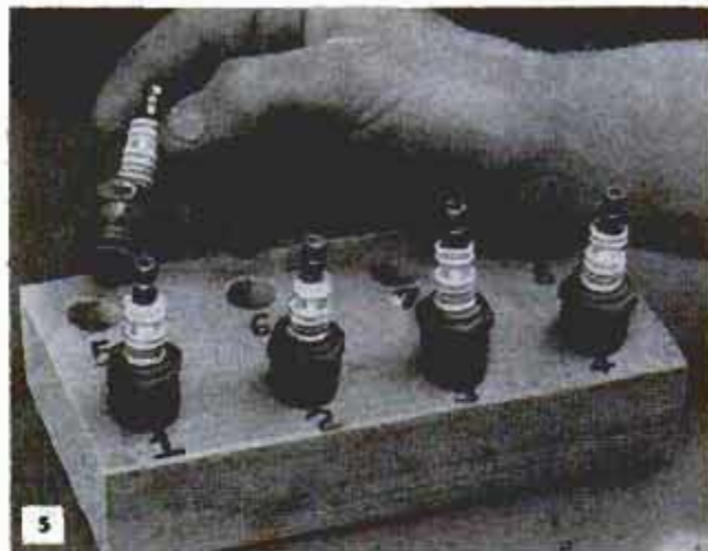
5 To check on condition of each cylinder, fit plugs into drilled block, numbered to match engine cylinders
