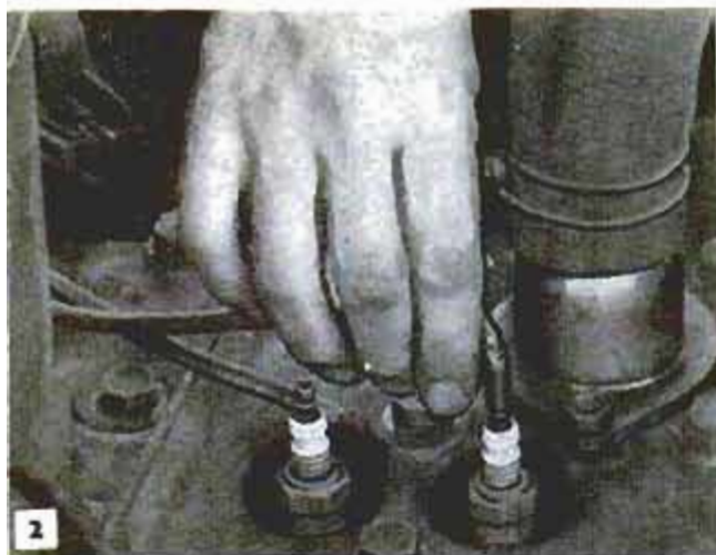
2 When removing wires from spark plugs, grasp connectors to prevent loosening connectors from wires
