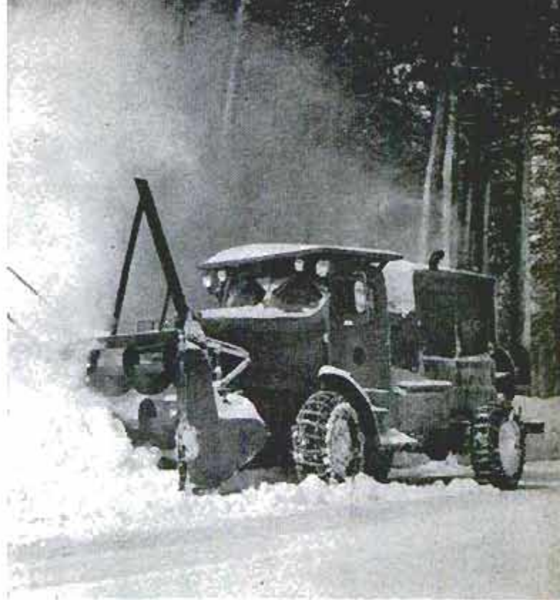
Driver of a rotary snowplow patiently guides his machine at two miles per hour through roadside drifts
