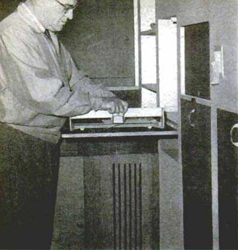
Paper cutter is located in recessed cabinet at right end of sink. Ferrotypes storage racks are below sink
