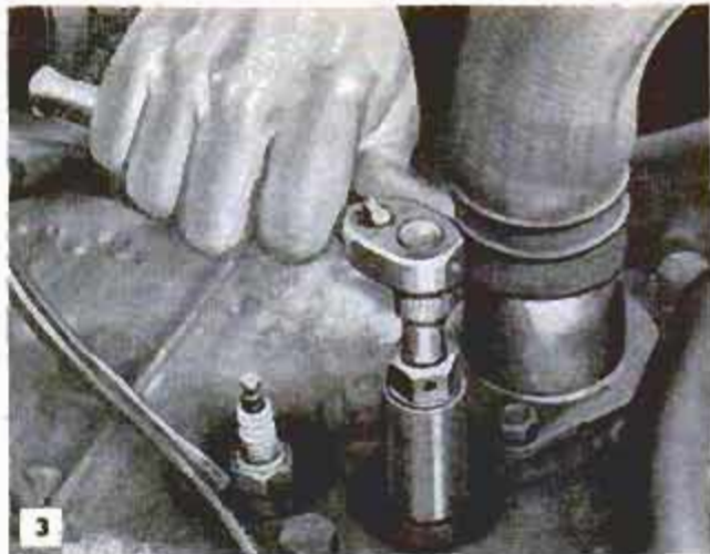
3 Use proper spark-plug wrench to avoid damaging plug removed, as well as porcelains of adjacent plugs
