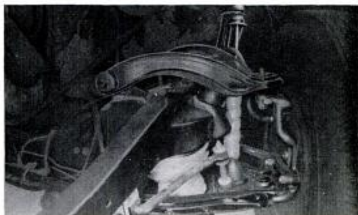
Above, front suspension arms are stampings. The center white area is air-suspension unit. Below, optional bucket seats
