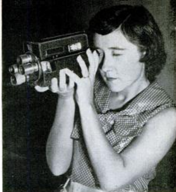
Camera has projector, wide-angle, telephoto, standard lenses. View finder shows field for each lens
