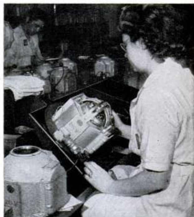
This is the first electronic automatic pilot designed for American precision bombers in World War II
