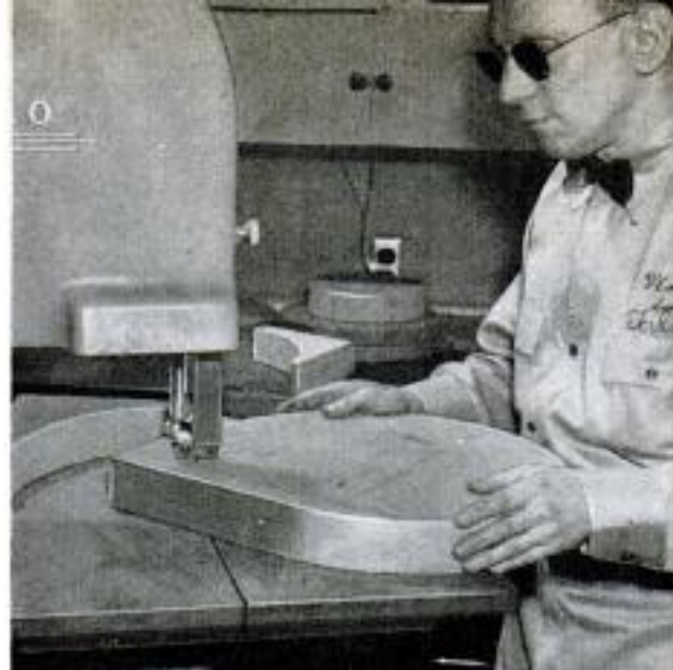
Turning the workpiece on the jig's pivot point, he saws out the disk, then prepares it for the lathe
