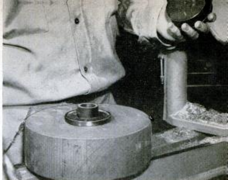
Using a marking disk he made himself, he marks holes on bottom surface to register with holes on faceplate
