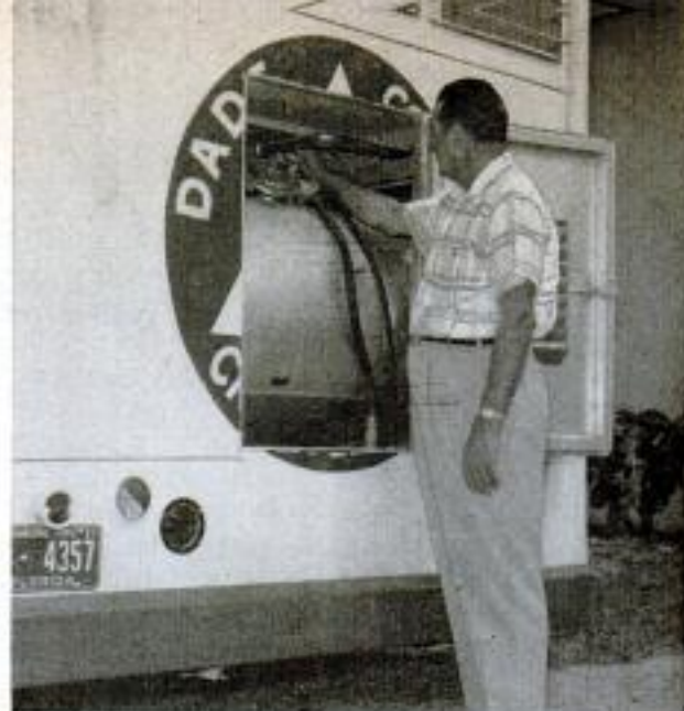
Unit carries 280 gallons of LP gas, enough to operate bus, kitchen equipment and lights for 36 hours
