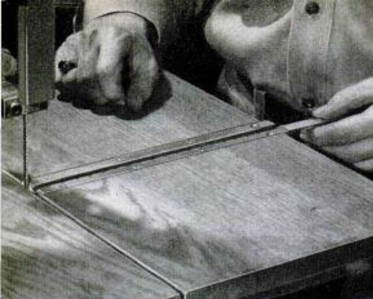
Special circle-cutting jig has a sliding scale which permits him to set the desired diameter by touch
