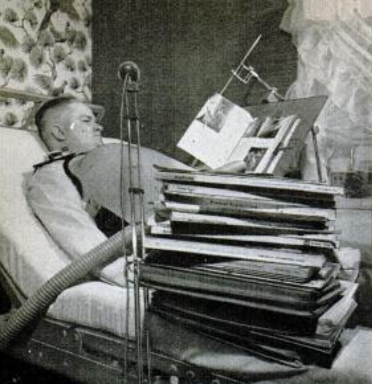
Scientists devised automatic page turner to help polio-paralyzed engineer condense scientific reports
