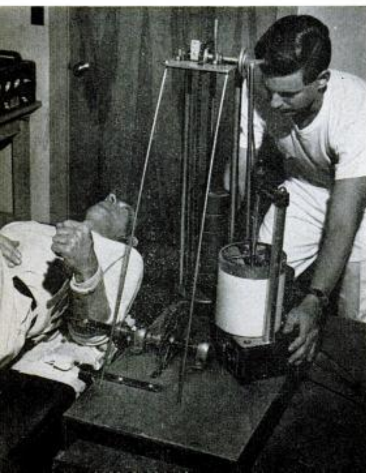
Ergograph machine measures muscle fatigue. Such tests tell something's physically wrong, but not what. Doctor Clarke's case studies diagnose these causes
