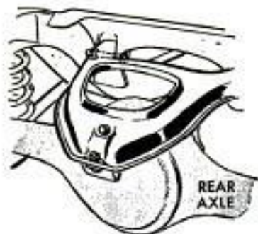
Atop Pontiac's rear axle is a U-shaped yoke to stop windup
