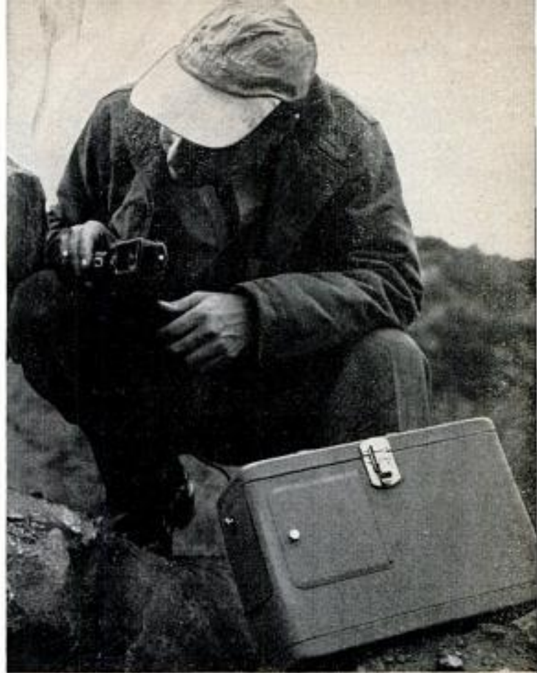
Prospector uses ultraviolet lamp to study characteristics of radioactive ore located by geiger counter
