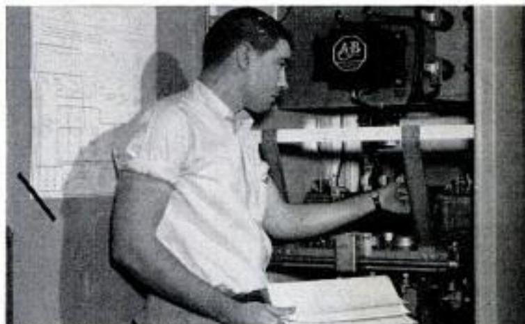
Allen-Bradley Co. Electronic Technician employs his skill to assemble complicated equipment, make tests and inspections of finished units; here he checks assembly and operation against line diagram.
