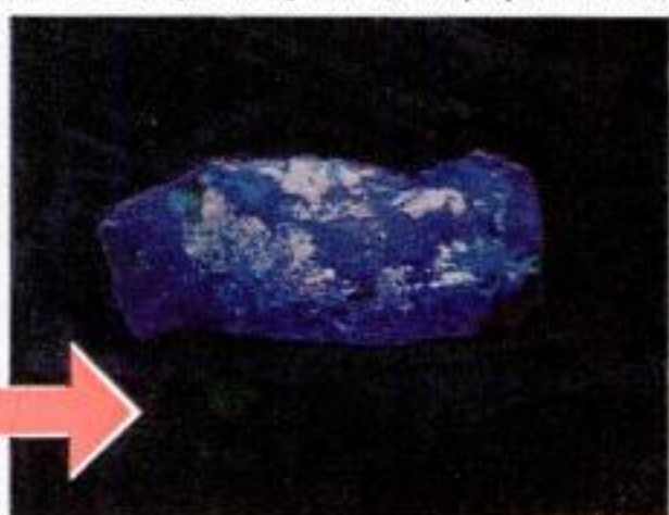
Ultraviolet reveals concentrations of uranium ore in patches of green against bluish-purple autunite
