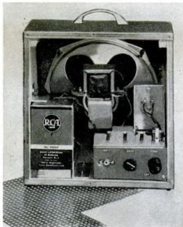
Fig. 1. Rear view of assembled system with back cover removed. Cover cut to make controls accessible
