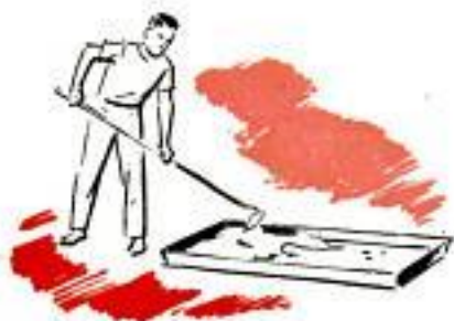
Top of chimney is reached with 18 courses above the ridge. Here fill is completed and ready to be grouted
