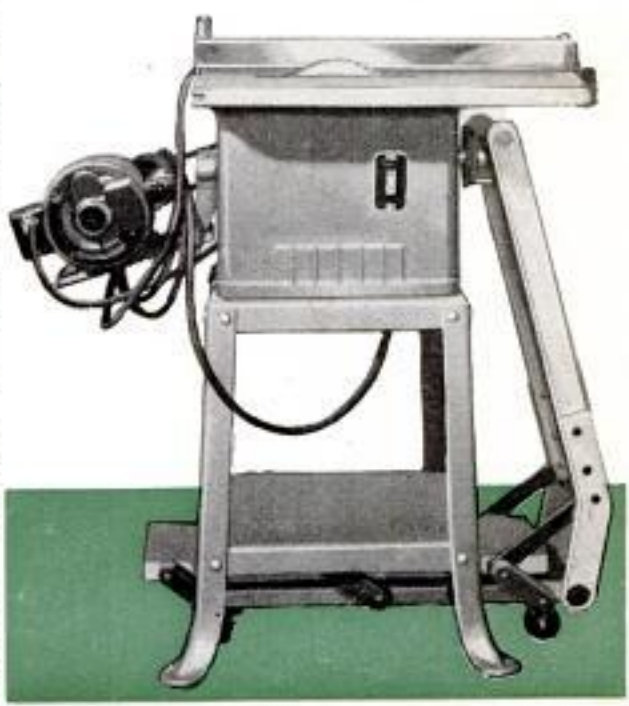
Above, just lower the handle of the dolly to raise the machine clear of the floor. Below, raising the handle lowers the platform to clear machine table
