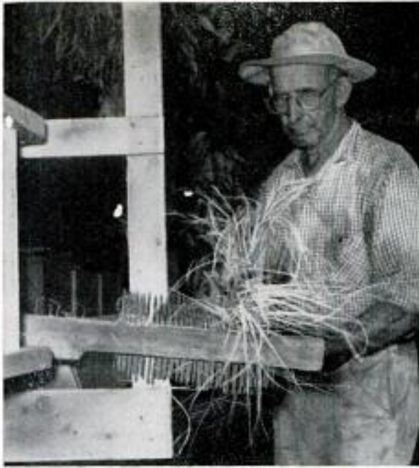
Palmetto buds are shredded on this nail-studded board. The end product may wind up in your home
