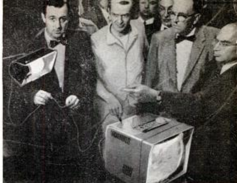
Technicians demonstrate how charged metal case of defective TV set can light a lamp. Simultaneous contact with case and grounded object could be fatal
