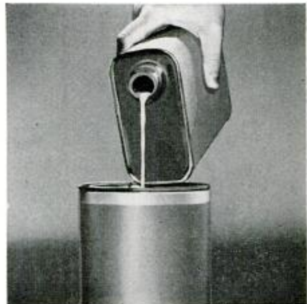
PROPER WAY TO POUR LIQUID from square or rectangular can is to have spout at top. Air enters smoothly, prevents gurgling and waste of material
