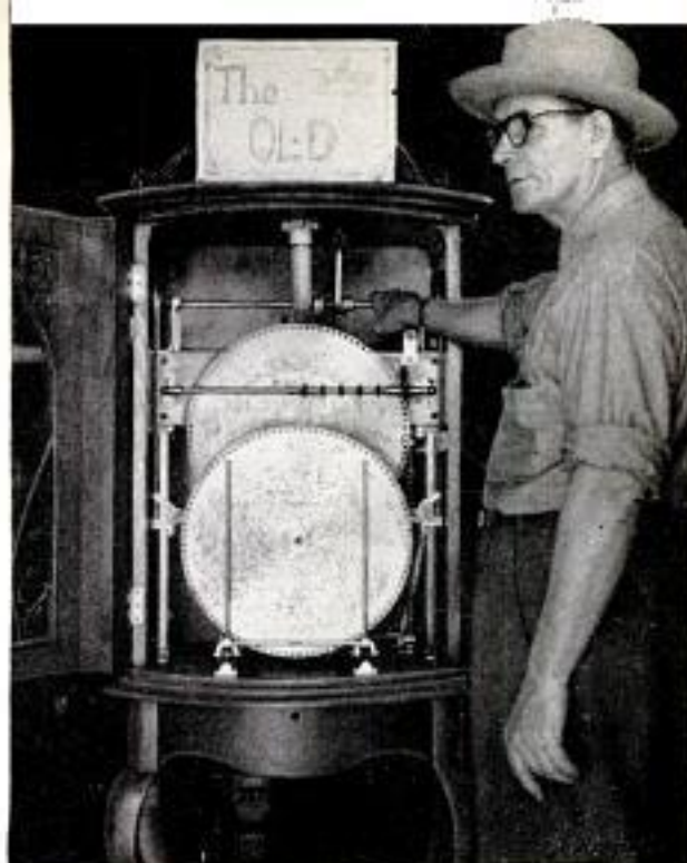
This 80-year-old forerunner of jukeboxes uses metal plates and has a selector unit similar to late models
