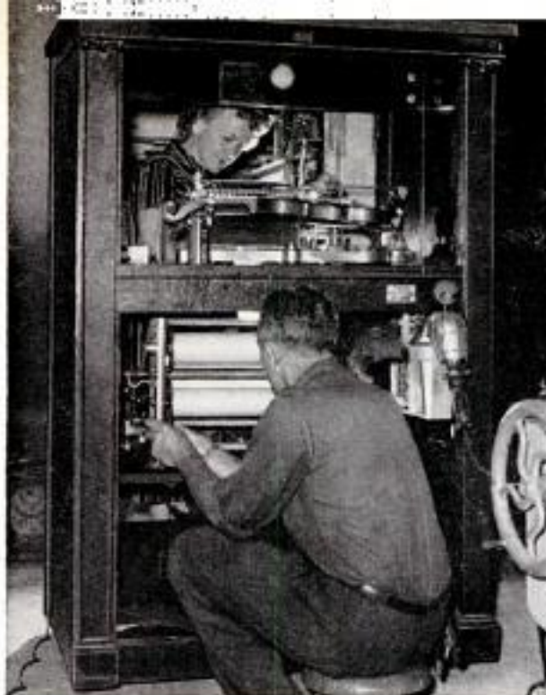
Operating from paper-roll guides, this combination violin-piano music box is being fixed for a museum
