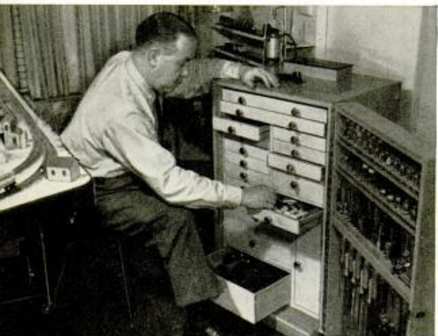
Orderly storage for parts and tools is provided in the former dental-instrument cabinet, above, which is mounted on casters
