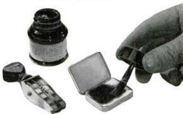
Aspirin tin becomes miniature, pocket-size stamp pad when filled with ink-saturated flannel cloth
