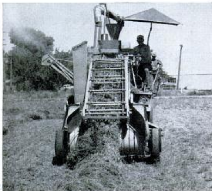
Elevator at front of rig picks up alfalfa hay from windrow, above, and feeds it into hammer mill. Pellets in truck bed, below, are inspected after they leave hopper at end of rig
