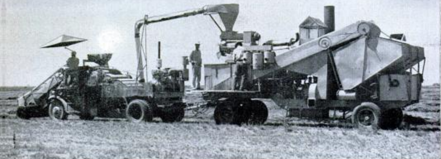
Two-section, 10-ton self-propelled hay pelletizer eats through windrow of alfalfa on a California farm
