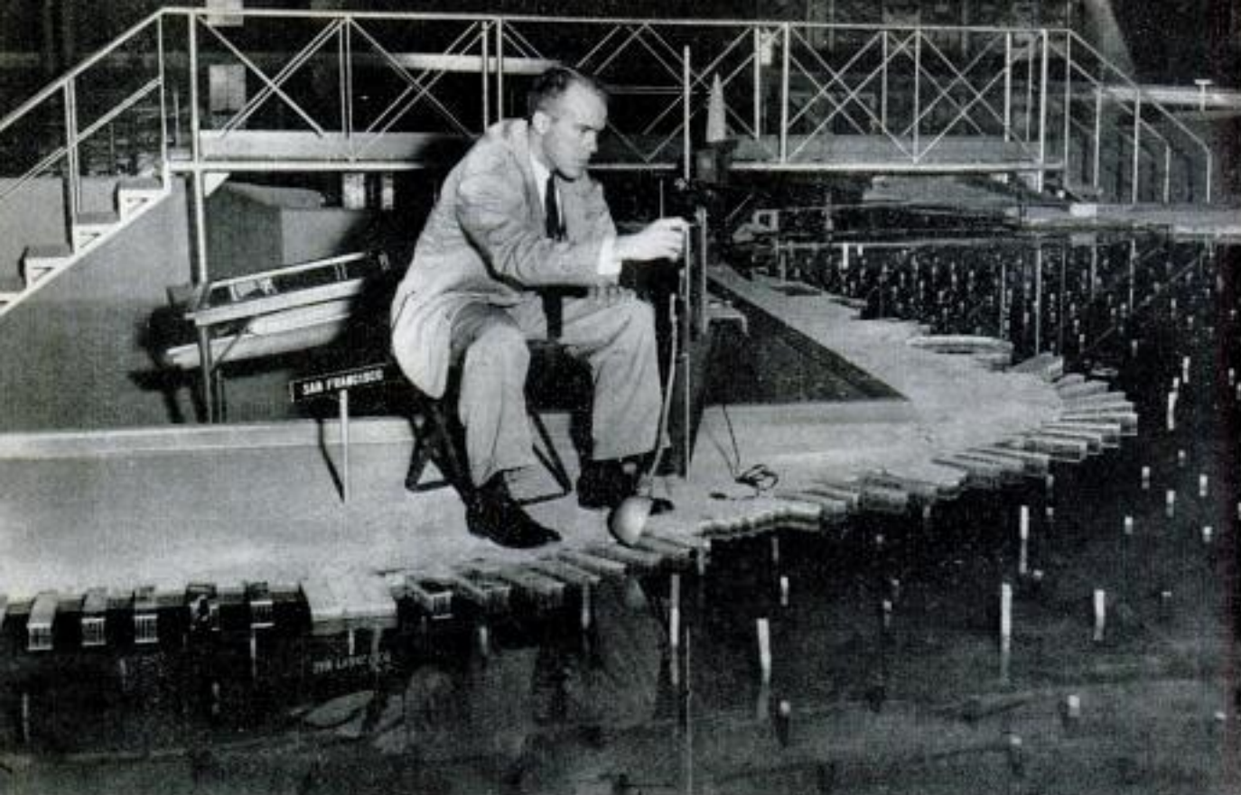
Engineer measures tidal movements. Copper strips in the water control the duplicated ebb and flow of tides
