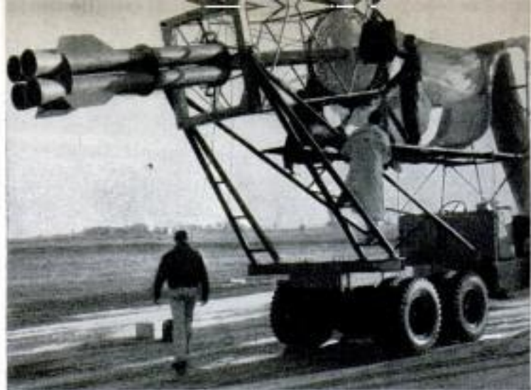
Mobile carrier holds 1900-pound rocket in its "cradle," which is attached to polyethylene balloon ready for 100,000-foot trip
