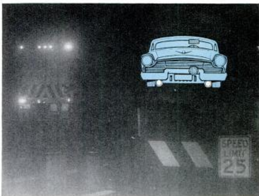
Vision improves sharply when the lights are mounted low, reducing back scatter. Diagram at bottom of page explains why
