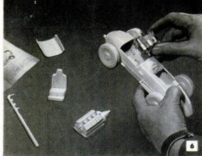
Discarding dummy engine and seat when assembling car provides room for electric motor and dry cells
