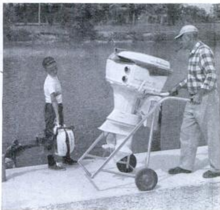
The 50-horsepower V4, biggest motor of the line, meets the smallest, a three-horsepower job. The V4 weighs about 200 pounds, has a lifting ring and a tilt-assist spring. Below, the all-new motor has sufficient power to pull six water skiers simultaneously
