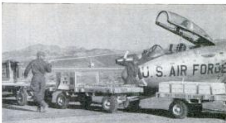
"Pig" on a pole is lead container for atomic cloud samples. Material is shipped to Atomic Energy Commission lab for study
