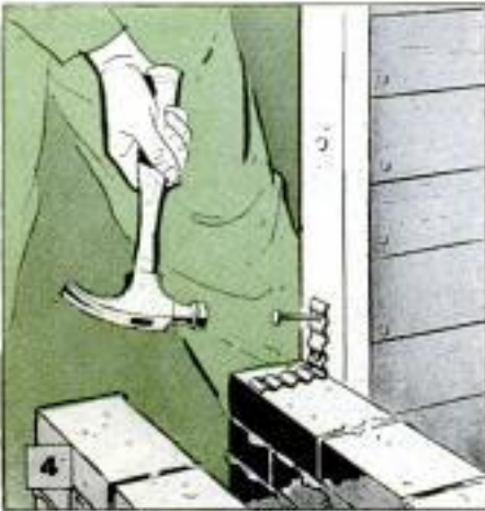
Outside wall of fireplace is anchored to framed opening with corrugated sheet-metal ties which are placed between every six or eight courses and nailed. Side-view drawing shows proper placement of common brick
