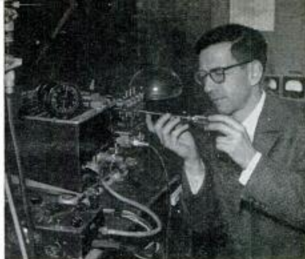
Researcher makes adjustment on electronic blander, which virtually eliminates aircraft radio static
