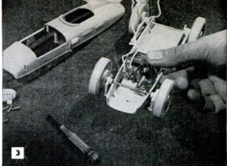
Above, after car is assembled and pinion gear is on axle, hold motor in position to check mesh of gears
