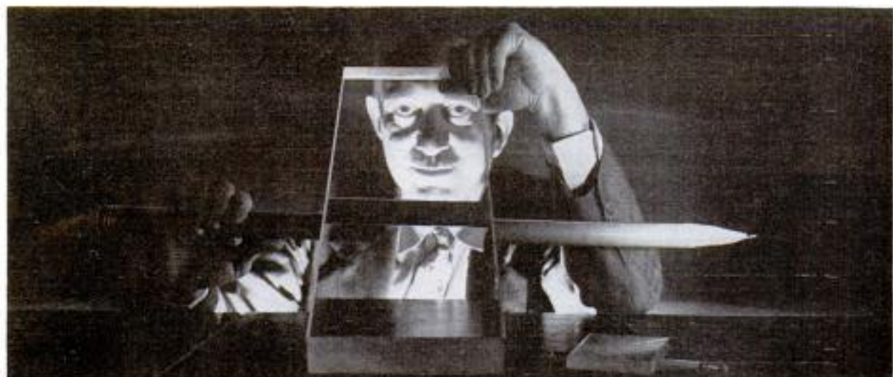
Two-foot pencil, viewed partially through slab of plastic, appears broken, demonstrating light refraction
