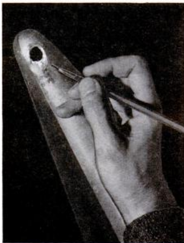
Hole about the size of a dime was drilled in this jet-trainer tail cone by bolt of natural lightning
