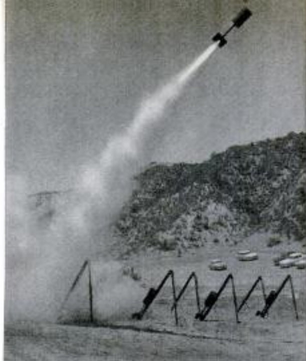
Man at left is attaching igniter wires to rocket which will propel 8½-gallon container of fire extinguisher. Above is a rocket on its way to a fire
