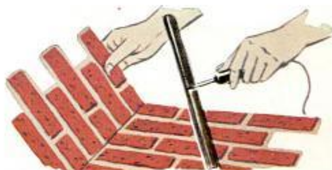
Electric corner-bending iron does neat job on inside and outside corners. Iron softens brick in seconds
