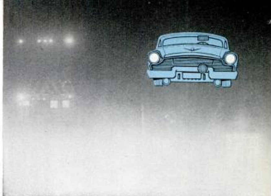
Behind standard headlights, driver faces blinding night fog that makes road invisible and the truck only faintly visible in the distance. Light scattered by fog droplets obscures view
