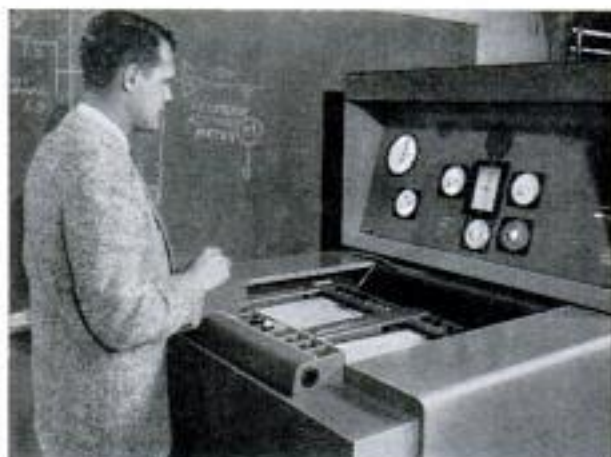
Engineer manipulates small stick at a control panel to fly the supersonic X-7 missile by remote control
