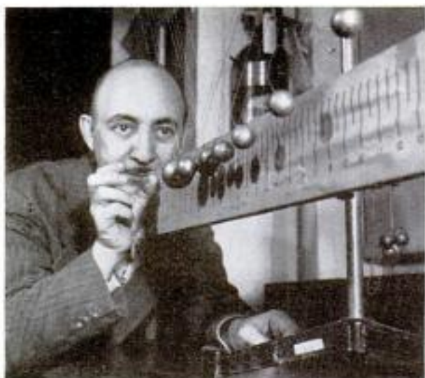
When professor releases heavy ball, first in line, its light bump sends lighter ball on other end flying
