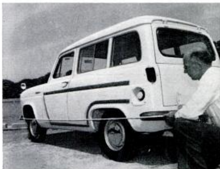
Above, about 11½ feet long, the wagon is shorter over-all than the sedan. Below, with the rear seat down, the floor is 45 inches long. Rear-door opening is 27 inches high. Rear seat in the wagon is not very comfortable for adults, say some owners
