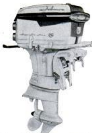
From shroud to propeller, V4 has sleek but powerful lines. Shroud is airtight except for one baffled air-intake port. Left, parts are easily accessible when shroud is removed
