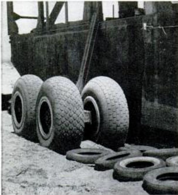
Tractors haul 400-ton dredge across the desert on B-17 wheels. Auto tires pave the way over soft sand
