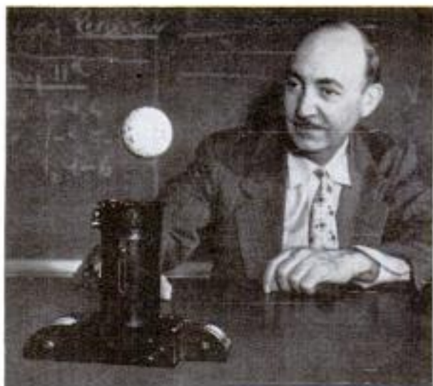
Ball fired straight up from a moving cannon moves forward with the cannon, drops back into muzzle
