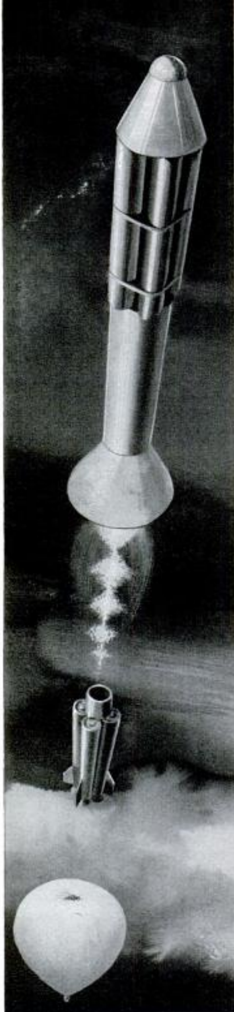
Mobile carrier holds 1900-pound rocket in its "cradle," which is attached to polyethylene balloon ready for 100,000-foot trip
