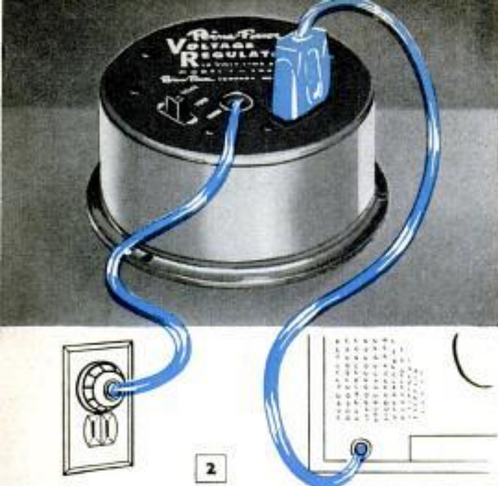
Appearance and installation of a typical voltage regulator transformer. Three-position switch may be adjusted for high, low or normal line voltage
