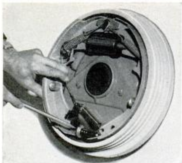
Cable (under fingers) pulls lever which turns cogwheel (end of pencil) to adjust brake automatically
