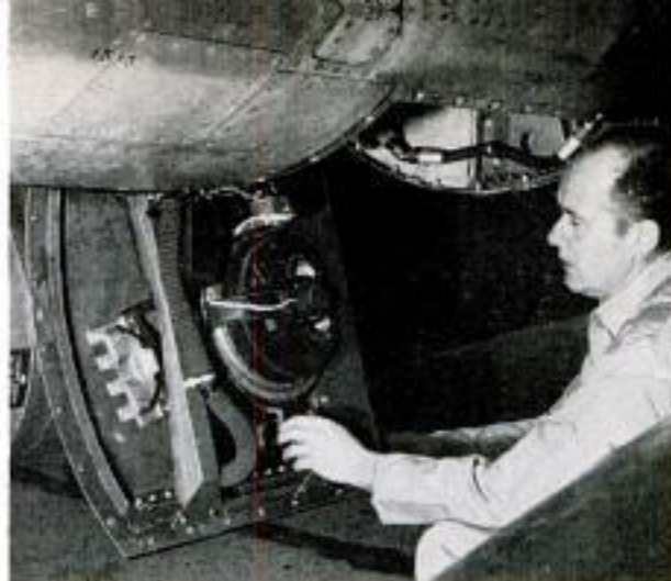
Rotating antennas, tucked in the belly of a jet fighter, throw out twin beams ahead of the craft
