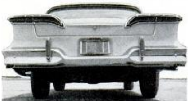
Manhole view of Edsel's stern emphasizes horizontal taillights. Half of each extends into the trunk lid
