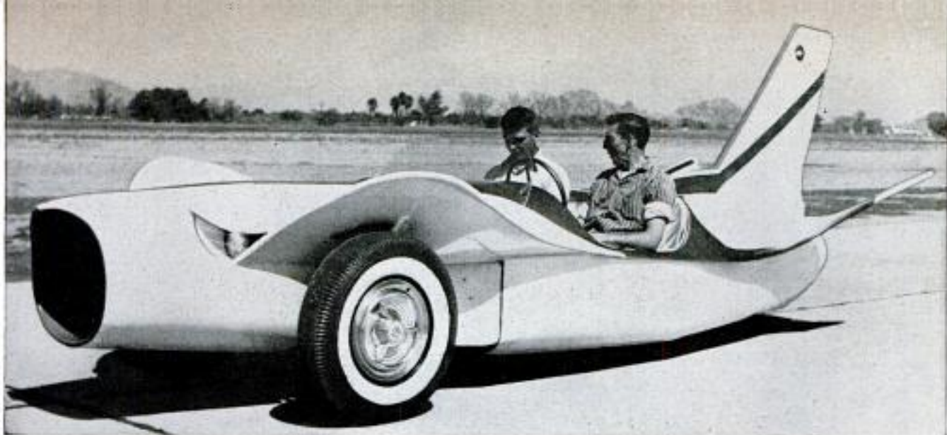
Three-wheel Sabre Jet car was built of aluminum from an old British auto, can travel 80 miles per hour
