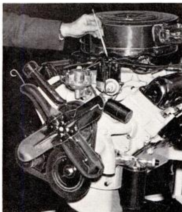
Distributor (pencil points to it) is mounted forward on the engine, designed for service accessibility
