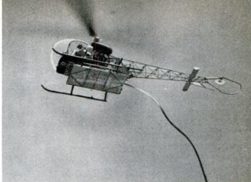
Helicopter, above, is used in Forest Service experiments to lay as much as 1500 feet of linen hose across rough country
