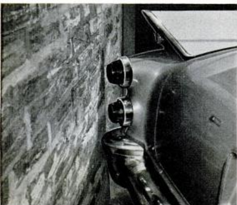
Dodge taillights extend almost as far back as bumper, making them extremely vulnerable to damage
