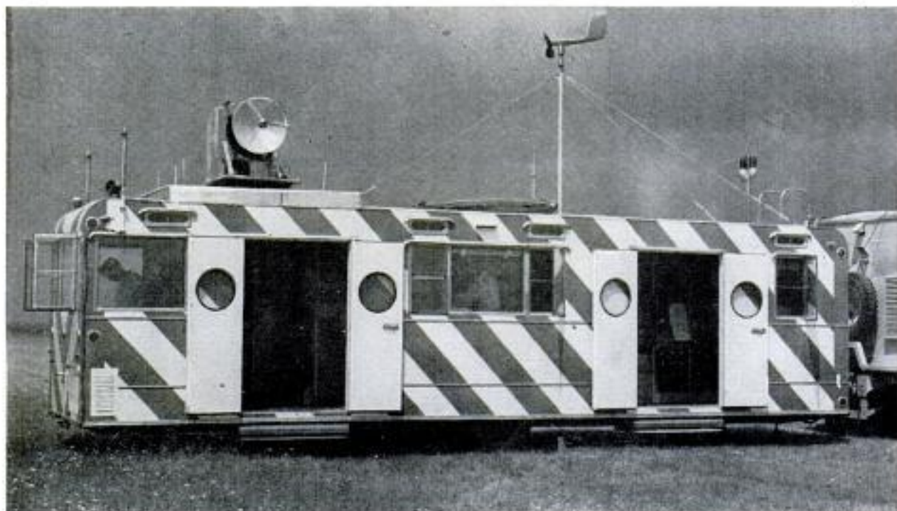
Equipment for ACLS is mounted in a trailer for tests. Computer sends out orders as radar locates the plane
