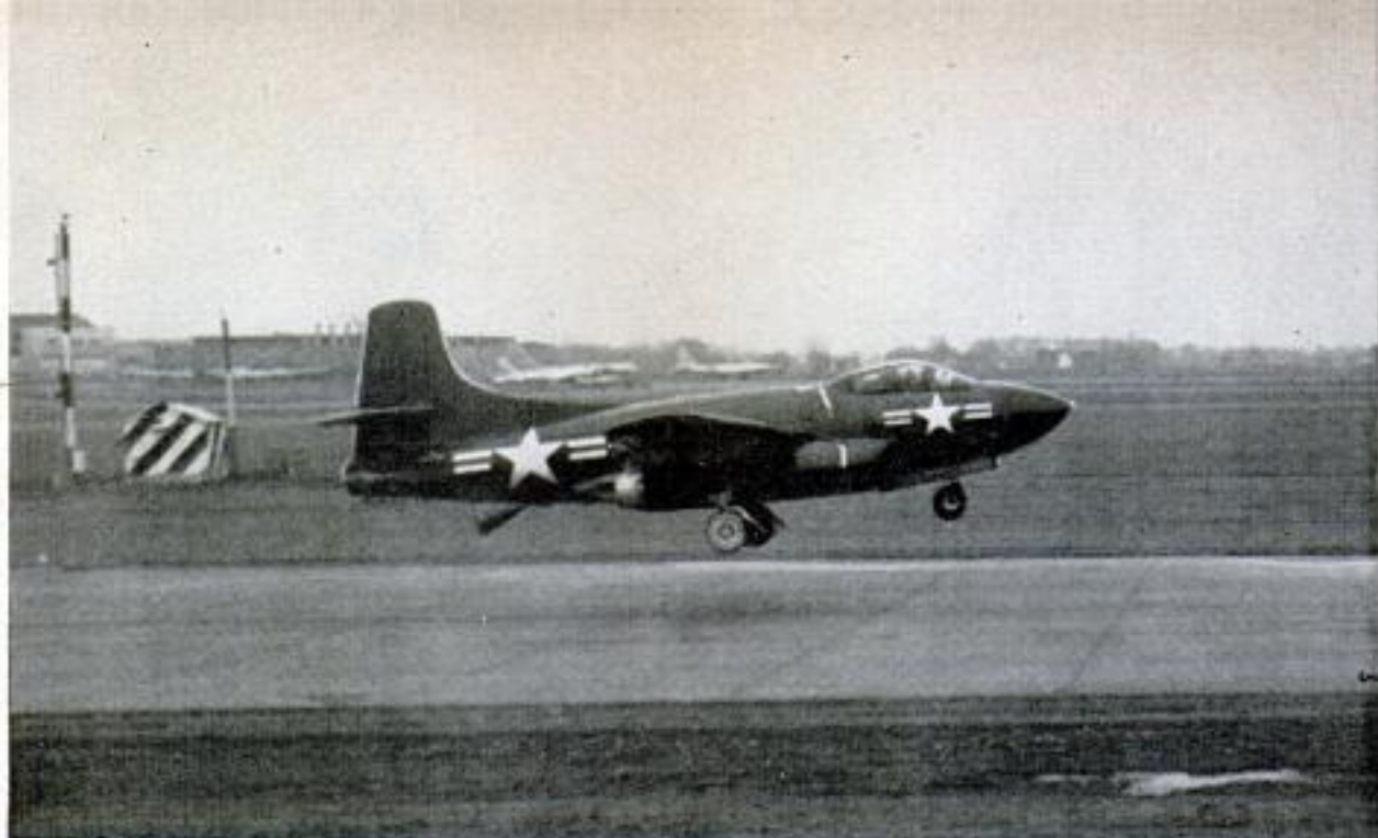
With radar beams bouncing off the landing gear, Navy fighter makes perfect landing without pilot's help
