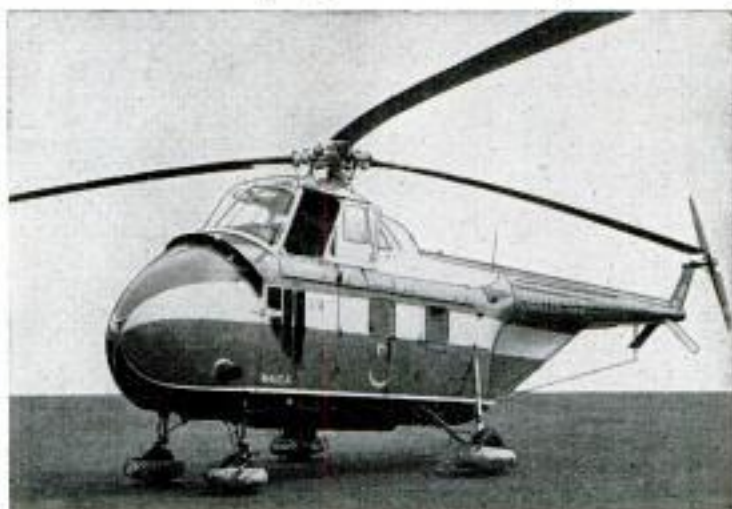
Above, diagram indicates storage chamber with 3000 pounds per square inch of compressed air and pneumatic lines to floats around wheels. Below, copter uses floats in ground landing
