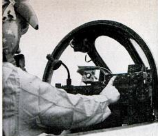
RADAN , a smaller version of "66," has a switch panel and dial indicating drift angle and ground speed
