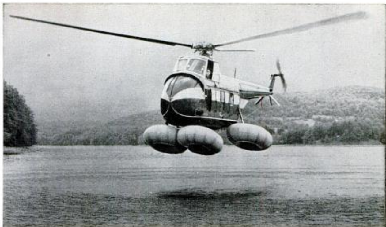
Sikorsky S-55 helicopter makes simulated emergency landing on water with inflated, rubberized "doughnuts"
