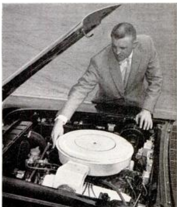
Front-hinged hood is a safety factor, but it does limit accessibility of forward-mounted distributor
