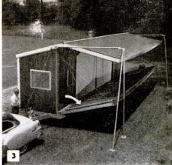
3 Two people are needed to operate the winches at the front and rear of the trailer. Here, the floor and outside wall are being lowered after raising the roof
