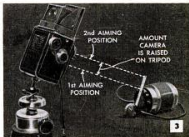
Above, camera is focused on object 200 ft distant and dot made in center of viewer, C, to coincide with prominent point in image. Below, steel tape propped against subject provides target at which to aim camera in registering lens-to-lens measurement with mark C and finding amount camera must be raised
