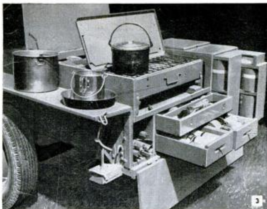
Fig. 2, gasoline lantern is carried in plywood box and has plywood cutout fitted over top of lantern to protect it from damage when traveling. Fig. 3, hinged sideboards are handy work and serving tables
