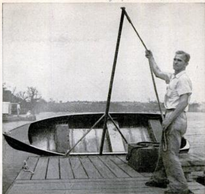
Hoist shown in photos is designed for 14-ft. boat but all members of hoist can be made longer to accommodate larger boats
