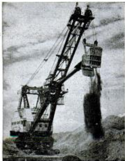
Two men are dwarfed by the River Queen's mammoth dipper, which can dig 100,000 tons of earth in 24 hours
