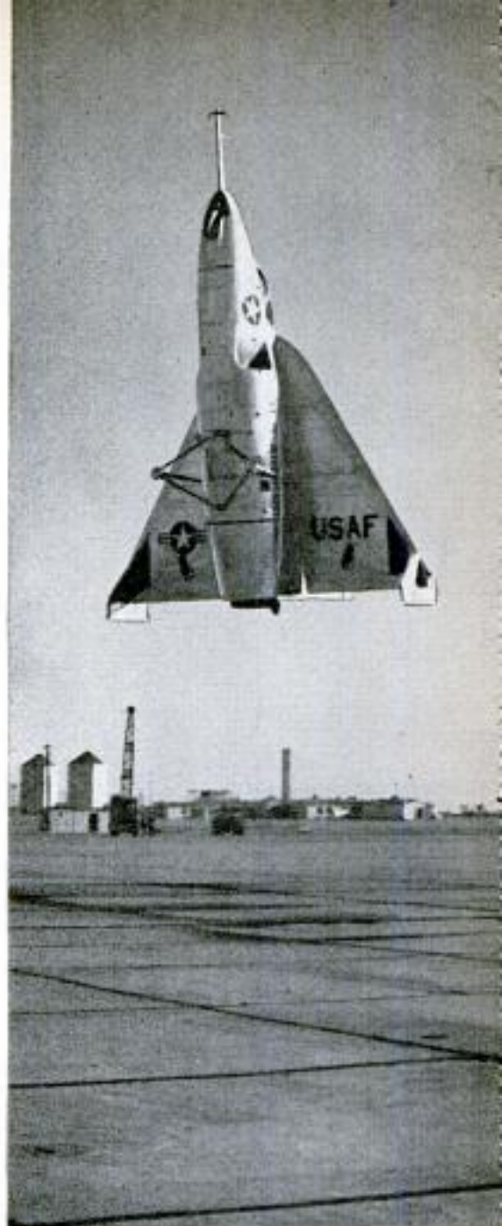
Vertijet can remain motionless few feet above ground. Rolls-Royce Avon jet engine develops 10,000-lb. thrust
