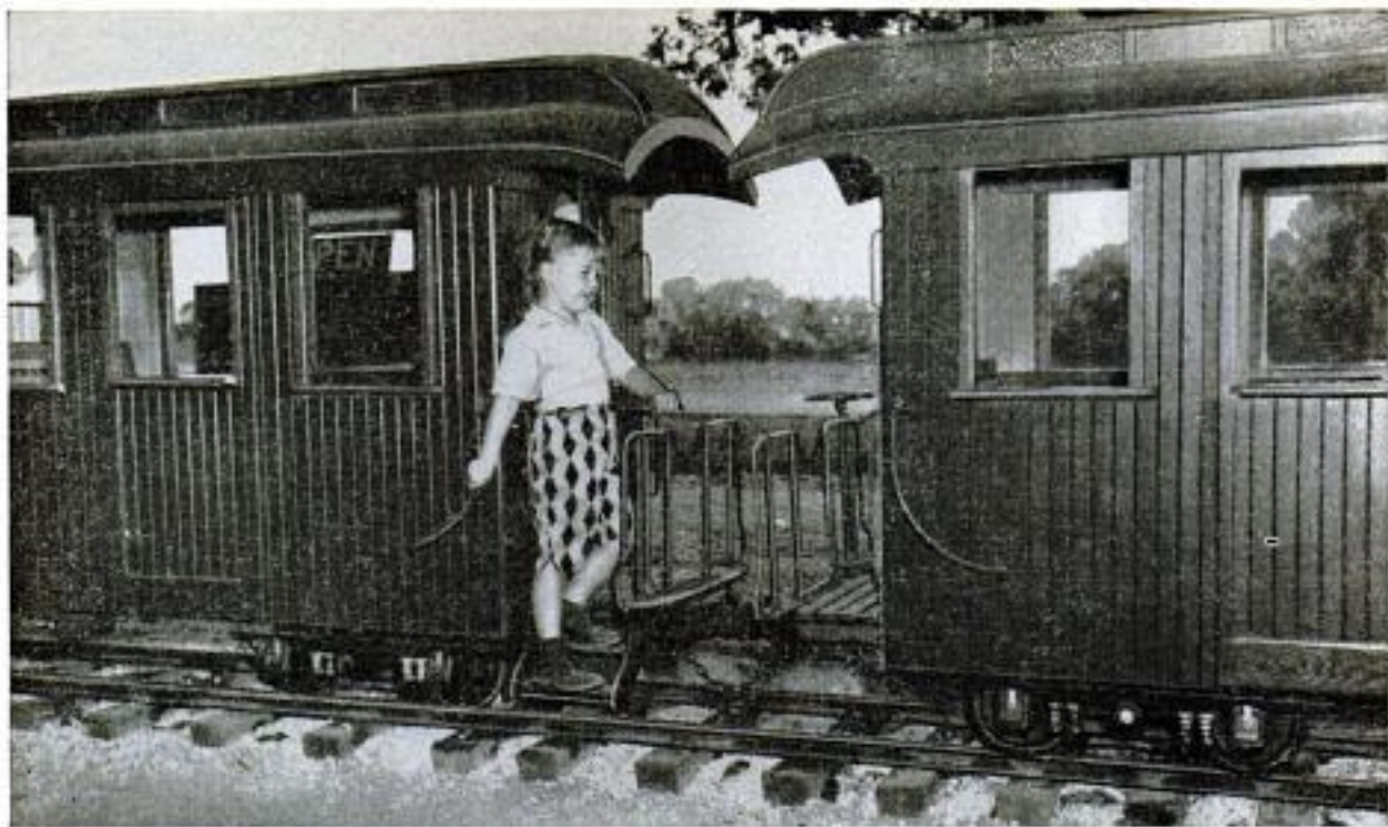
H. T. & W.'s ornate eight-passenger cars are one quarter actual size, have authentic link-and-pin couplers
