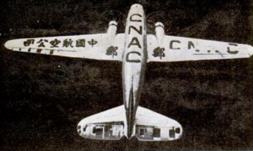
DC-2½, a Chinese "gooney bird" with its right wing blasted off, flew back to its base using a 10-foot shorter DC-2 wing
