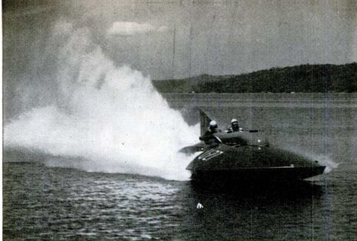
Fabulous Slo-Mo-Shun IV had big air fin to help boat track straight at high speed. Ted Jones is at wheel
