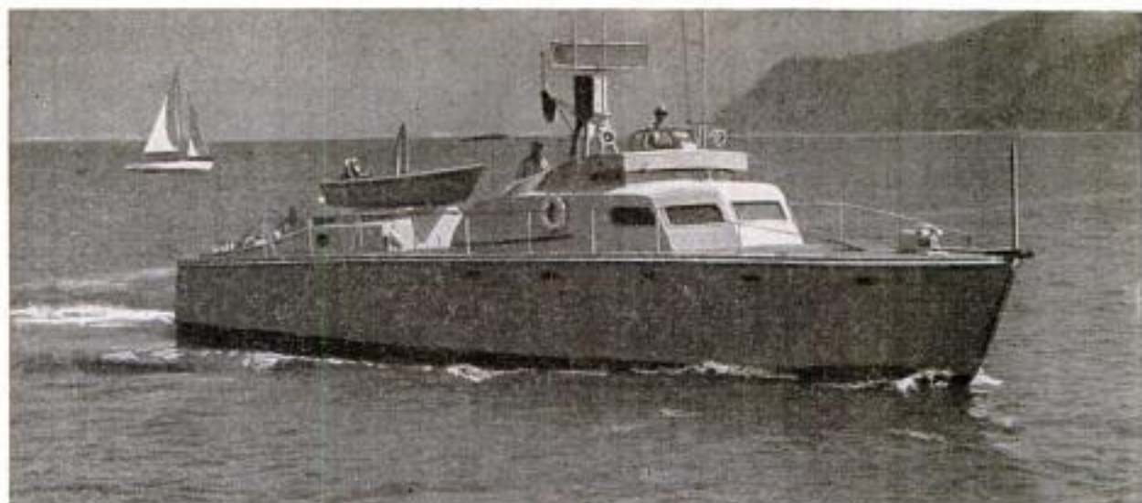
At almost 40 miles per hour the 63-foot Marlin outruns most craft in its area. This boat carries crew of four
