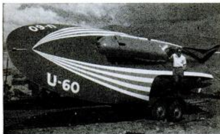
Above, Miss Thriftway, 1956 Gold Cup winner, carried driver in "conventional" place aft of the engine. Below, Thriftway, Too showing driver in the cockpit at forward end of the boat
