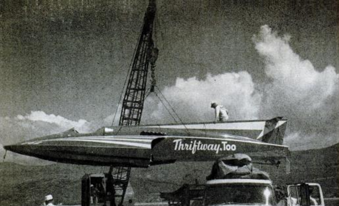
Side view of Thriftway, Too being hoisted from trailer. Exhaust ports of left engine bank are aft of intake
