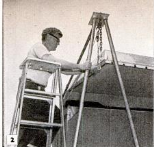
2 Steel bipods at corners help support the roof and 35-foot wall section while trailer is being folded or unfolded. Bipods are furnished with the trailer
