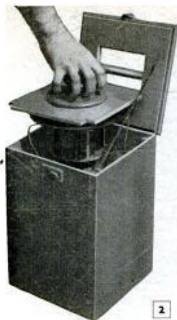
Fig. 2, gasoline lantern is carried in plywood box and has plywood cutout fitted over top of lantern to protect it from damage when traveling. Fig. 3, hinged sideboards are handy work and serving tables
