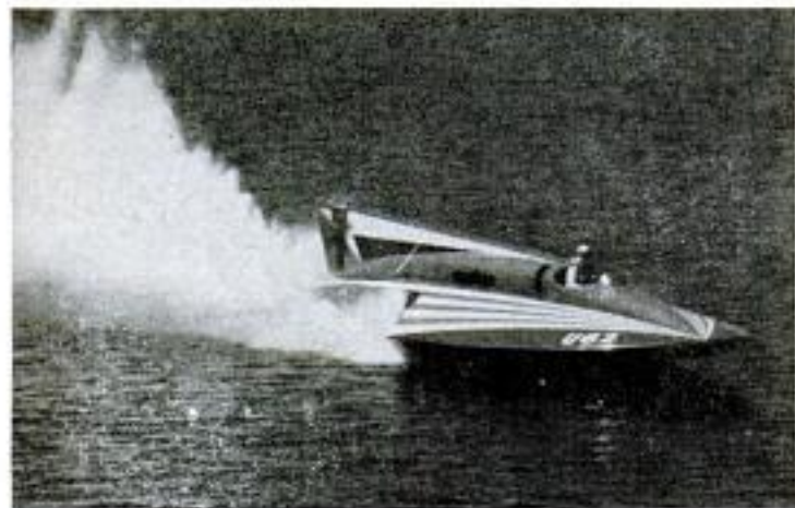
Above, Miss Thriftway, 1956 Gold Cup winner, carried driver in "conventional" place aft of the engine. Below, Thriftway, Too showing driver in the cockpit at forward end of the boat
