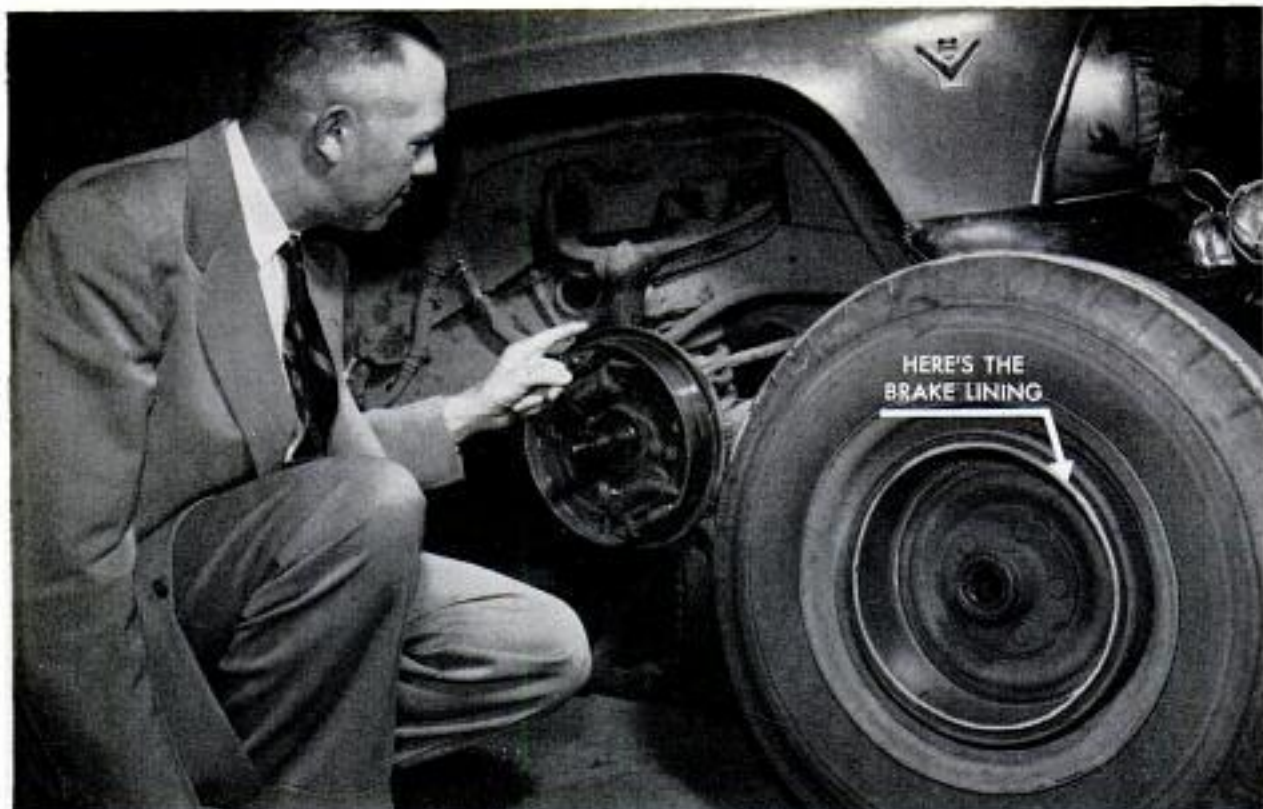
Each shoe has a shiny copper lining fused to it. Frictional lining is bonded to the inside of the drum
