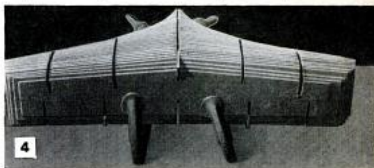
Above, bottom view of partly assembled hull shows bow, stern block, side walls and top deck in place
