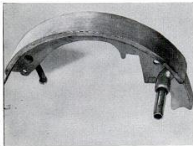
Arrows show flow of cooling water through the shoes. Below, pipe at right extends through backing plate
