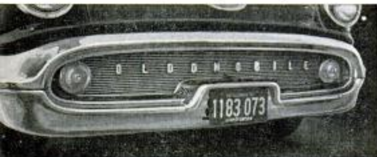
Rare indeed is this example of poor assembly, but it did occur on the test car: incorrectly spelled name
