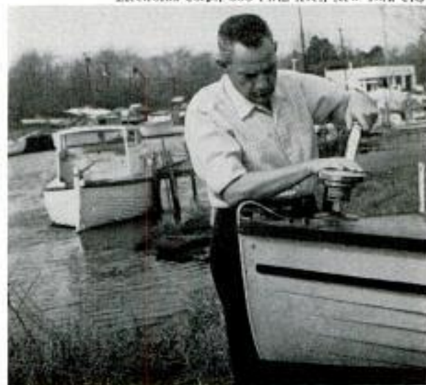
Air from vacuum cleaner operates \frac{1}{8} -inch drill on standard drill chuck (above), sands boat bow (below) Electrolux Corp., 500 Fifth Ave., New York City
