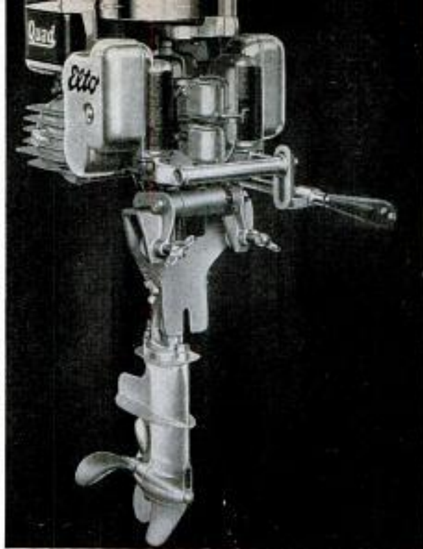
By 1929 outboard motors had come into their own. This four-cylinder Super Elto had 25 horsepower
