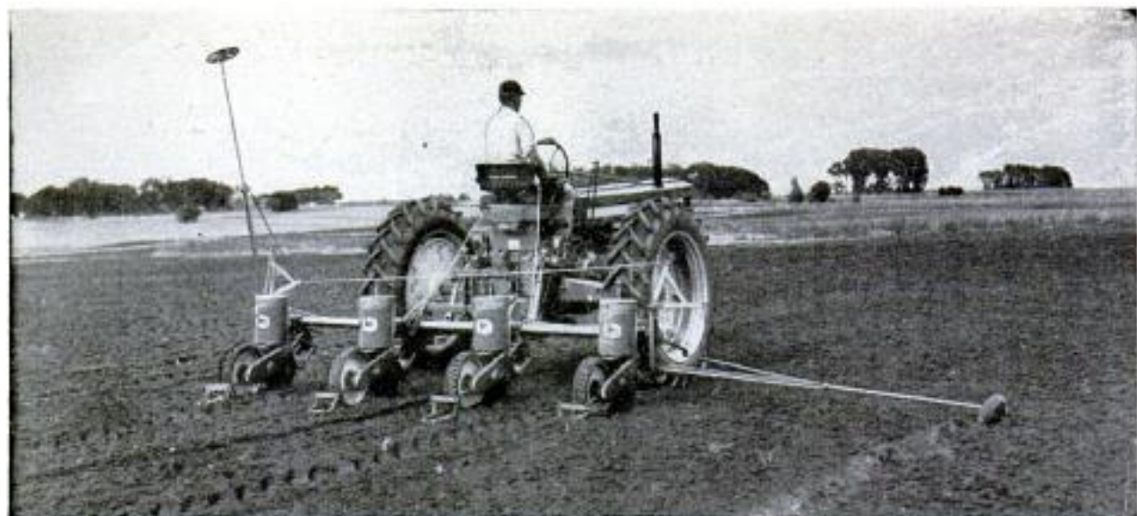
Self-driven drills can be clamped on any square tool bar, permitting flexibility in the spacing of crop rows
