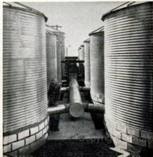
A 32-inch fan distributes dry air to six grain bins on Vinson Vanderford ranch at Yuba City, Calif.
