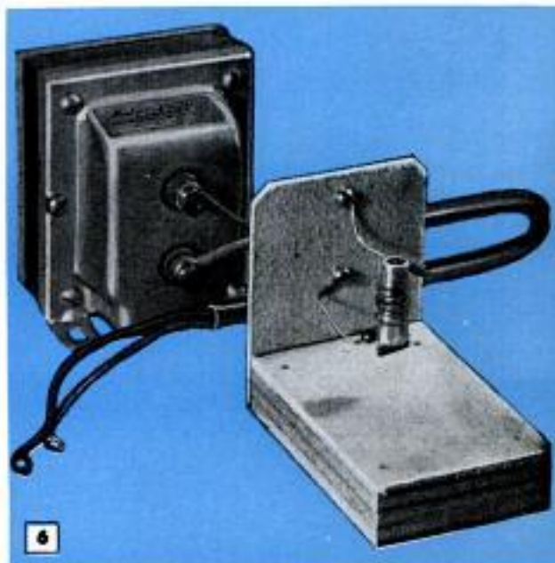
6 Above, crucible without hardware-cloth guard and asbestos top. Below, solder being melted in unit
