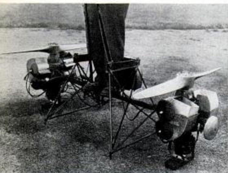
Close-up of first flying platform, above, shows it was something like two small helicopters. Putting duct around blades proved to be much more efficient
