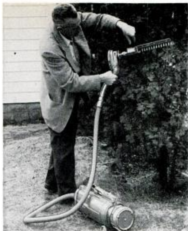
Hedge-trimmer attachment operates smoothly with power supplied by vacuum cleaner via rotating unit
