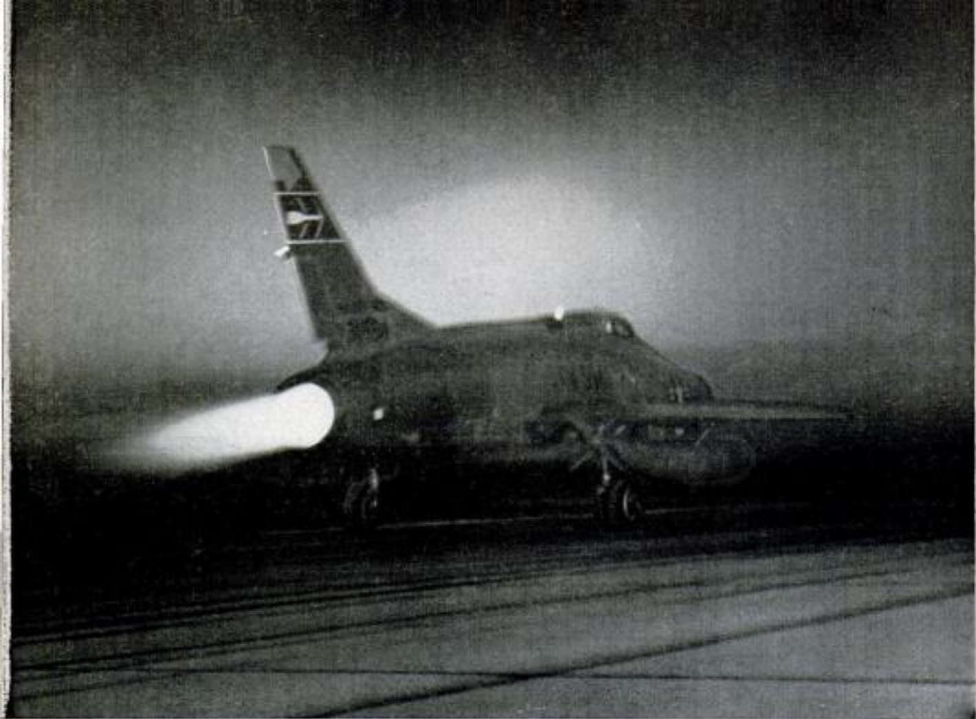
F-100 Super Sabre afterburner generates big exhaust flame on take-off. Chemical fuels will give more power
