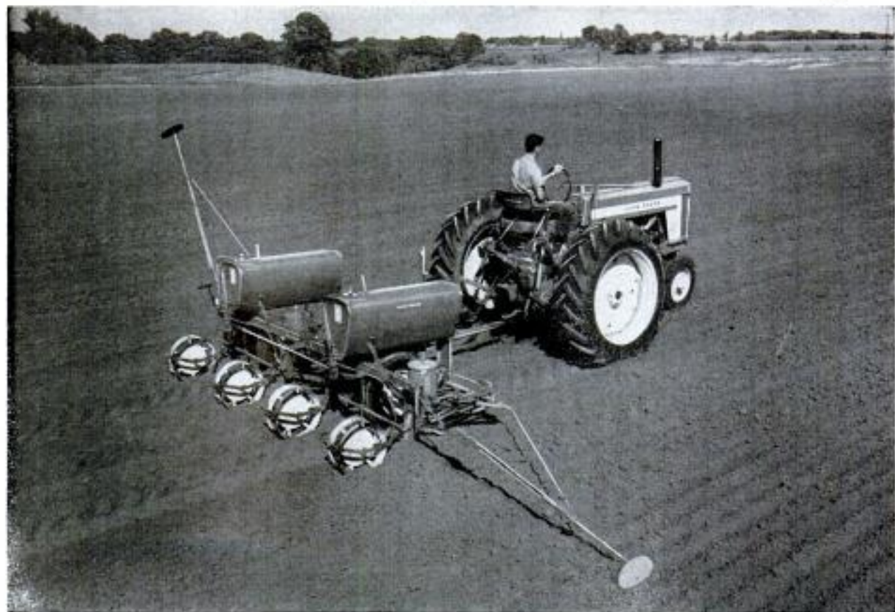
Twin-tank attachment is mounted on a corn planter, converting it into a liquid-fertilizer applicator
