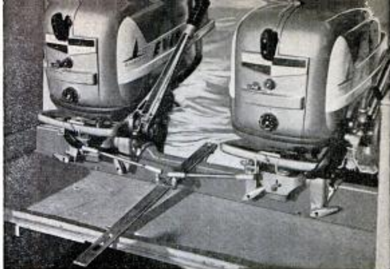
Steering clamps of type shown permit secure attachment of tie-rod assembly to steering bars of motors and quick disconnecting when motors are removed
