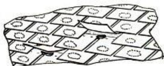
DABS OF QUICK-SETTING ASPHALT CEMENT (1" MIN. DIA.) TO HOLD COMPOSITION SHINGLES
