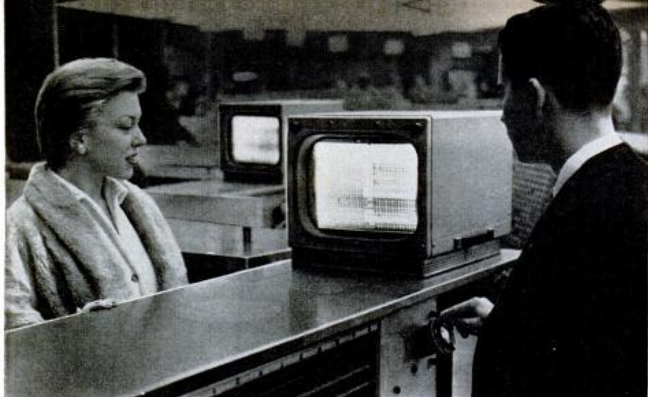
Closed-circuit television shows traveler Pullman space available when clerk dials train's code number
