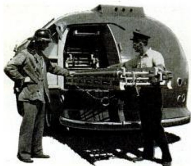
Members of Bend, Ore., fire department used their spare time to convert a bus into this fire truck
