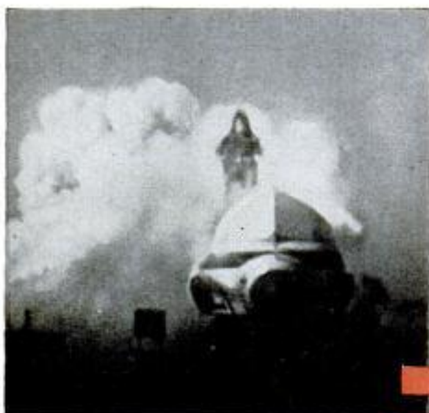
Billows of rocket smoke indicate the supersonic speed of this test sled in a sequence of front-view photos showing how a rocket attached to the ejection seat of lifelike dummy propels it from the sled's cockpit
