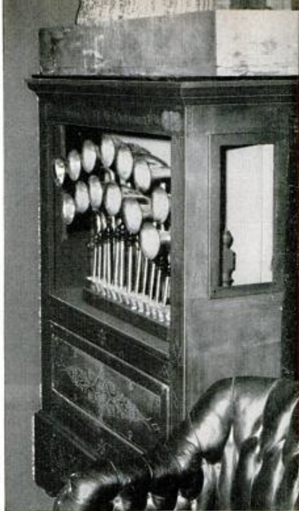
This is a DuKleist military-band organ used on a merry-go-round about 1898. It has to be hand-cranked. Note array of horns in the front opening
