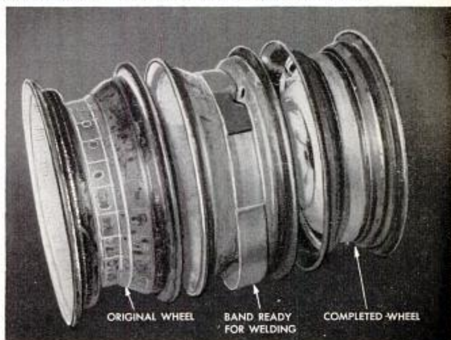
Above, three steps in forming the shot channel in the wheel. Below, automatic machine welds band to wheel in three minutes
