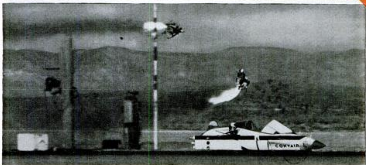
Two dummies are rocket-ejected from a simulated-airplane sled traveling faster than the speed of sound
