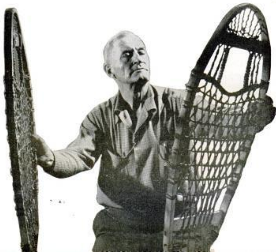
Top left, McKenney makes leather thongs by pulling circle of leather, cut from boot, against knife beside whittled wood block. Left and top right, he builds snowshoes in campus shop
