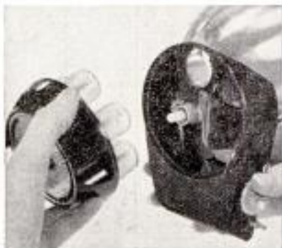
LOADED DISC OF BULBS is placed in magazine on the back of the flashholder. Bulbs are changed by simply rotating the magazine turret.
