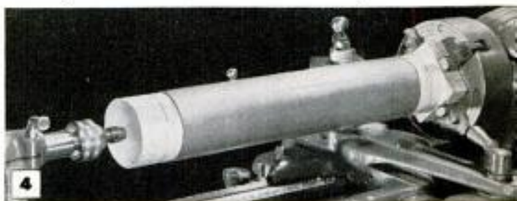
Above, hardwood turning is sawed apart to make two step centers. Below, tube mounted on step centers
