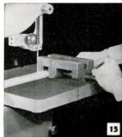
Above, work up to 2 in. in dia. can be held in this V-block with improvised clamp and a guide bar which rides in table groove. Below, three views picturing use of hand screw and drill-press vise as holders for tubing of large and small diameters. Fig. 13 shows handscrew used as clamp with sliding guide. Figs. 14 and 15 show hand screw and drill vise used freehand
