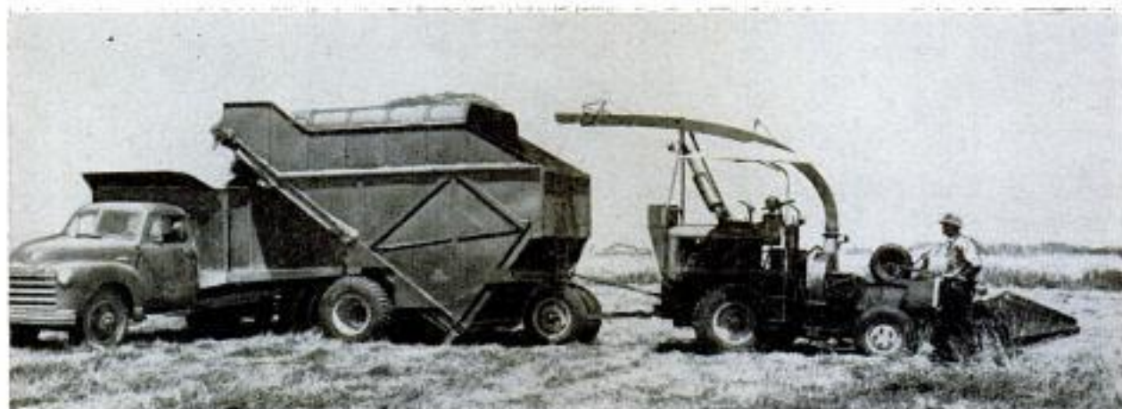
Harvesting unit moves through field until trailer is filled. Below, conveyor then unloads trailer into truck
