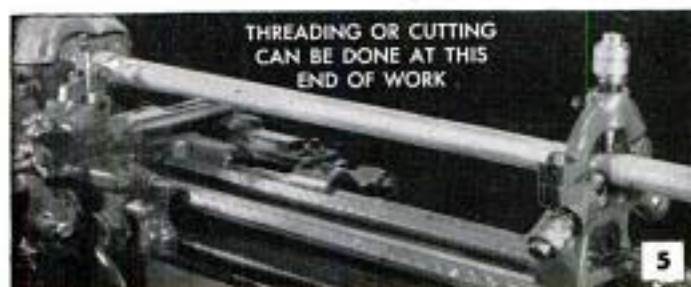
Above, end of long tube is supported in steady rest. Below, improvised rest supports large-diameter tubing
