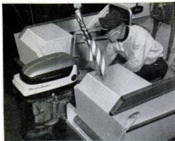
Pivoted hood swings down to provide convenient access to outboard motor. Evinrude 35 sent Sea Knight skimming along at 26 m.p.h. during the trial runs
