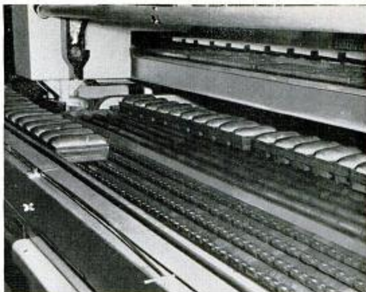
Above, baked loaves emerge from oven to conveyor system that takes them past air jet which loosens loaves for depanner
