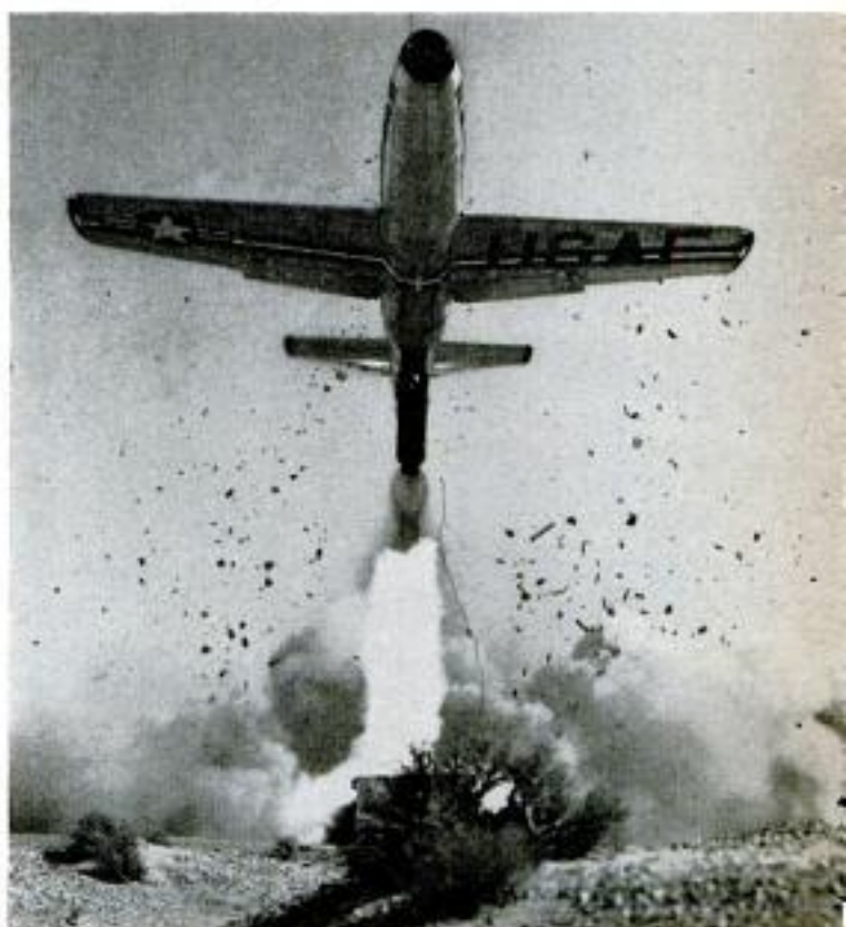
Sled's shock wave sometimes tosses trackside cameras 30 ft. although they're bolted down in metal boxes
