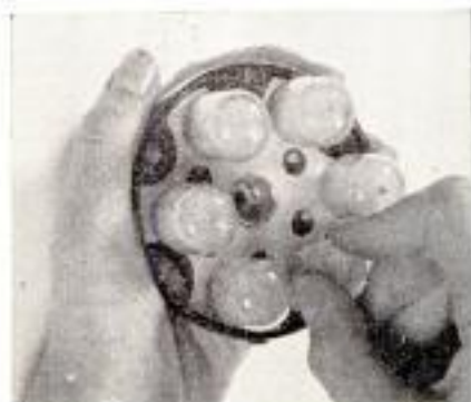
FAST, EASY LOADING. Six M2 flashbulbs are slipped into each of the two carrier discs that come with the Kodak Rotary Flashholder.
