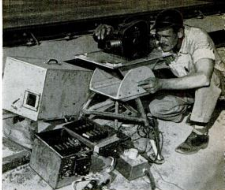
Sled's shock wave sometimes tosses trackside cameras 30 ft. although they're bolted down in metal boxes
