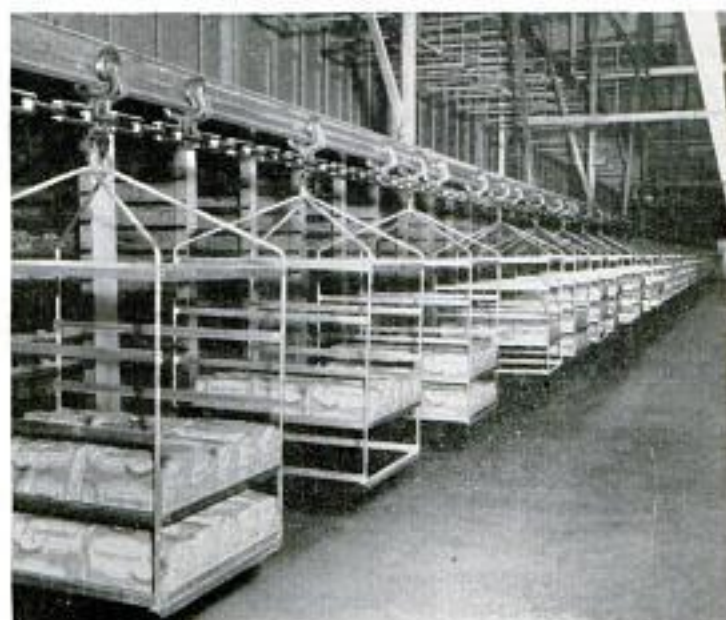
Below, after a trip through wrapping machine, which automatically slices, wraps and seals them in cellophane, the finished loaves are taken by conveyor system to the shipping room
