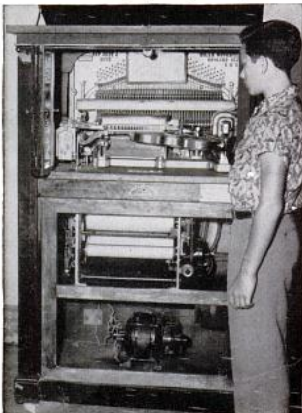
Remarkable Violano Virtuoso plays violin-piano duets with steel fingers plucking melody on violin
