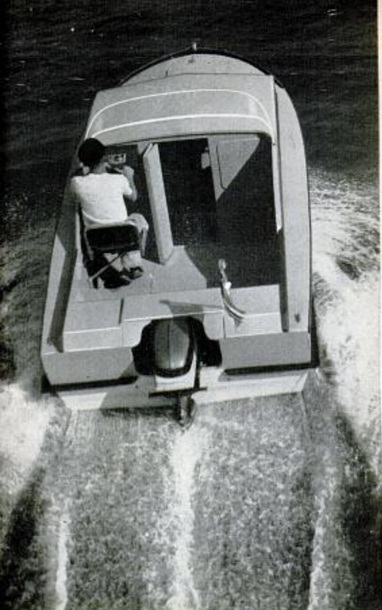
Pivoted hood swings down to provide convenient access to outboard motor. Evinrude 35 sent Sea Knight skimming along at 26 m.p.h. during the trial runs
