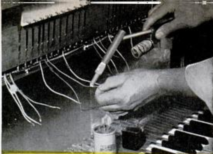
Above, Sommer solders connection to choke unit in the organ-stop circuit. Plastic stops at top operate "roll" switches similar to those actuated by keys. Keyboard from piano shows shortened black keys
