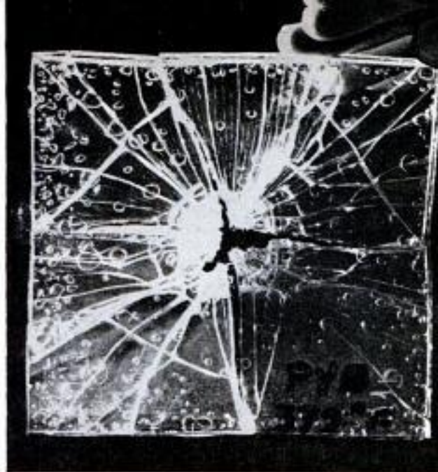
Windshield glass with older plastic interlayers at 375 degrees F. shatters when hit by foreign matter
