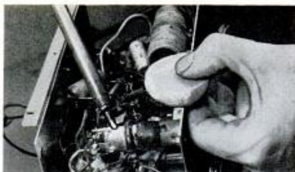
Beeswax, a nonconductor of electricity, forms protective coating over receiver-coil windings, holds wires in place and seals other radio parts
