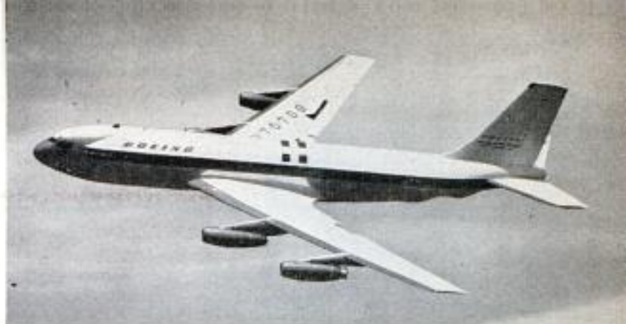
This 707 prototype has only a dozen windows while the passenger model will have more window area than any other plane
