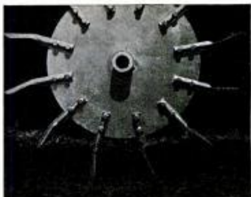
Soil ventilator "spoons" slice into dirt and lifts out earth for deep fertilization
