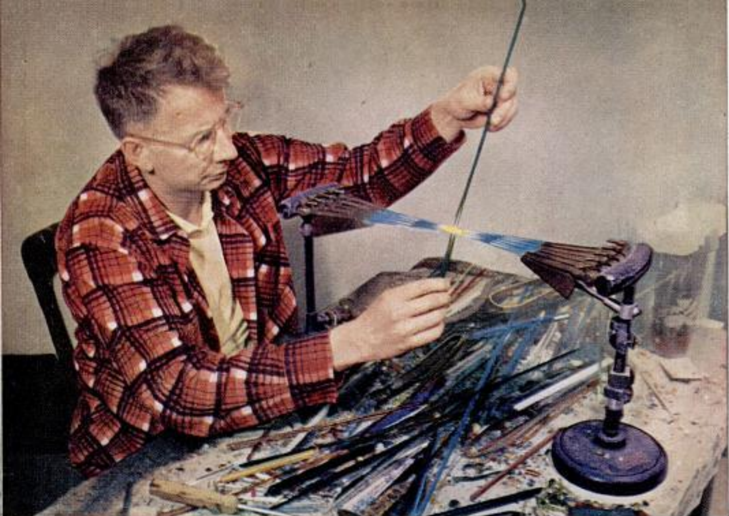
Above, Johnson begins work on a striped fish by heating a green rod to form the first stripe, No. 1 below
