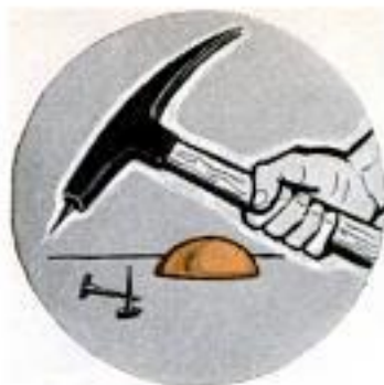
Left, small tack is easy to start with wax-coated hammer. Right, beeswax is good medium for statue-model carving
