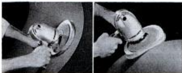
Cushion-type resilient pad sands with smooth, even pressure on contour or flat surfaces without leaving swirl marks.
