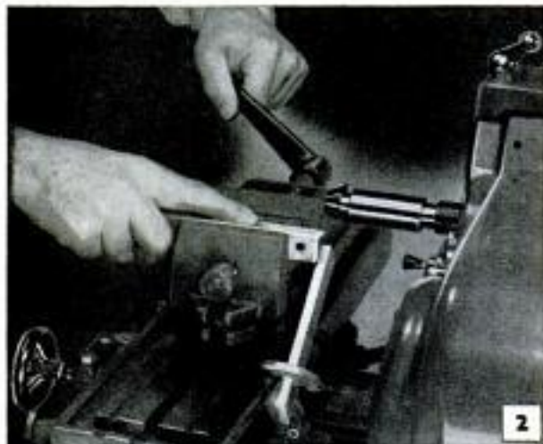
Chamfer is most common cut made with angular cutter. Stop clamped to machine table assures accuracy
