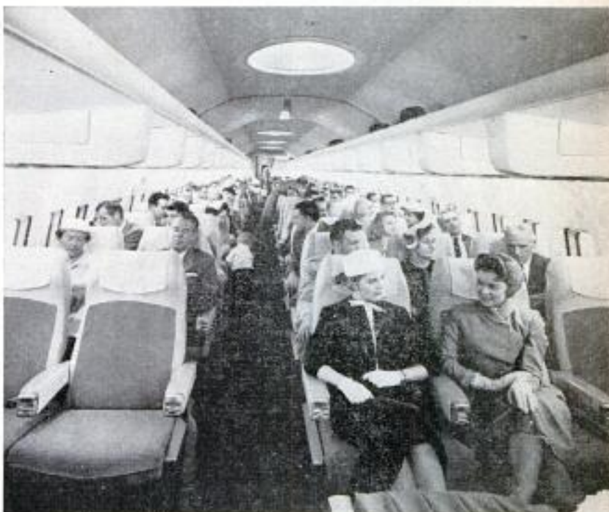
Mock-up cabin shows first-class seating for 131 passengers. Tourist version with three seats on each side will carry 162
