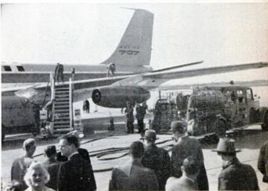
Huge tanks hold 12,000 gallons of fuel. Using 1800 gallons an hour, plane can span the nation and still have plenty left
