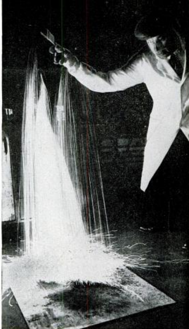
Purified manganese-bismuth, a material for making supermagnets, bursts into fiery waterfall when scattered in air. Because it catches fire spontaneously, it must be prepared in atmosphere of helium. Below, sample of it is weighed in a gas chamber
