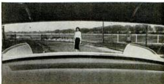
Above, there's the view the driver gets when backing up. Tailfins act as reference points for close maneuvering
