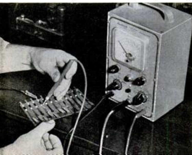
Sommer prepares to test a group of "roll" switches used in conjunction with the organ's keys and stops
