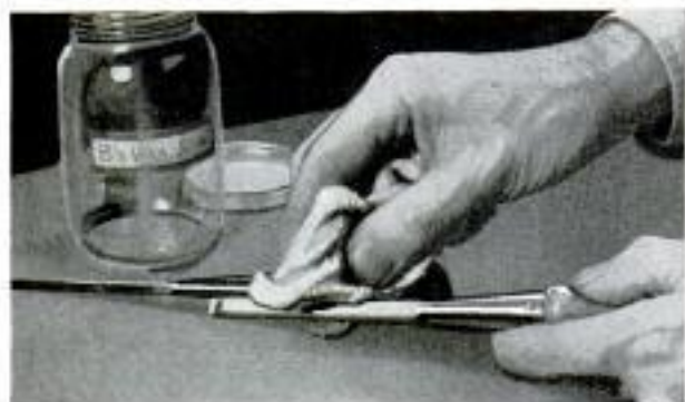
Above, cloth saturated with mixture of wax and turpentine is used for coating metal surfaces of cutting tools to protect them from corrosion
