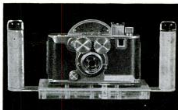
Above, after brass gears are silver-soldered to appropriate fittings for film advance and speed controls, the latter two are installed in place of knobs
