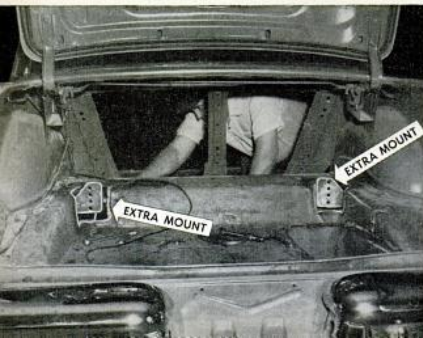
Nonessentials are stripped from the trunk of highly tuned race cars. Additional mounts are needed for the beefed-up suspension
