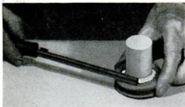
Above, cardboard tube "soldered" to wooden disk with beeswax, using heated steel rod to melt the wax, demonstrates its usefulness as an adhesive
