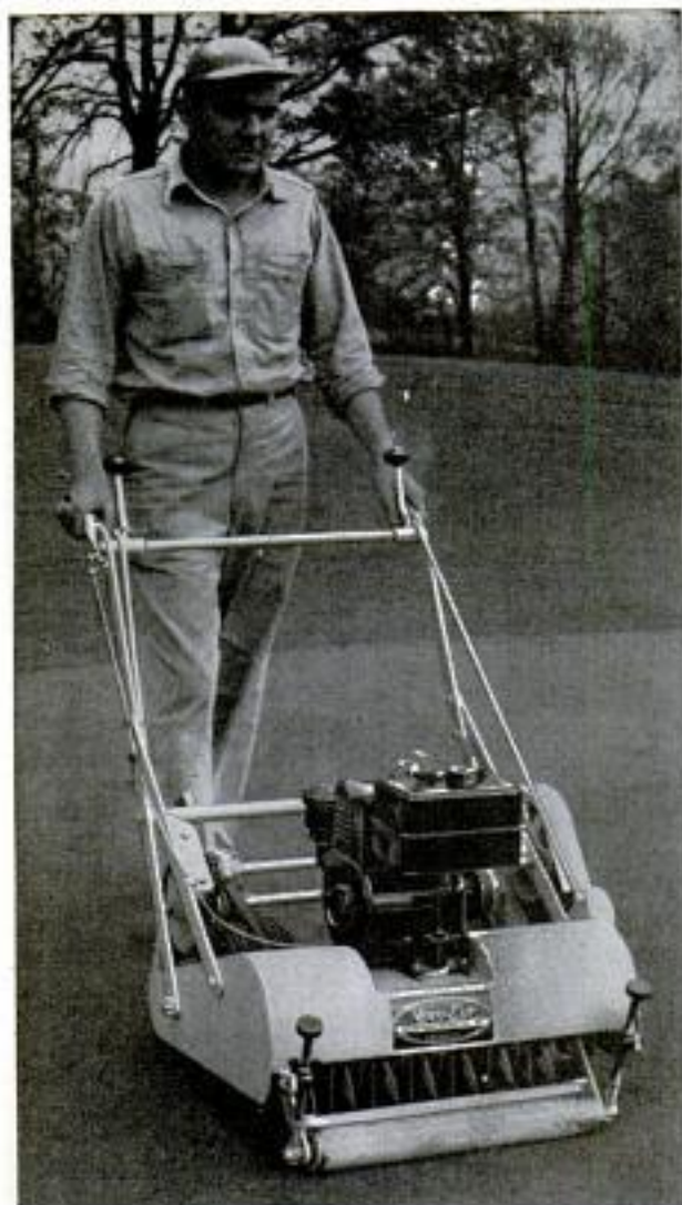
Verti-Cut unit slices into turf and trims runners and outspread leaves to get better putting green
