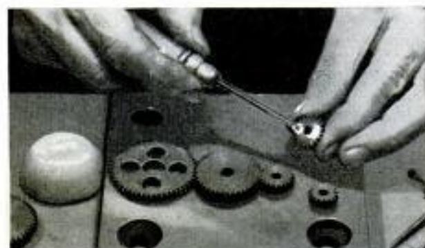
Above, wax holds small gears on steel plate temporarily while precise arrangement of gear train is developed. Below, wax lubricates closet-door latch
