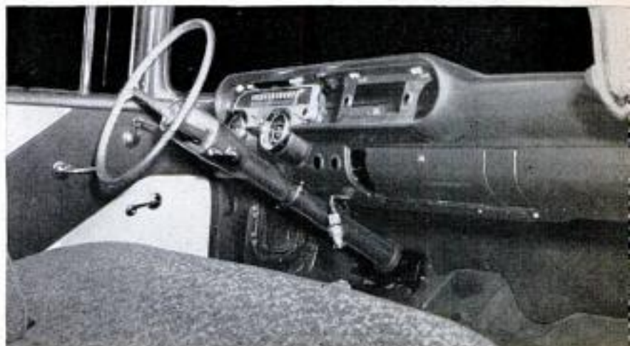
There's nothing fancy about the dash of a Pontiac when it's ready for the race. Everything unnecessary has been removed
