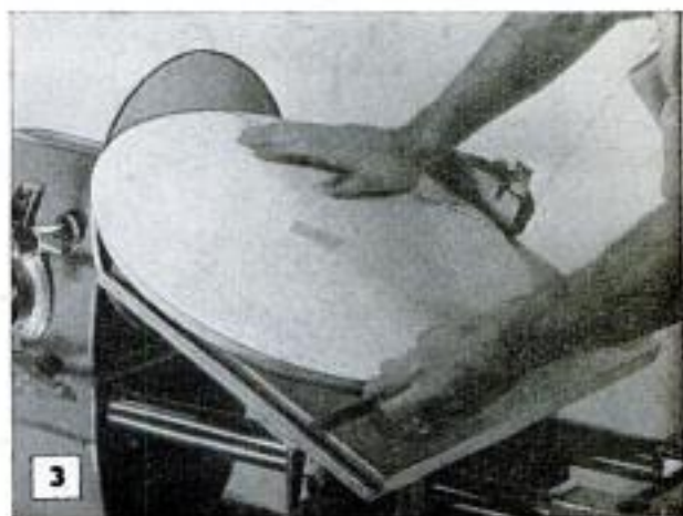
Accurate sanding of 30-deg. bevel on round top is accomplished by "pivot sanding" it on disk sander
