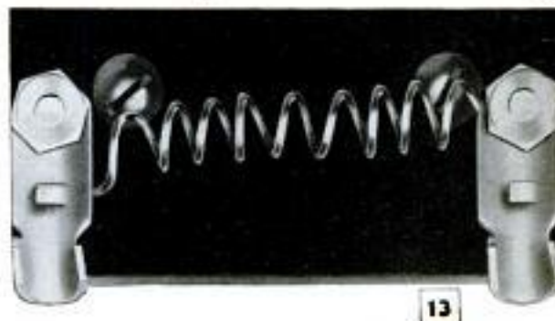
Above, tight wheel bearings are essential on trailer equipped with electric brakes. Below, resistor in circuit between battery and hand control reduces voltage
