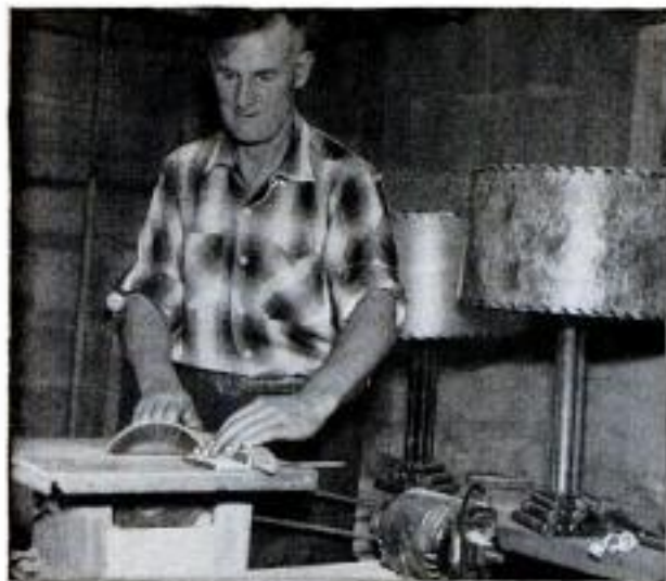
Diamond-impregnated blade works off 1/2-hp. motor
