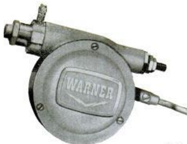
HYDRAULIC ADAPTER (TO ELEC. BRAKE CONTROLLER)
