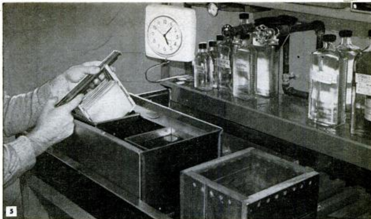
Fig. 5. Place loaded film hanger in empty tank. Repeat with successive hangers, using hand as spacer to prevent scratching film. Later, transfer entire group to developing tank at once. If fast-acting developer (3 to 5 min.) is used, stay with films until timer rings, immerse them in water 2 min., hardener-hypo bath 10 min., and water wash 30 min.
