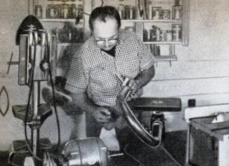
Jigsaw of the type having a swiveling arm, or gooseneck, requires an arm support attached to bench top
