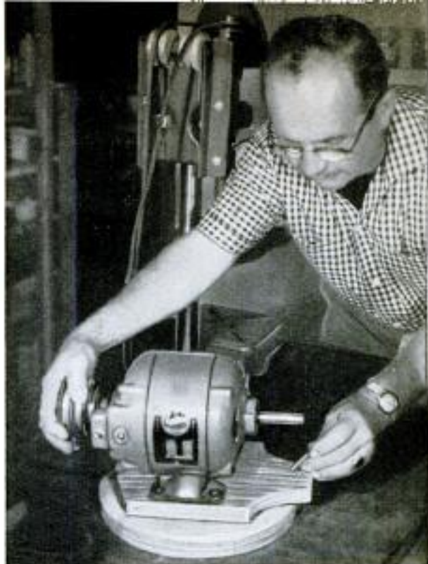
Swiveling base, or turntable, permits the motor to be positioned to drive any one of the four machines
