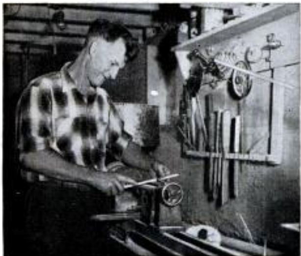
Lathe and soft polisher put bright finish on a core
