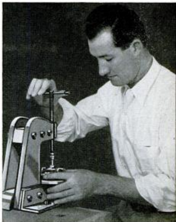
This arbor press is what would rate as small bench size and has a screw-type ram. Although slower than rack-and-pinion type, ram is more sensitive to pressure
