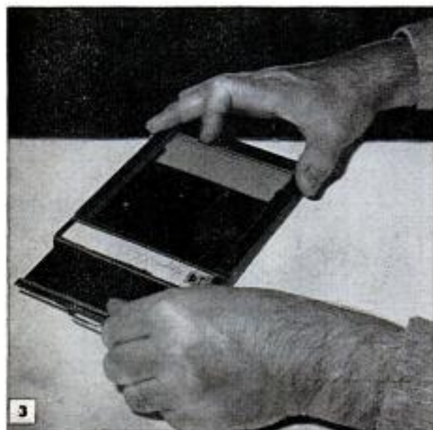
Fig. 3. When removing film, anchor holder to table by pressing along bottom edge with right hand. Draw out slide about 2 in. with left hand and remove film, being careful not to touch emulsion with fingers
