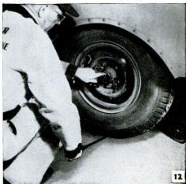
Above, tight wheel bearings are essential on trailer equipped with electric brakes. Below, resistor in circuit between battery and hand control reduces voltage
