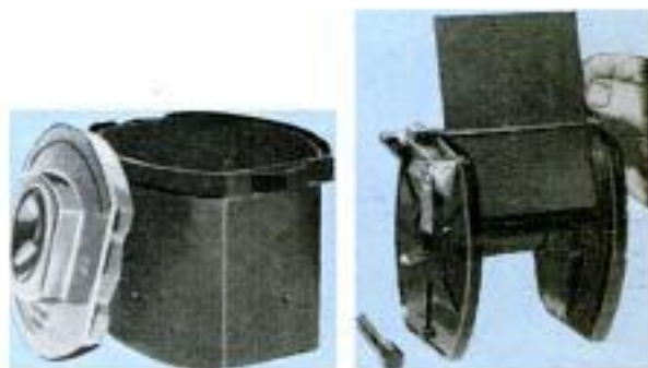
Fig. 6. Daylight tank permits processing sheet film outside of darkroom. After loading grooved reel with exposed film in total darkness, place reel in tank, secure lid, fill with developer and agitate with rod
