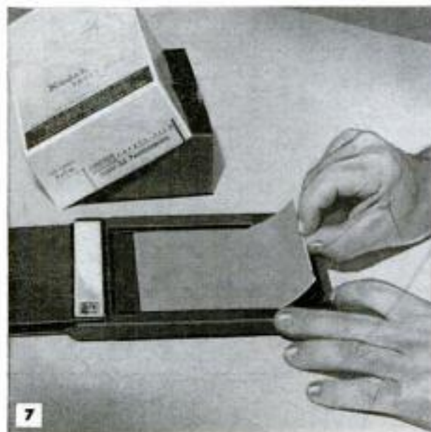
Fig. 7. Before loading film, insert slides \frac{1}{2} in. into holder. In darkroom open bottom flap and slide film in guides with notches in upper-right corner, emulsion side up. Fig. 8, after film is inserted, press end flap down and push slide in until flap is engaged. Then turn locking pin to closed position to prevent slide from being pulled out of flap accidentally
