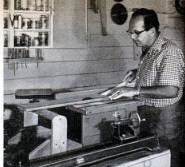
Stock support for the circular saw permits ripping long boards. Need not be removed after attaching
