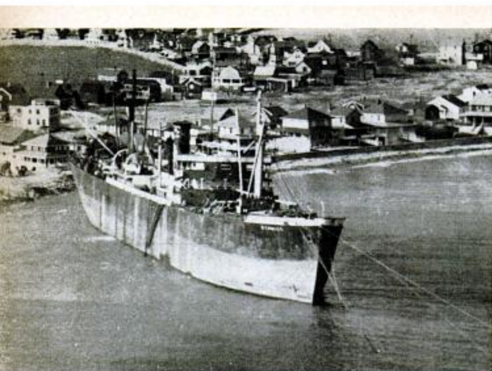
Kedge anchors were laid in deep water offshore. Heavy cables then were attached to the ship's winches so the freighter could pull herself free
