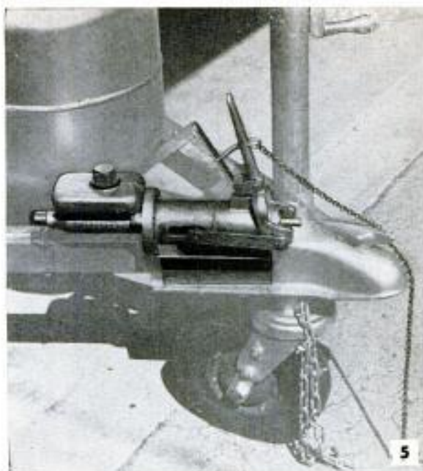
Above, hydraulic cylinder mounted on trailer drawbar. Below, breakaway switch sets brakes on trailer Courtesy Warner Electric Brake & Clutch Co.
