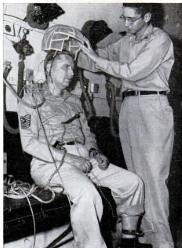
Electrical leads are attached to body of airman in altitude chamber. They report changes during test
