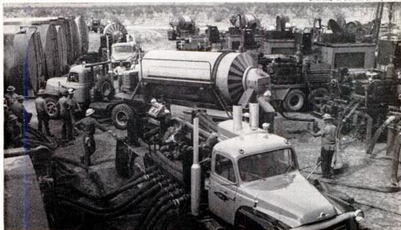
Intake hoses carry water to truck for blending with sand. Mixture goes to high-pressure pump trucks for transfer to oil well
