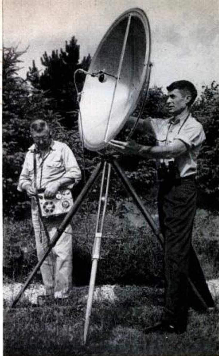
Prof. Carl Reese (left) carries battery-operated tape recorder, as Prof. Donald Berror adjusts parabolic reflector
