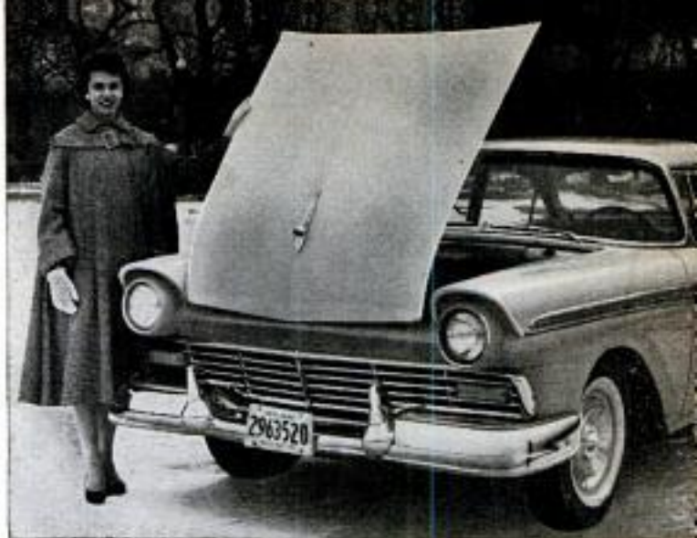
Owners praise front-hinged hood for safety and engine accessibility; others say it's hard to close
