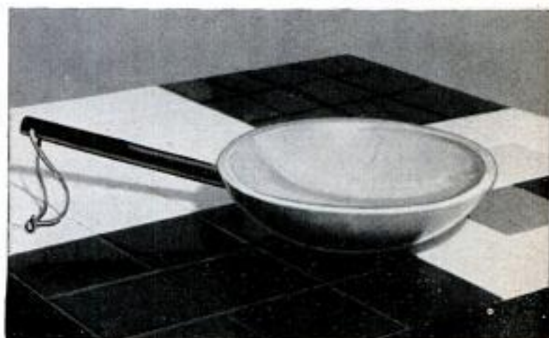
Above, for snack server, glue 8-in. length of \frac{3}{8} -in. dowel in hole drilled in bowl, add leather thong. Below, wheelbarrow fruit bowl is made from four lengths of \frac{3}{8} -in. dowel and 3-in.-dia. wooden wheel
