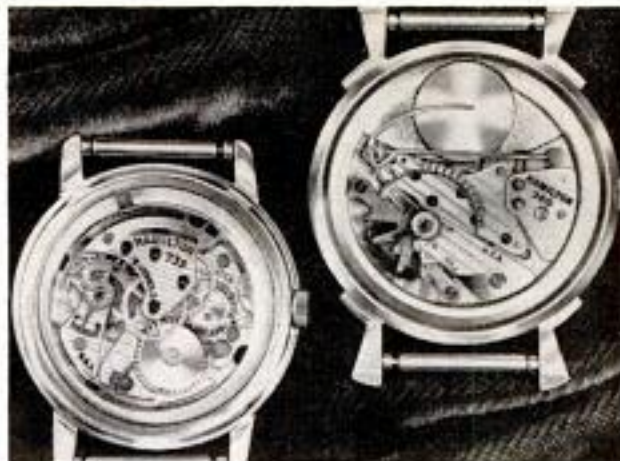
Manually wound watch is at left. Electric watch is at right, with energizer in circle at top center
