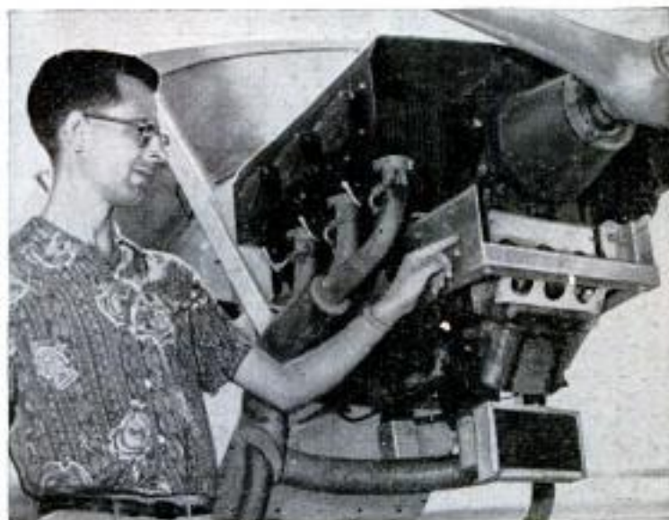
Above, the aircraft's controls are set between the rigid channels of bolted, twin, six-inch aluminum metal pieces. Below, the "girder's" creator, William Marlman, points to the box fuselage
