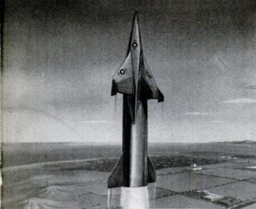
Shuttle craft would transport personnel to satellite at 600-mile altitude. Lower rocket portion detaches after take-off
