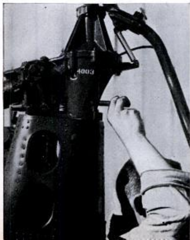
Pilot reaches just above head to pull small lever which brakes rotor for quick slowdown of machine
