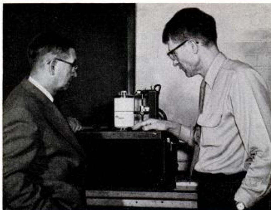
Audiospectrograph makes a chart of a bird's song, which later will be analyzed as part of this research project at Ohio State University
