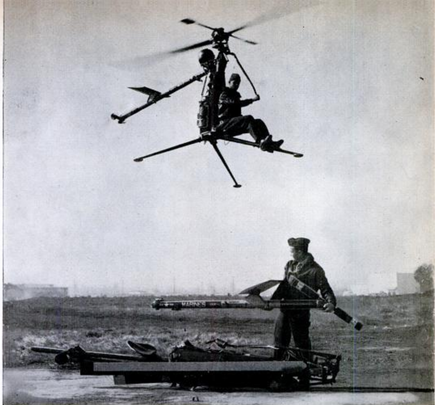
Hiller's one-man helicopter is designed to be collapsed into compact unit for easy transportation or air drop
