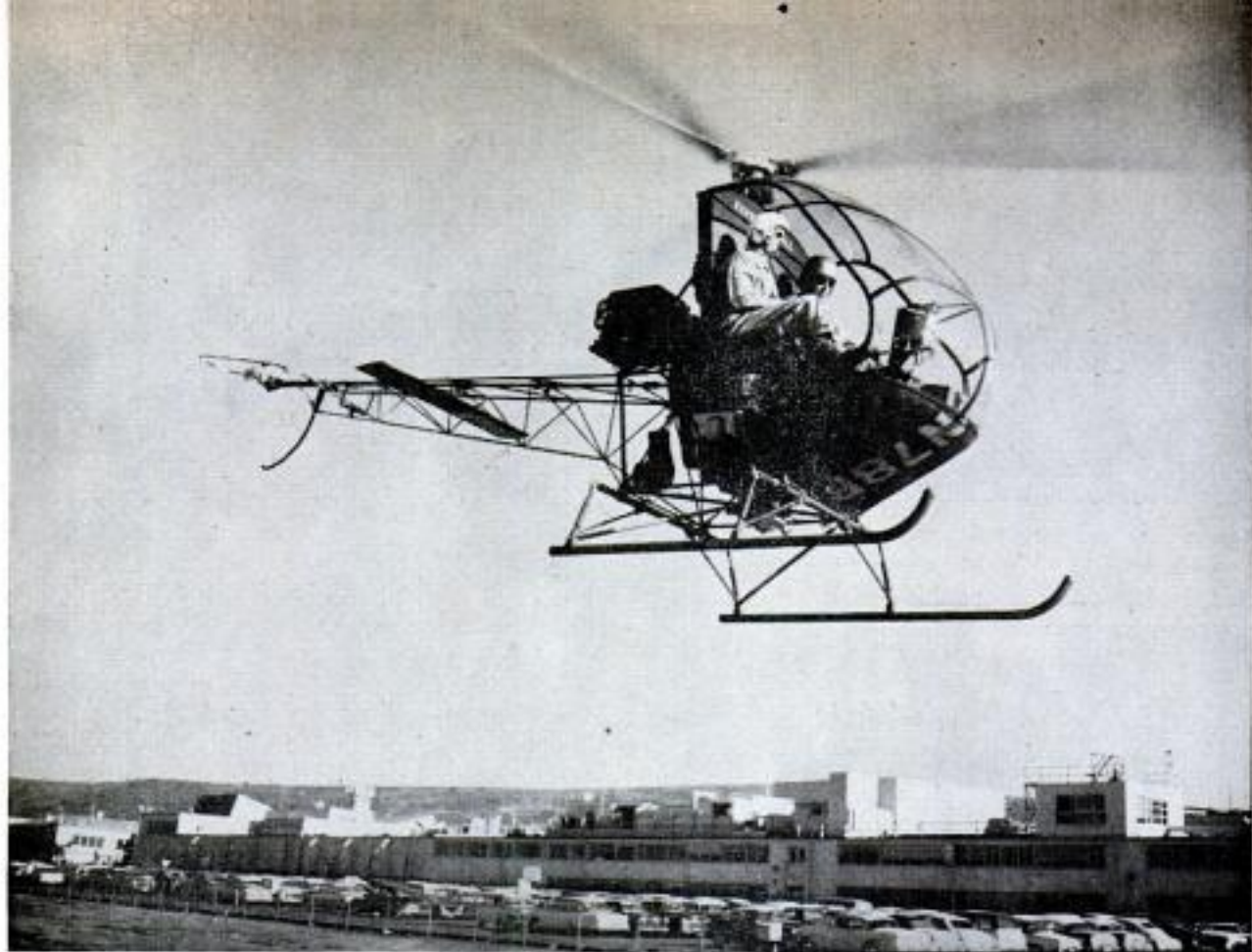
Hughes' two-man copter is 8½ feet high, 19 feet 5 inches long, and can climb at rate of 1400 feet per minute
