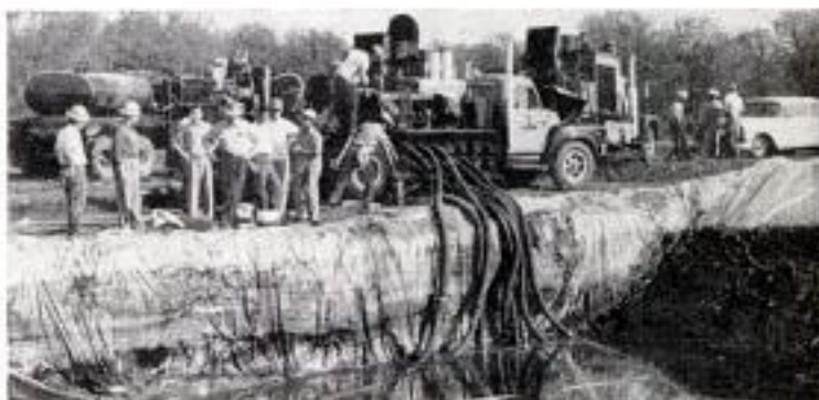
Intake hoses carry water to truck for blending with sand. Mixture goes to high-pressure pump trucks for transfer to oil well
