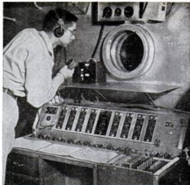
Machine outside the altitude chamber records effects of altitude on brain waves of the subject inside
