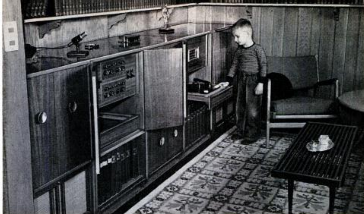
Radio, phonograph, tape and microphone sound are piped from this music panel to main and tenant houses
