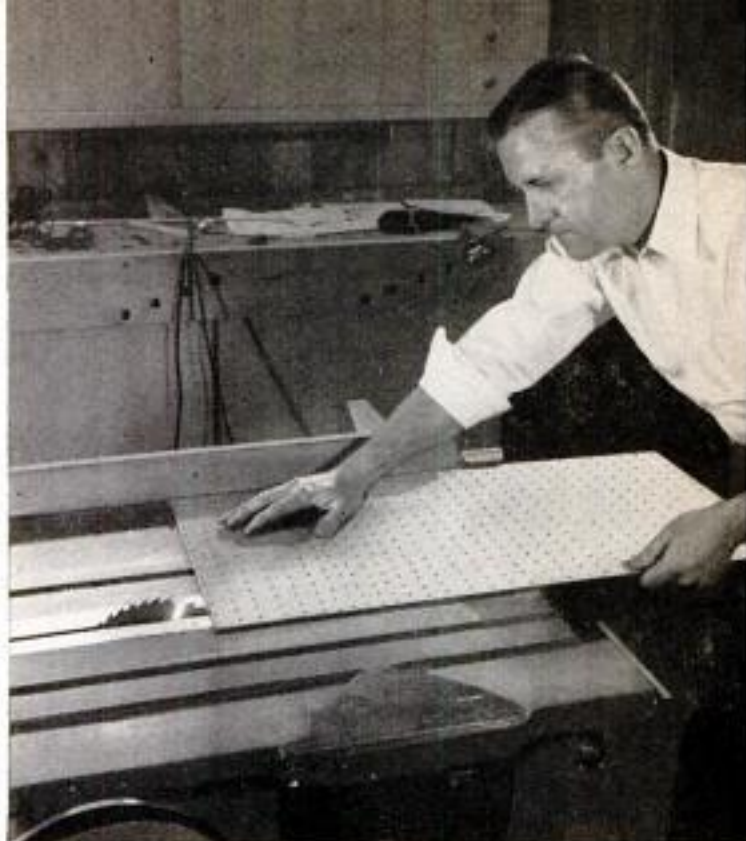
Perforated hardboard for the doors is both decorative and practical as it ventilates the interior. Saw the material slowly to avoid chipping the edges
