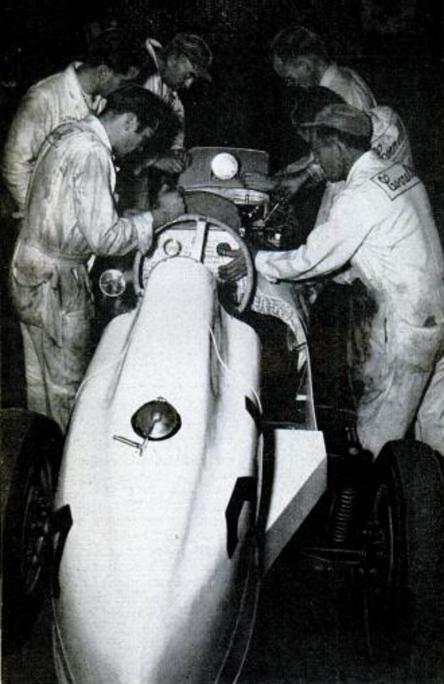
Above, four-wheel-drive racing car driven by Milliken has its tachometer mounted over the engine so driver can read it without lowering his eyes dangerously. Below, another of his cars is filled with special instrumentation to measure its stability
