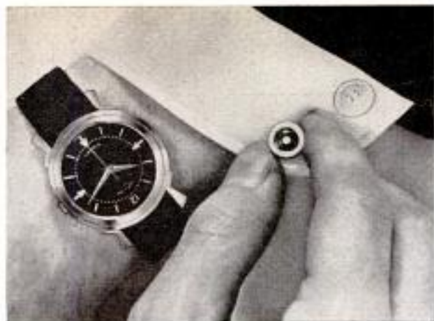
Electric wrist watch receives its power from energizer that is no bigger than the button on a shirt
